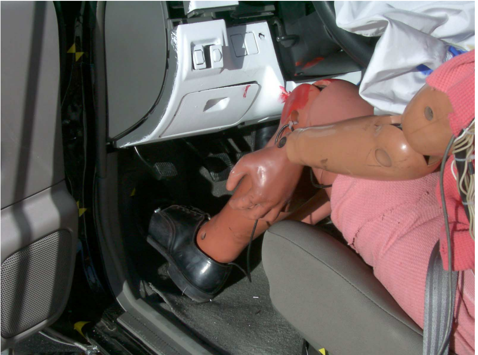
Figure A-34: Driver Dummy Feet and Knee Contact, Post-Test (Correct NHTSA #M25204)
