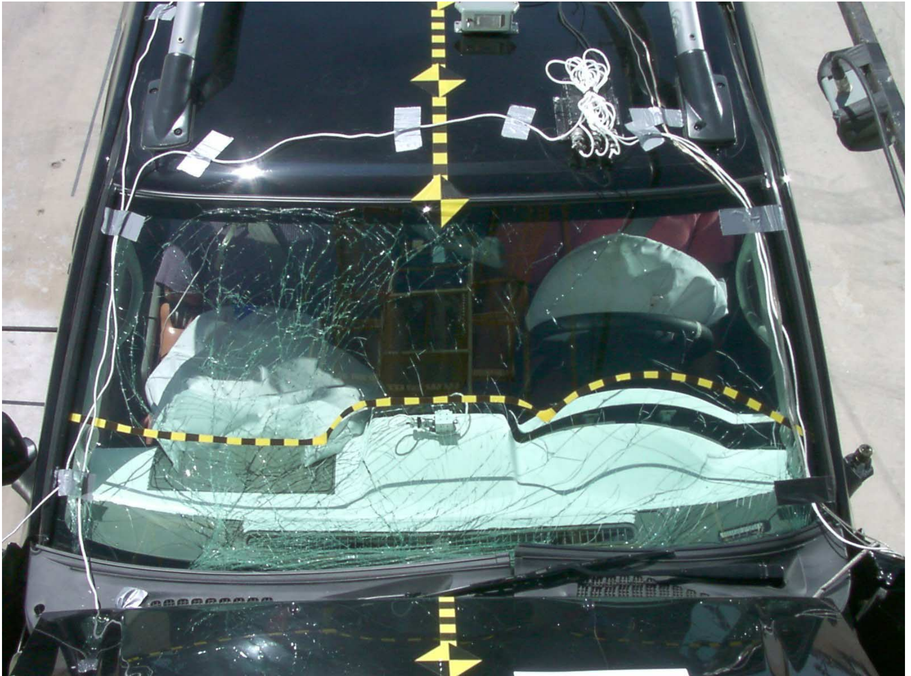
Figure A-16: Windshield, Post-Test (Correct NHTSA #M25204)
