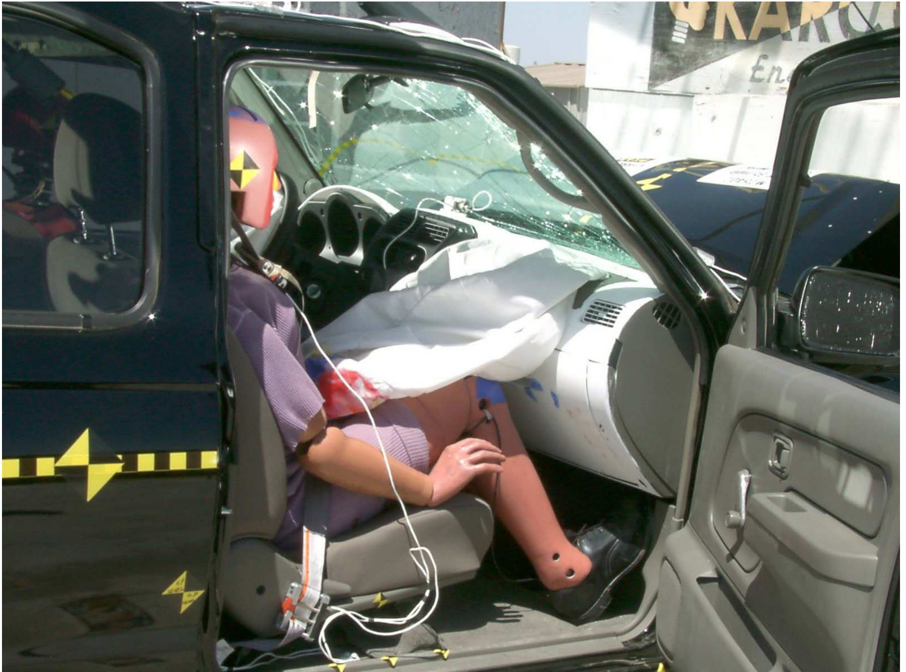
Figure A-46: Passenger Dummy Door Open, Post-Test (Correct NHTSA #M25204)
