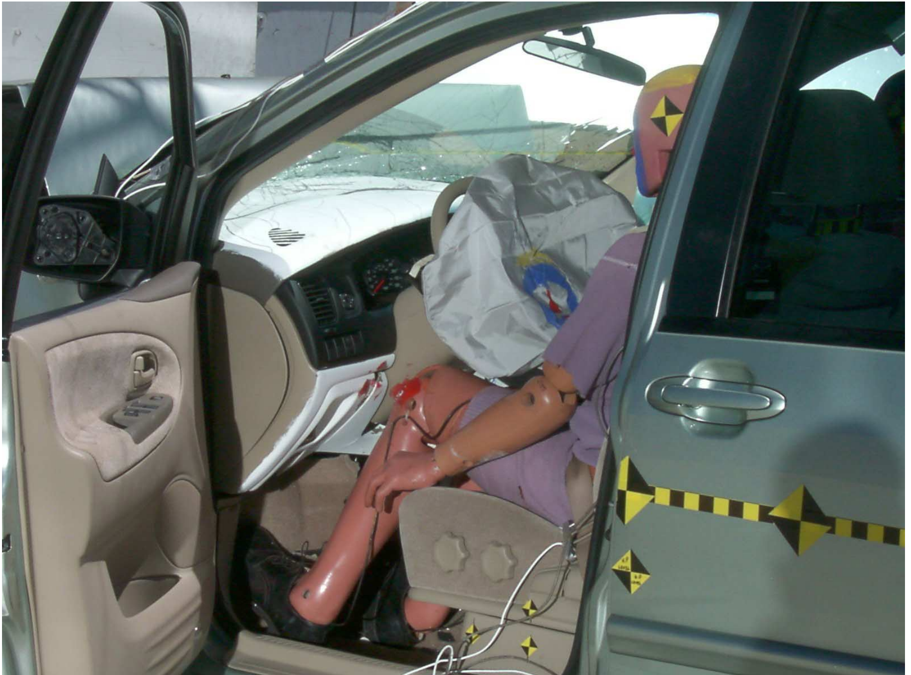
Figure A-30: Driver Dummy Door Open, Post-Test
