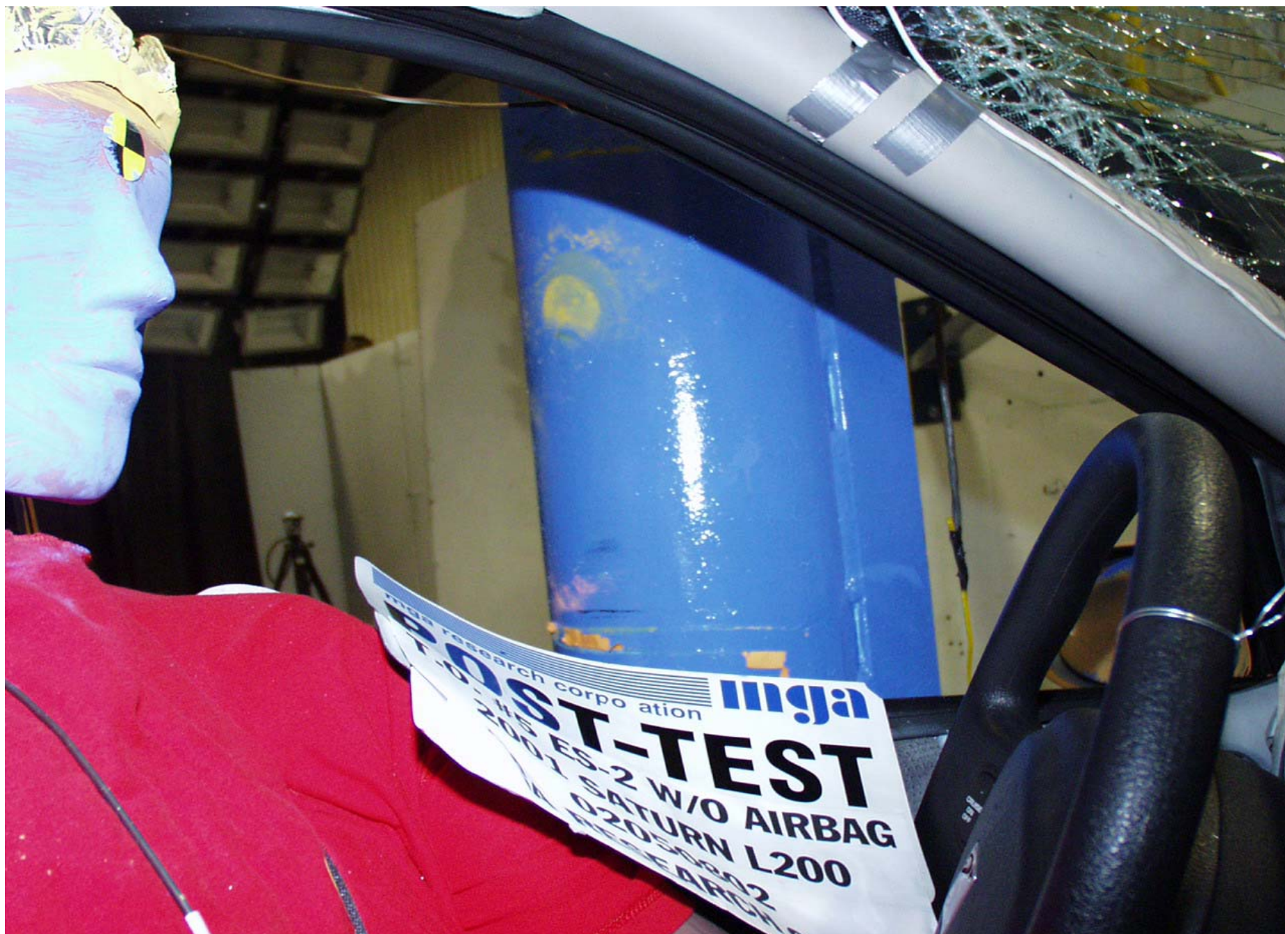
Post-Test Driver Dummy Head Contact with Pole
