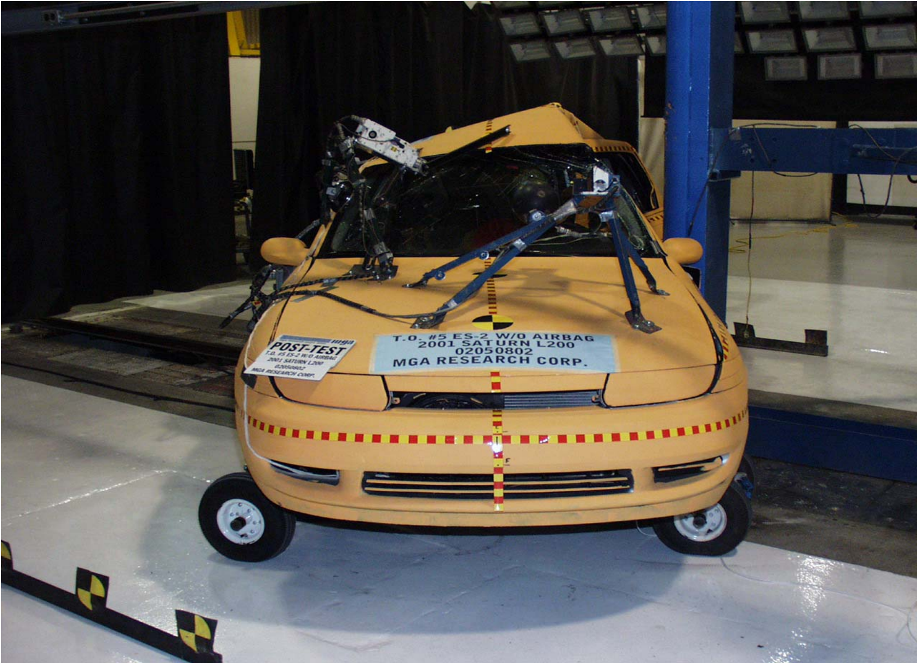
Post-Test Front View of Test Vehicle
