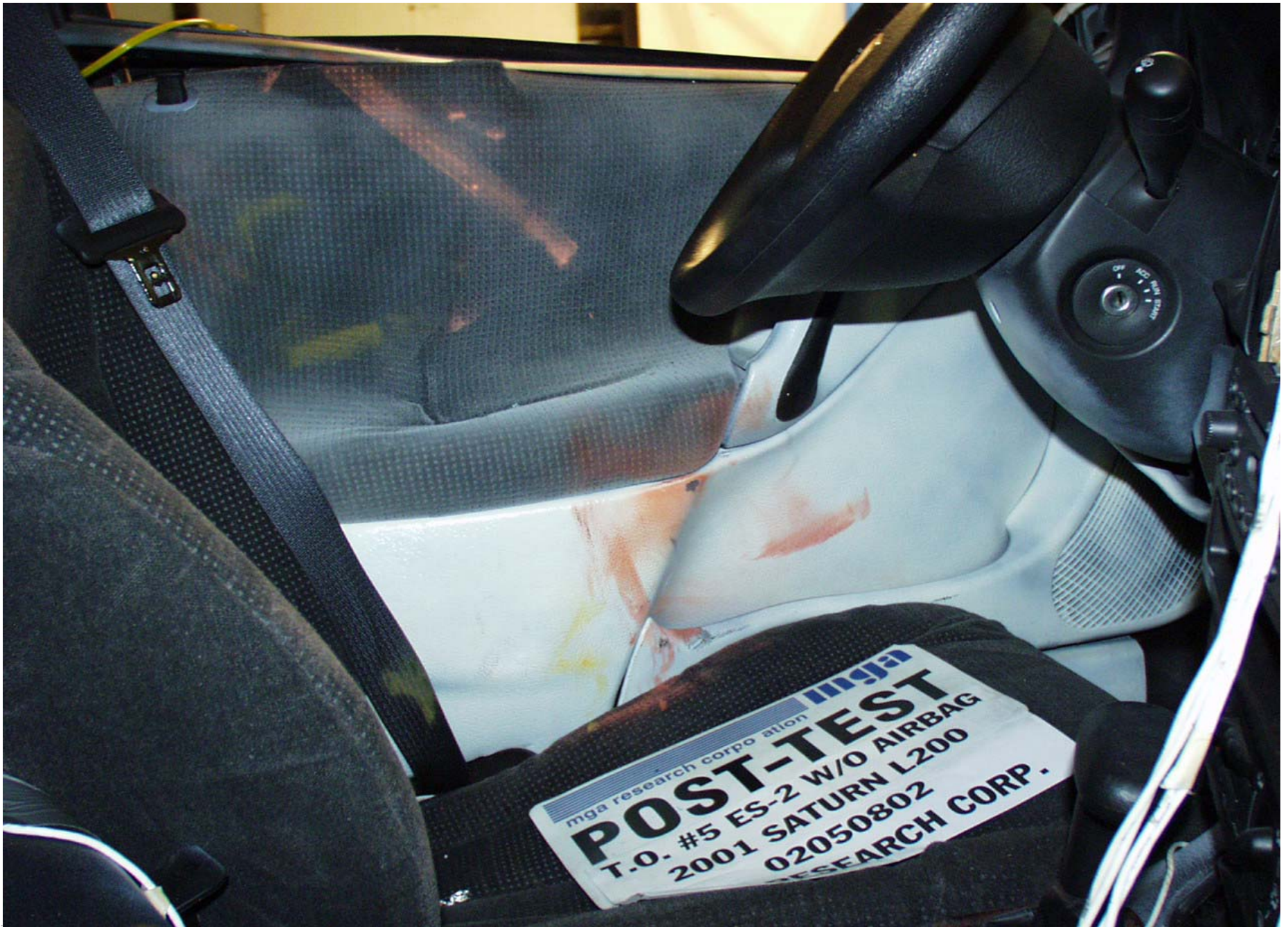
Post-Test Driver Dummy Contact
