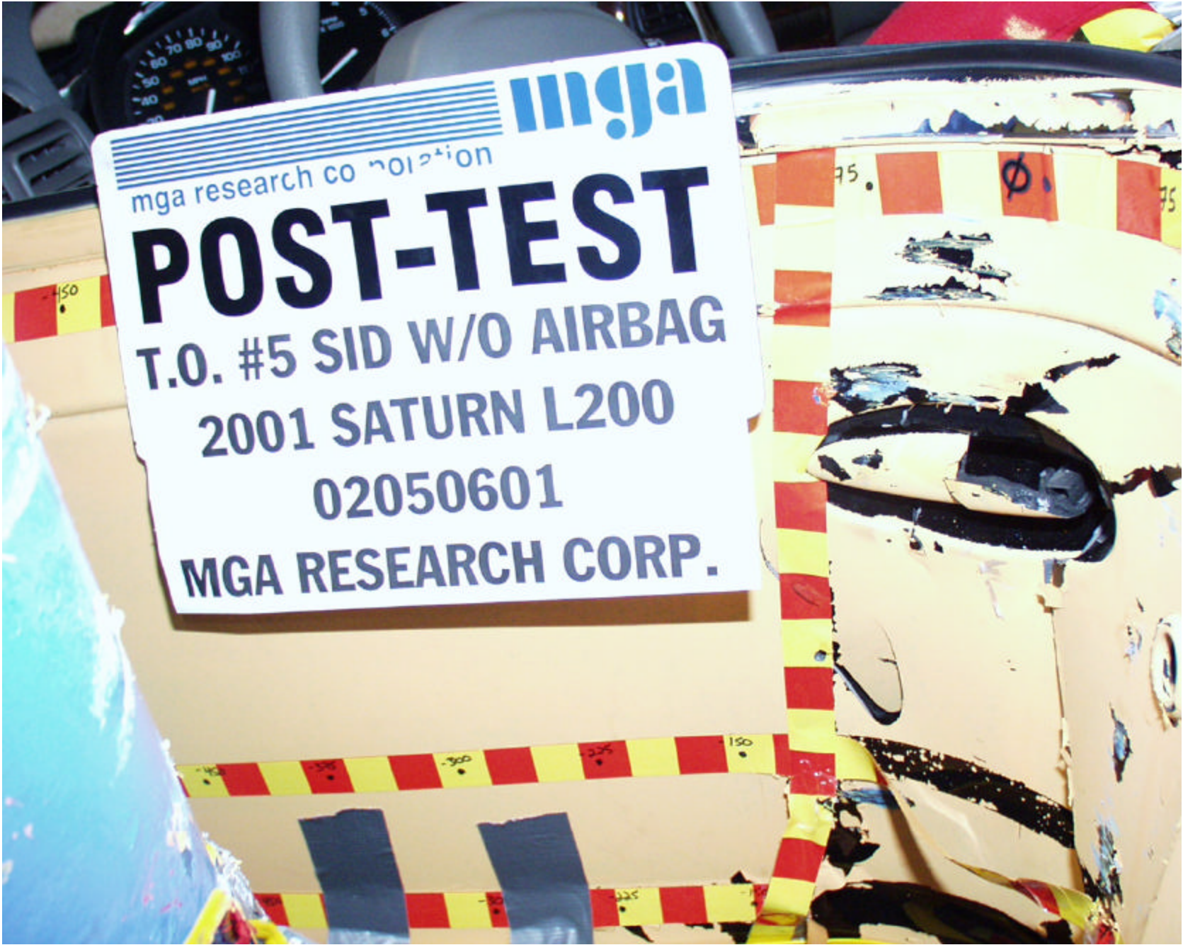
Photo No. A-27 - Post-Test Impact Point on Test Vehicle
