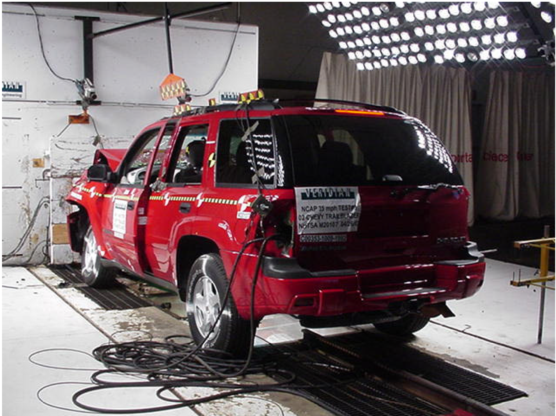
Figure A-11 POST-TEST LEFT REAR THREE-QUARTER VIEW (Door remained closed and latched during the event – Opened by technicians prior to photograph)
