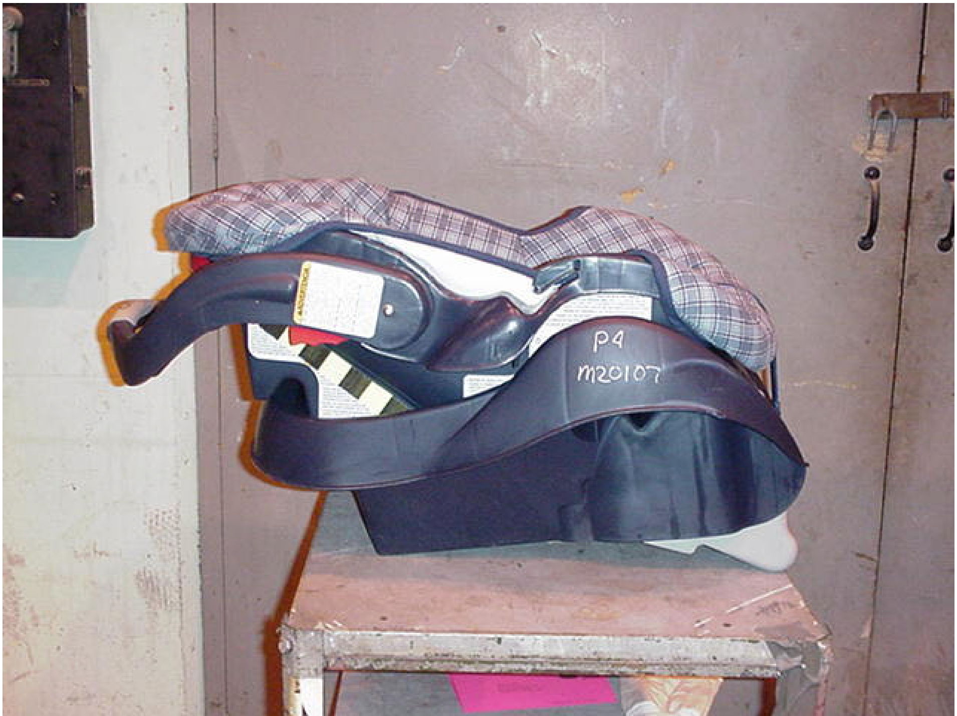
Figure 3-18 POST-TEST RIGHT SIDE VIEW OF POSITION 4 CRS
