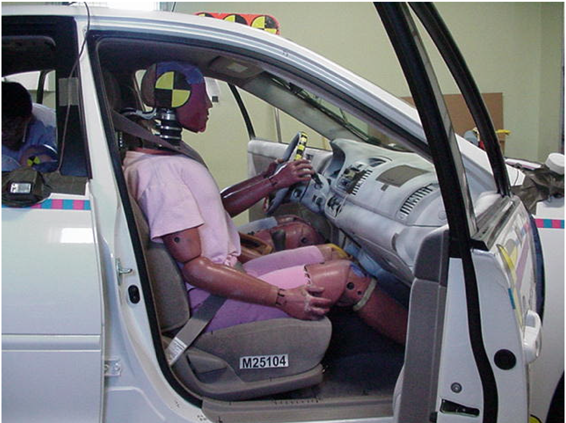
Figure A-24 PRE-TEST PASSENGER POSITION VIEW
