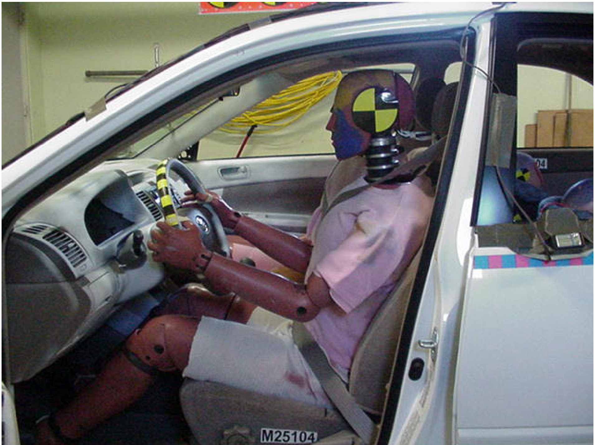
Figure A-22 PRE-TEST DRIVER POSITION VIEW
