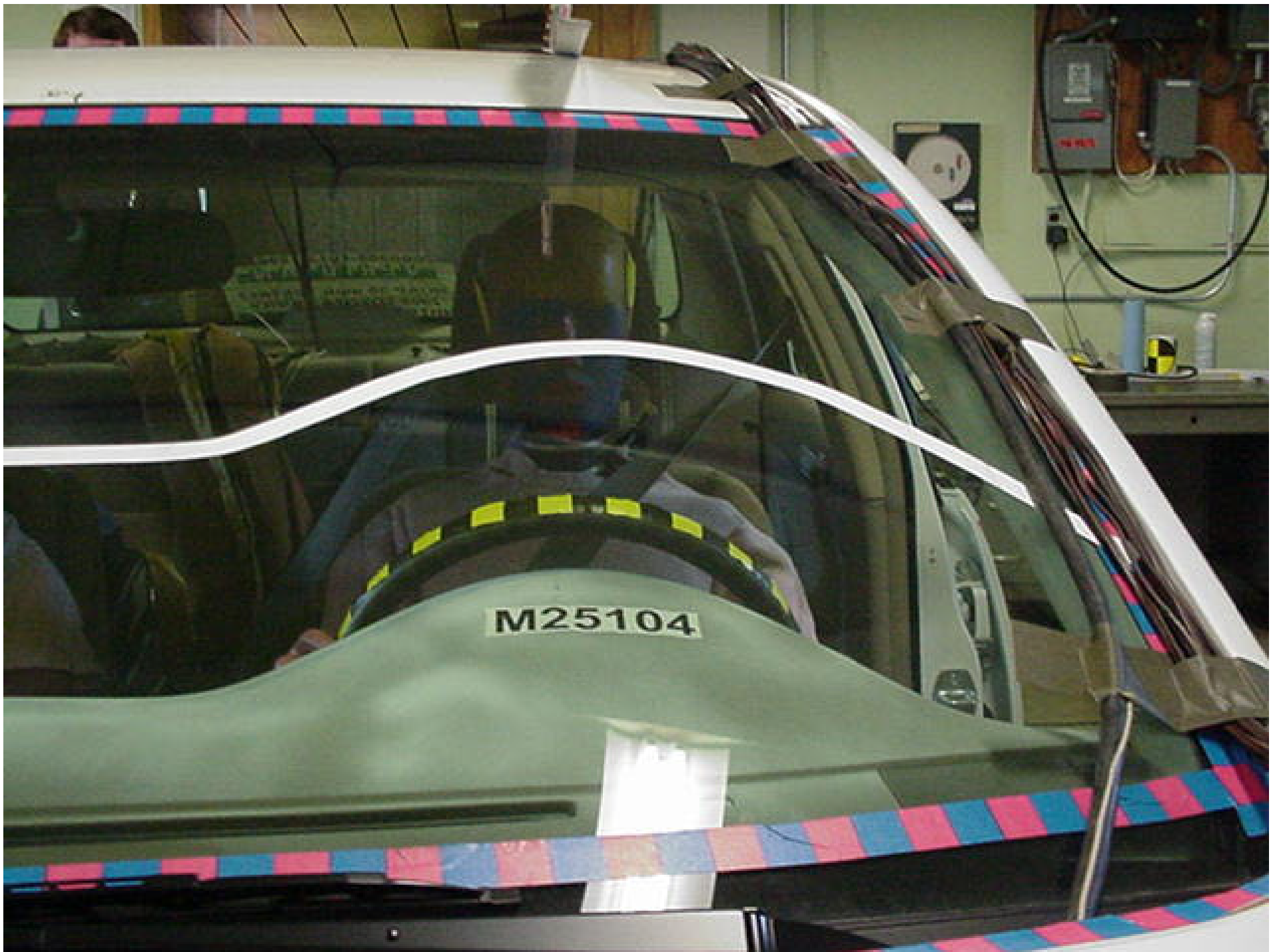
Figure A-30 PRE-TEST DRIVER HEAD LOCATION
