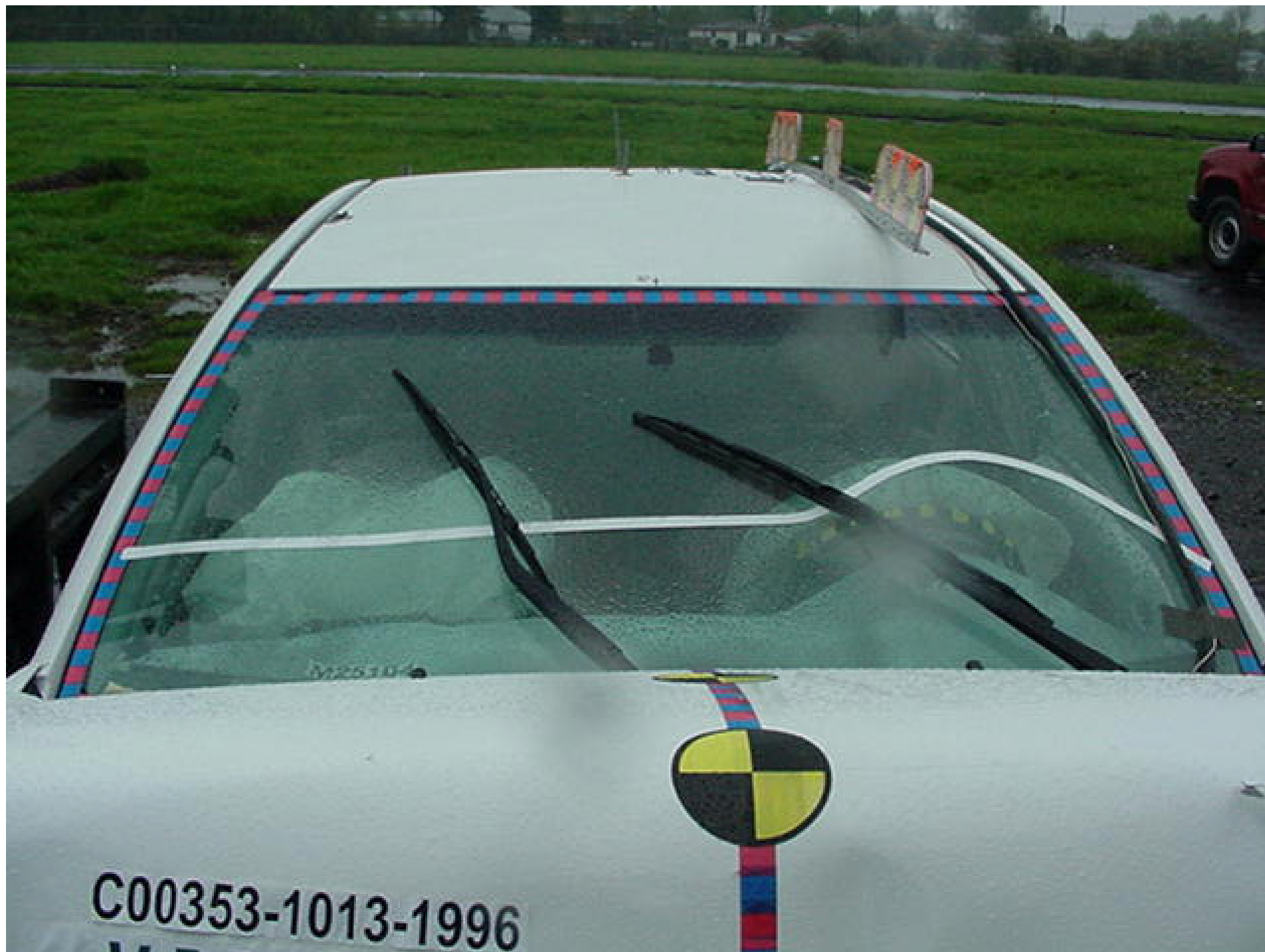
Figure A-13 POST-TEST WINDSHIELD VIEW
