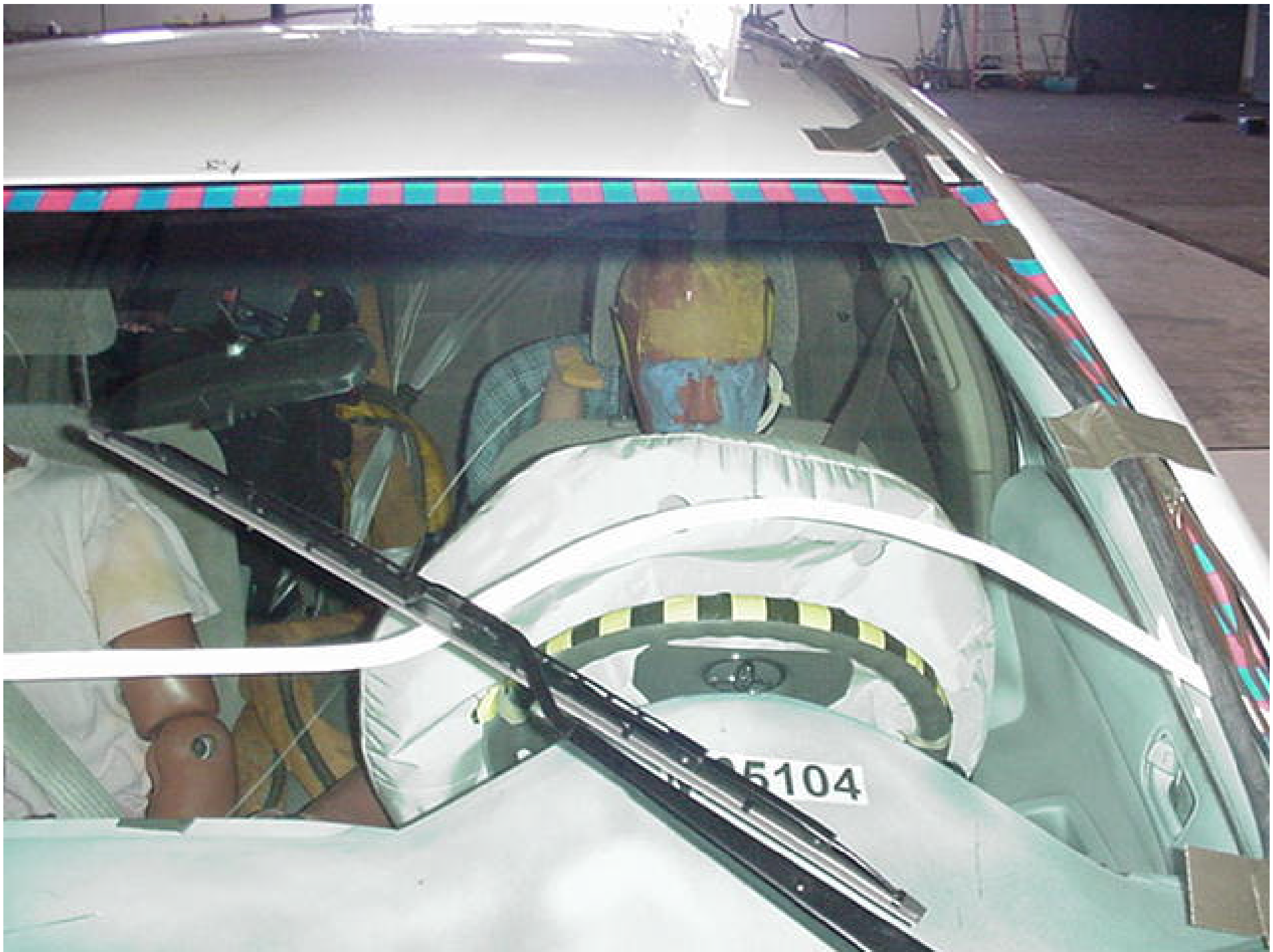
Figure A-31 POST-TEST DRIVER HEAD LOCATION
