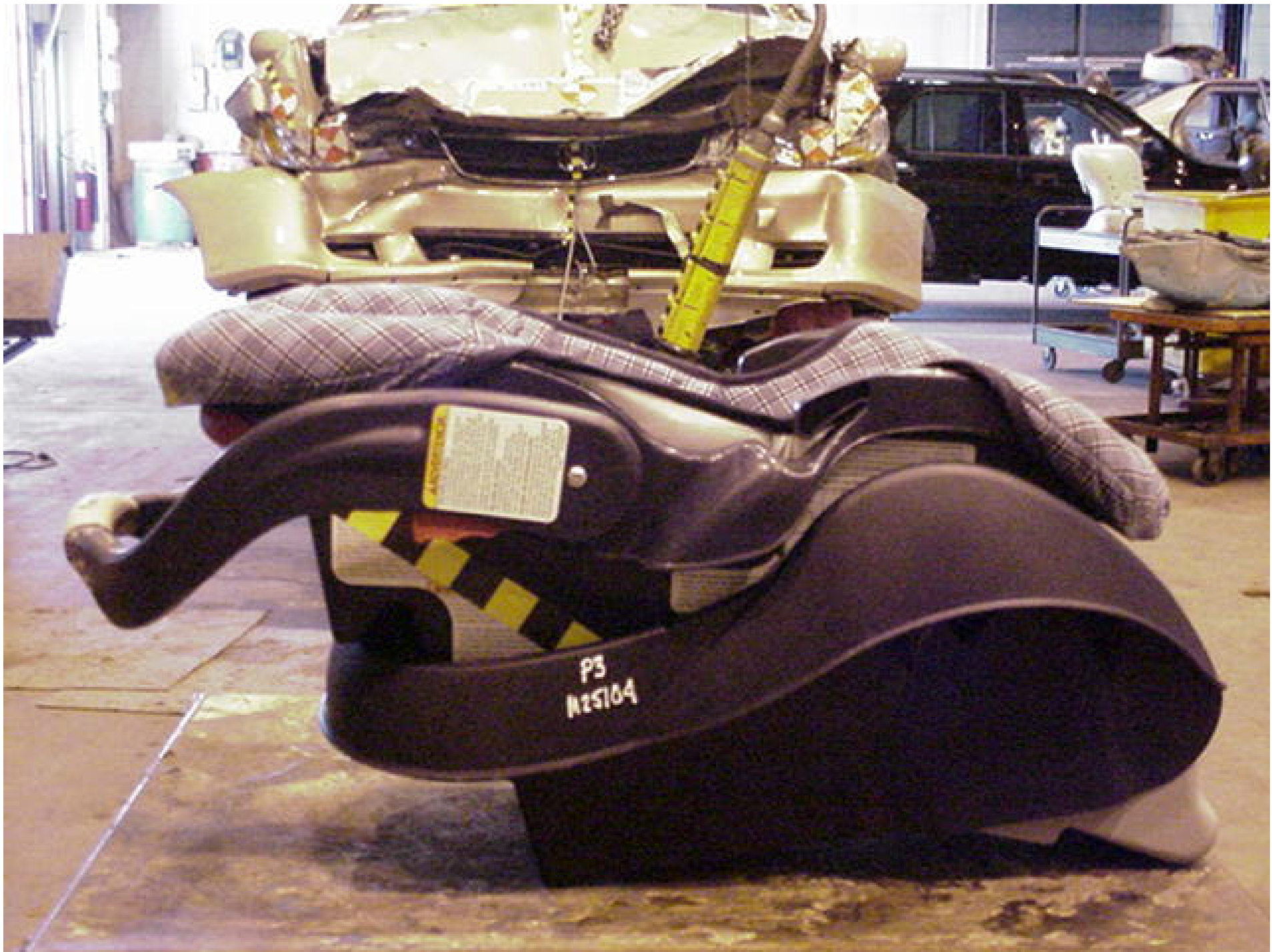
Figure 3-9 POST-TEST RIGHT SIDE VIEW OF POSITION 3 CRS
