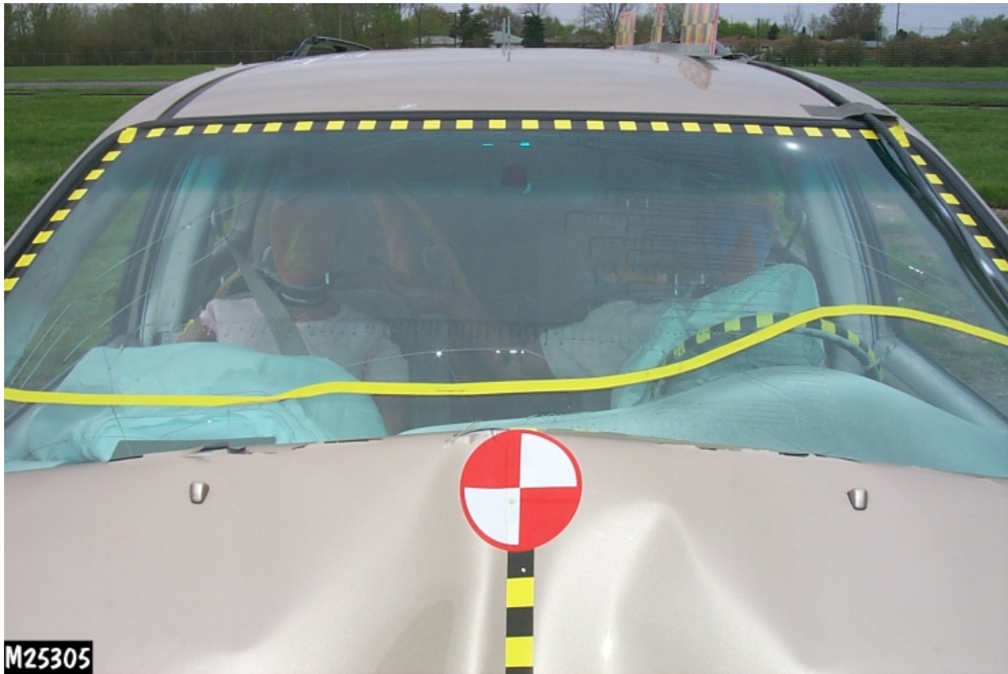
Figure A-13: POST-TEST WINDSHIELD VIEW
