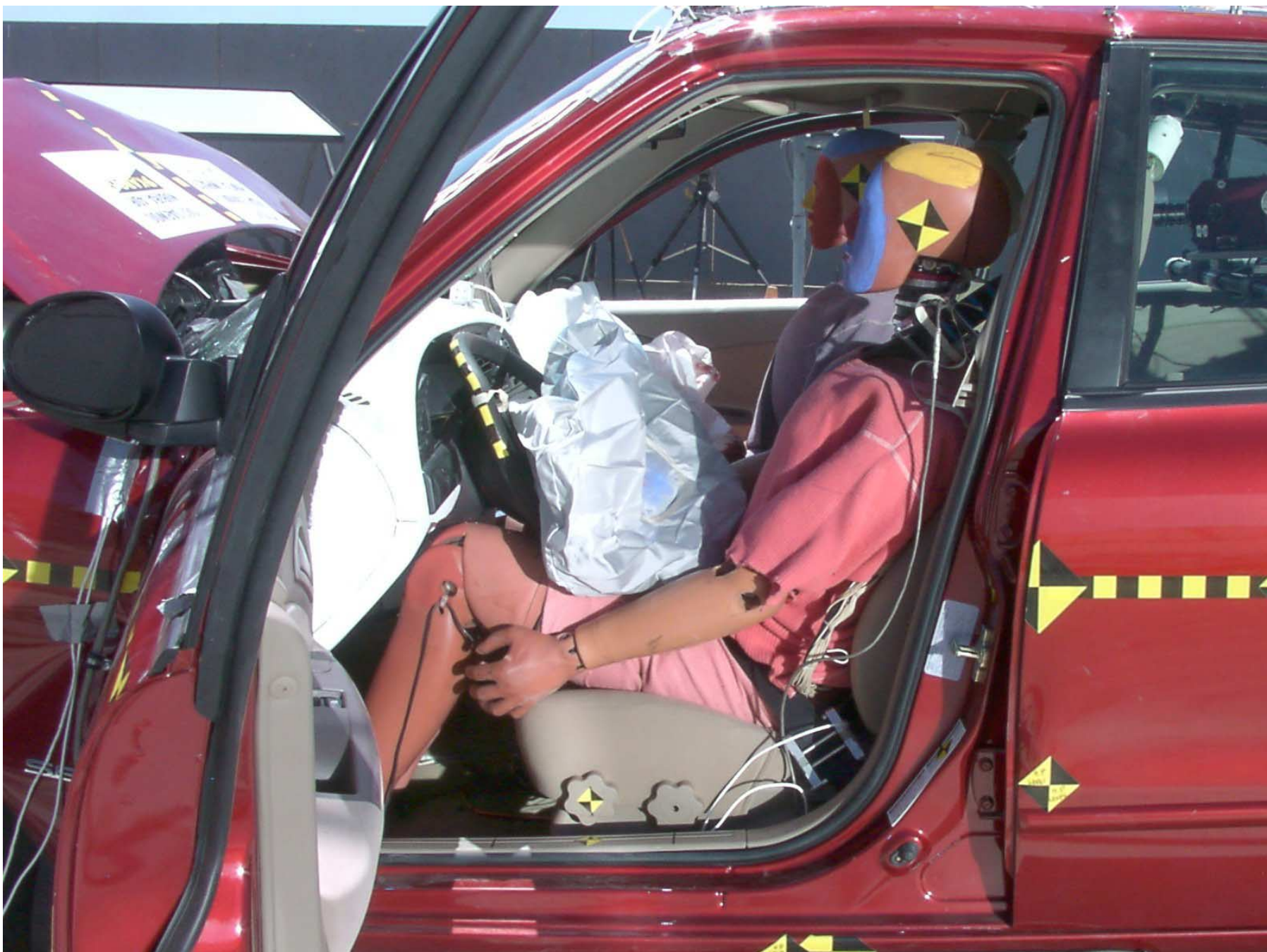
Figure A-32: Driver Dummy 90° To Vehicle, Post-Test
