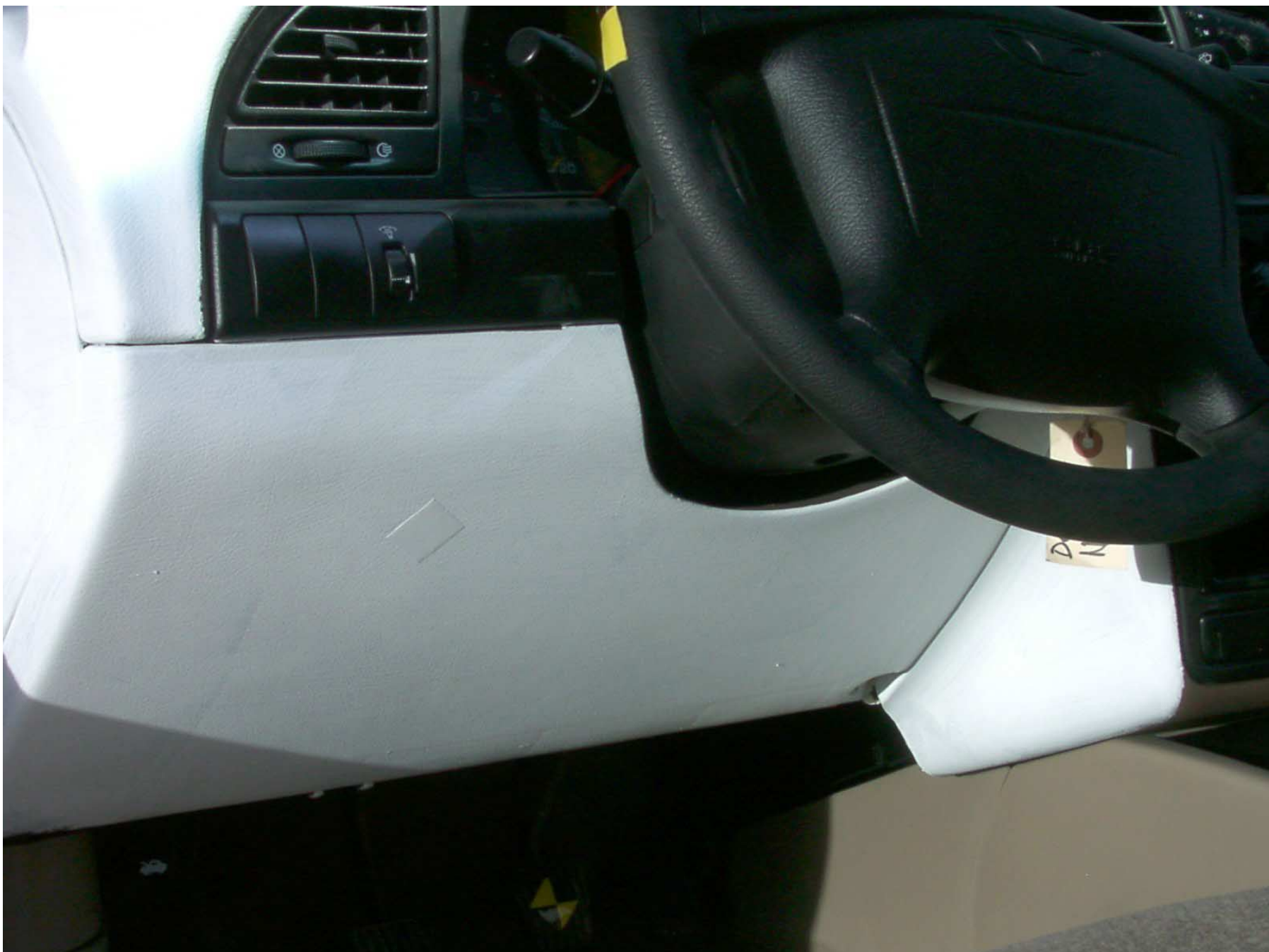
Figure A-35: Driver Side Knee Bolster, Pre-Test
