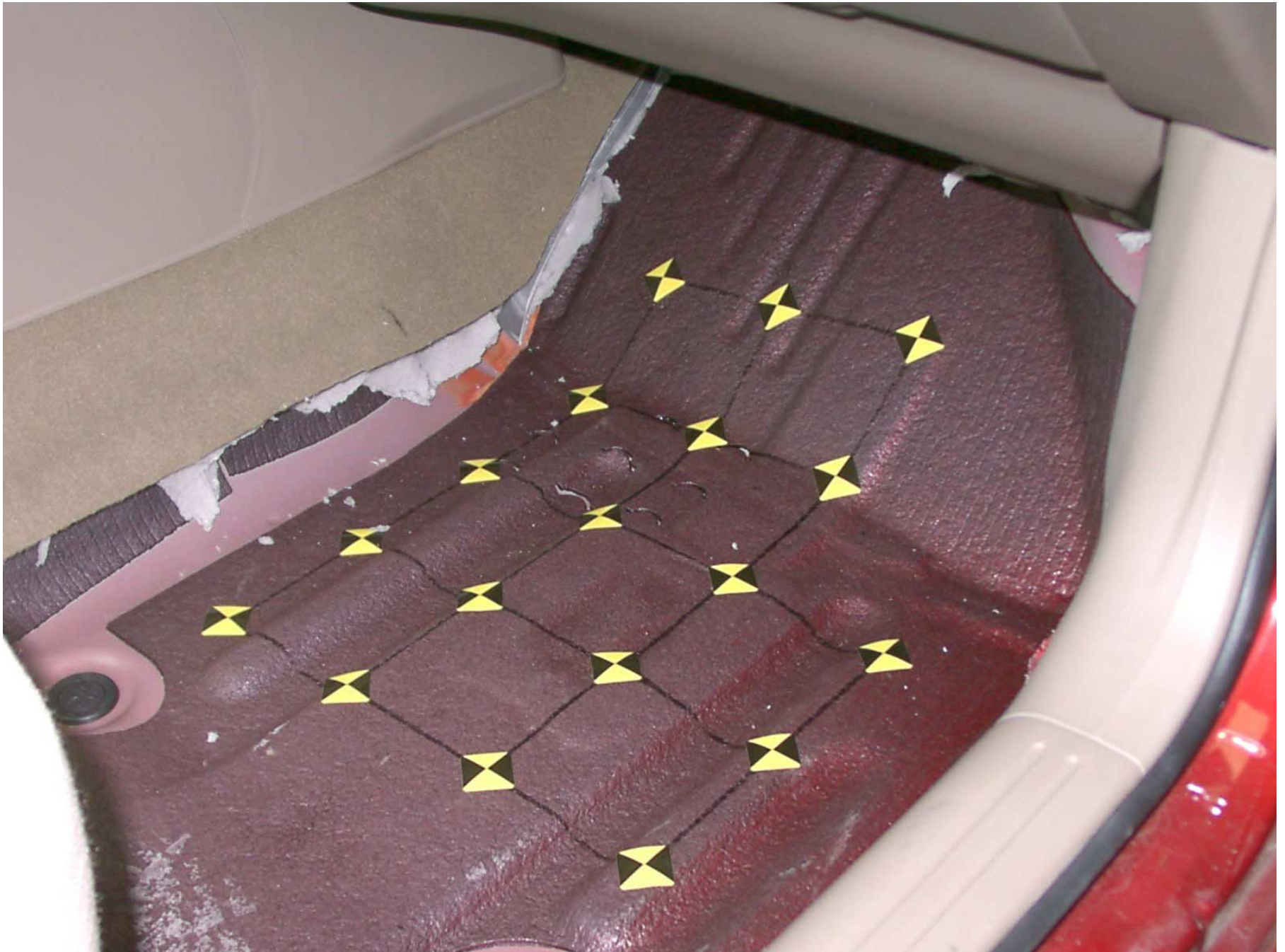
Figure A-51: Passenger Side Floor Pan, Pre-Test
