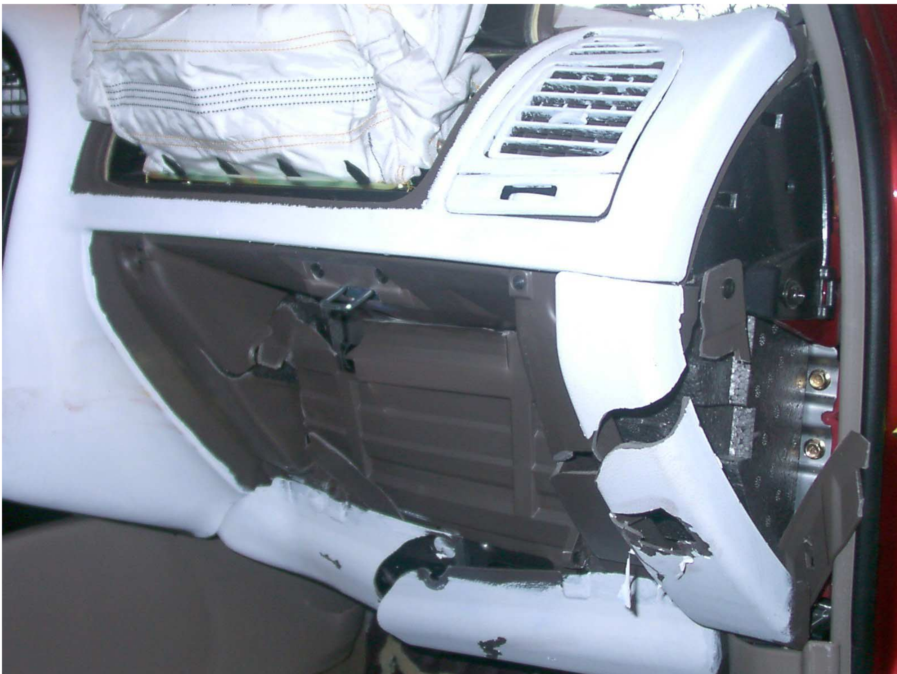
Figure A-54: Passenger Side Knee Bolster, Post-Test
