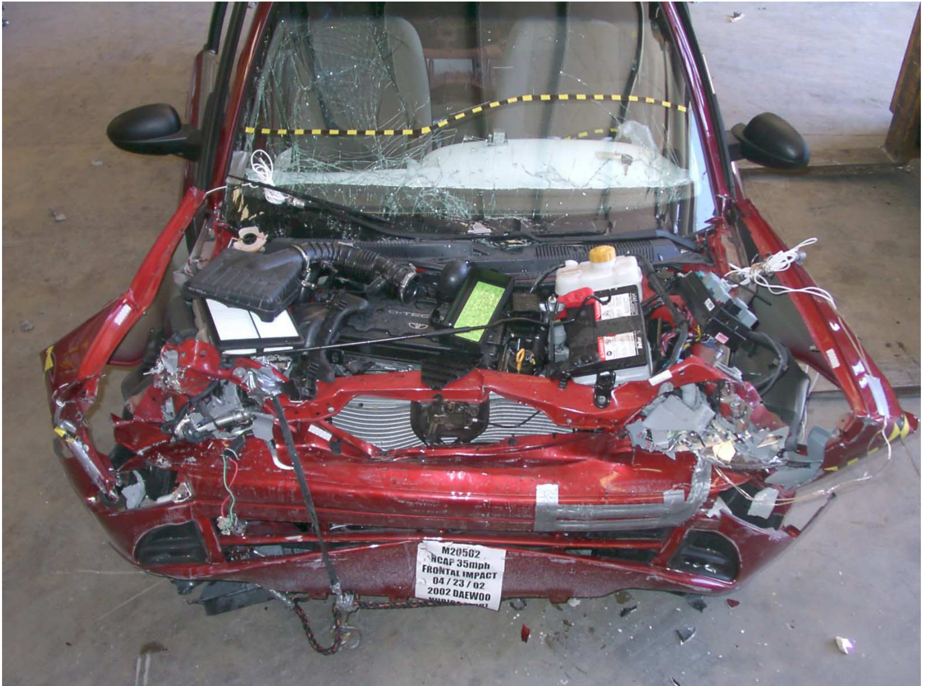
Figure A-18: Engine Compartment, Post-Test
