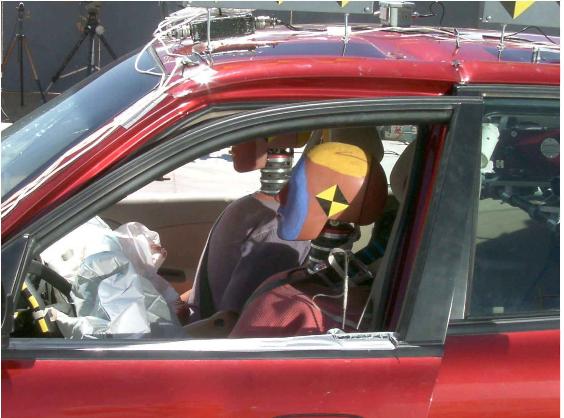
Figure A-28: Driver Dummy Through Window, Post-Test
