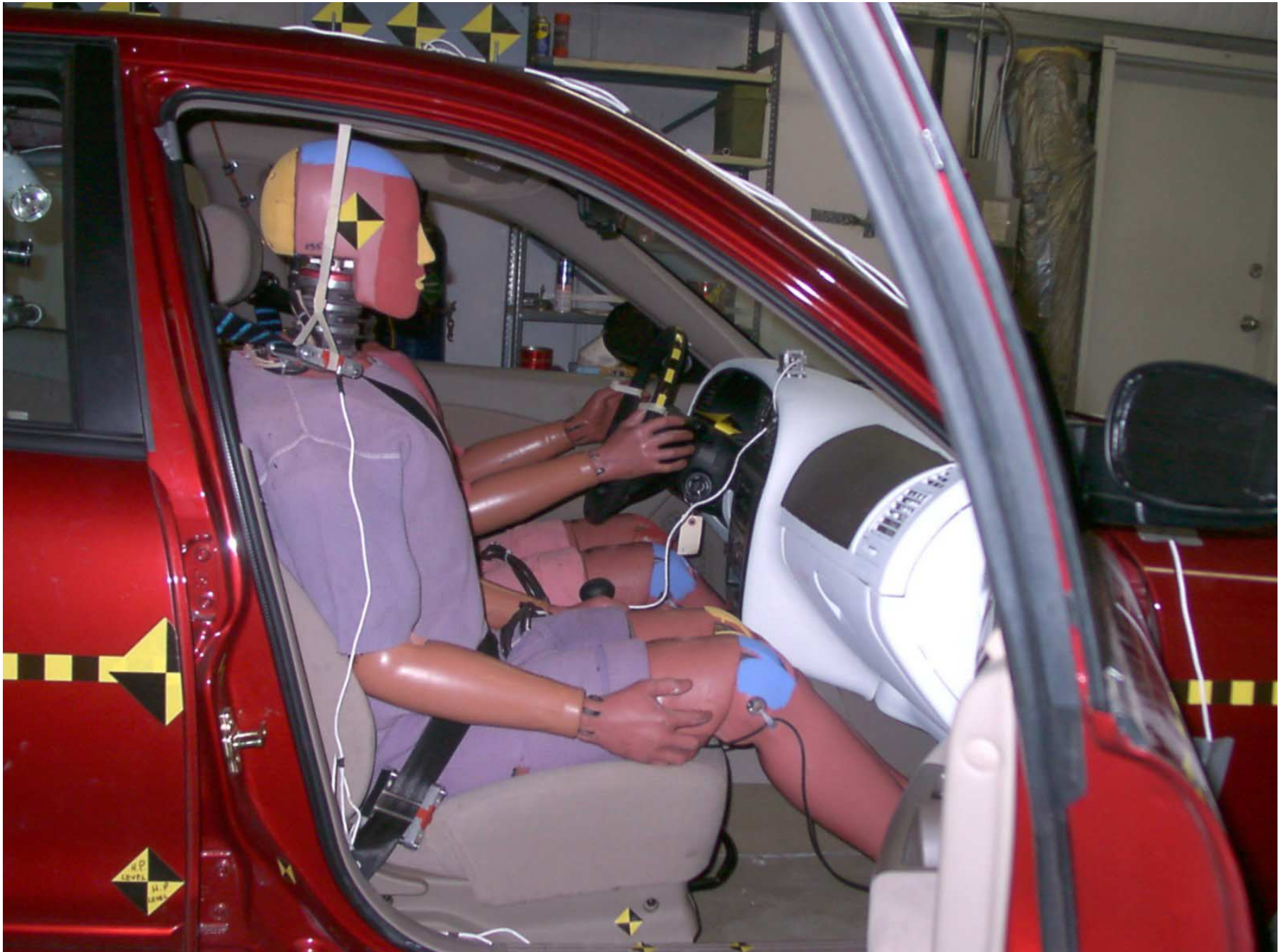
Figure A-47: Passenger Dummy 90° To Vehicle, Pre-Test
