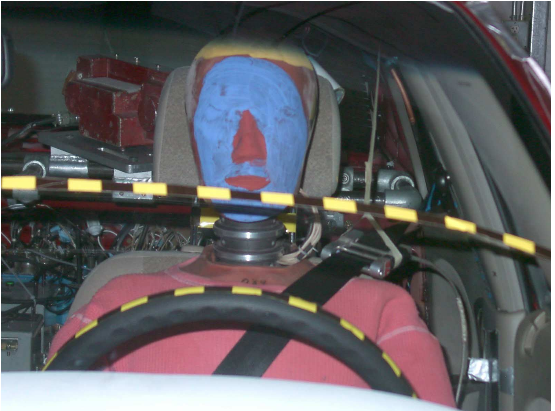
Figure A-25: Driver Dummy Front View, Pre-Test
