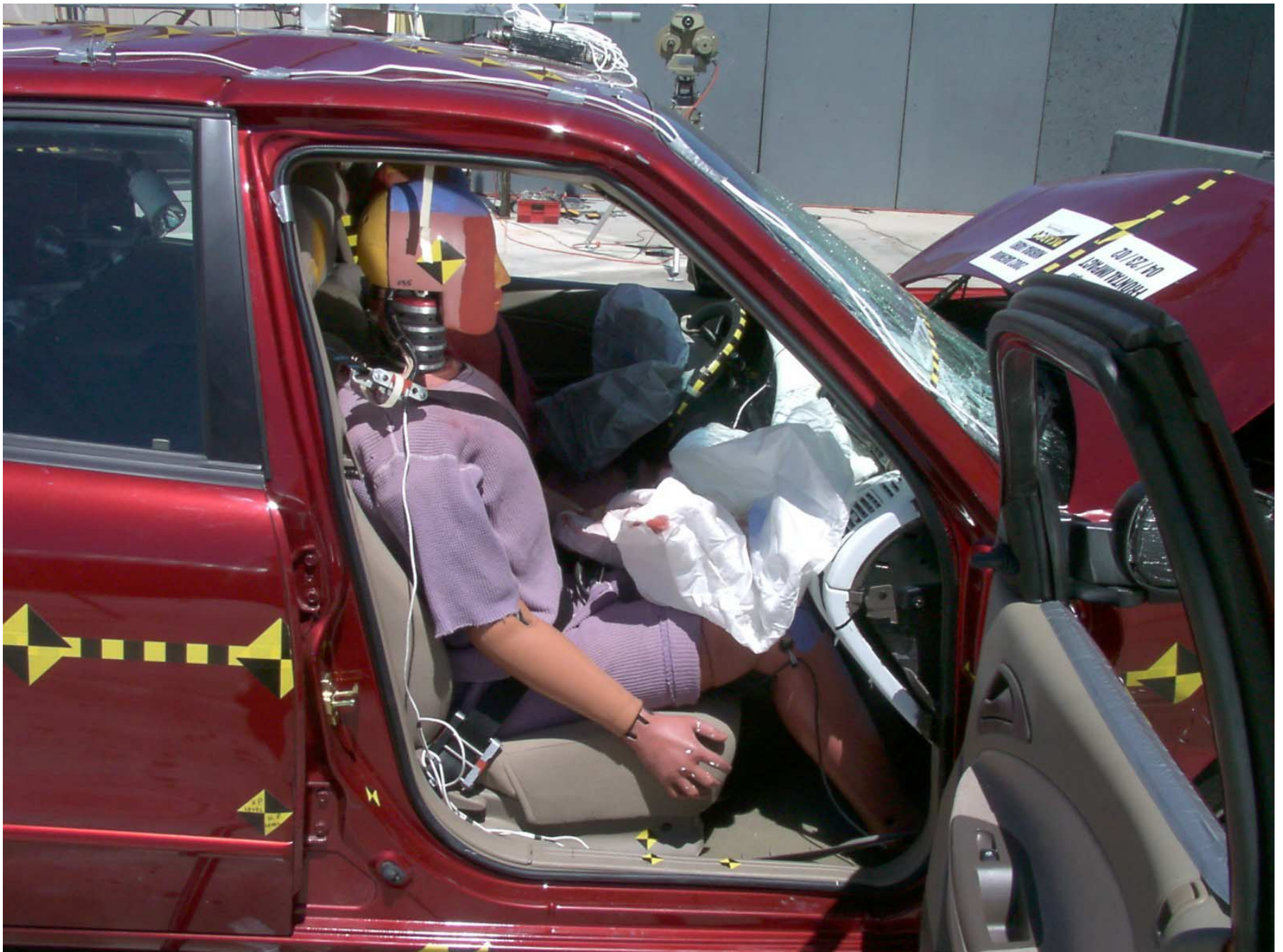
Figure A-48: Passenger Dummy 90° To Vehicle, Post-Test
