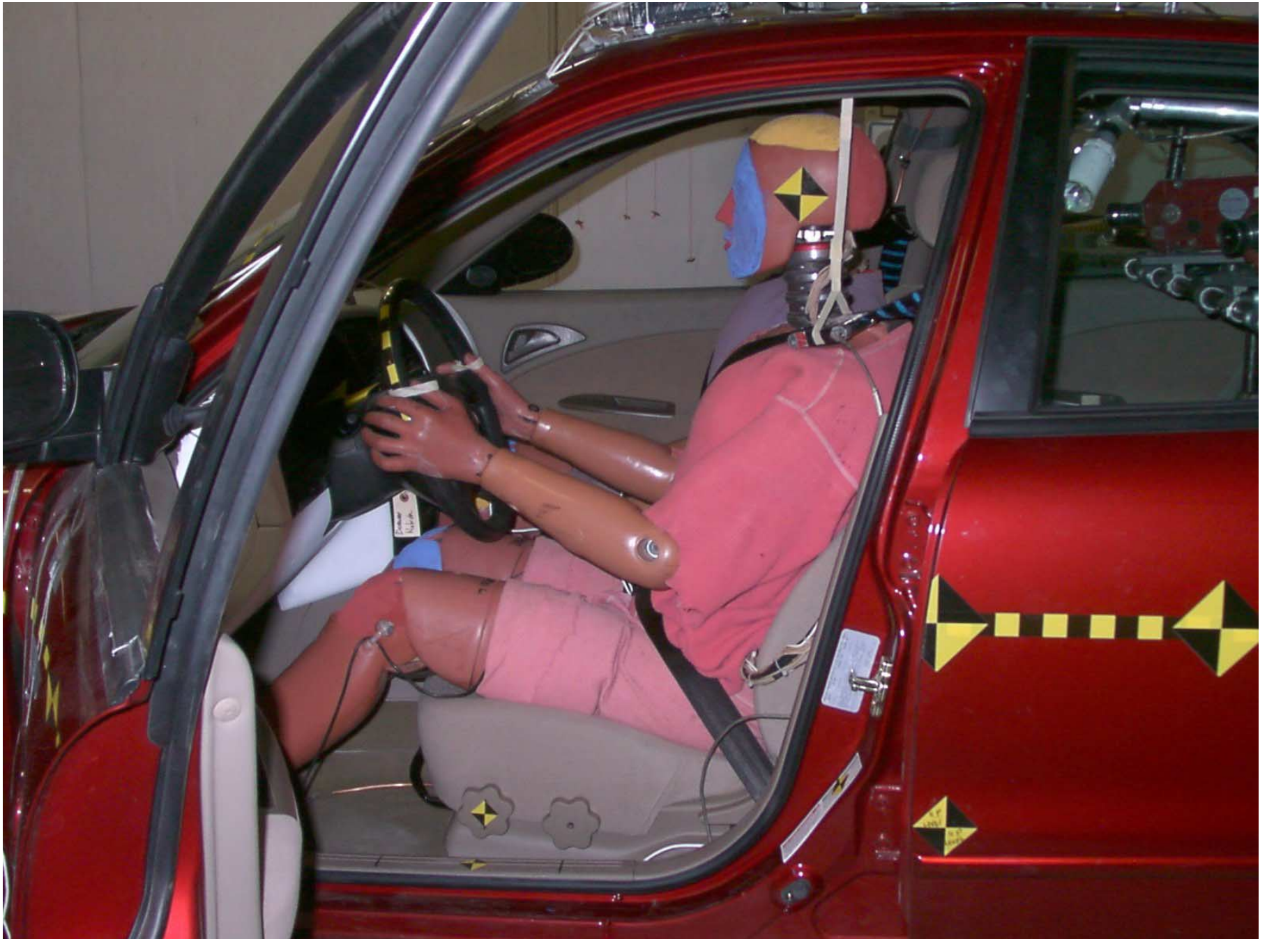
Figure A-31: Driver Dummy 90° To Vehicle, Pre-Test
