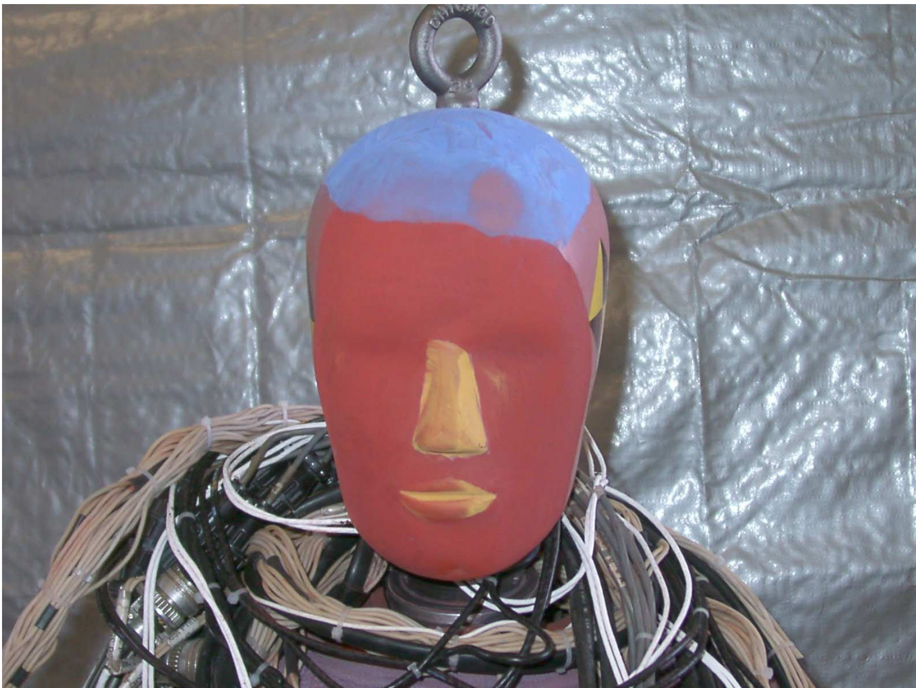
Figure A-55: Passenger Head, Post-Test
