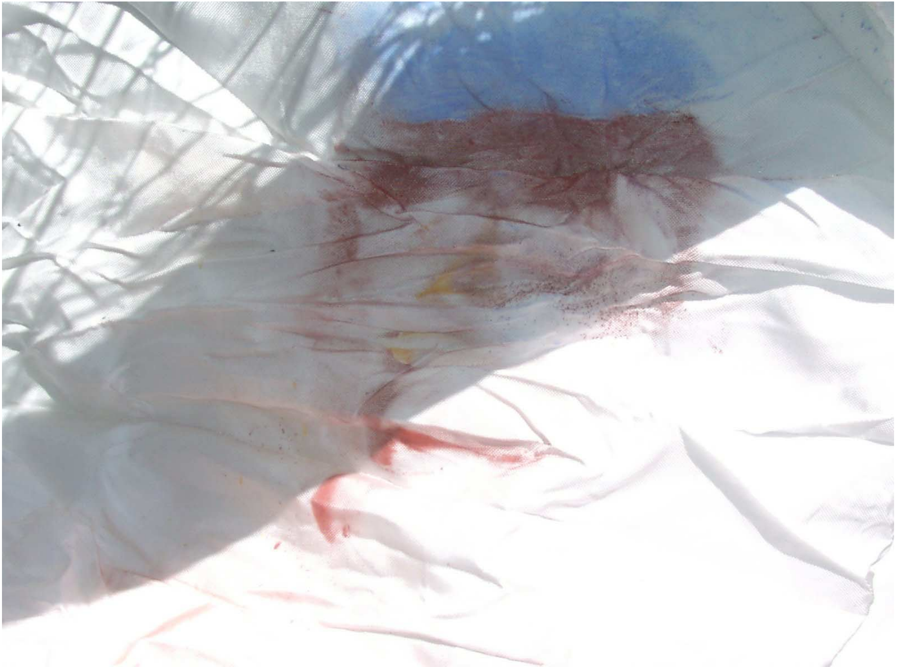
Figure A-56: Passenger Dummy Contact, Post-Test
