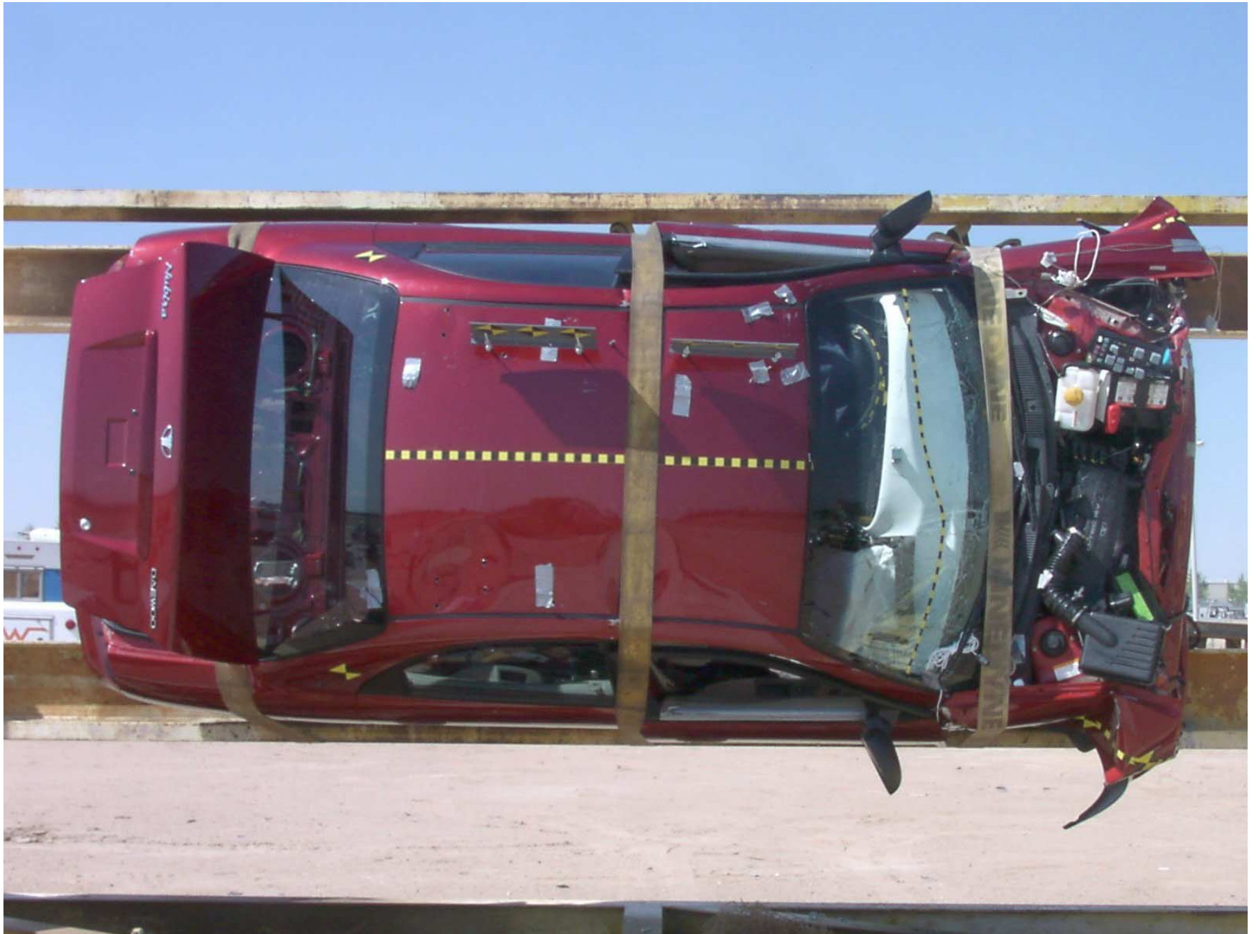
Figure A-59: Vehicle on Rollover Device
