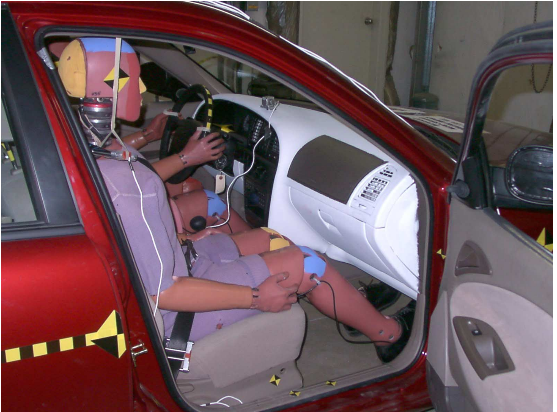
Figure A-45: Passenger Dummy Door Open, Pre-Test
