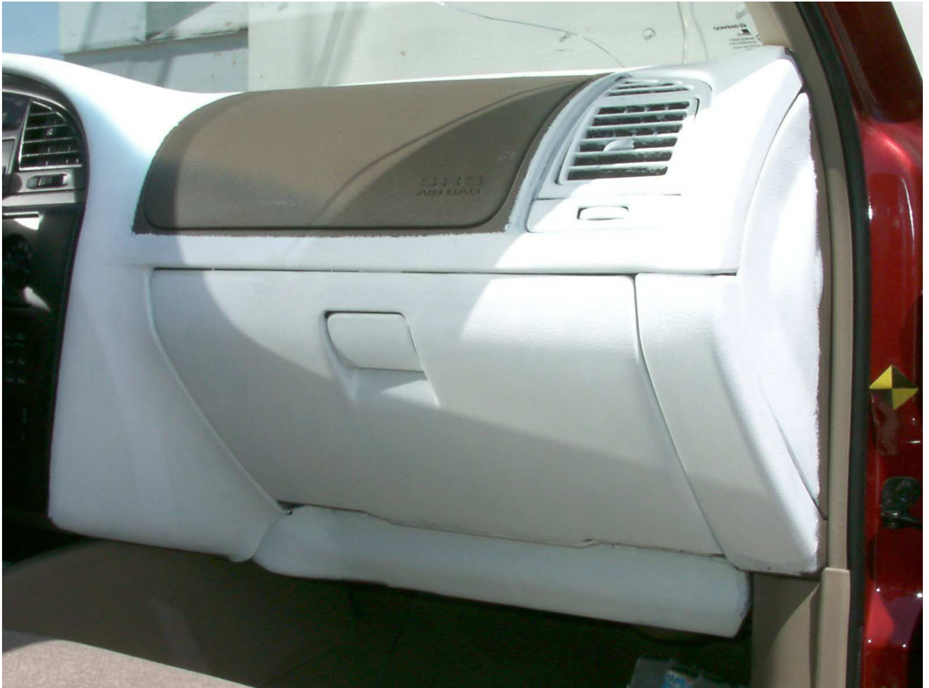
Figure A-53: Passenger Side Knee Bolster, Pre-Test
