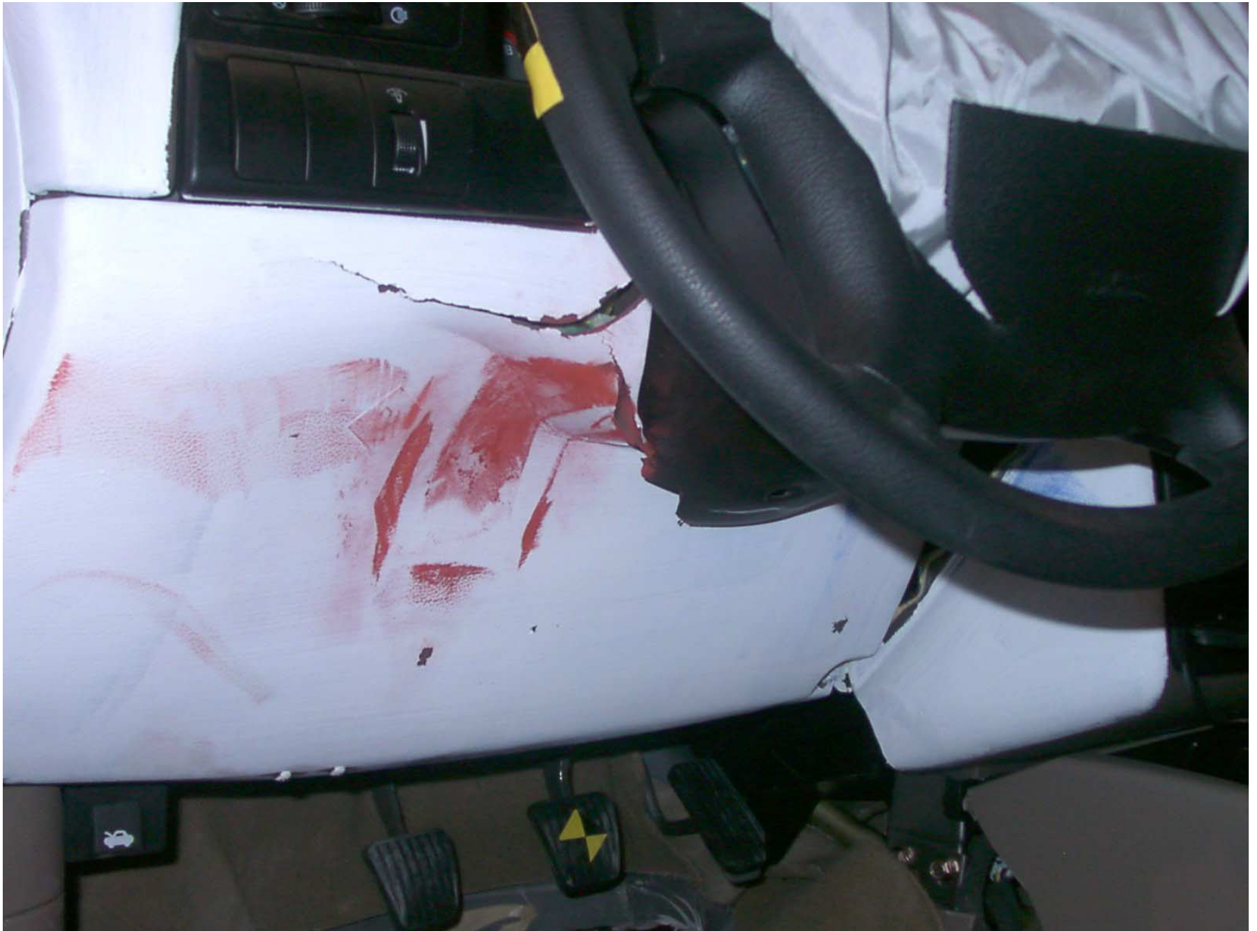
Figure A-36: Driver Side Knee Bolster, Post-Test
