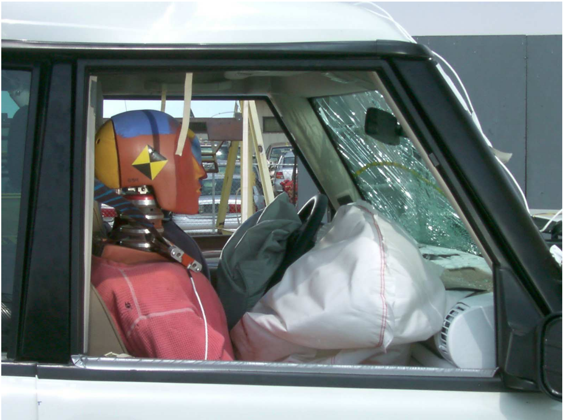
Figure A-44: Passenger Dummy Through Window, Post-Test
