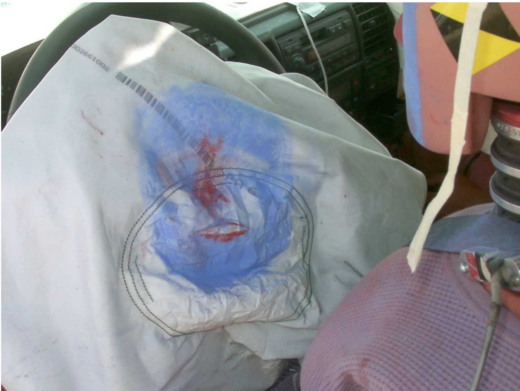
Figure A-40: Driver Dummy Contact, Post-Test
