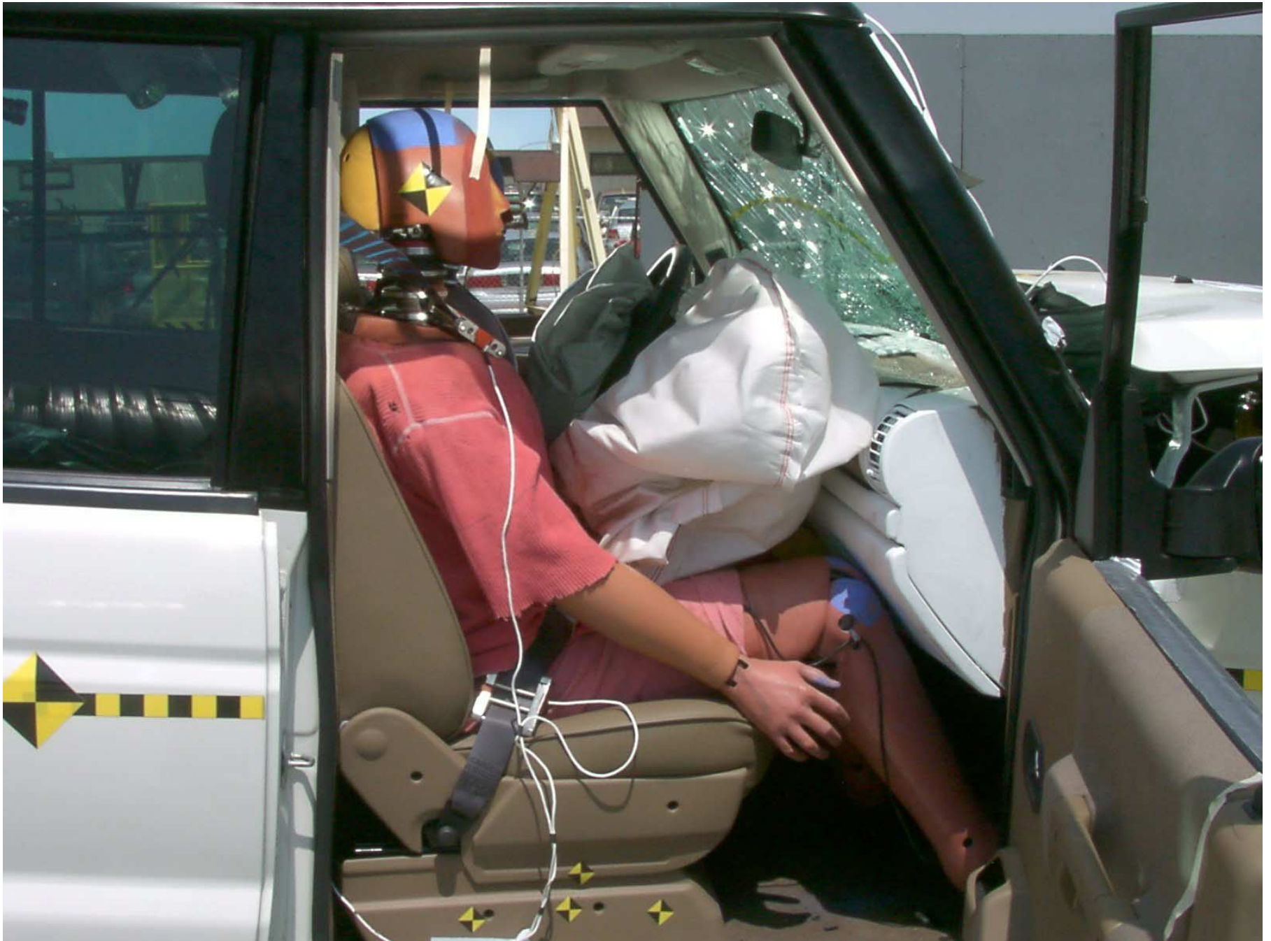
Figure A-48: Passenger Dummy 90° To Vehicle, Post-Test
