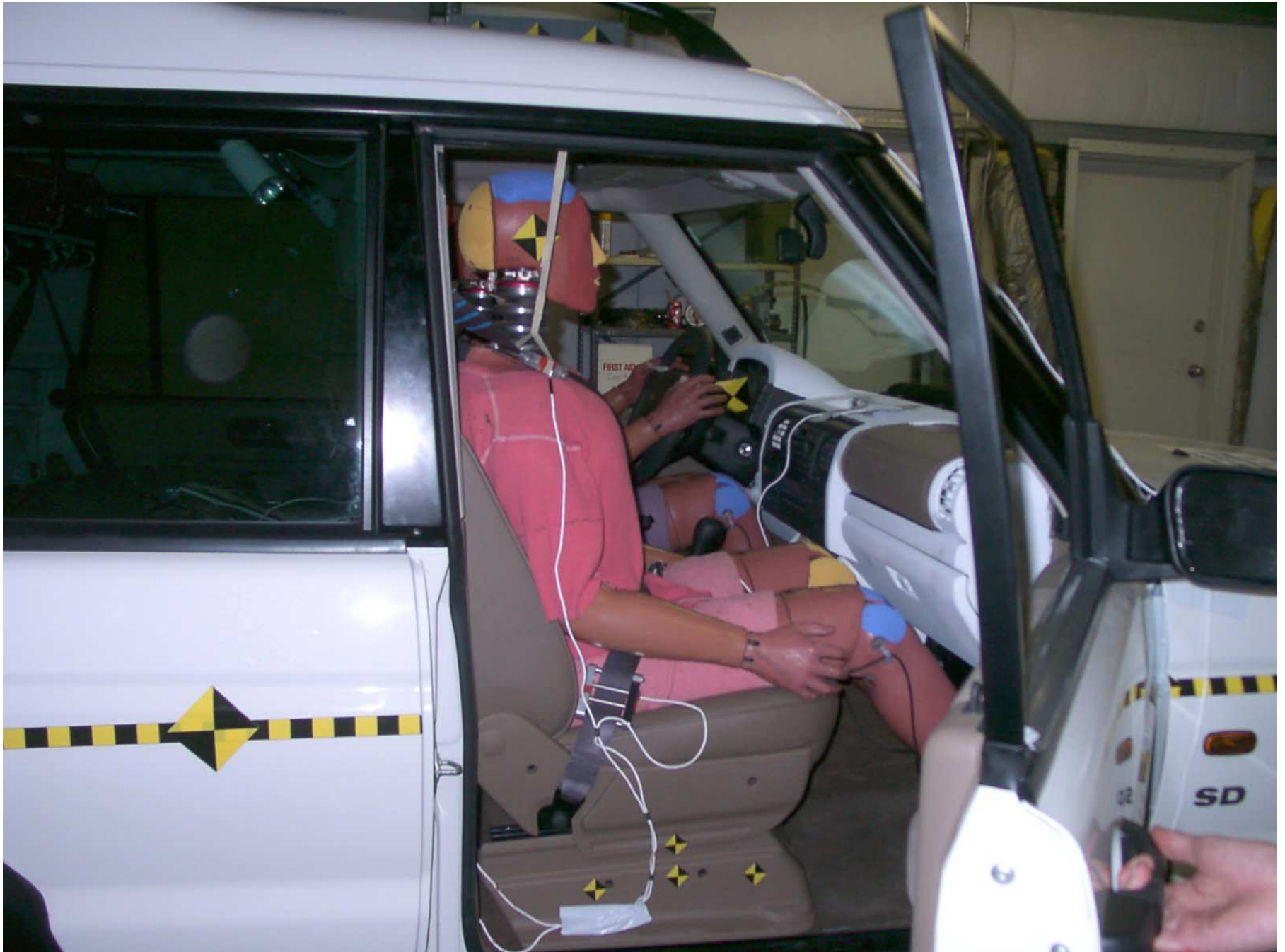
Figure A-47: Passenger Dummy 90° To Vehicle, Pre-Test
