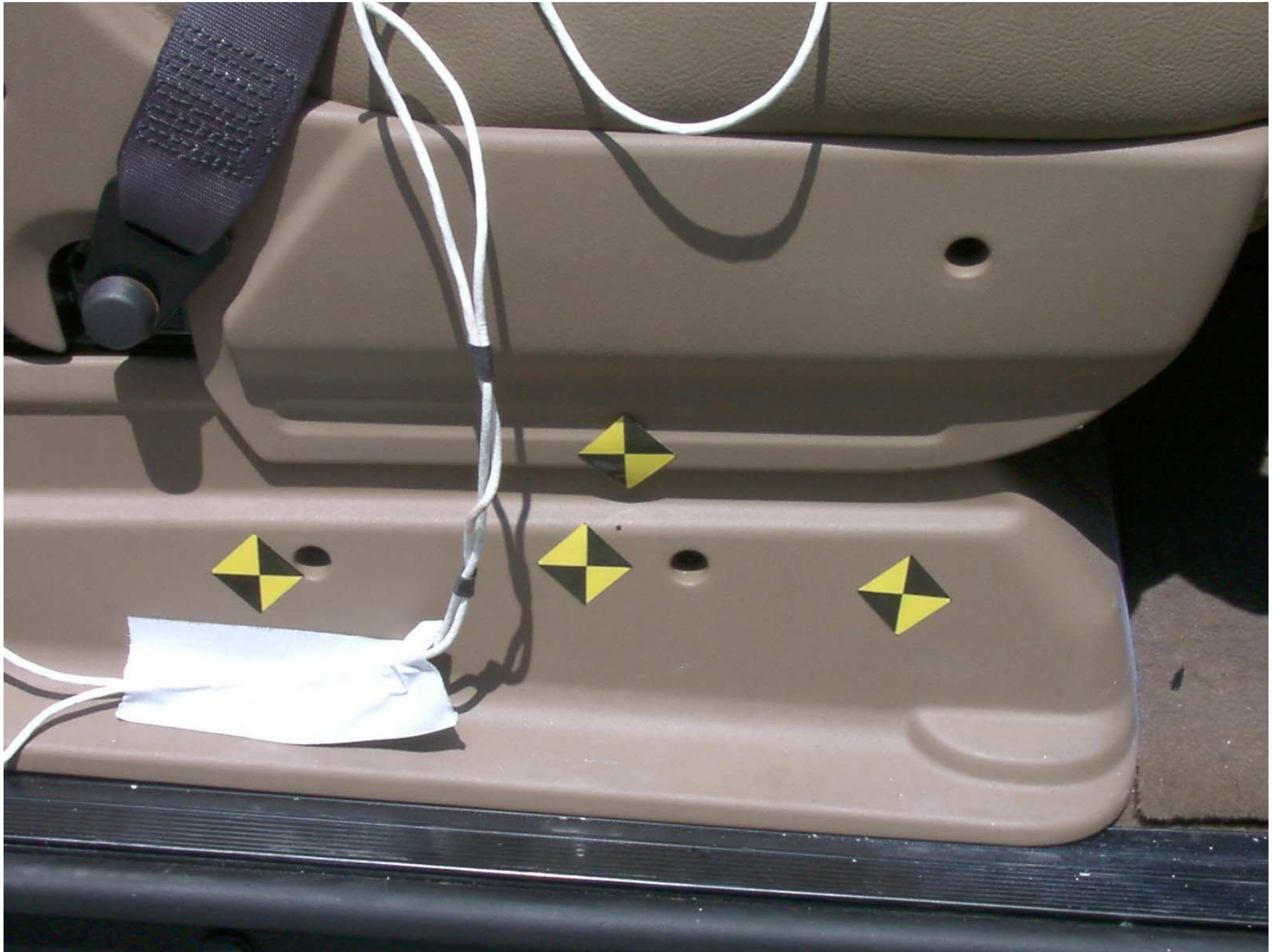
Figure A-62: Right Side Seat Track Movement, Post-Test
