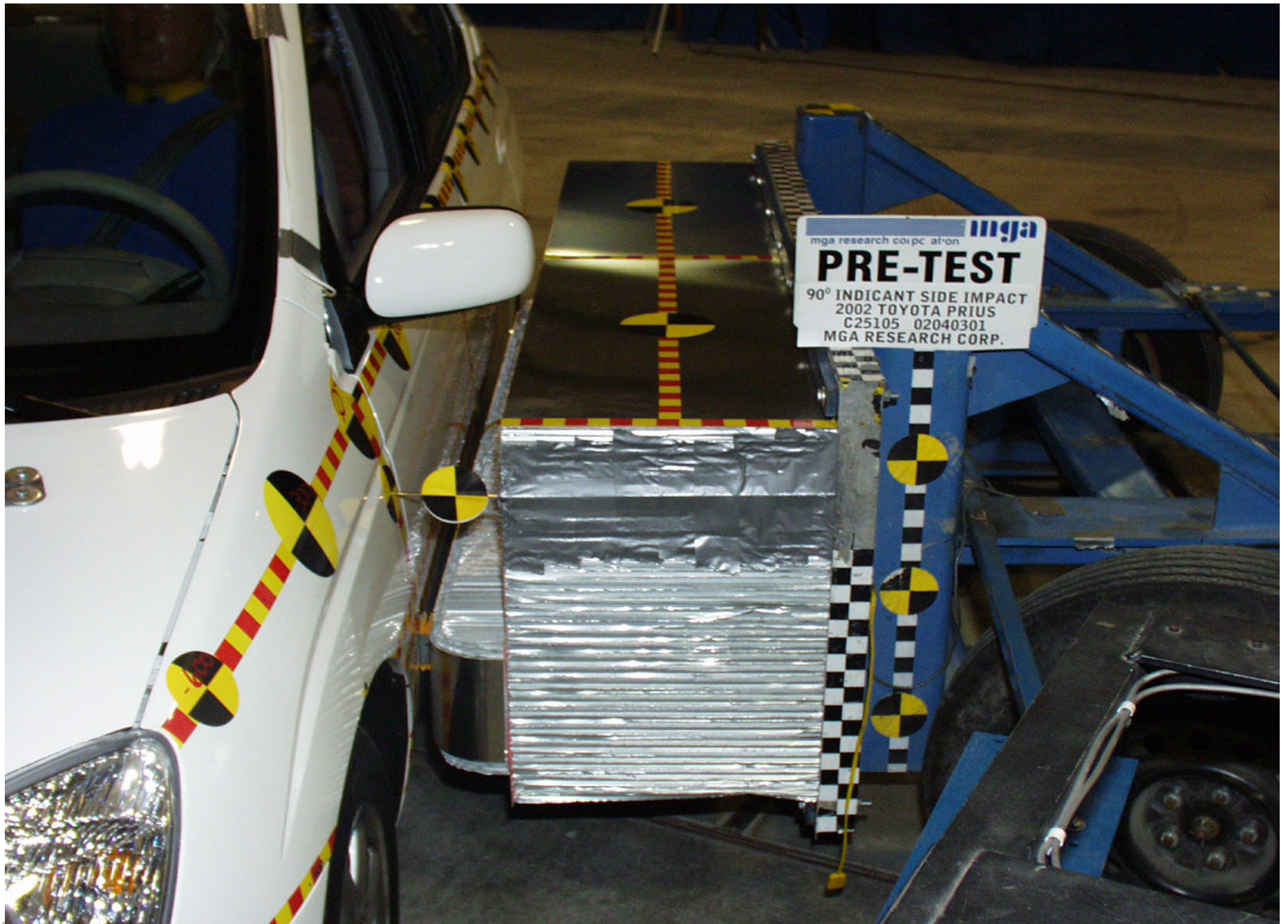
Pre-Test MDB Positioned Against Vehicle (left side)
