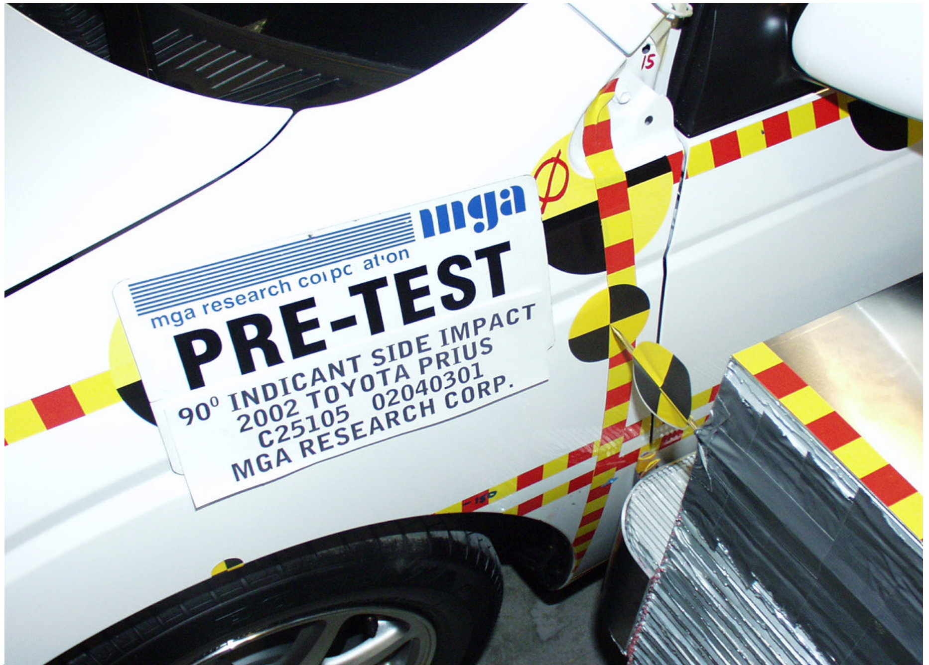
Pre-Test Left Front Impact Point on Vehicle
