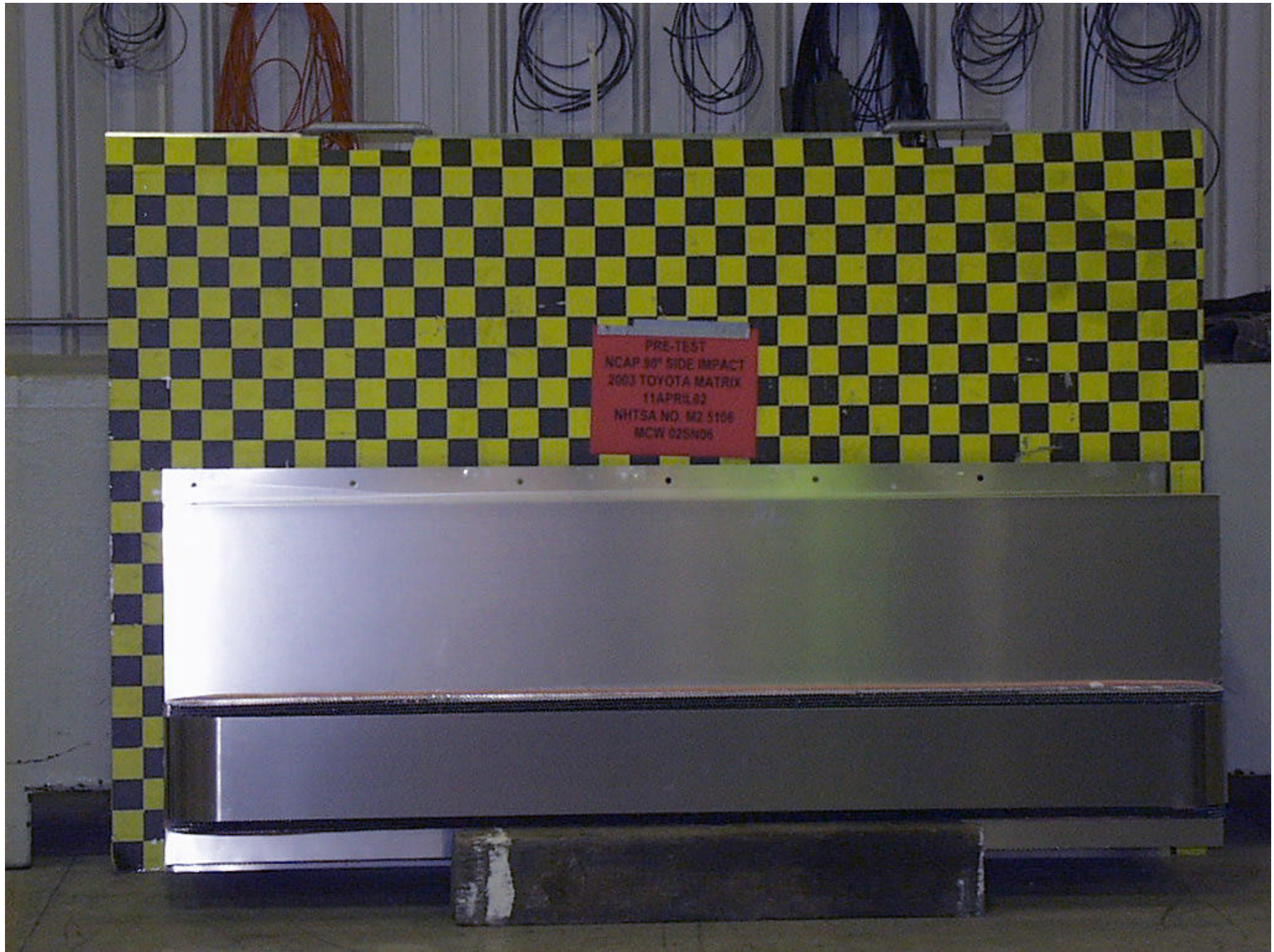
Figure A-45: PRE-TEST ALUMINUM BARRIER FRONT
