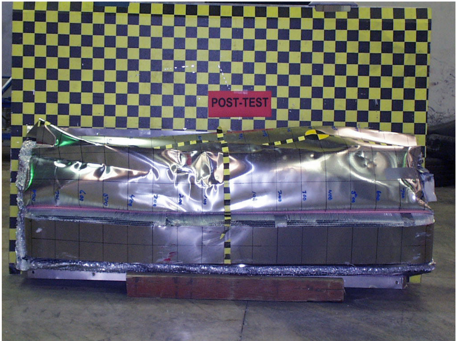
Figure A-46: POST-TEST ALUMINUM BARRIER FRONT
