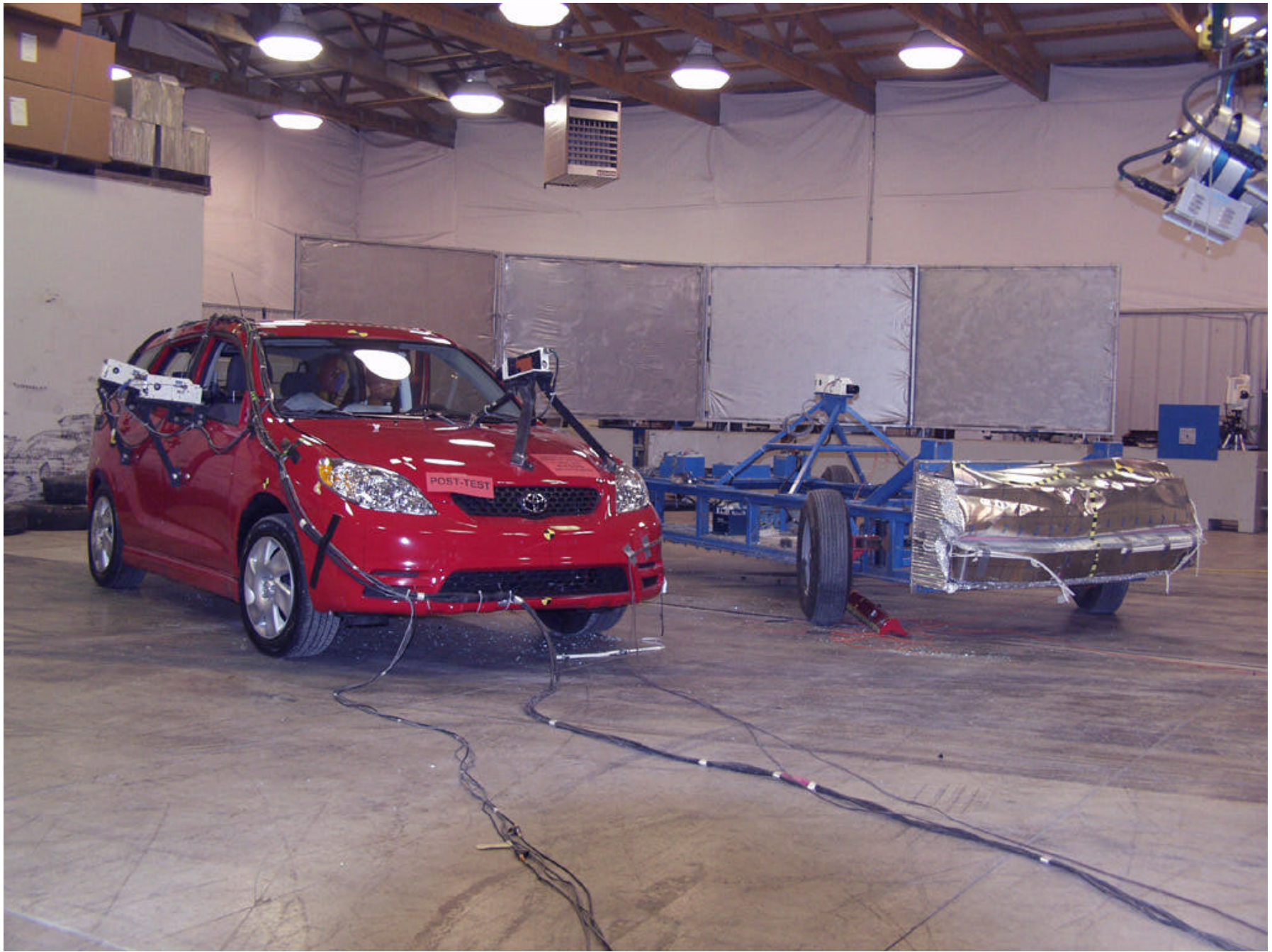
Figure A-32: POST-TEST FRONT RIGHT VIEW OF MDB
