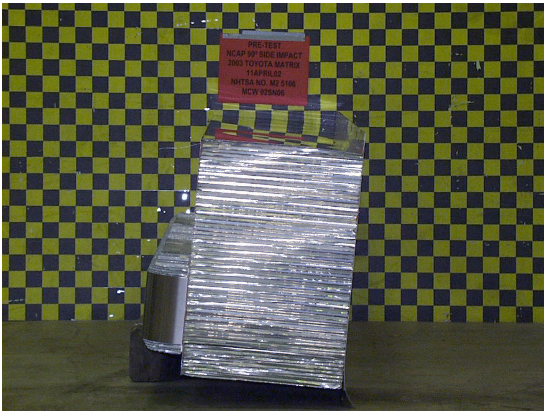
Figure A-47: PRE-TEST ALUMINUM BARRIER LEFT SIDE
