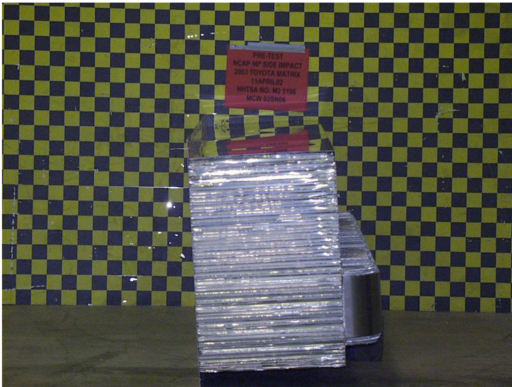
Figure A-49: PRE-TEST ALUMINUM BARRIER RIGHT SIDE
