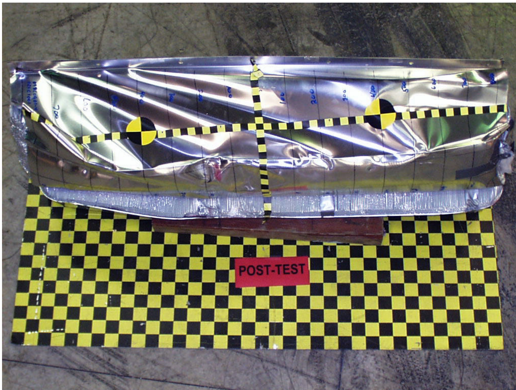
Figure A-52: POST-TEST ALUMINUM BARRIER OVERHEAD
