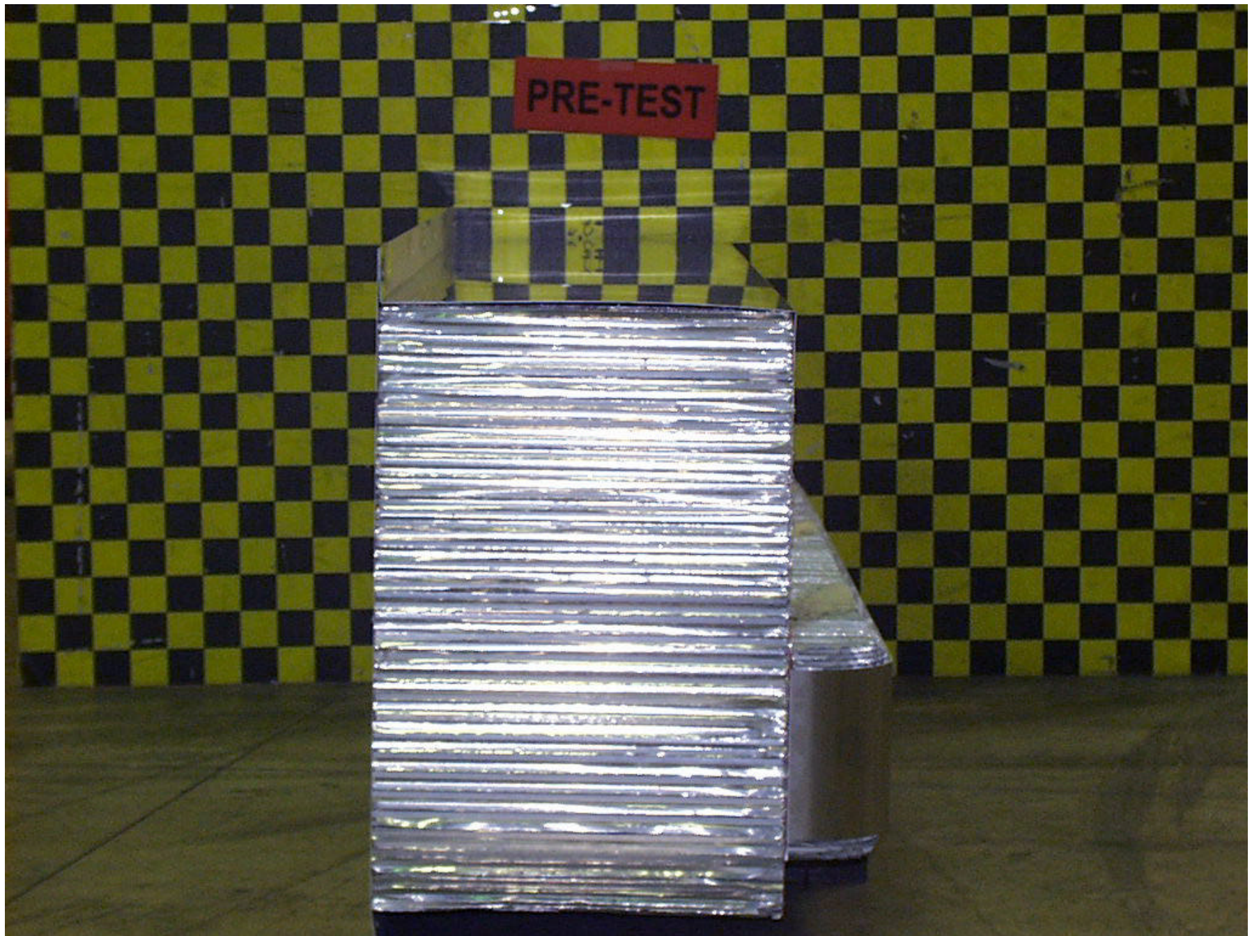
Figure A-48: PRE-TEST ALUMINUM BARRIER RIGHT SIDE
