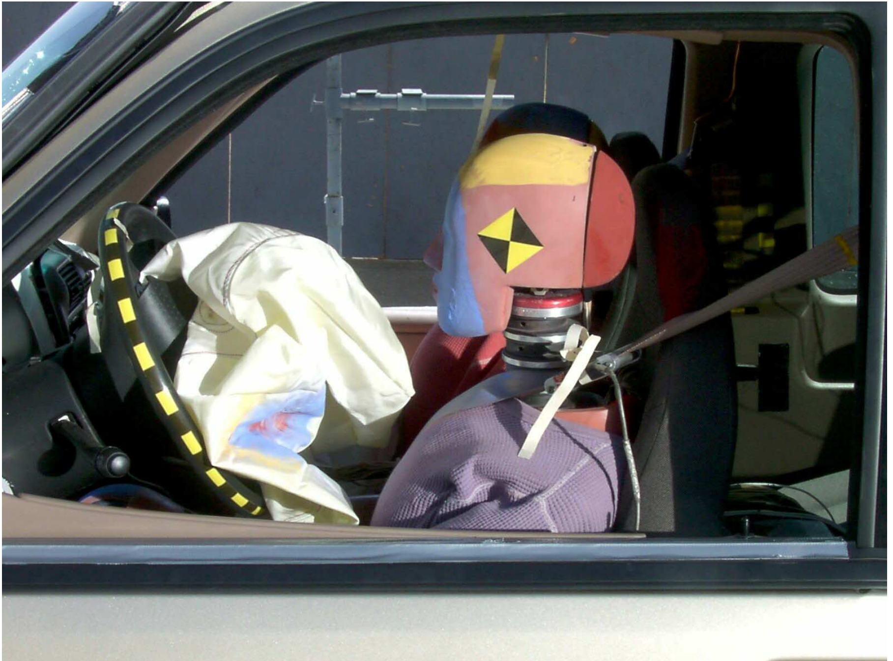
Figure A-28: Driver Dummy Through Window, Post-Test
