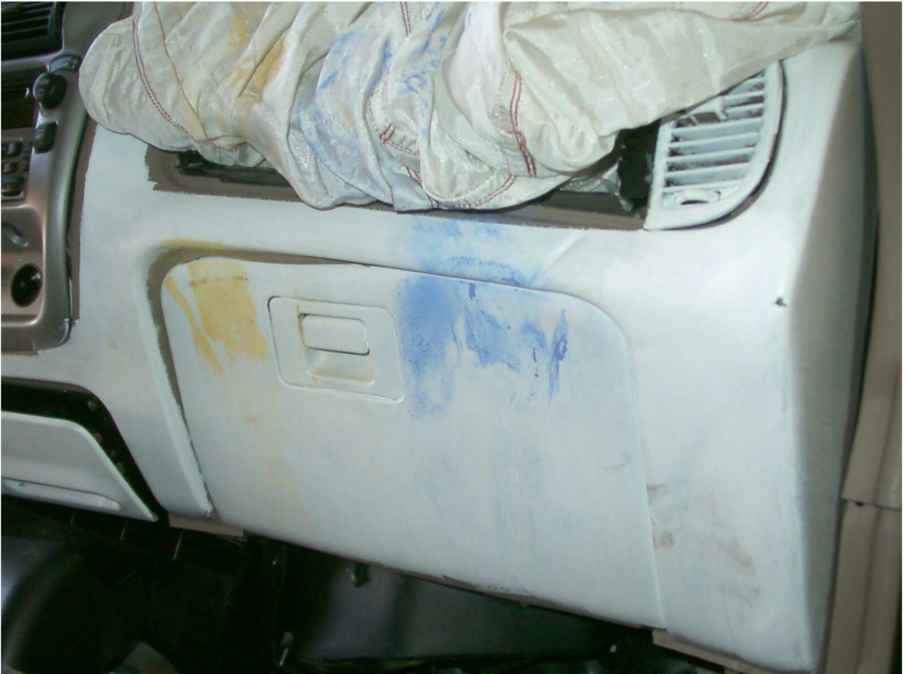
Figure A-54: Passenger Side Knee Bolster, Post-Test
