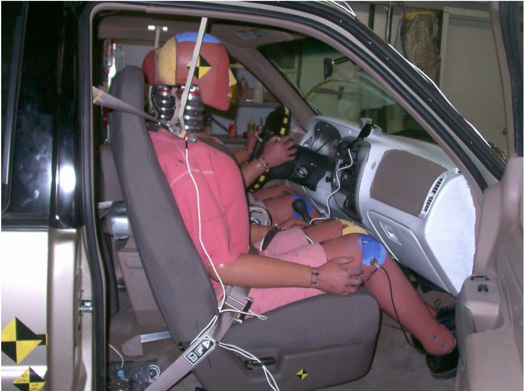
Figure A-47: Passenger Dummy 90° To Vehicle, Pre-Test
