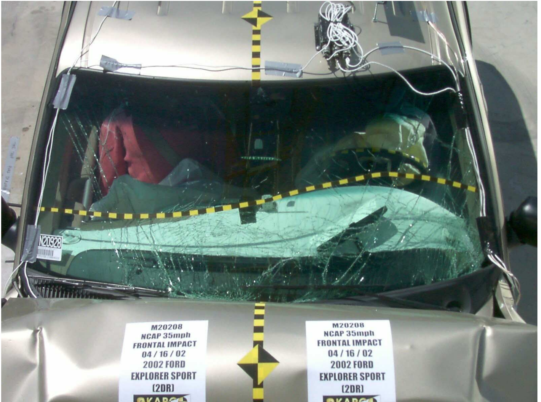
Figure A-16: Windshield, Post-Test
