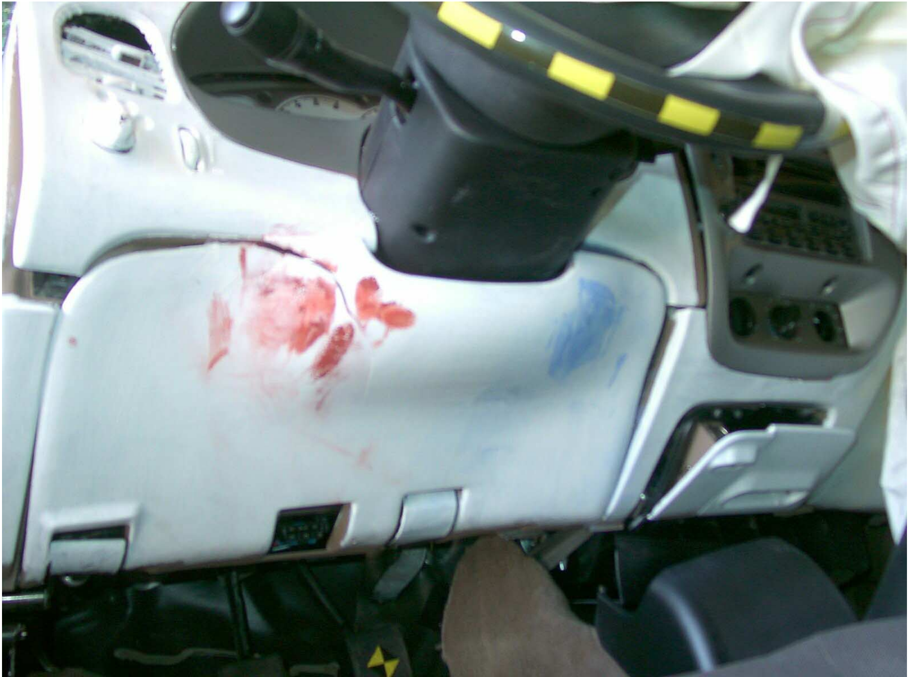
Figure A-36: Driver Side Knee Bolster, Post-Test
