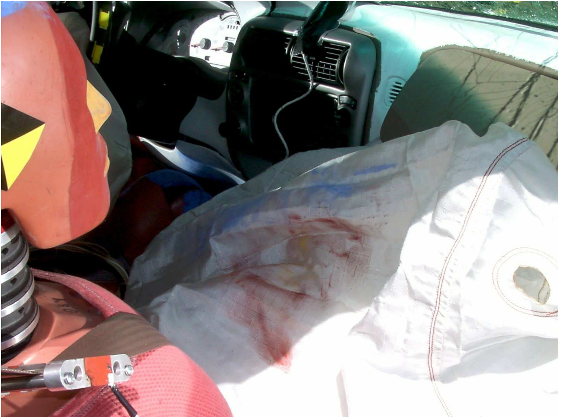
Figure A-56: Passenger Dummy Contact, Post-Test
