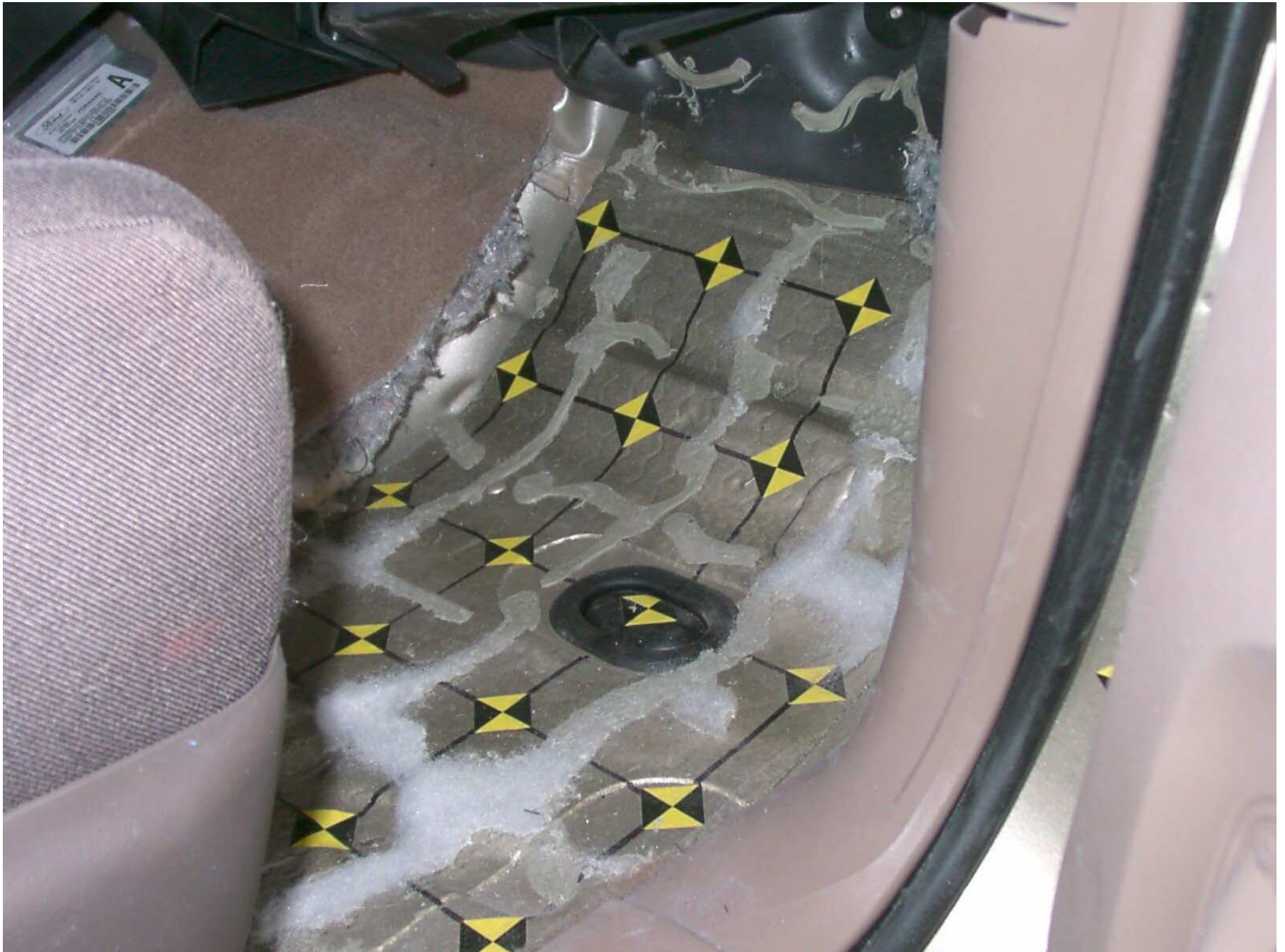
Figure A-52: Passenger Side Floor Pan, Post-Test
