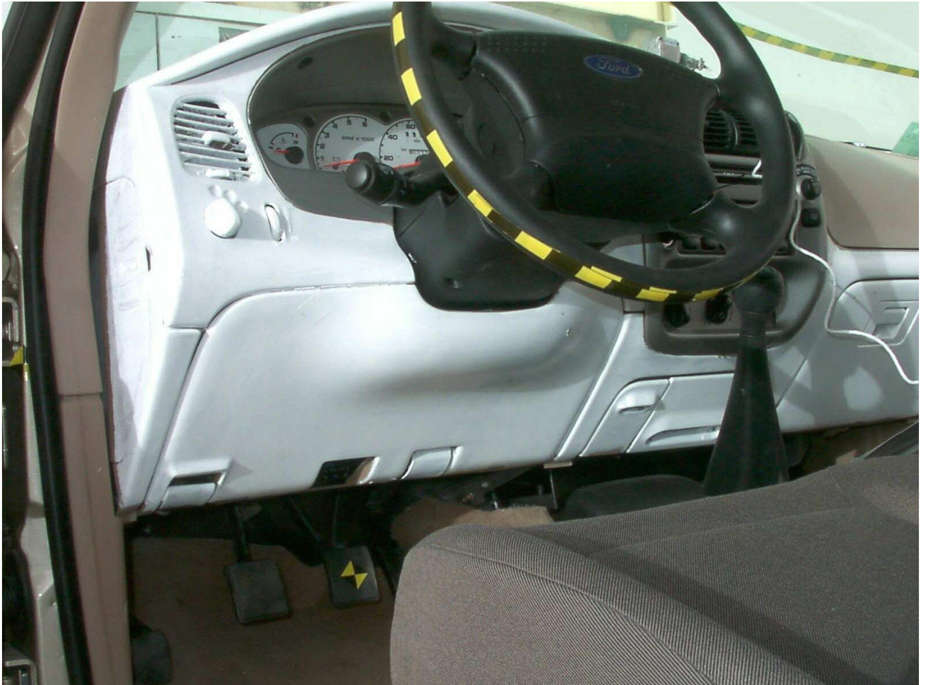
Figure A-35: Driver Side Knee Bolster, Pre-Test
