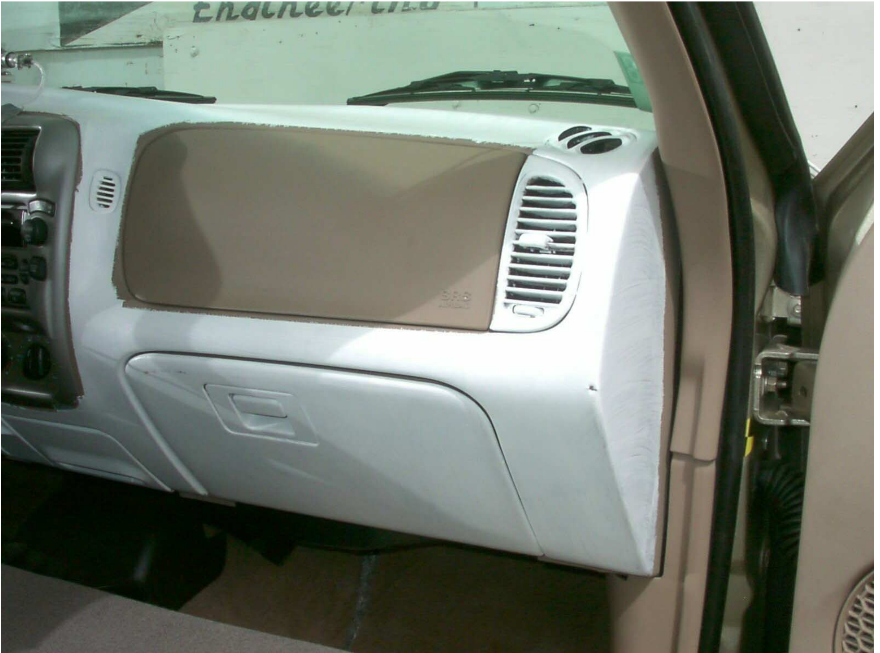
Figure A-53: Passenger Side Knee Bolster, Pre-Test
