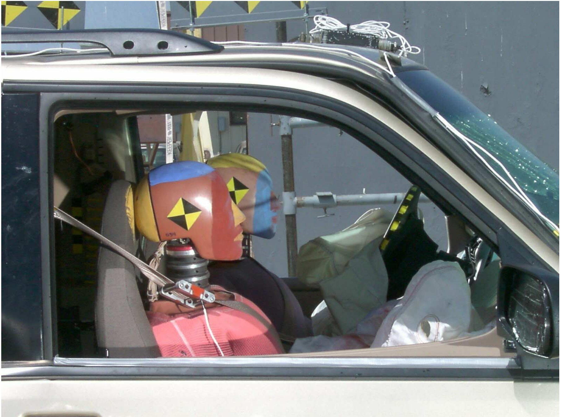
Figure A-44: Passenger Dummy Through Window, Post-Test
