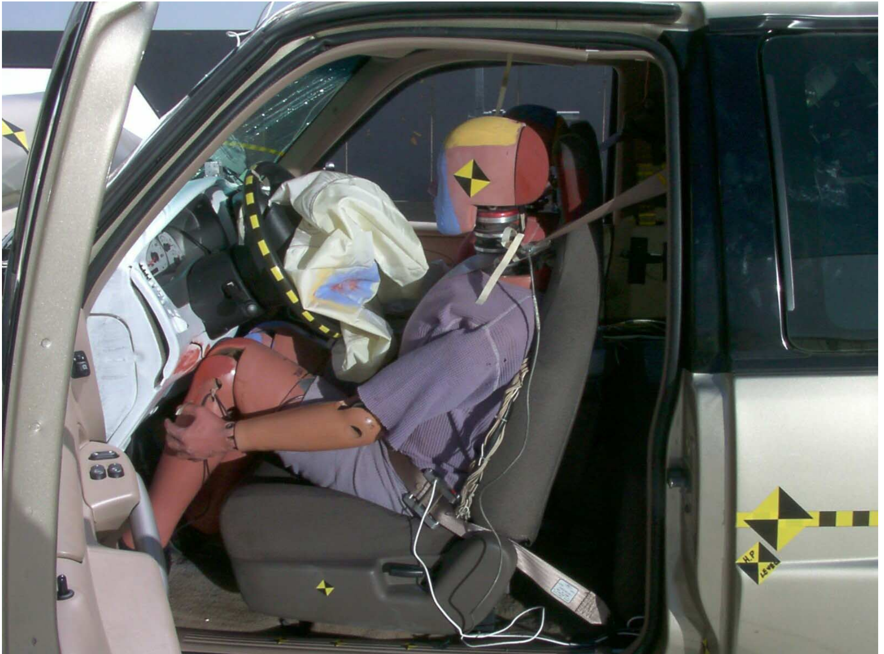
Figure A-32: Driver Dummy 90° To Vehicle, Post-Test
