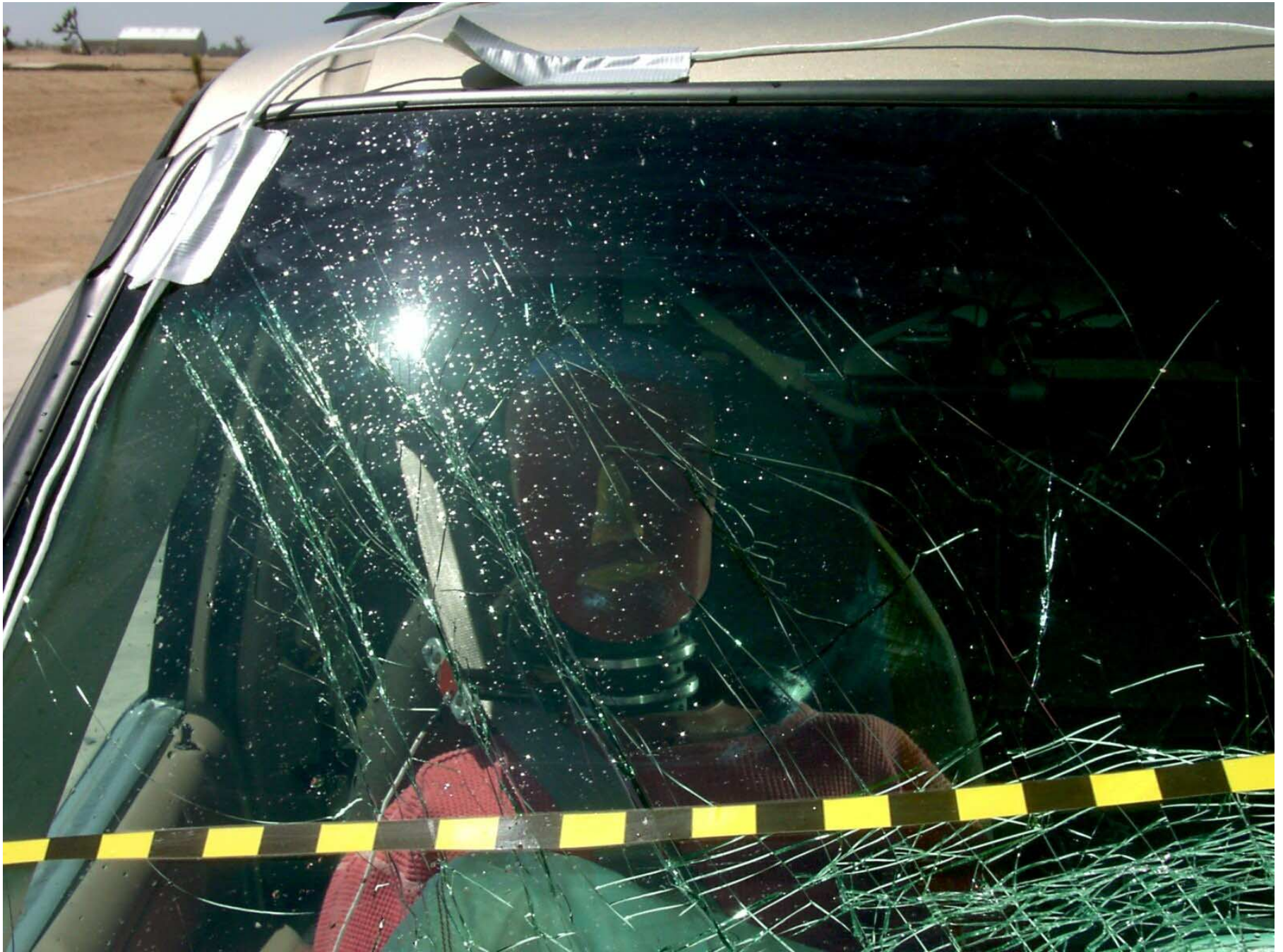
Figure A-42: Passenger Dummy Front View, Post-Test
