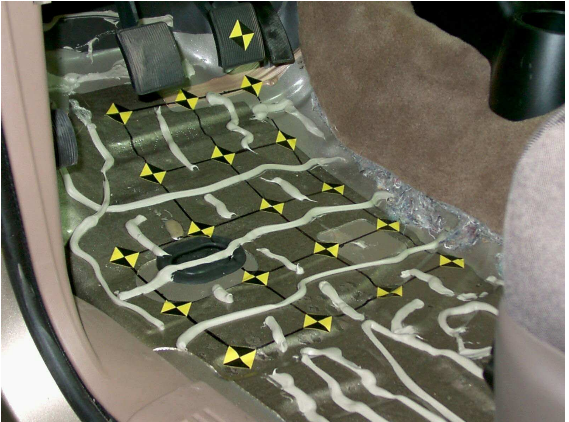
Figure A-37: Driver Side Floor Pan, Pre-Test
