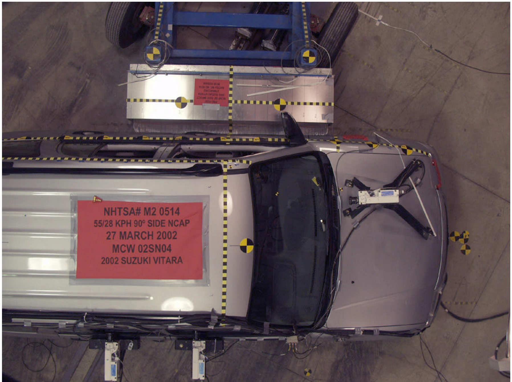
Figure A-33: PRE-TEST OVERHEAD VIEW OF MDB IN IMPACT POSITION
