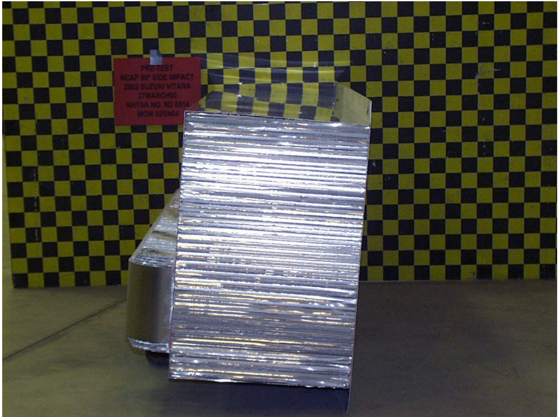
Figure A-47: PRE-TEST ALUMINUM BARRIER LEFT SIDE
