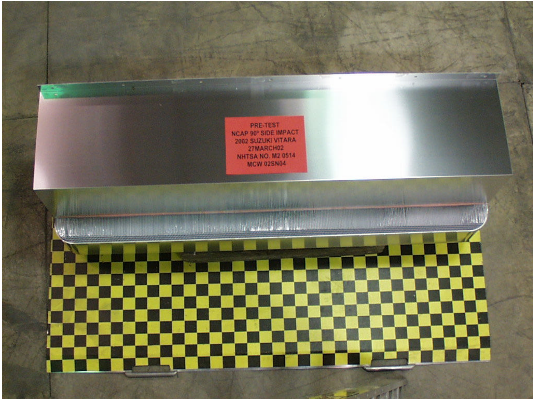
Figure A-51: PRE-TEST ALUMINUM BARRIER OVERHEAD
