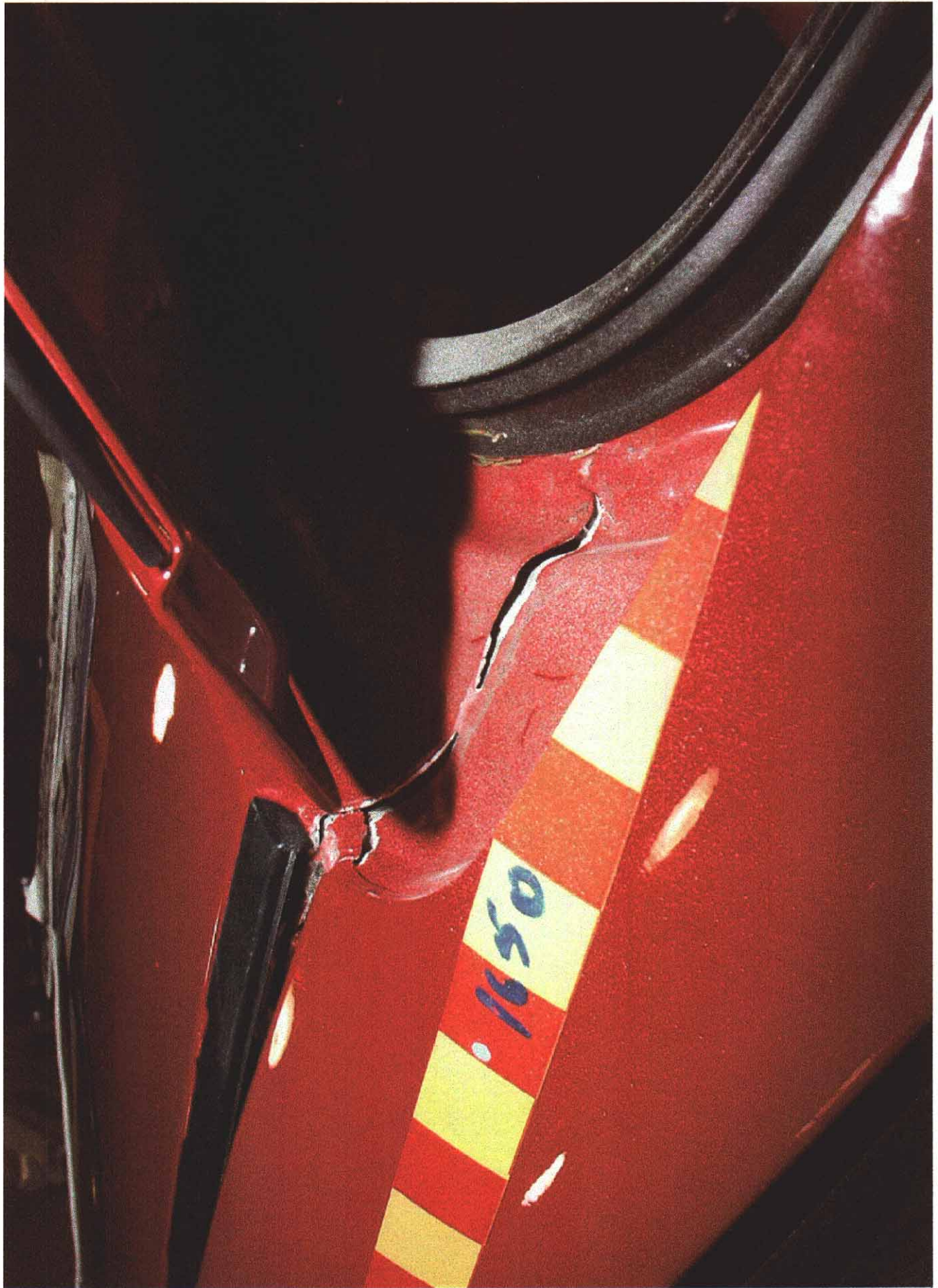
Roof Separation View of Test Vehicle
