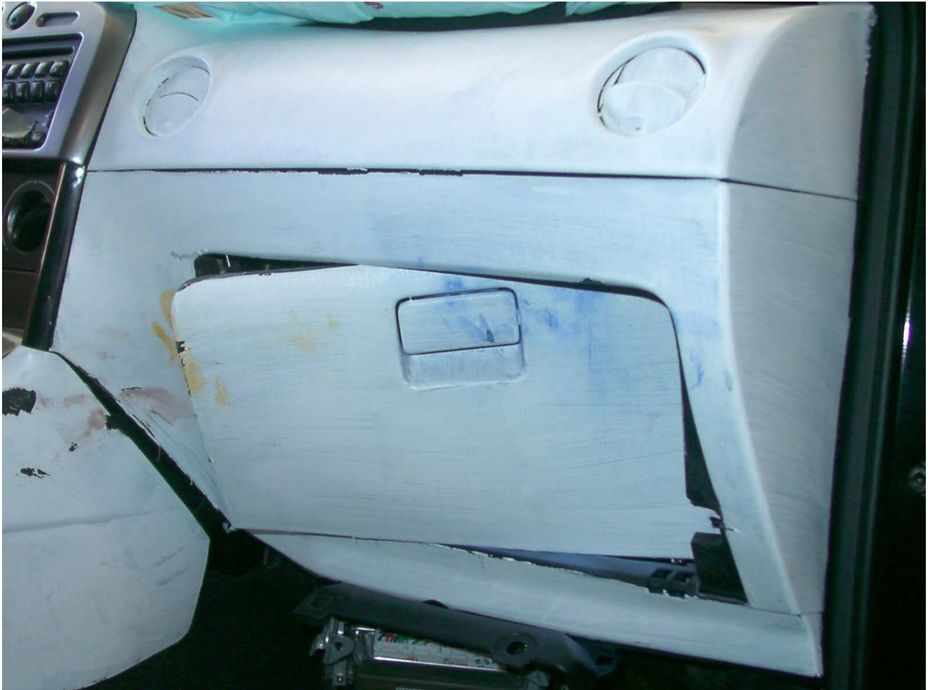
Figure A-54: Passenger Side Knee Bolster, Post-Test
