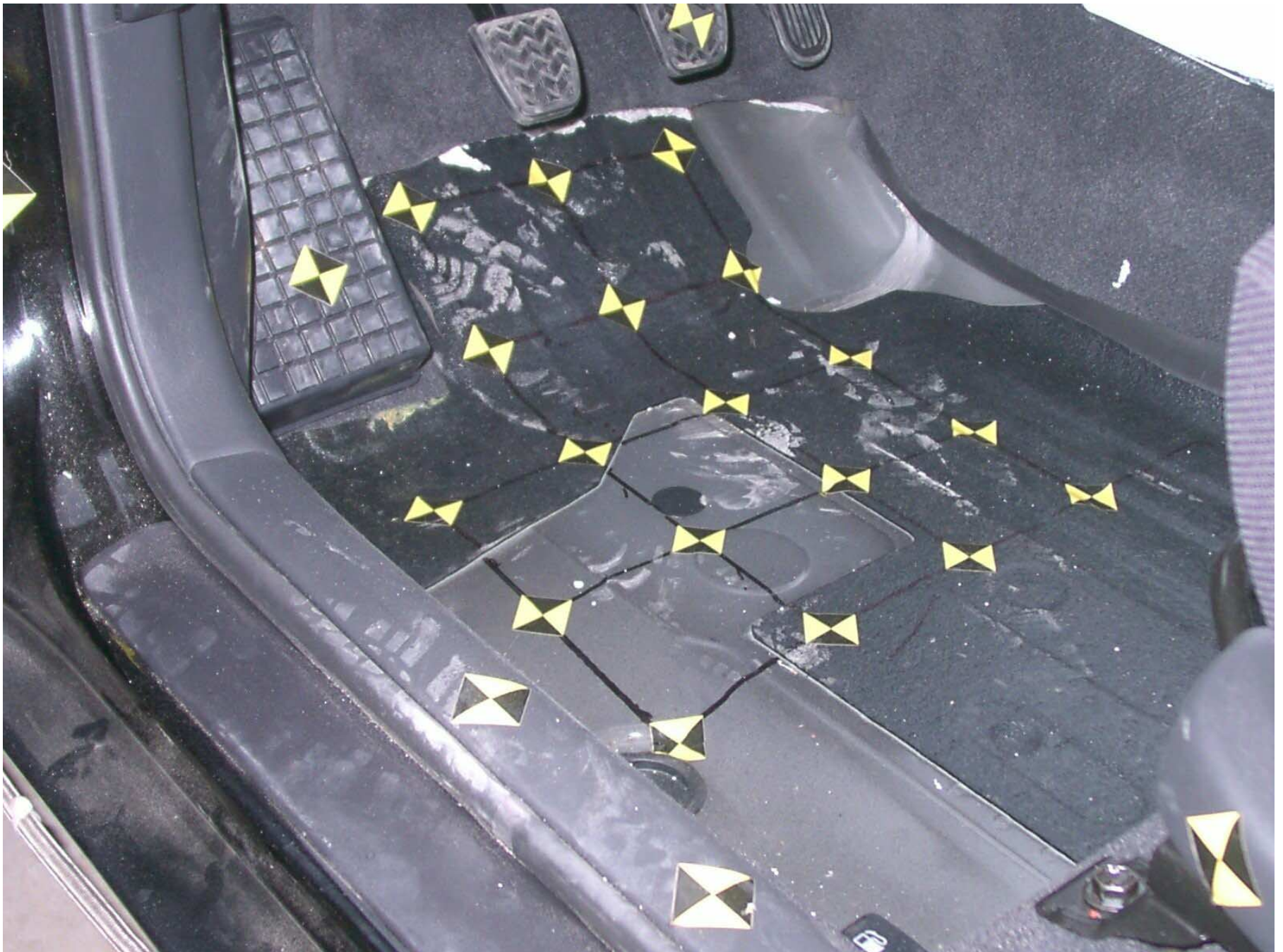
Figure A-37: Driver Side Floor Pan, Pre-Test
