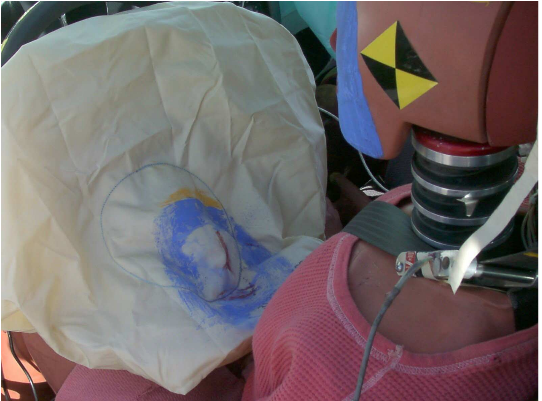
Figure A-40: Driver Dummy Contact, Post-Test
