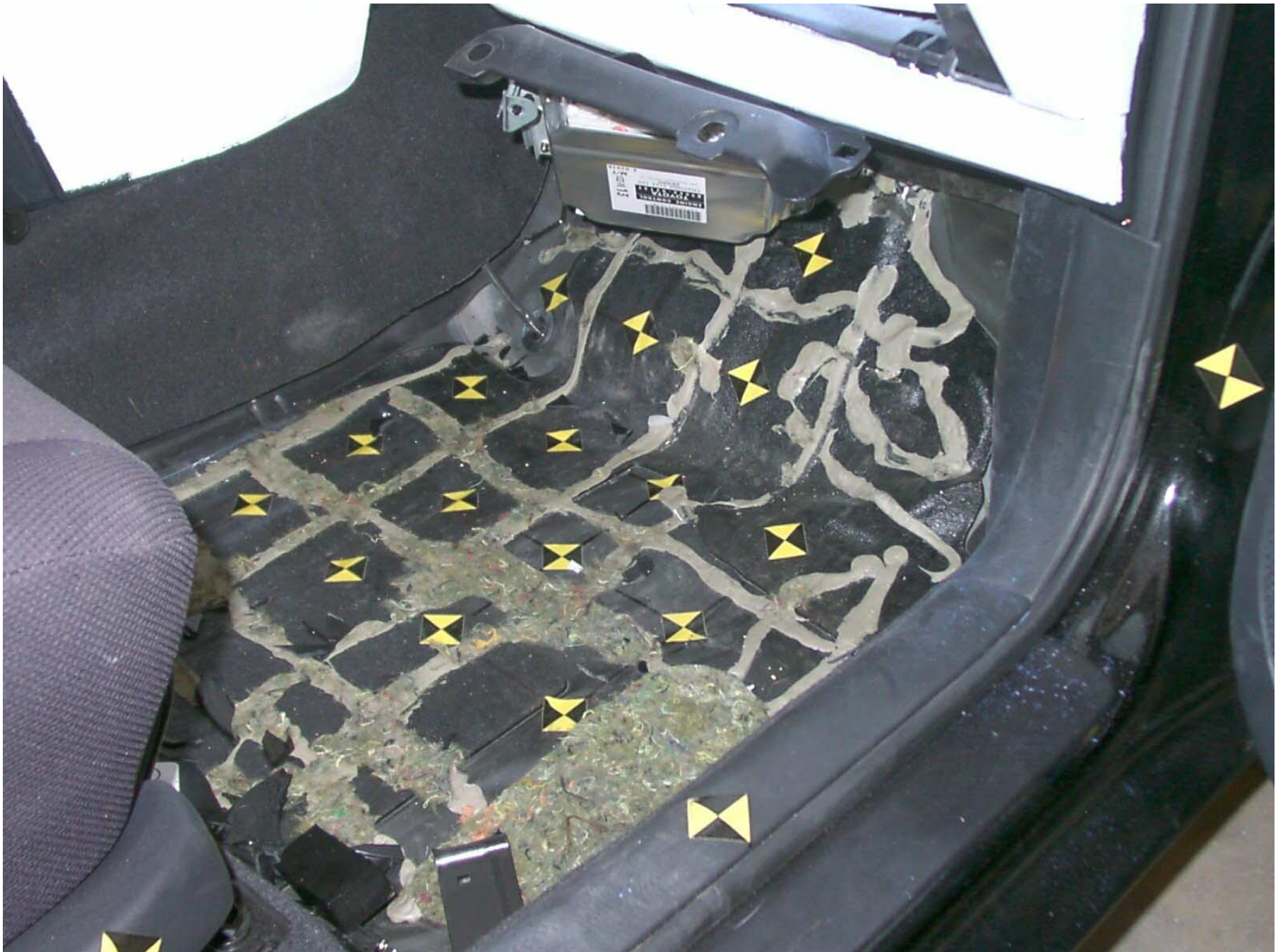
Figure A-52: Passenger Side Floor Pan, Post-Test
