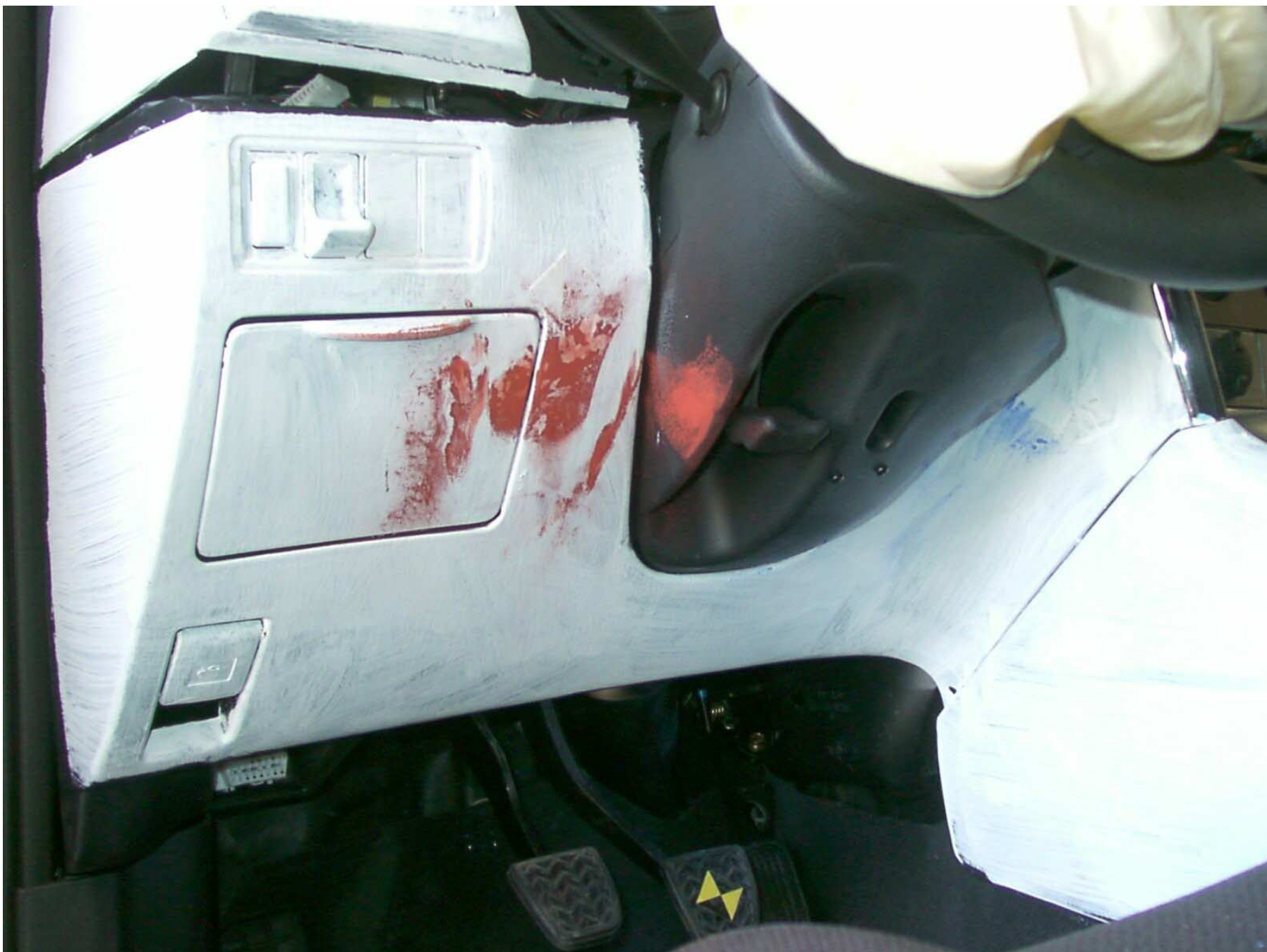
Figure A-36: Driver Side Knee Bolster, Post-Test
