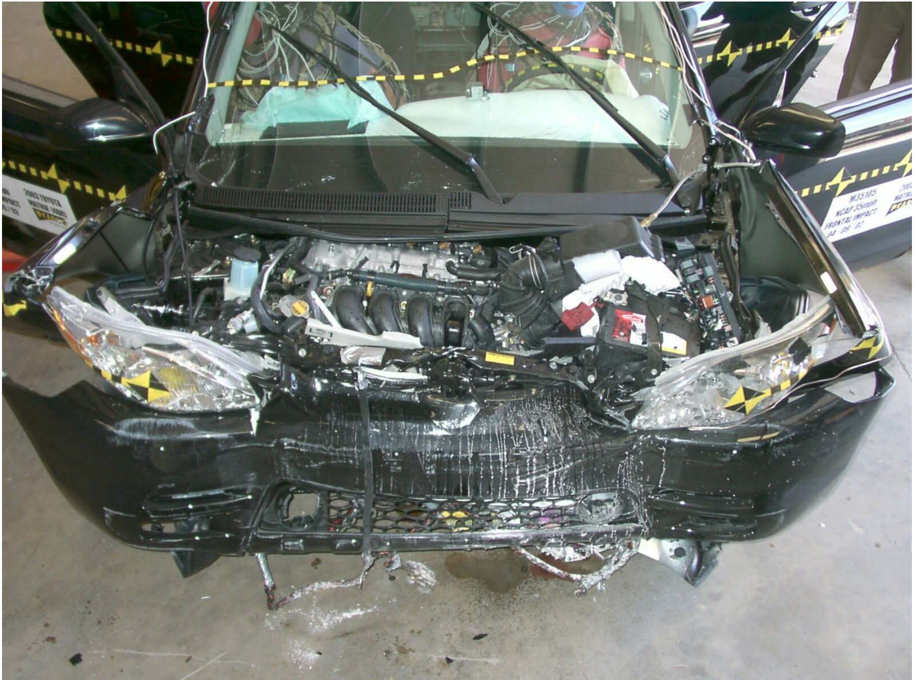
Figure A-18: Engine Compartment, Post-Test
