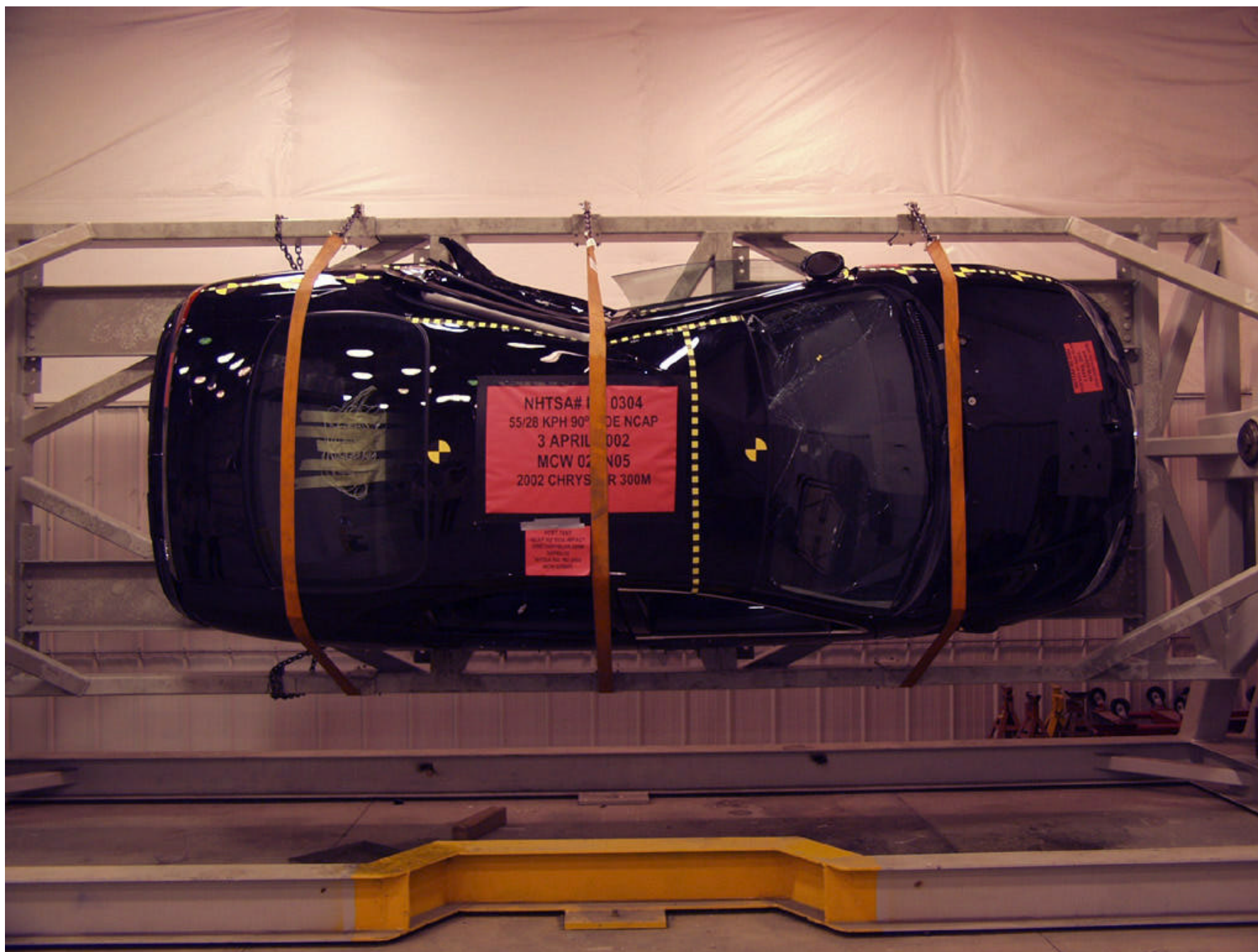
Figure A-43: ROLLOVER 270 DEGREES
