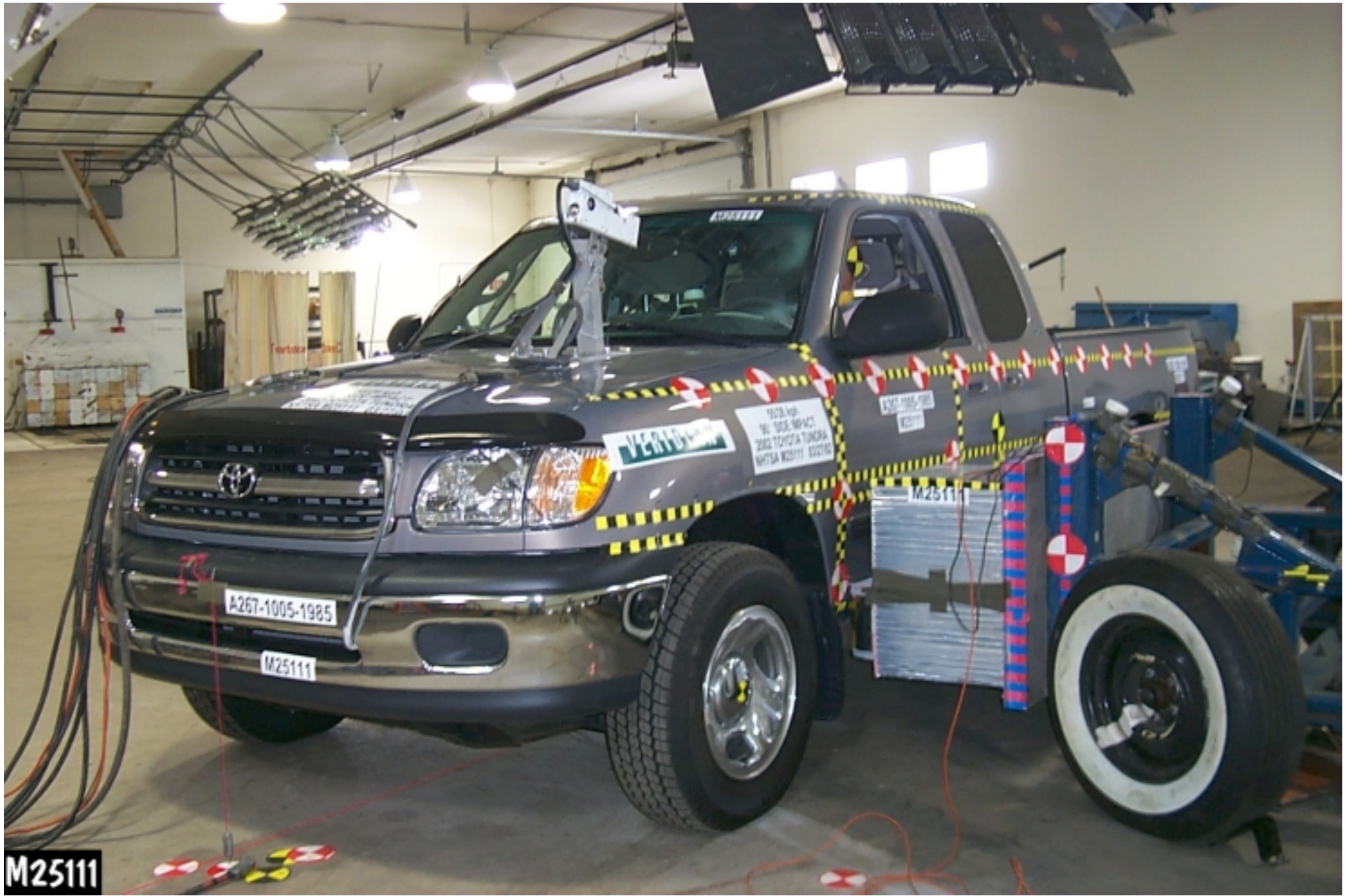
Figure A-31: PRE-TEST LEFT SIDE VIEW OF MDB WITH IMPACTOR FACE IN POSITION
