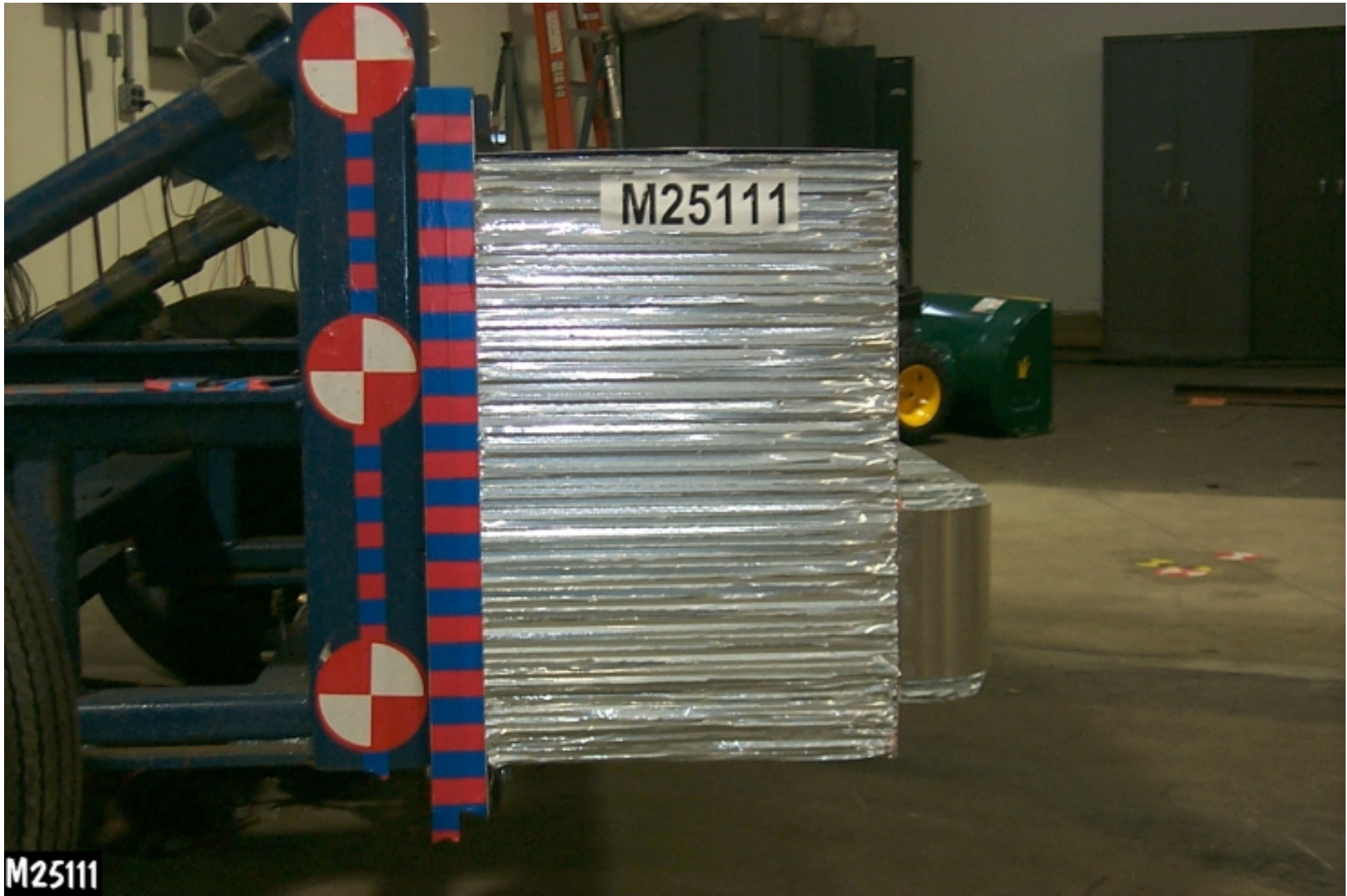
Figure A-19: PRE-TEST RIGHT SIDE VIEW OF IMPACTOR FACE
