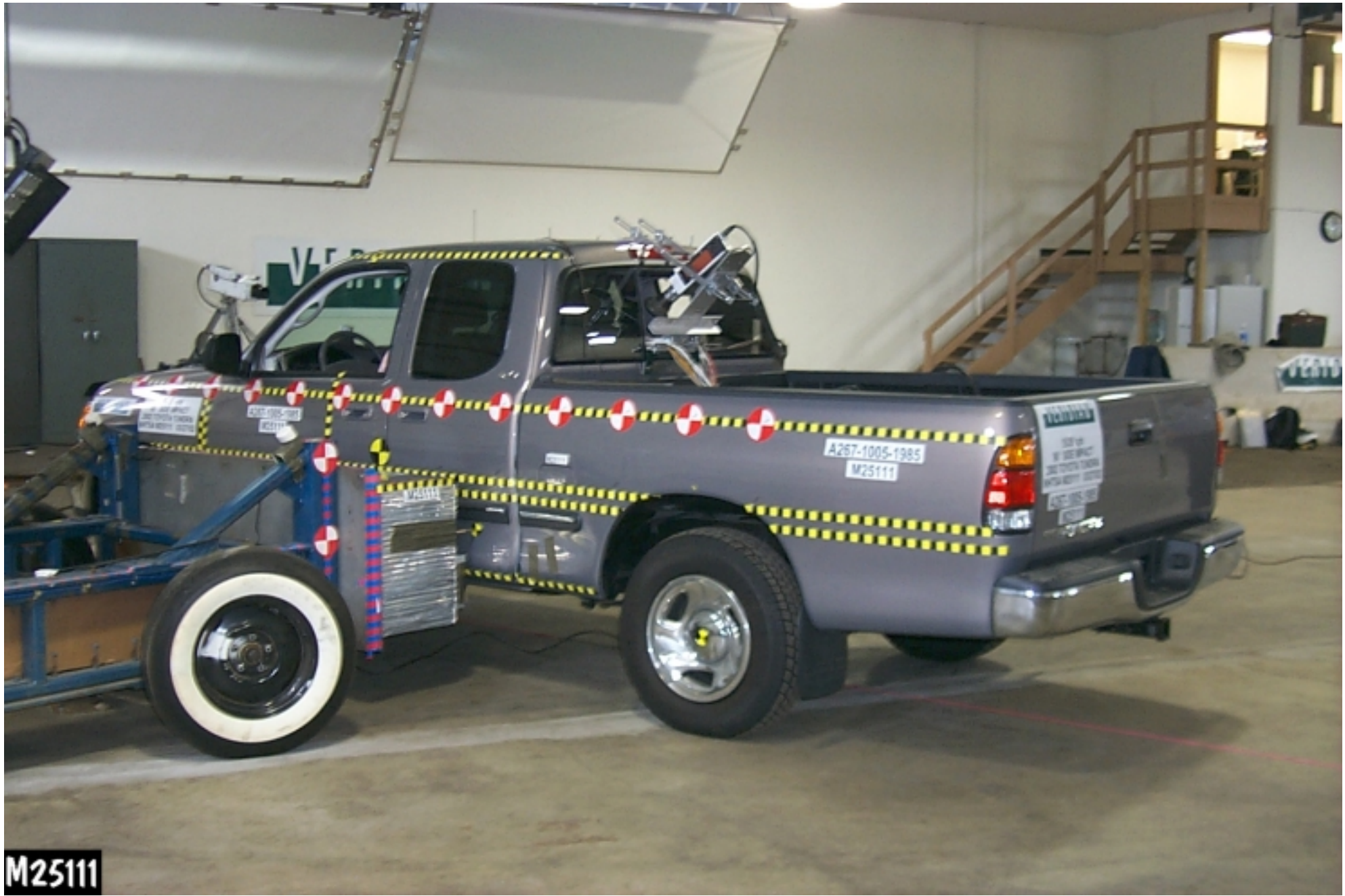
Figure A-32: PRE-TEST RIGHT SIDE VIEW OF MDB WITH IMPACTOR FACE IN POSITION
