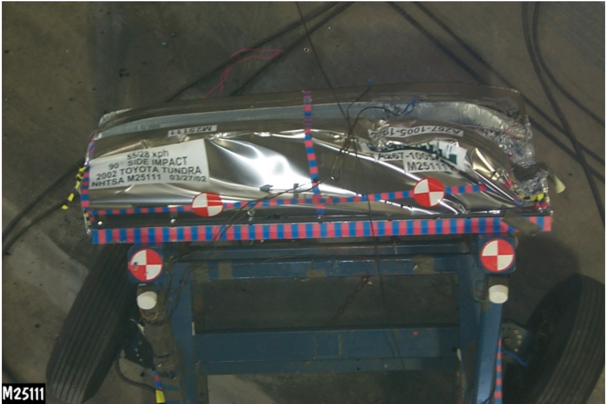
Figure A-22: POST-TEST TOP VIEW OF IMPACTOR FACE
