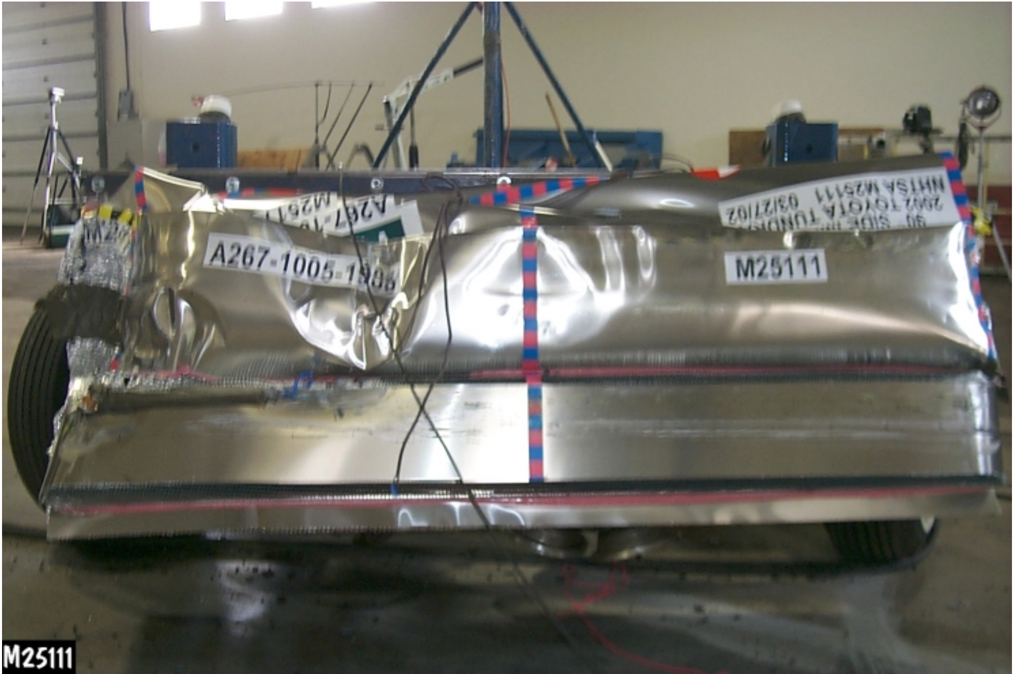
Figure A-16: POST-TEST FRONTAL VIEW OF IMPACTOR FACE
