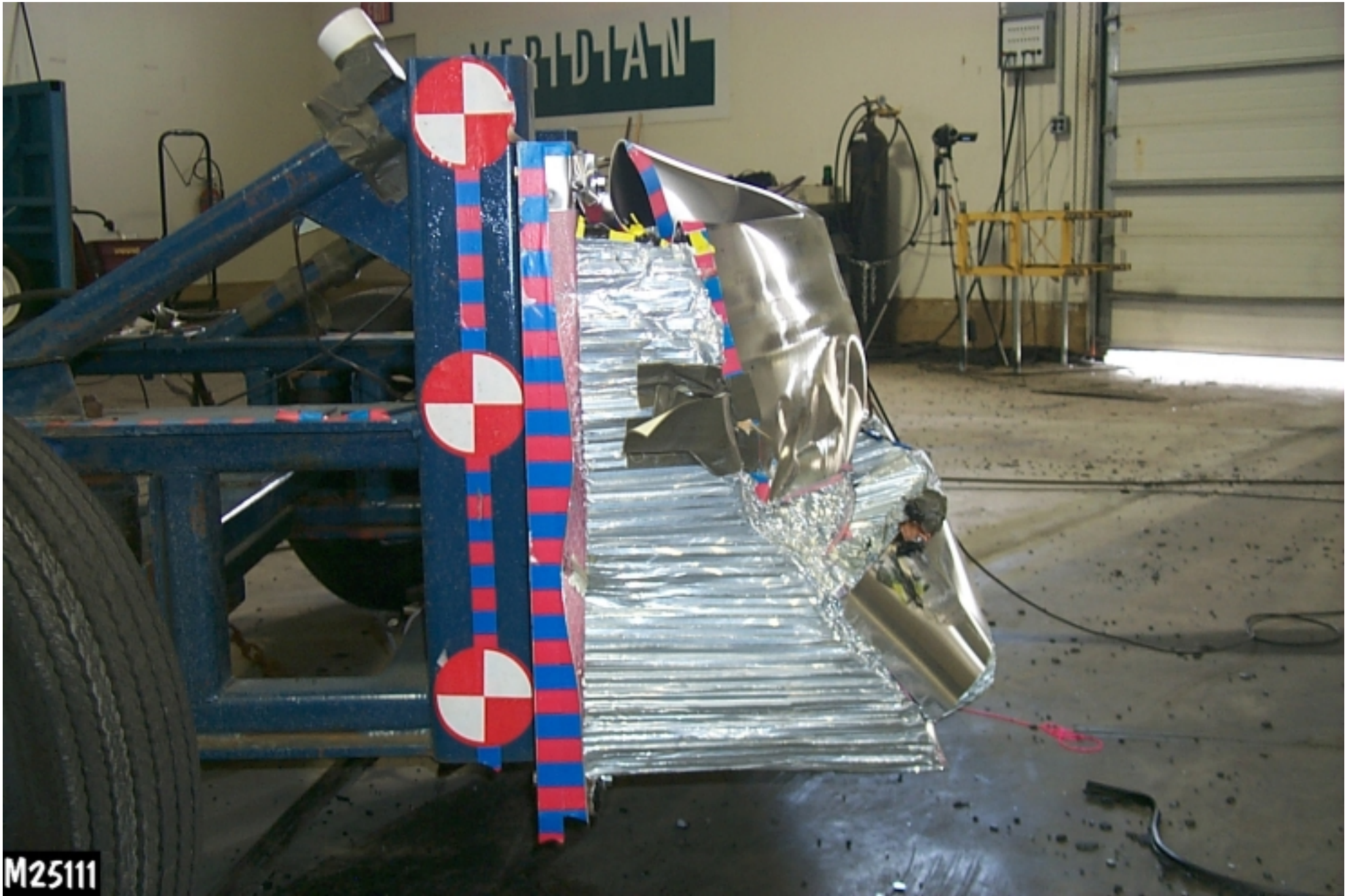
Figure A-20: POST-TEST RIGHT SIDE VIEW OF IMPACTOR FACE
