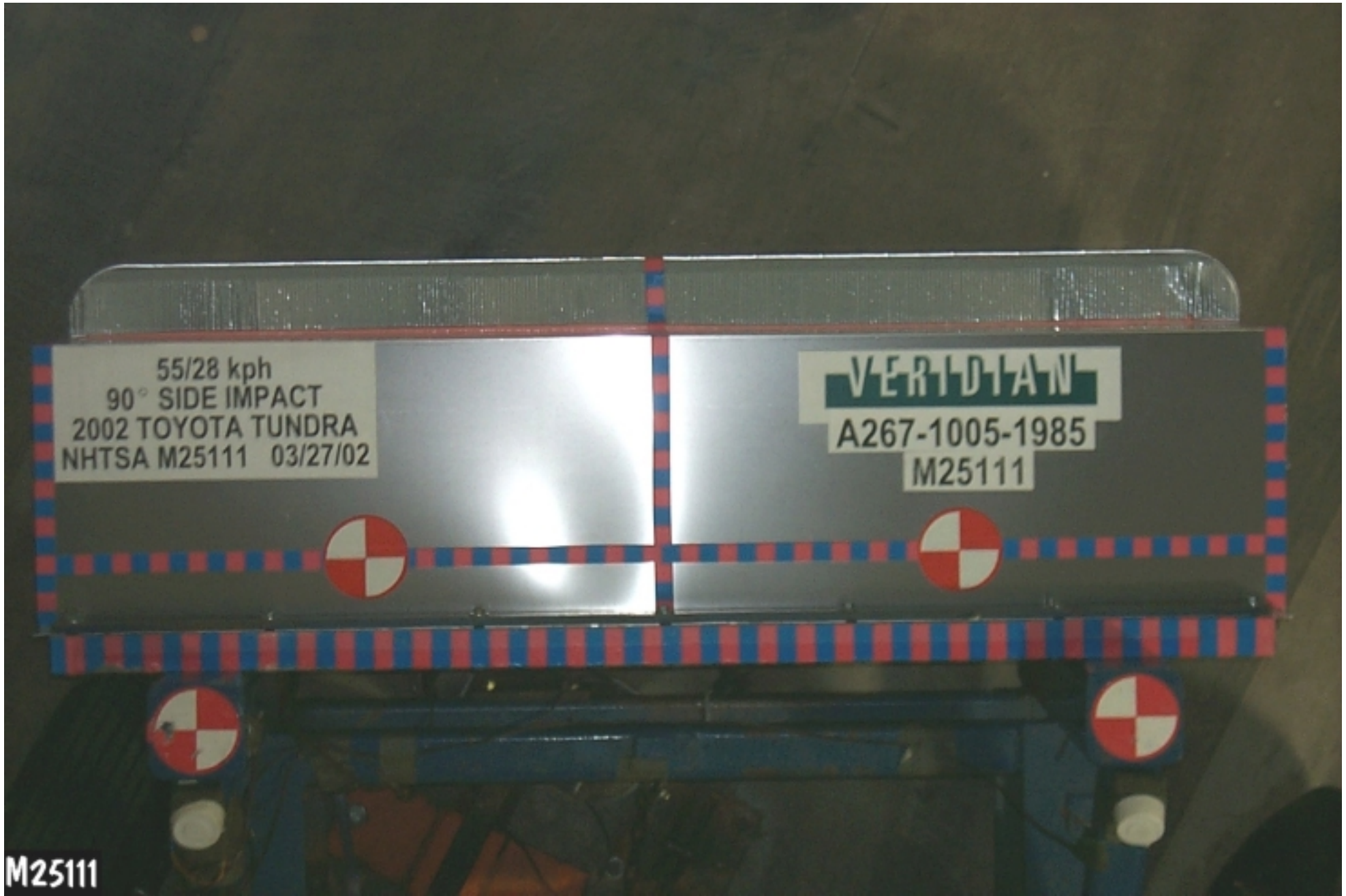
Figure A-21: PRE-TEST TOP VIEW OF IMPACTOR FACE
