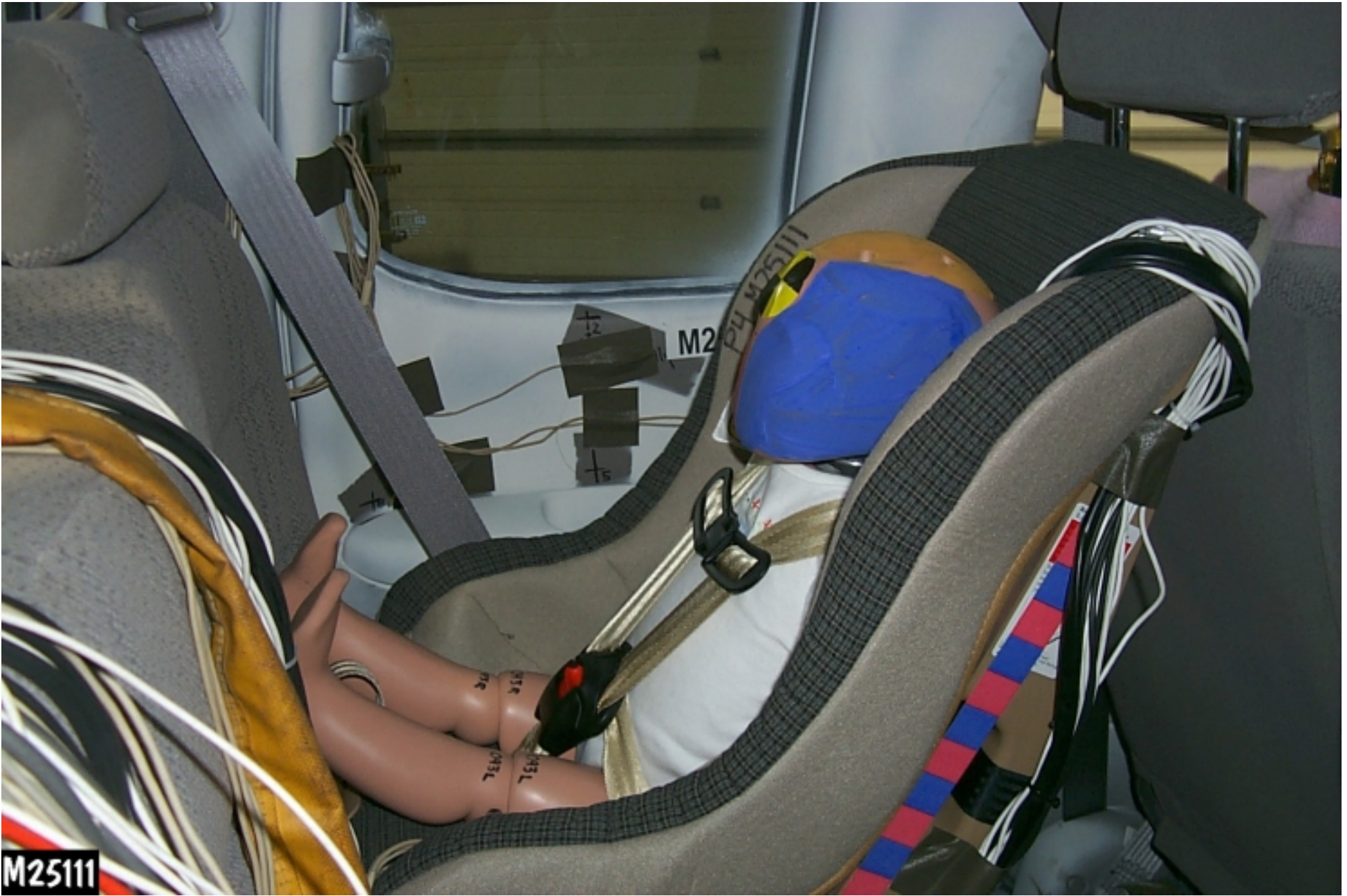
Figure 3-25: PRE-TEST POSITION 4 RIGHT SIDE VIEW
