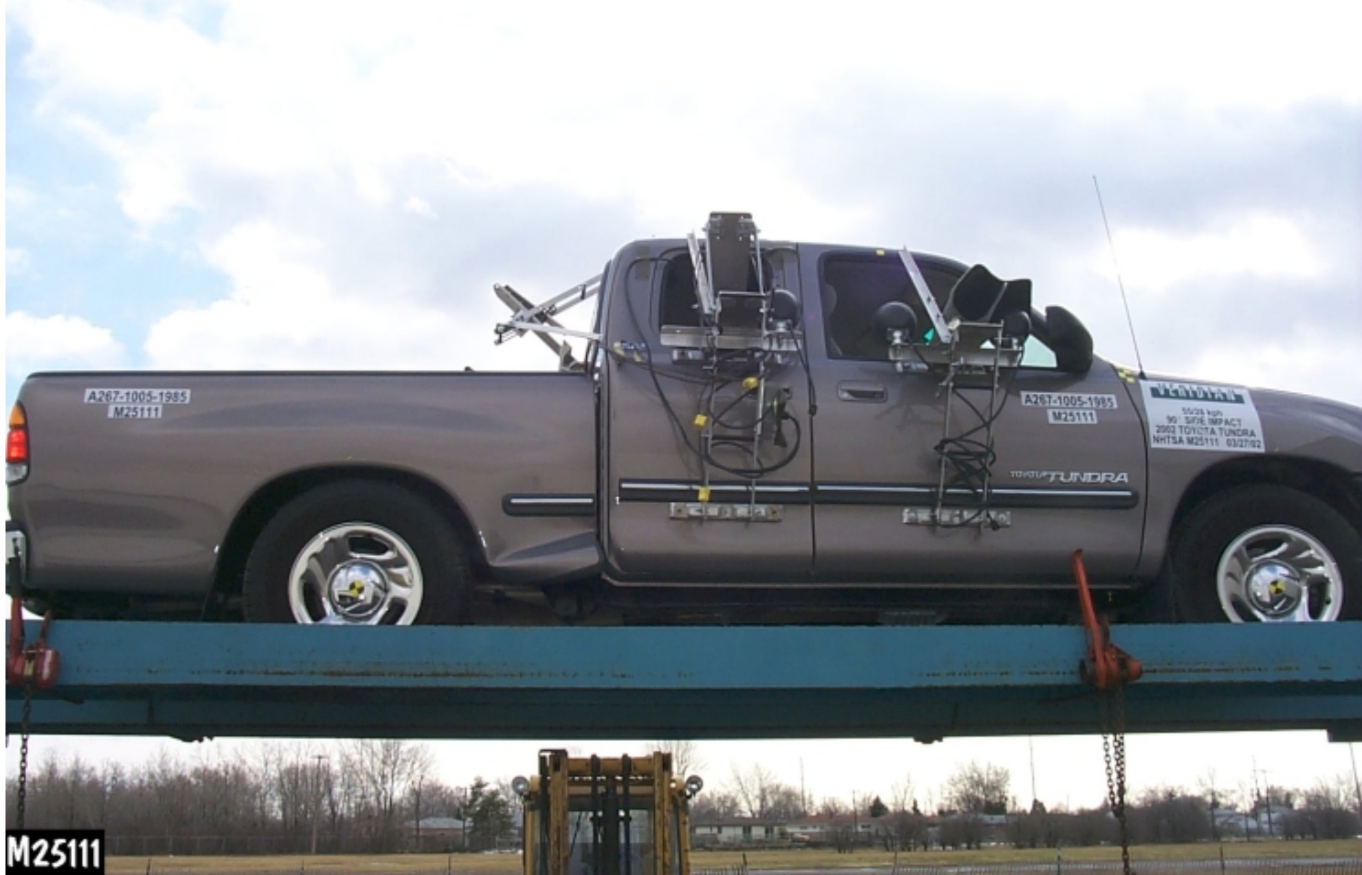
Figure A-40: ROLLOVER 360 DEGREES
