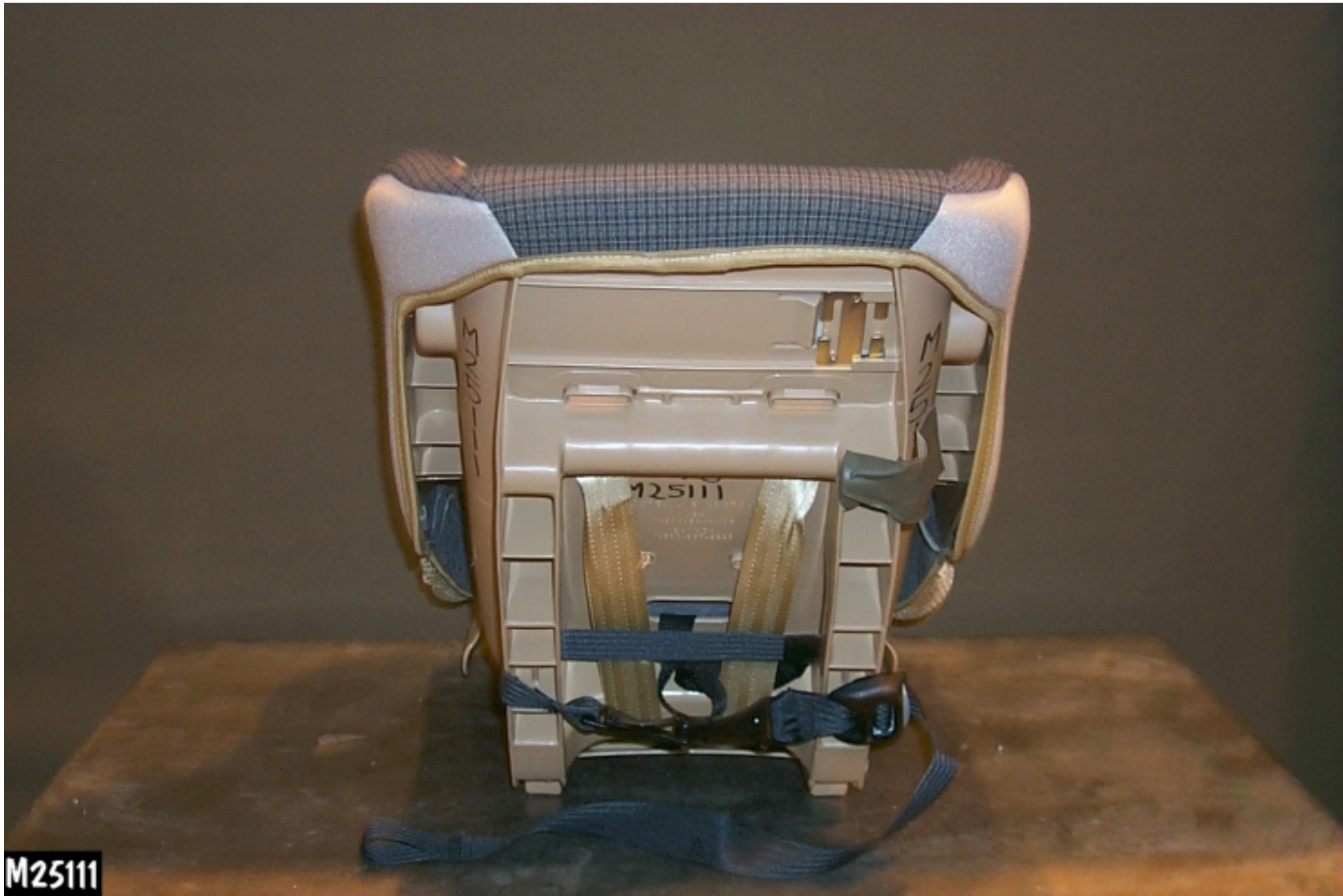
Figure 3-5: POST-TEST REAR VIEW OF POSITION 3 CRS
