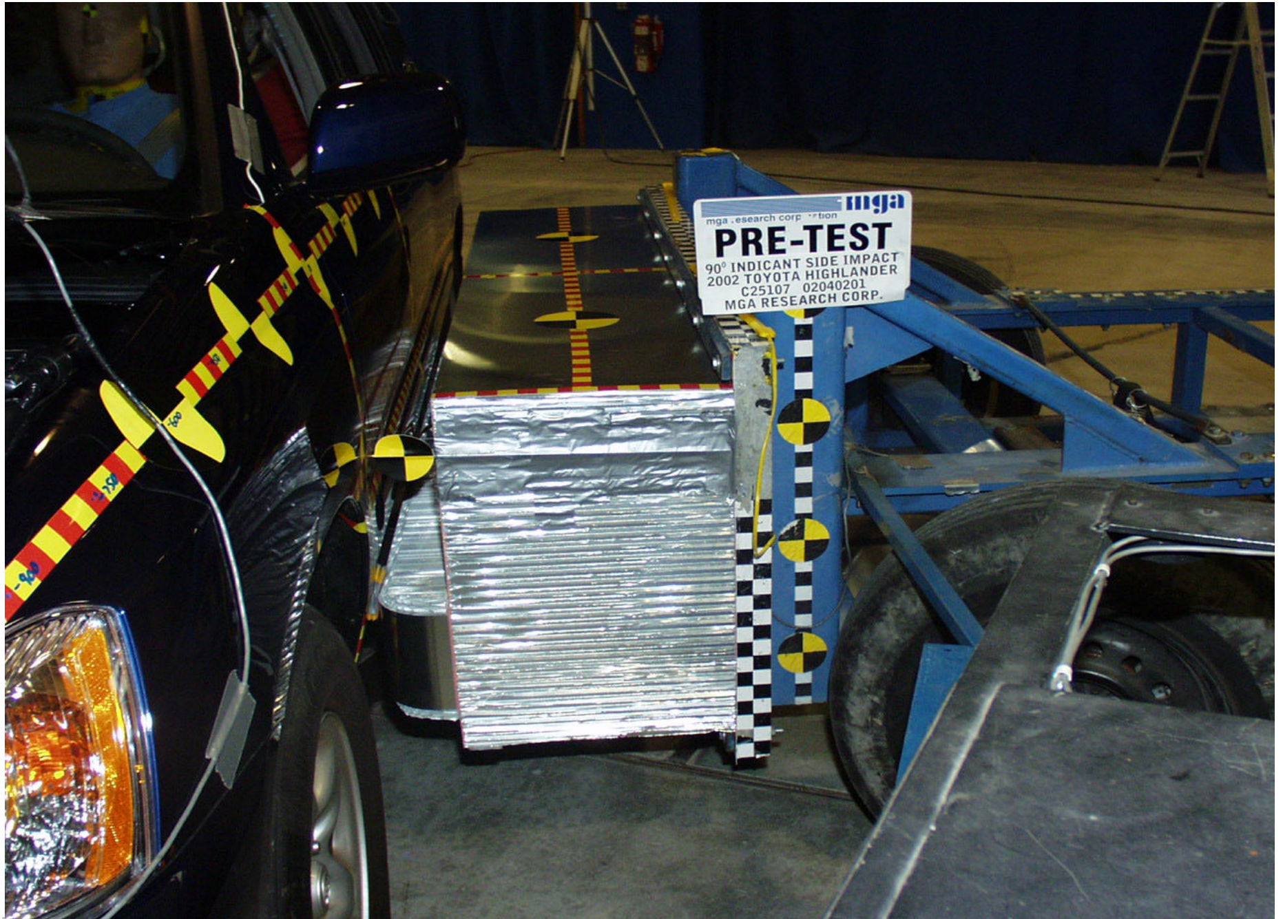
Pre-Test MDB Positioned Against Vehicle (left side)
