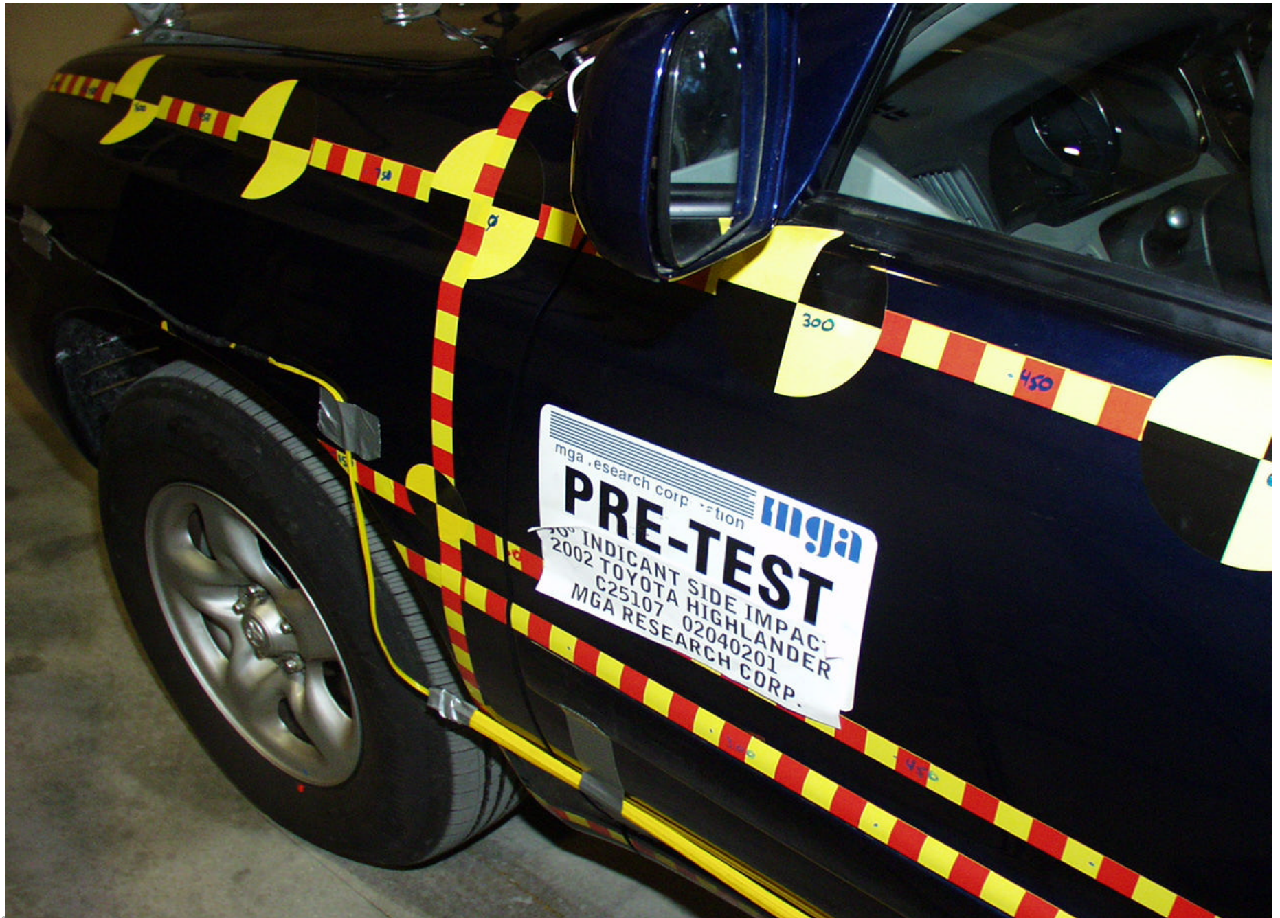
Pre-Test Left Front Impact Point on Vehicle
