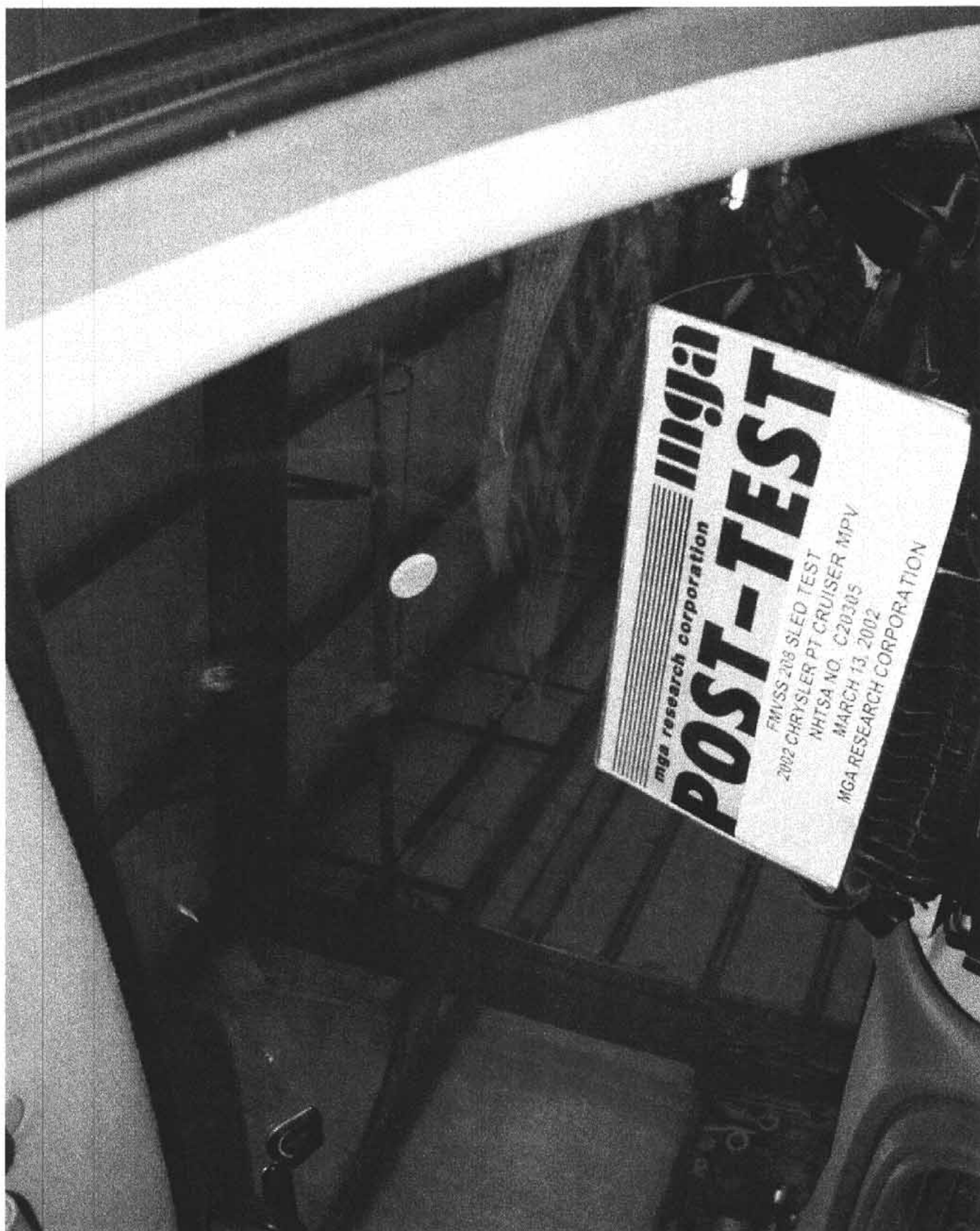
Photo No. A-20 - Post-Test Passenger Head Contact View (windshield)
