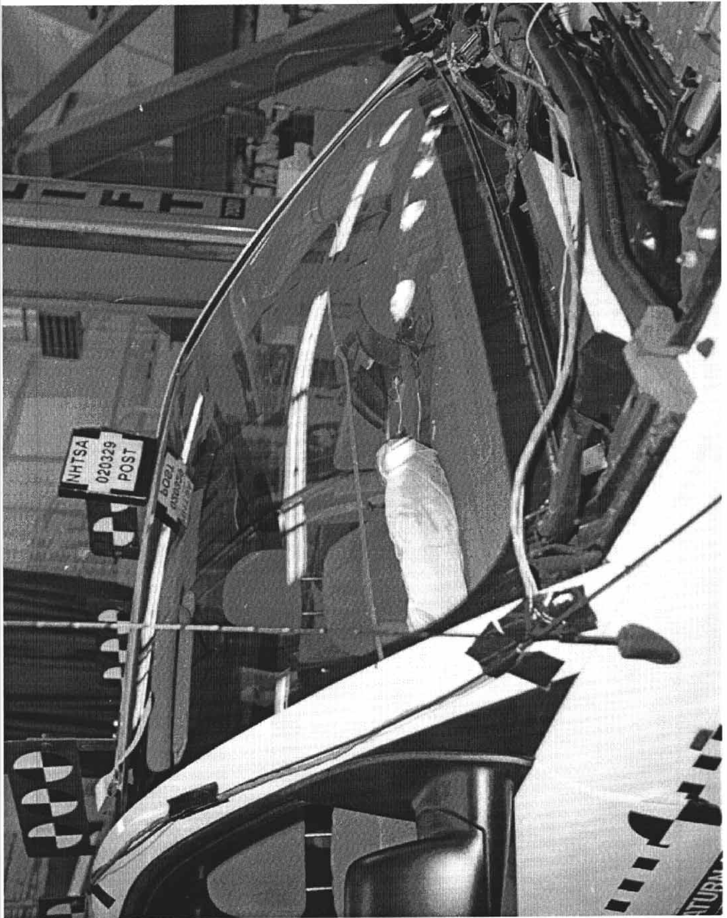
Figure A-15. Post-Test Right Windshield View with Cowl Removed
