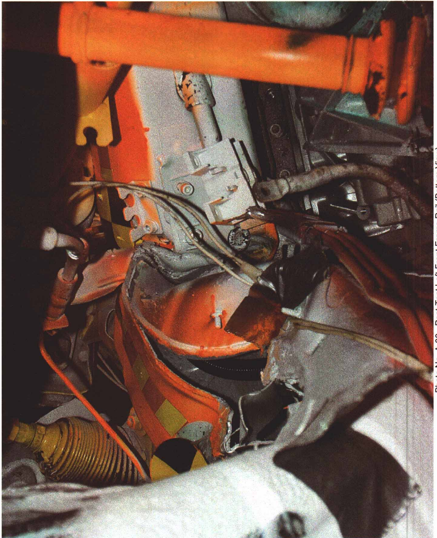
Photo No. A-38 - Post-Test Left Front Frame Rail (Bottom View)
