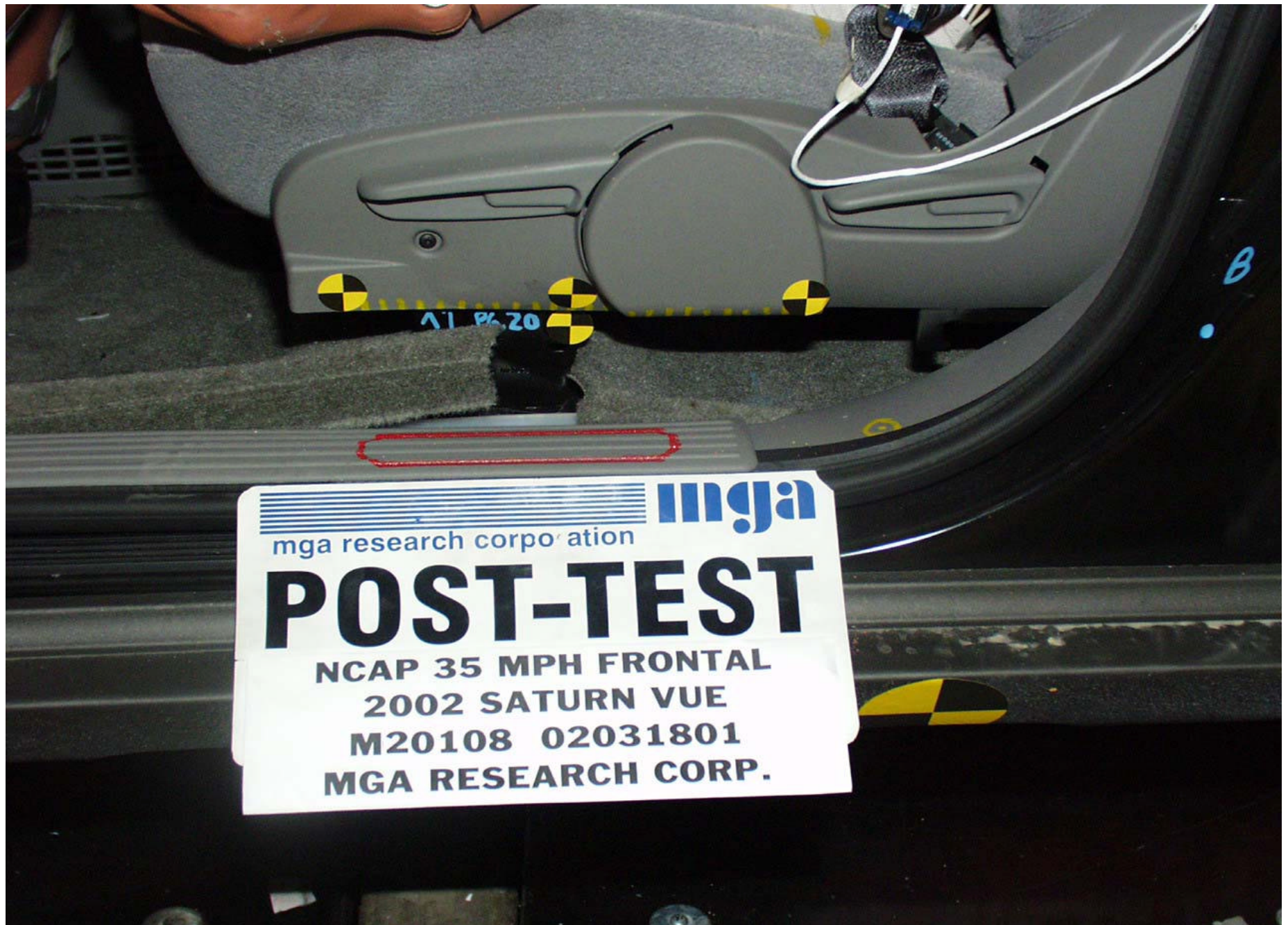
Post-Test Driver Seat Position View
