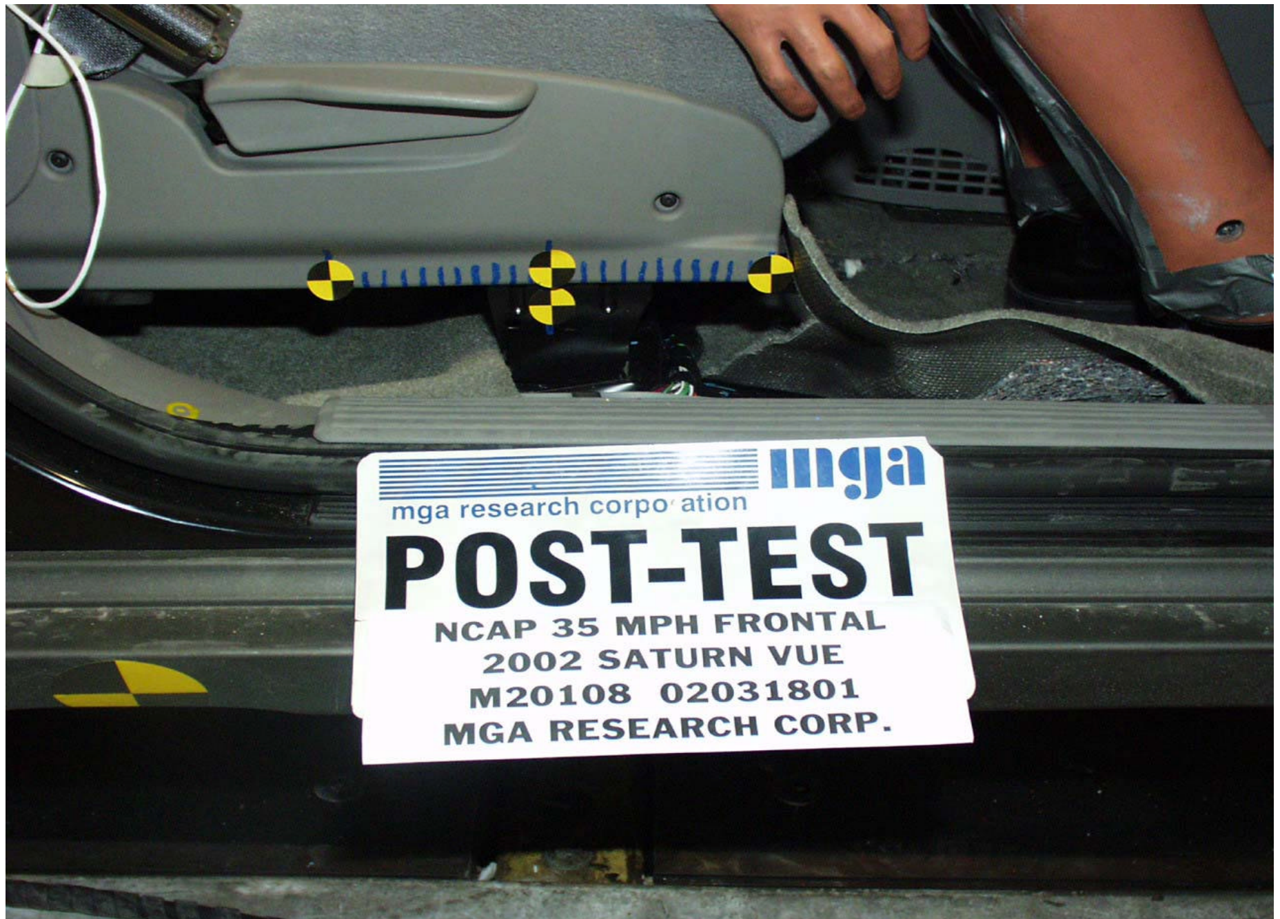
Post-Test Passenger Seat Position View
