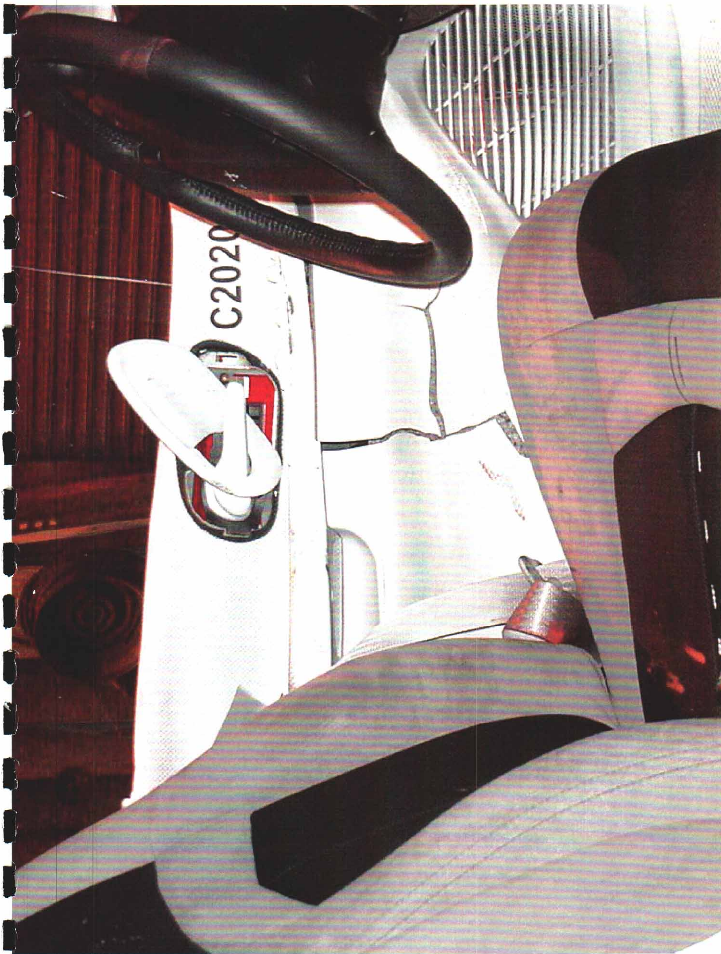
Figure A-22 POST-TEST INTERIOR OF FRONT DOOR SHOWING SID IMPACT LOCATIONS
