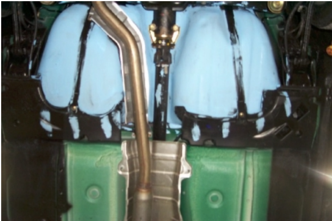
Filler and vapor pipe.
