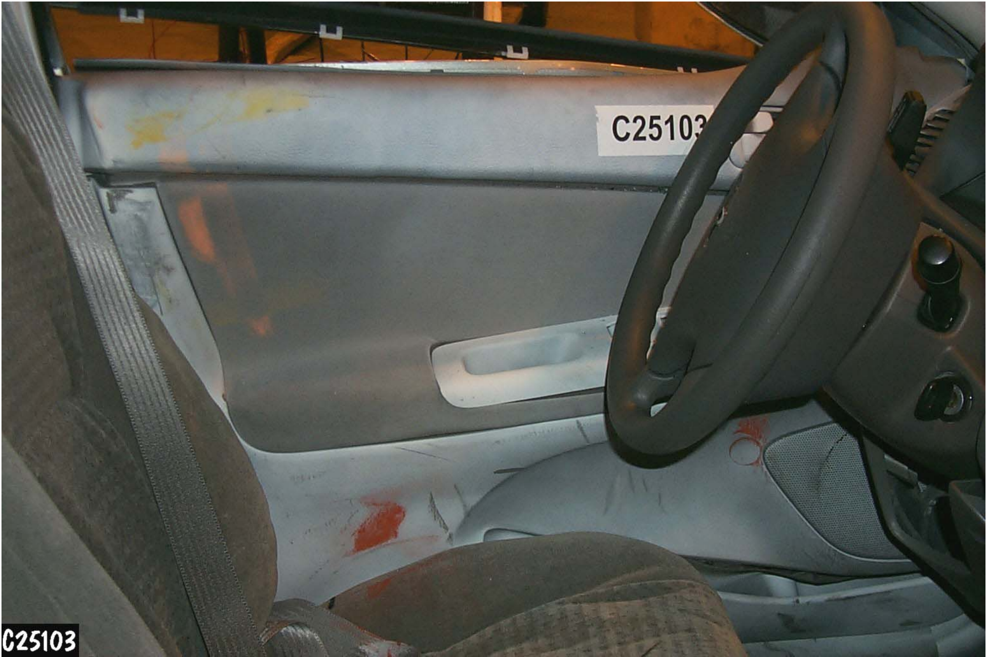
Figure A-26: POST-TEST FRONT INTERIOR TRIM SHOWING SID IMPACT LOCATIONS
