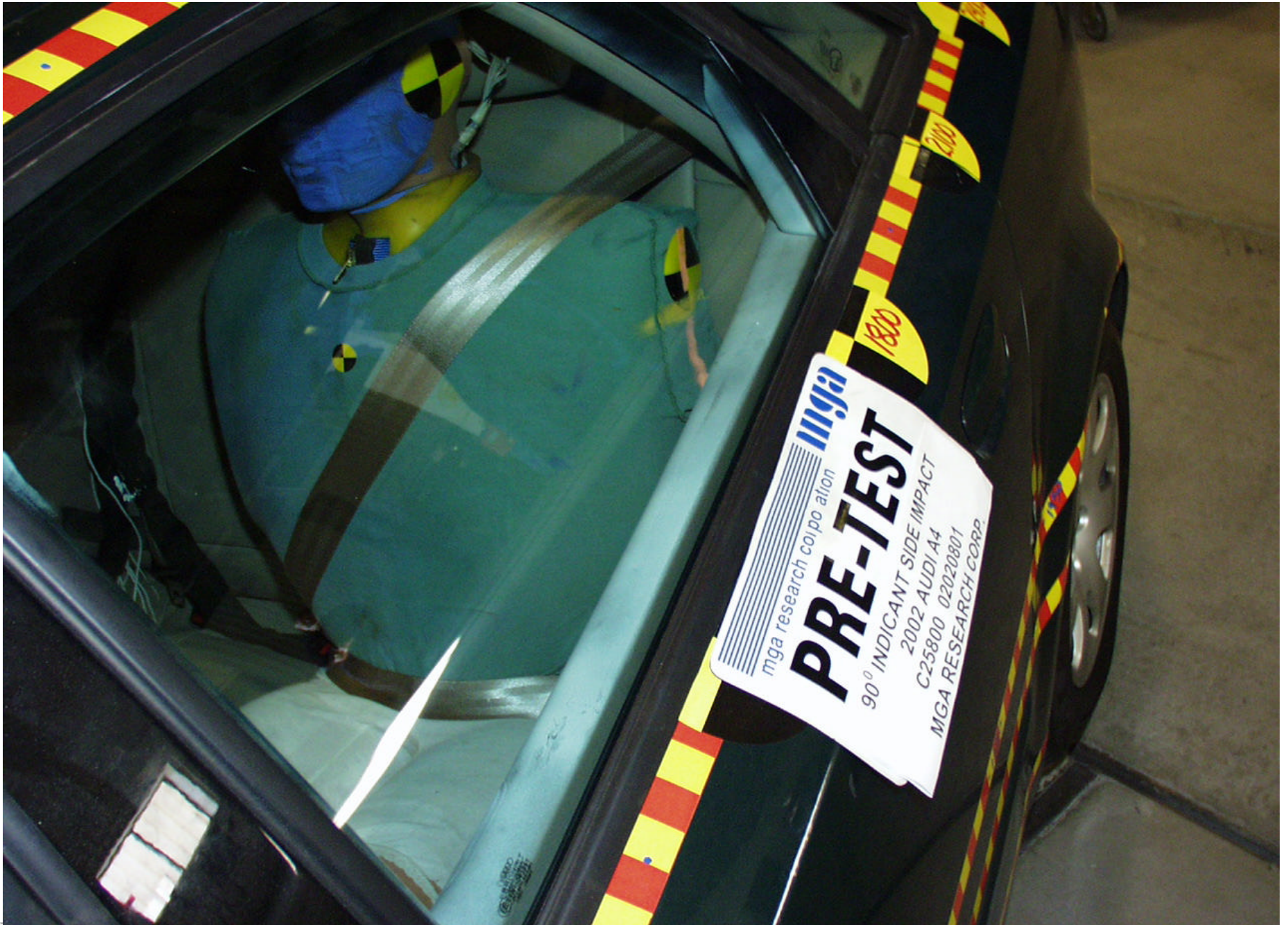
Pre-Test Passenger Dummy Shoulder and Door Top View
