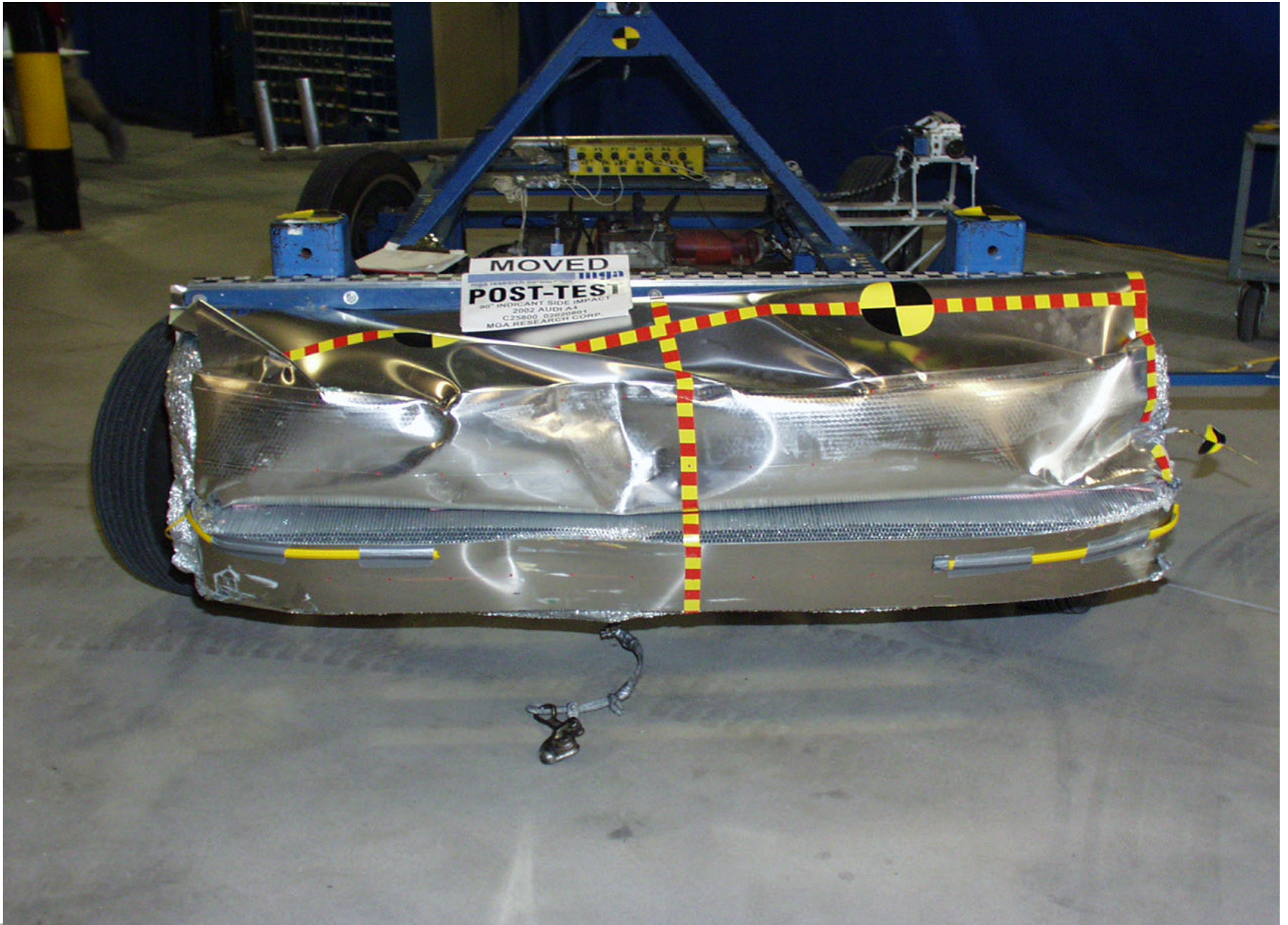
Post-Test MDB Front View
