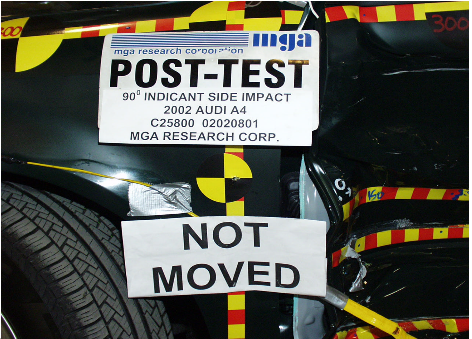
Post-Test Left Front Impact Point on Vehicle
