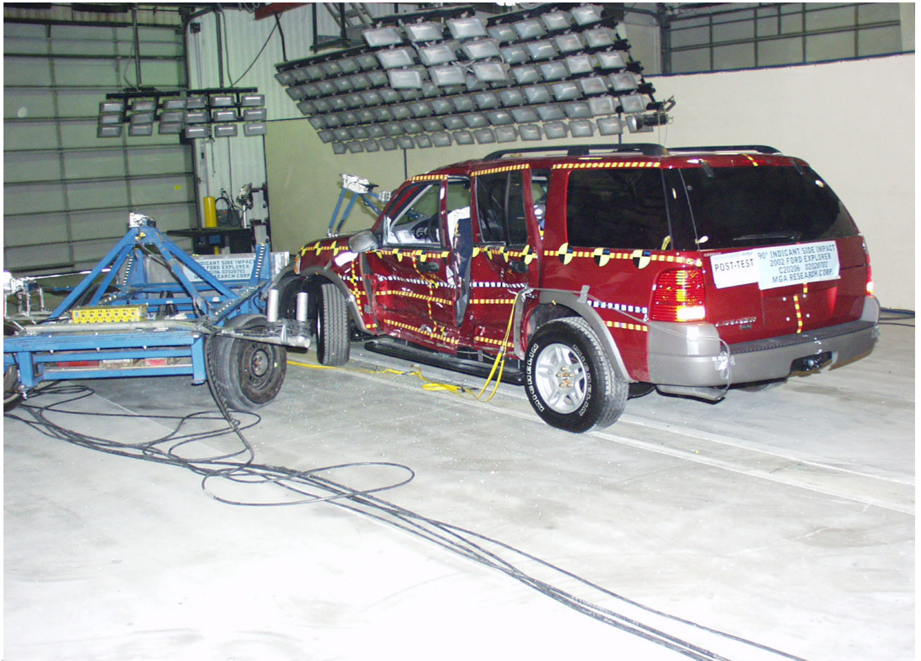
Post-Test MDB and Vehicle (right side)
