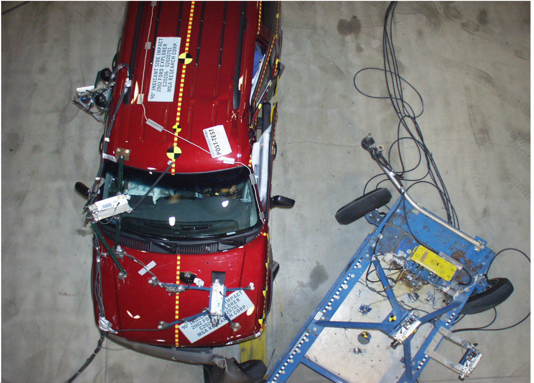
Post-Test MDB and Vehicle Overhead View
