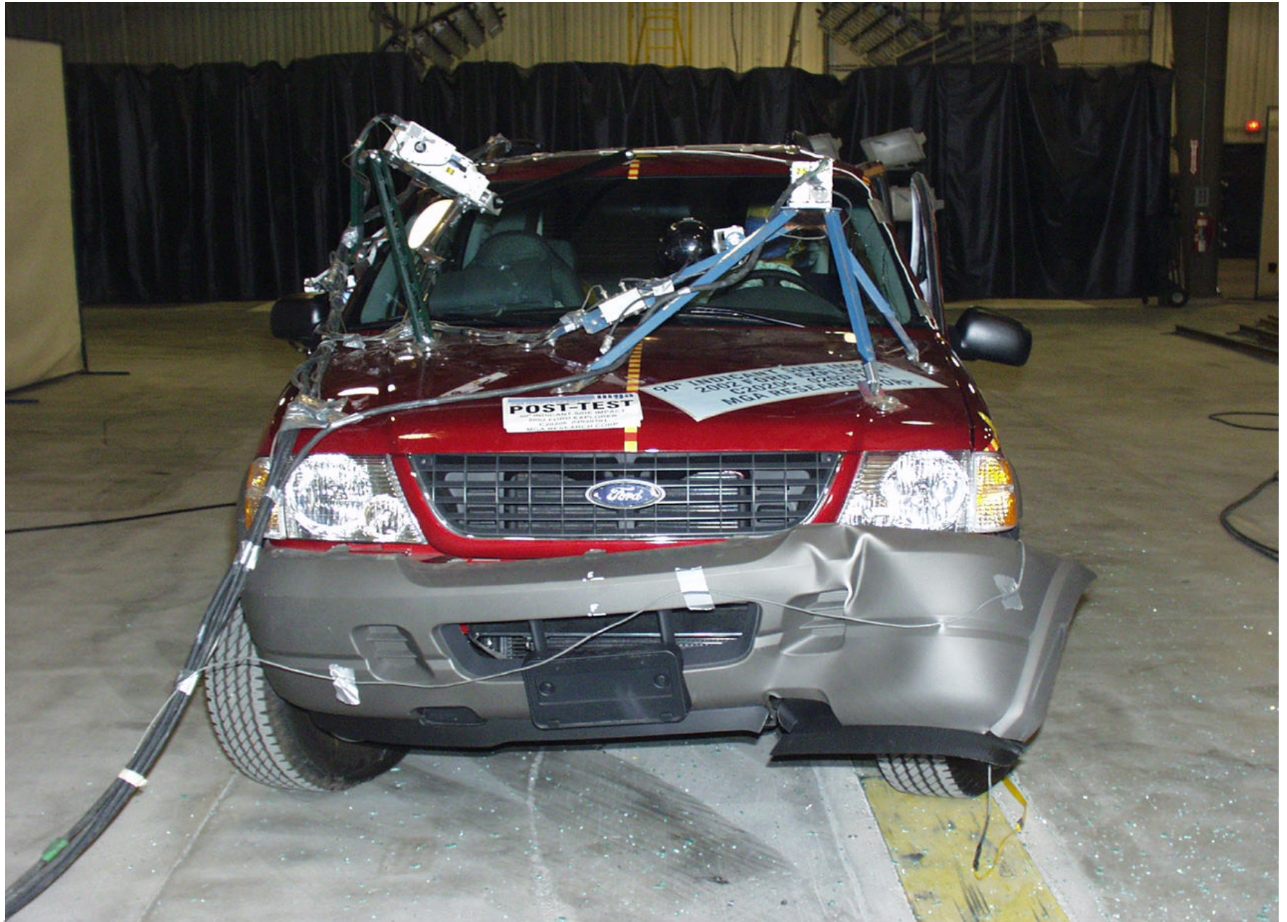
Post-Test Front View of Test Vehicle
