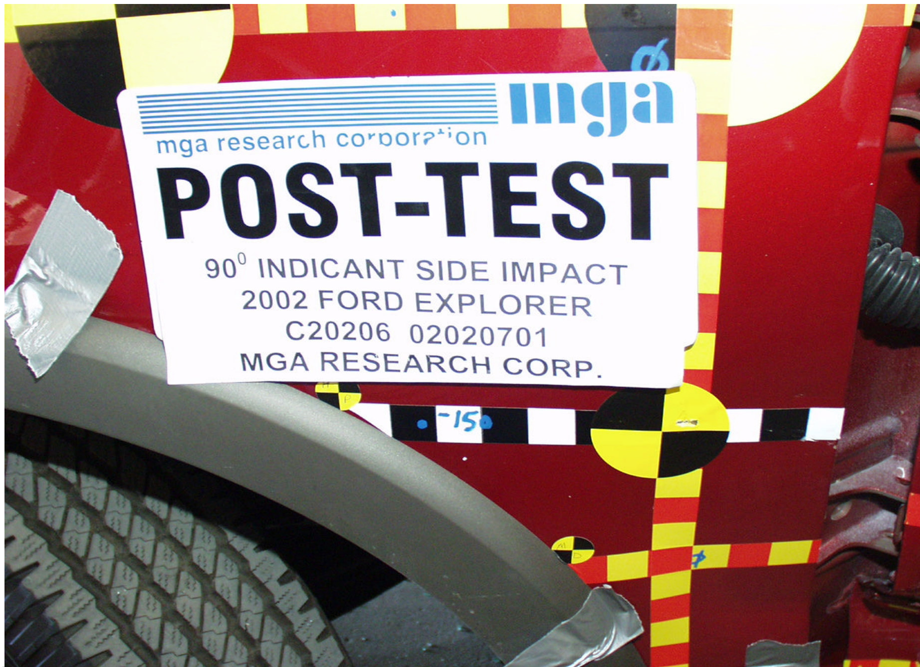
Post-Test Left Front Impact Point on Vehicle
