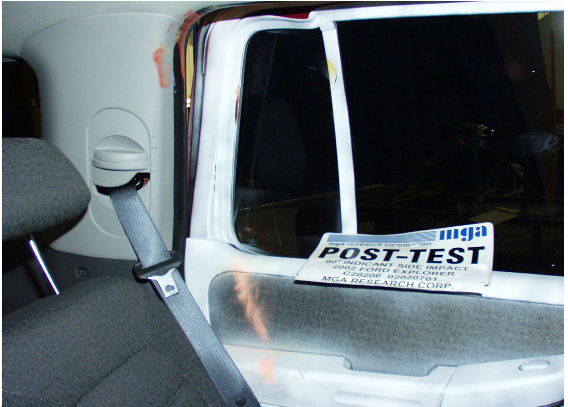
Post-Test Passenger Dummy Head Contact
