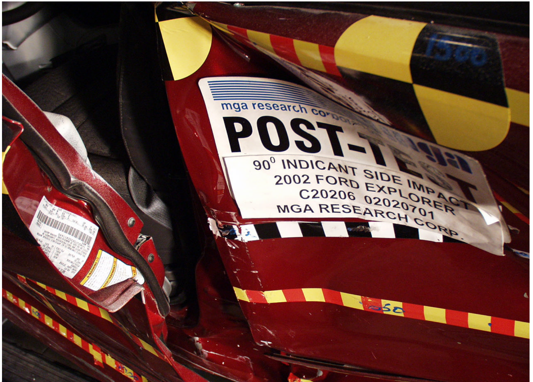
Post-Test Door Opening from Outside
