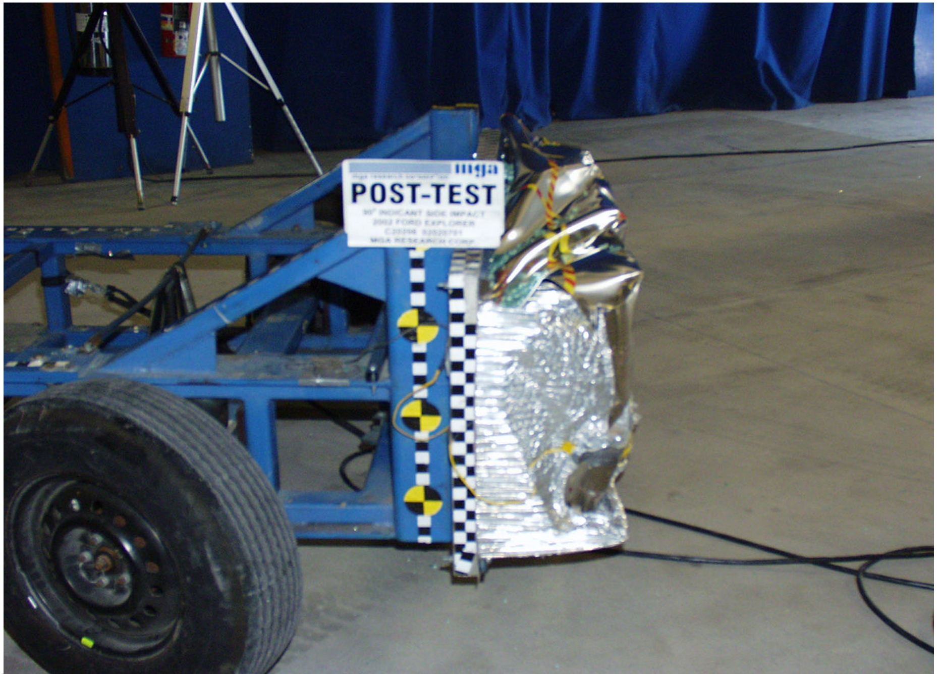
Post-Test MDB Right Side View
