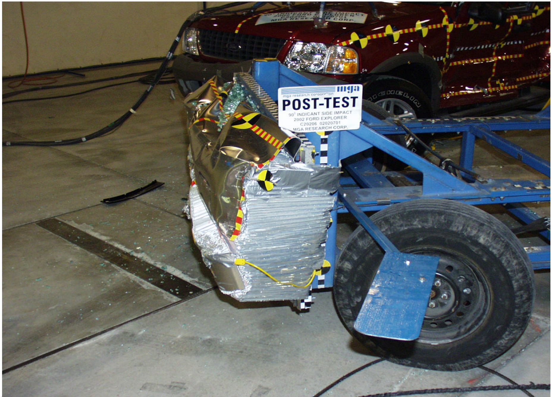
Post-Test MDB Left Side View
