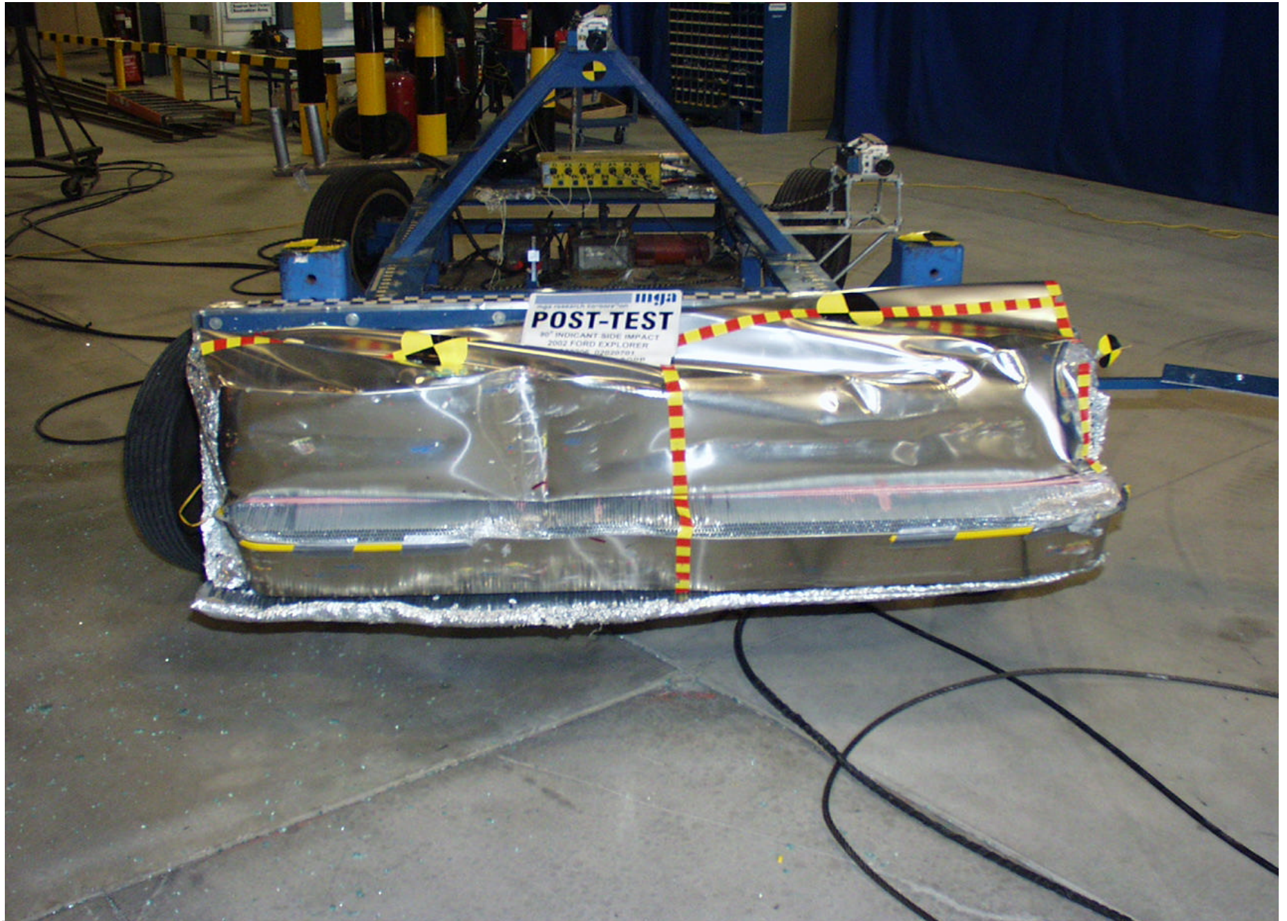
Post-Test MDB Front View
