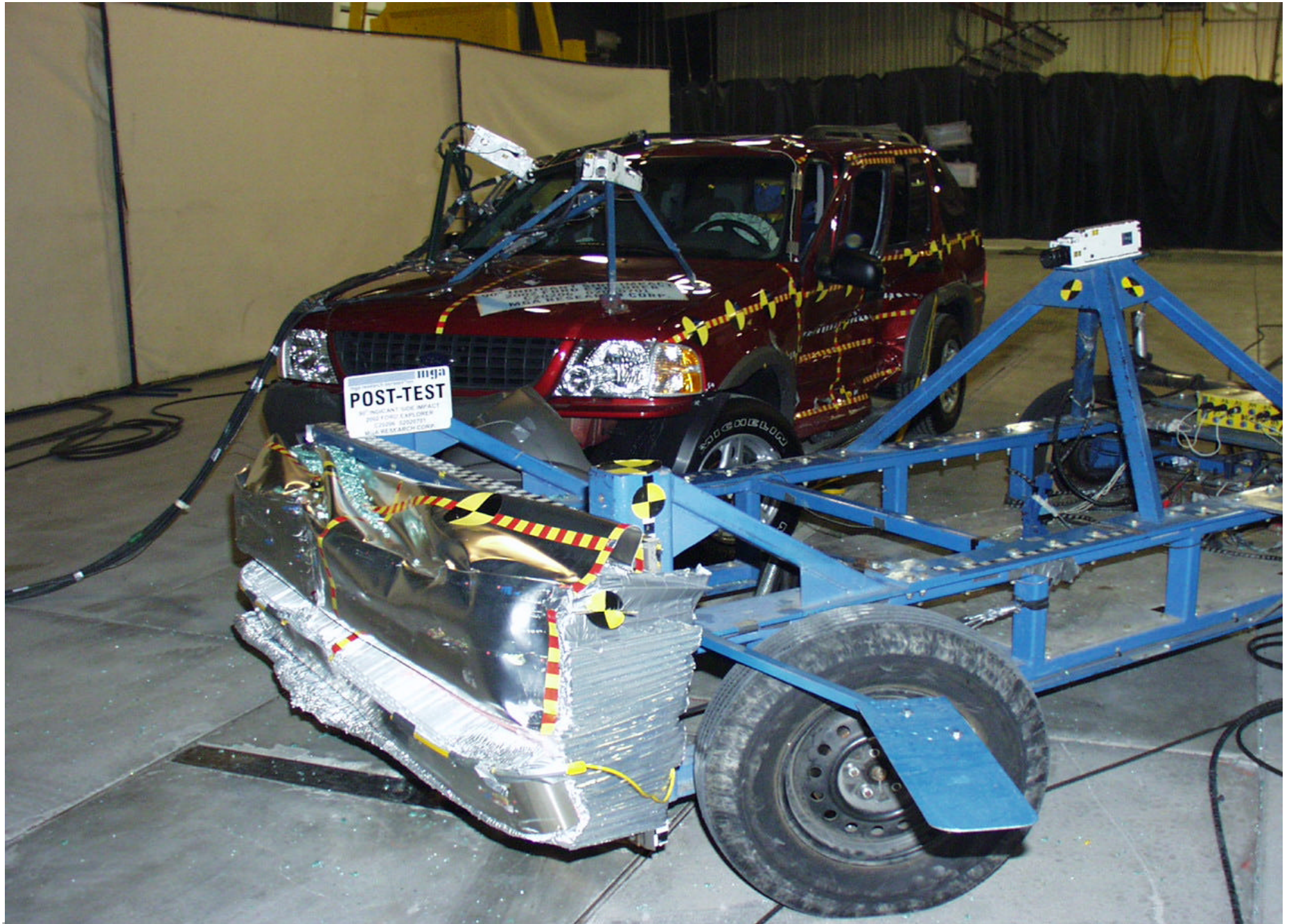
Post-Test MDB and Vehicle (left side)
