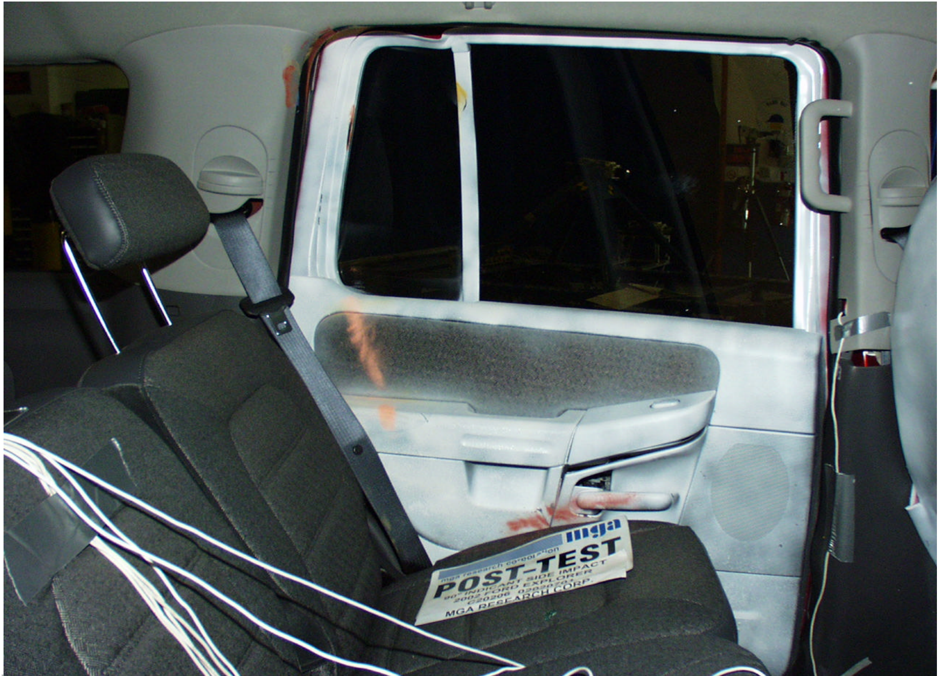
Post-Test Passenger Dummy Contact
