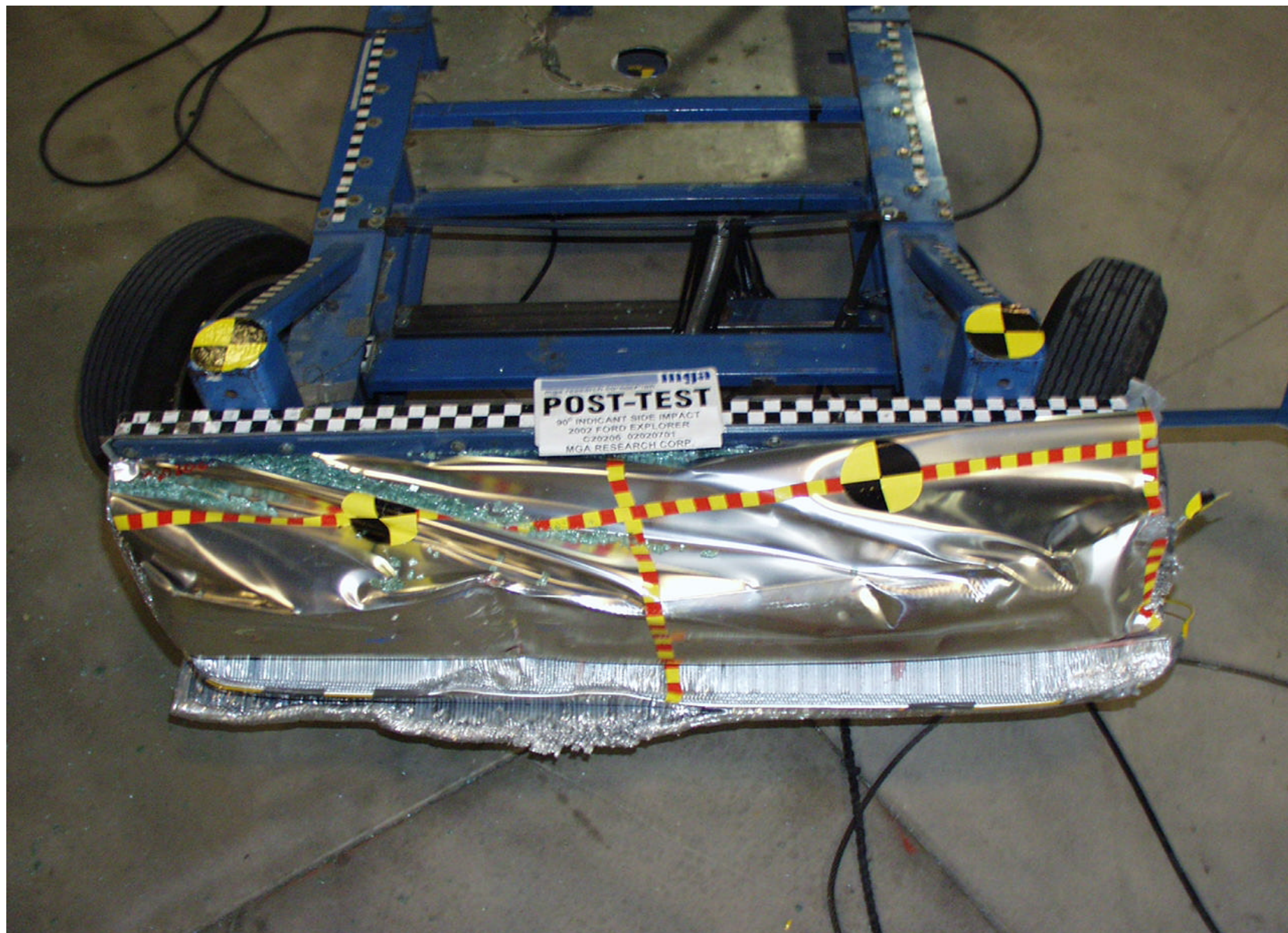
Post-Test MDB Top View
