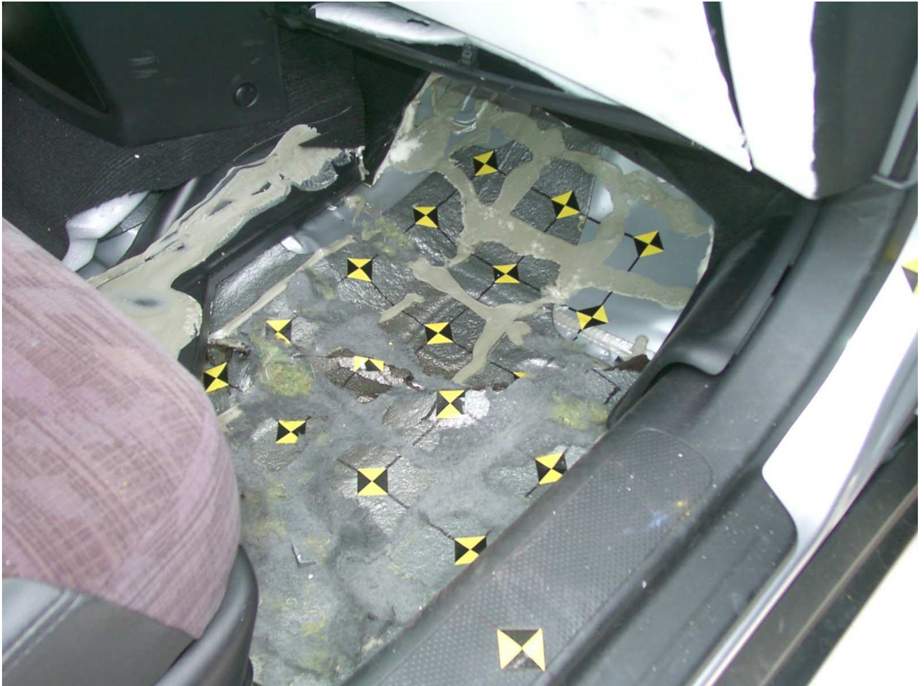
Figure A-52: Passenger Side Floor Pan, Post-Test
