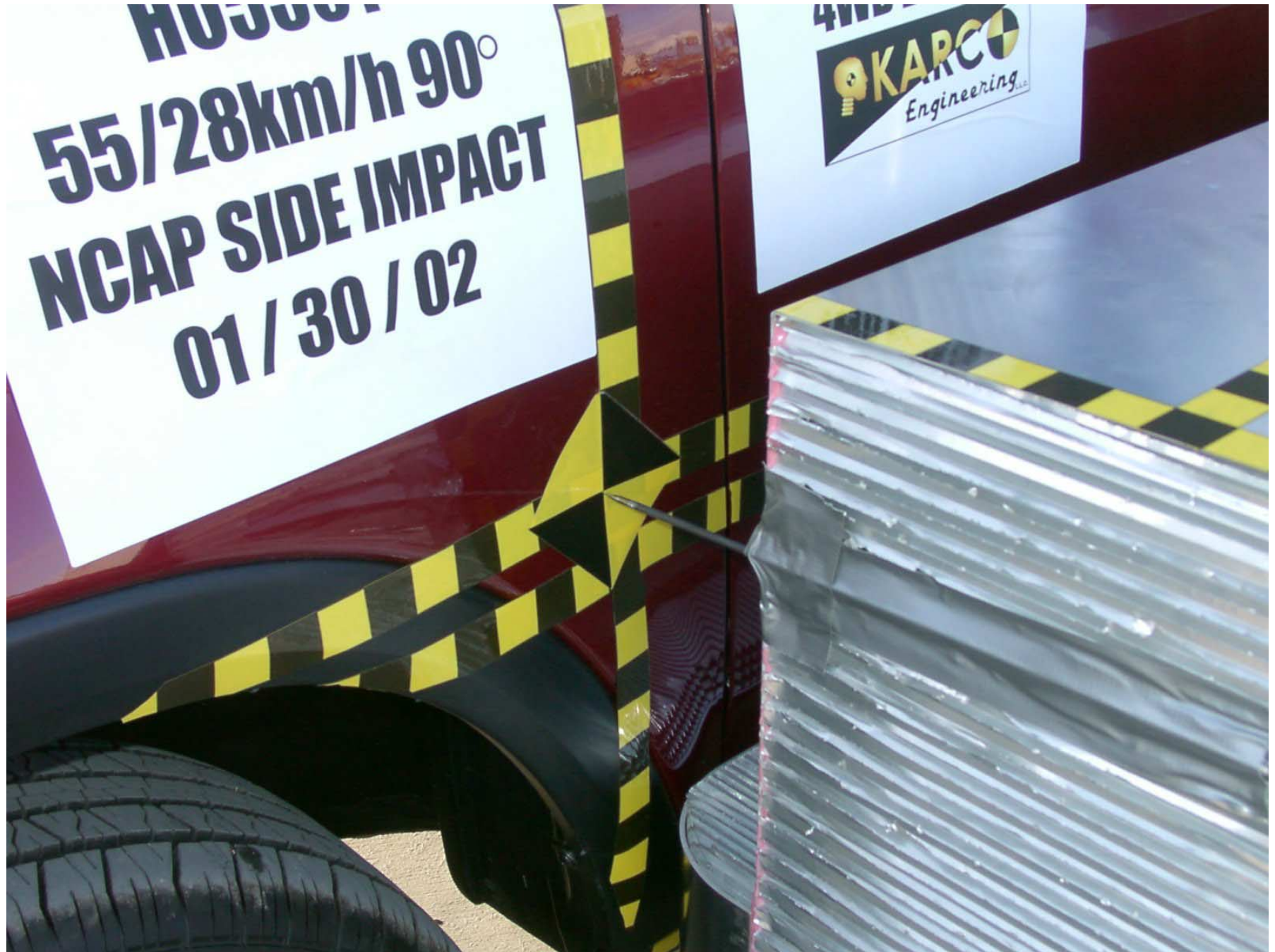
Figure A-19: Impact Point Target Set-up, Pre-Test
