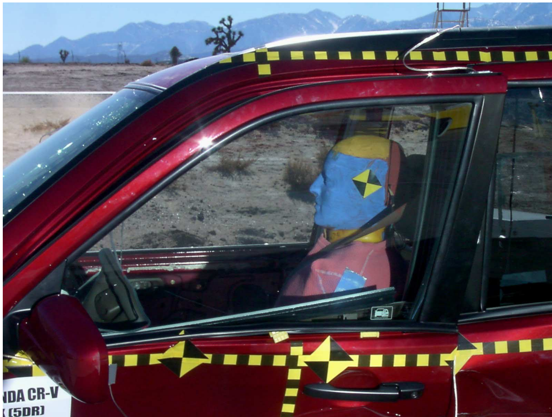
Figure A-31: Driver Dummy Left Side, Post-Test
