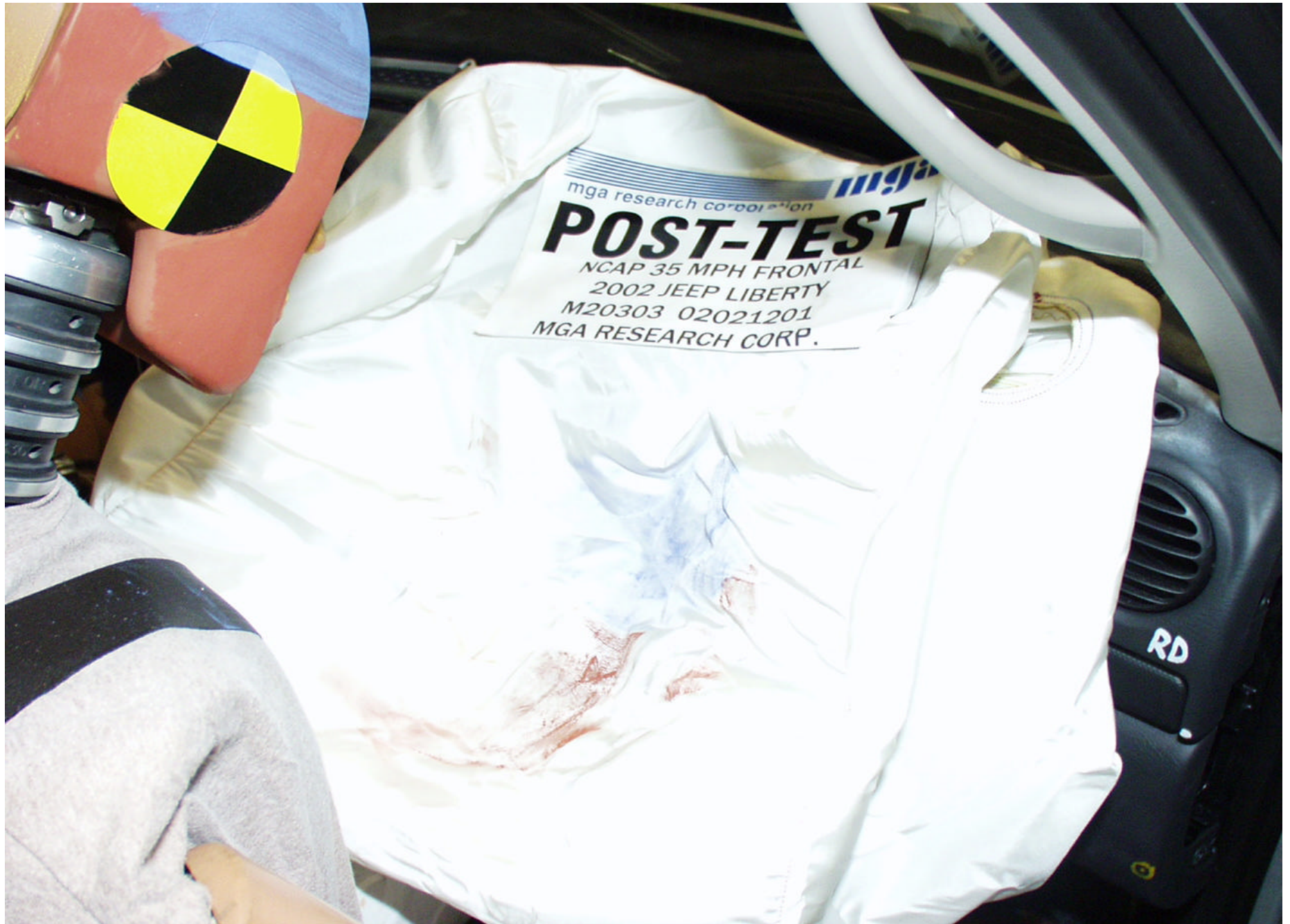
Post-Test Passenger Airbag Contact
