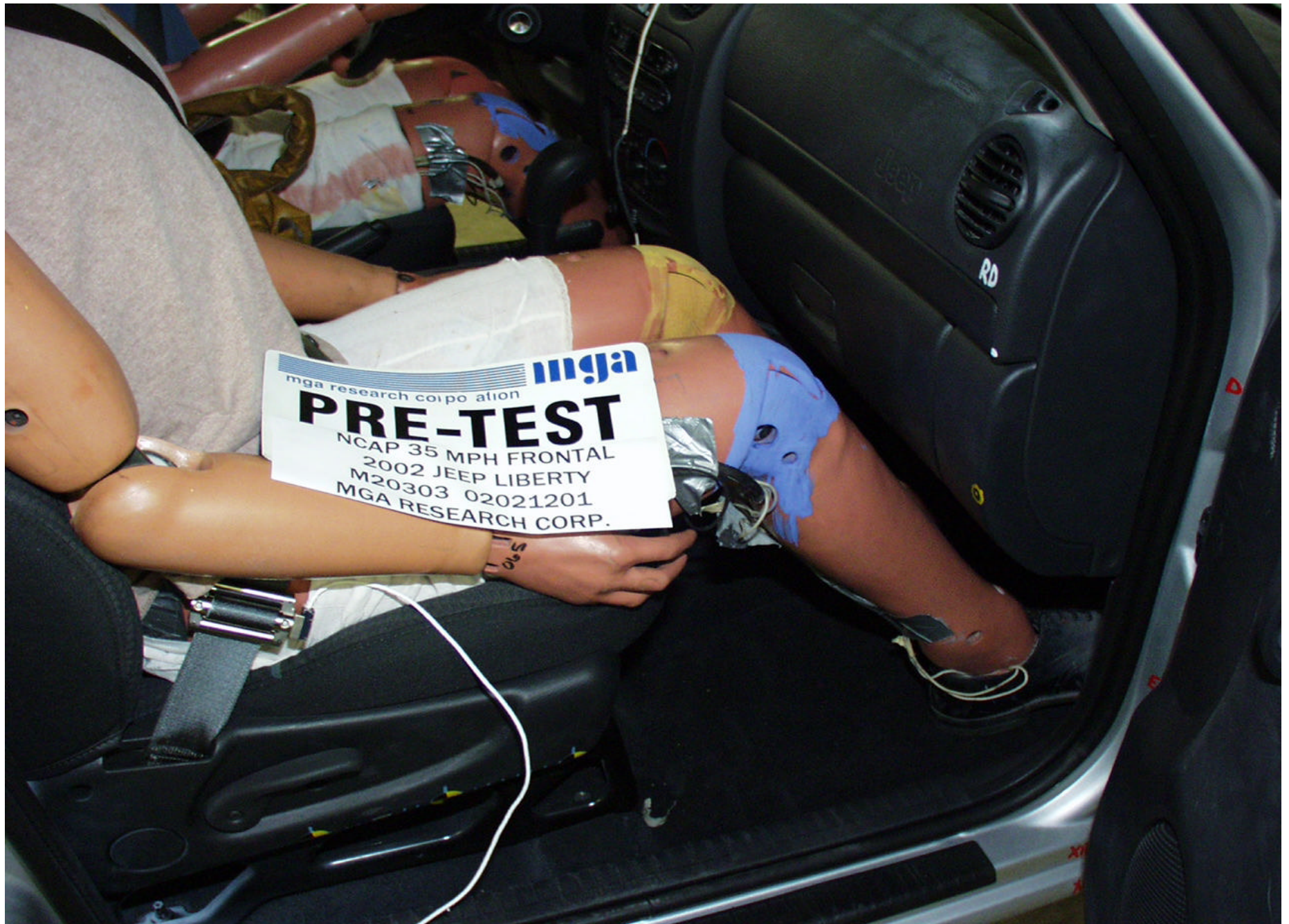
Pre-Test Passenger Dummy Knee Position
