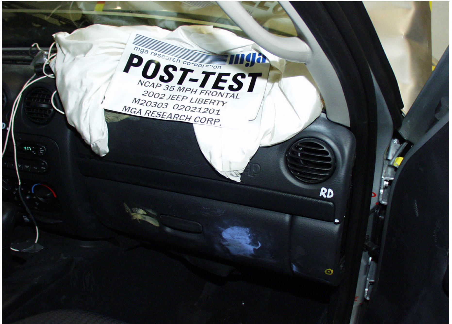
Post-Test Passenger Knee Contact View
