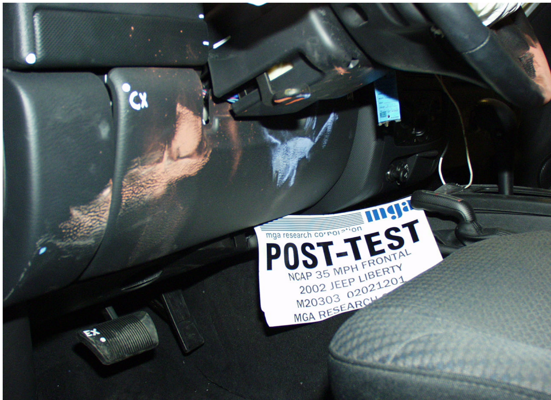
Post-Test Driver Knee Contact View
