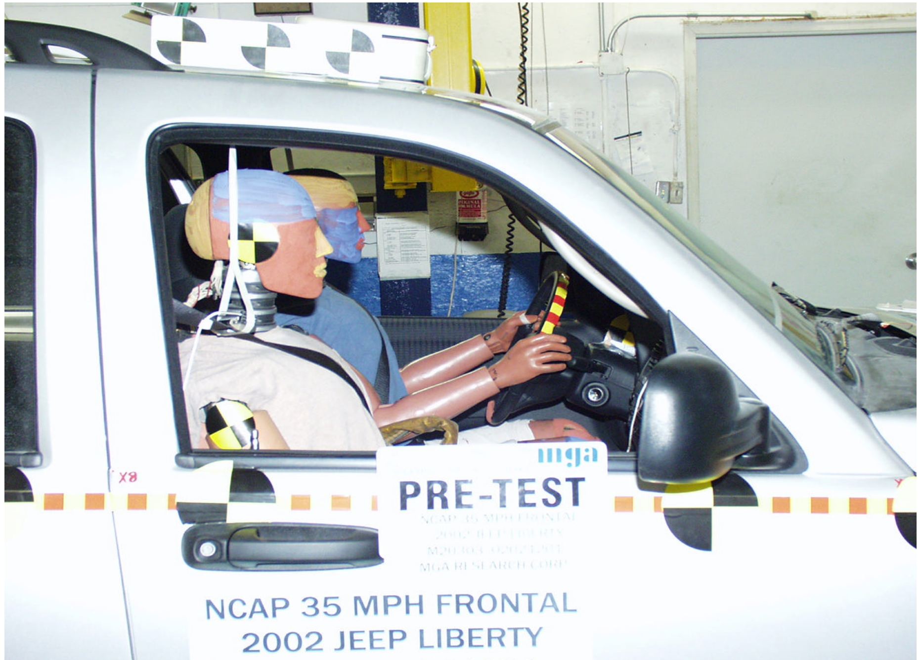
Pre-Test Passenger Dummy Position Right Side View
