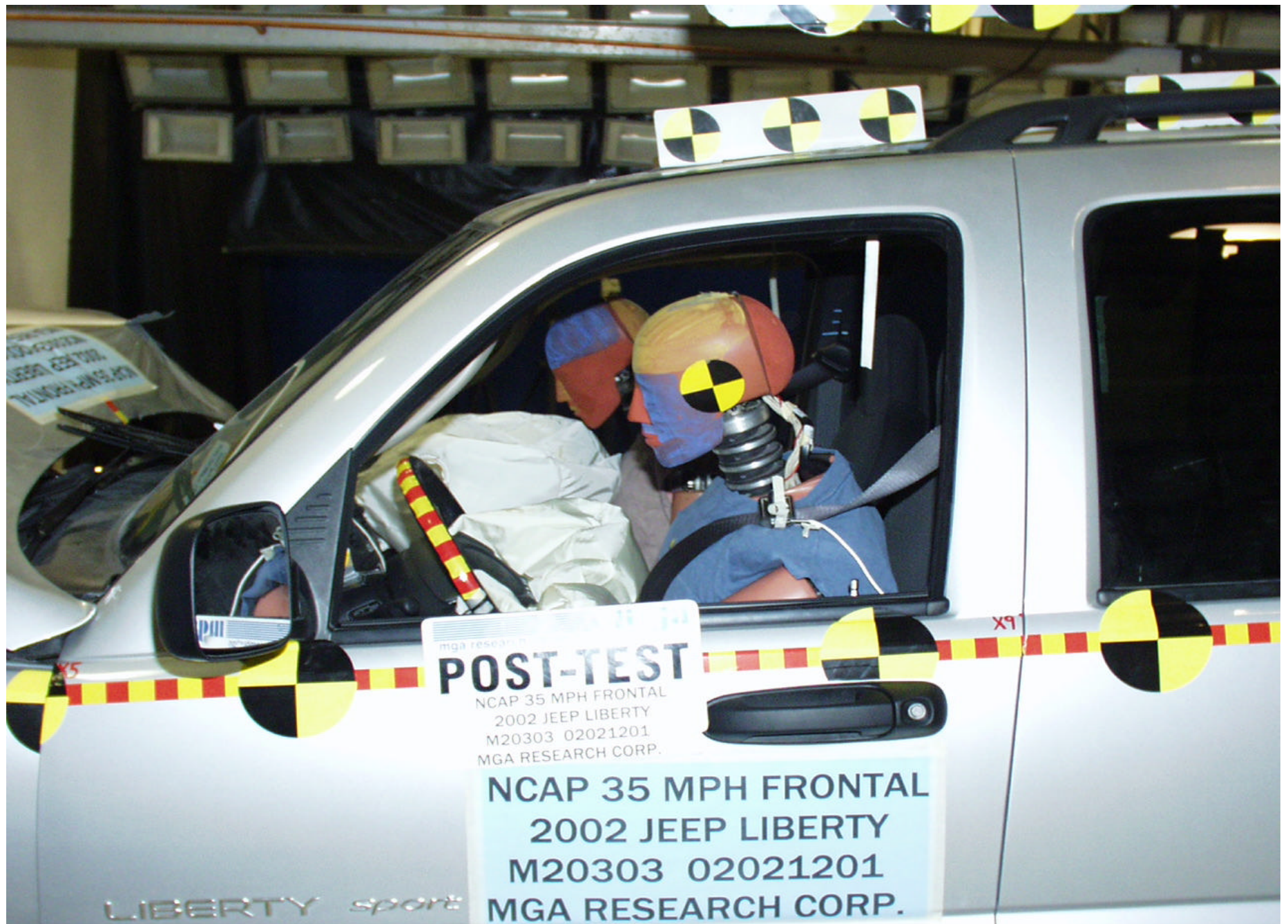
Post-Test Driver Dummy Position Left Side View
