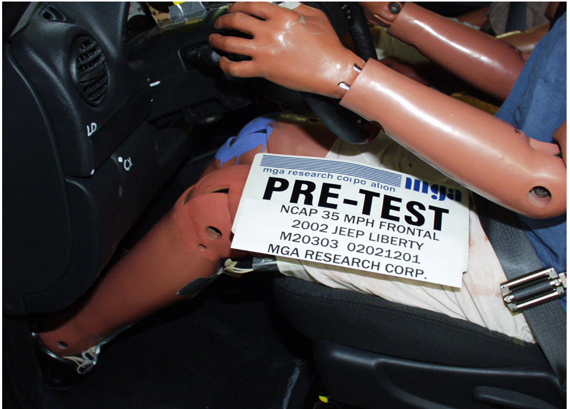
Pre-Test Driver Dummy Knee Position
