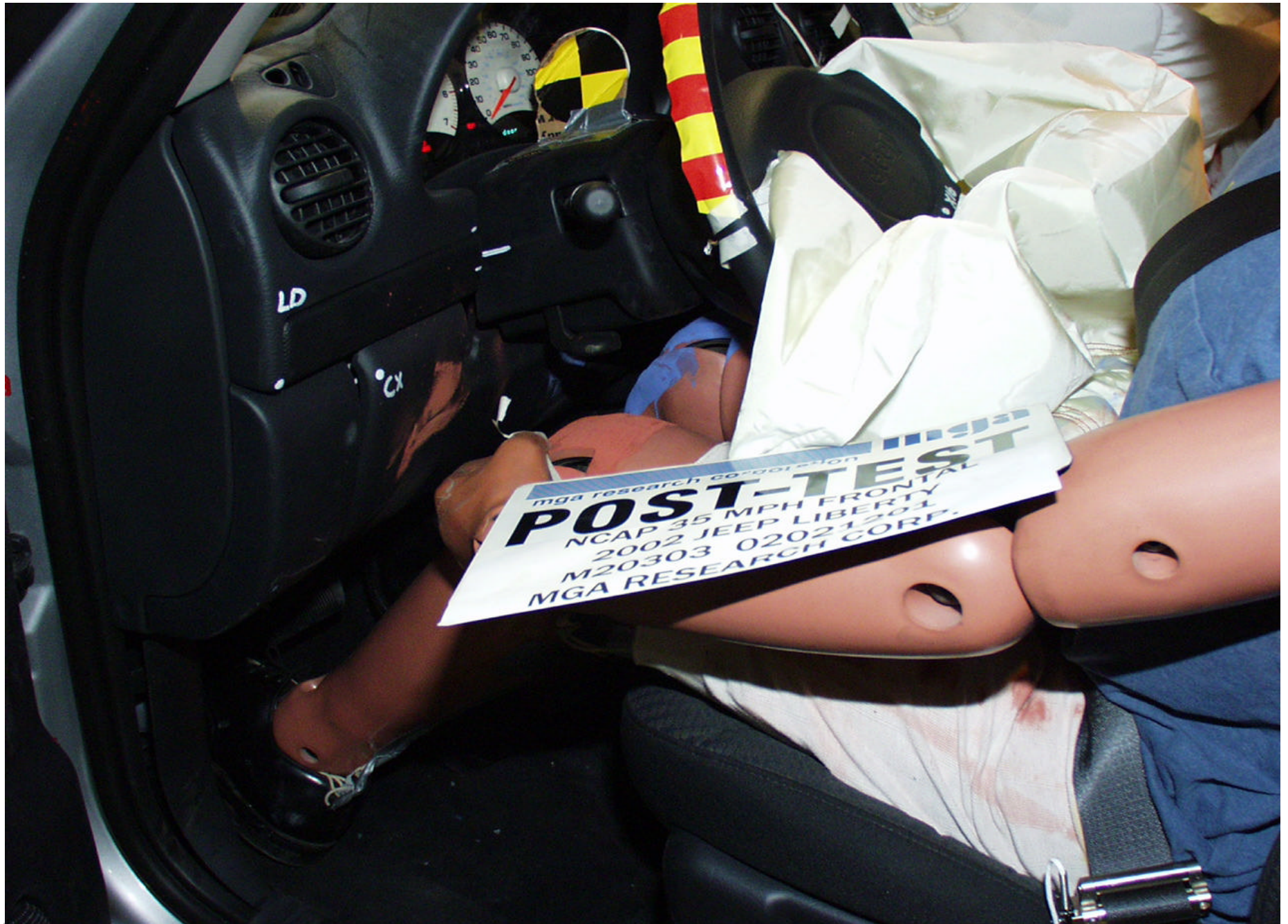
Post-Test Driver Dummy Knee Position
