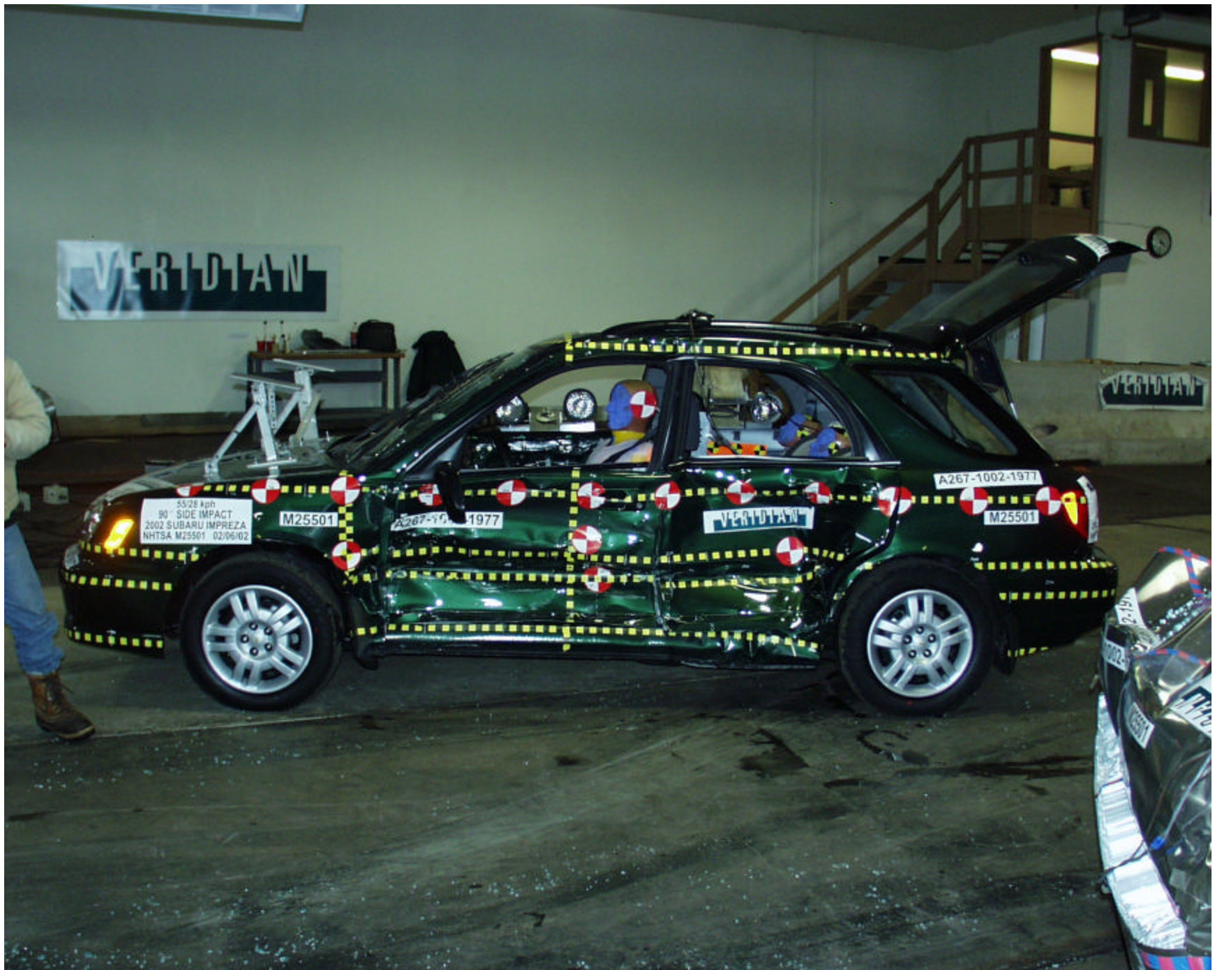
Figure A-6 POST-TEST IMPACTED SIDE VIEW OF TEST VEHICLE
