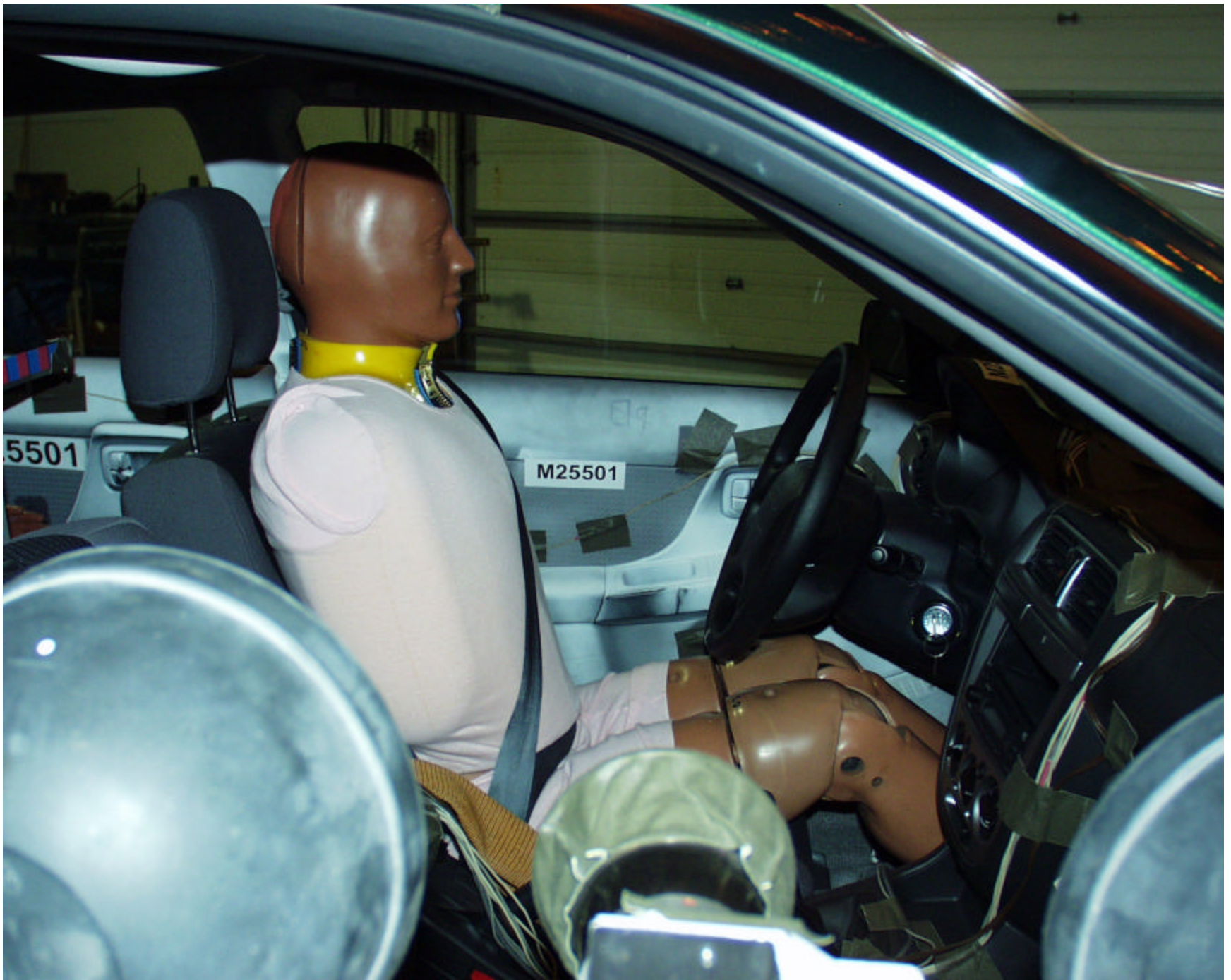
Figure A-25 PRE-TEST RIGHT OCCUPANT COMPARTMENT VIEW OF FRONT SID
