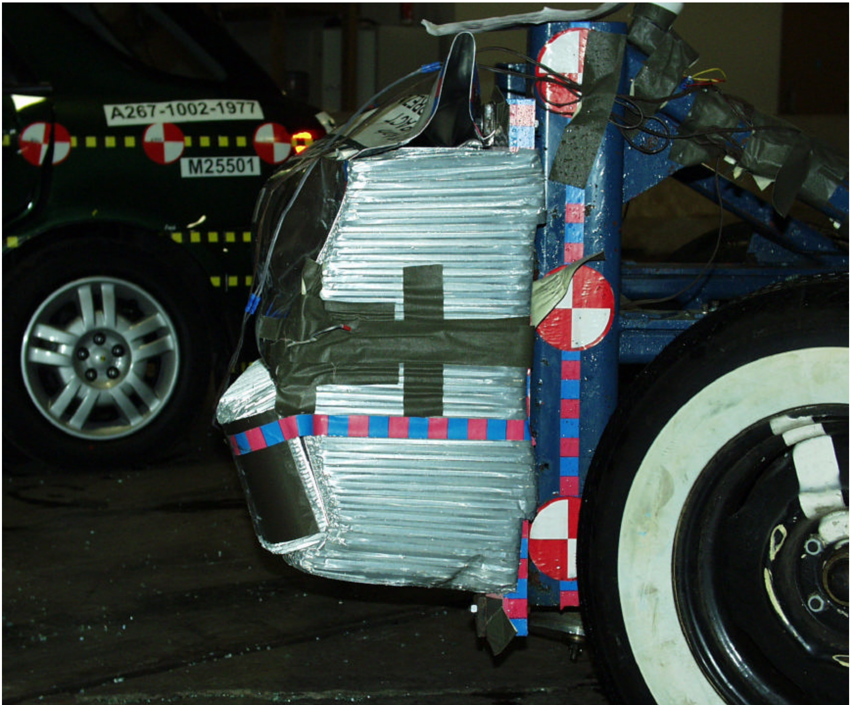
Figure A-18 POST-TEST LEFT SIDE VIEW OF IMPACTOR FACE
