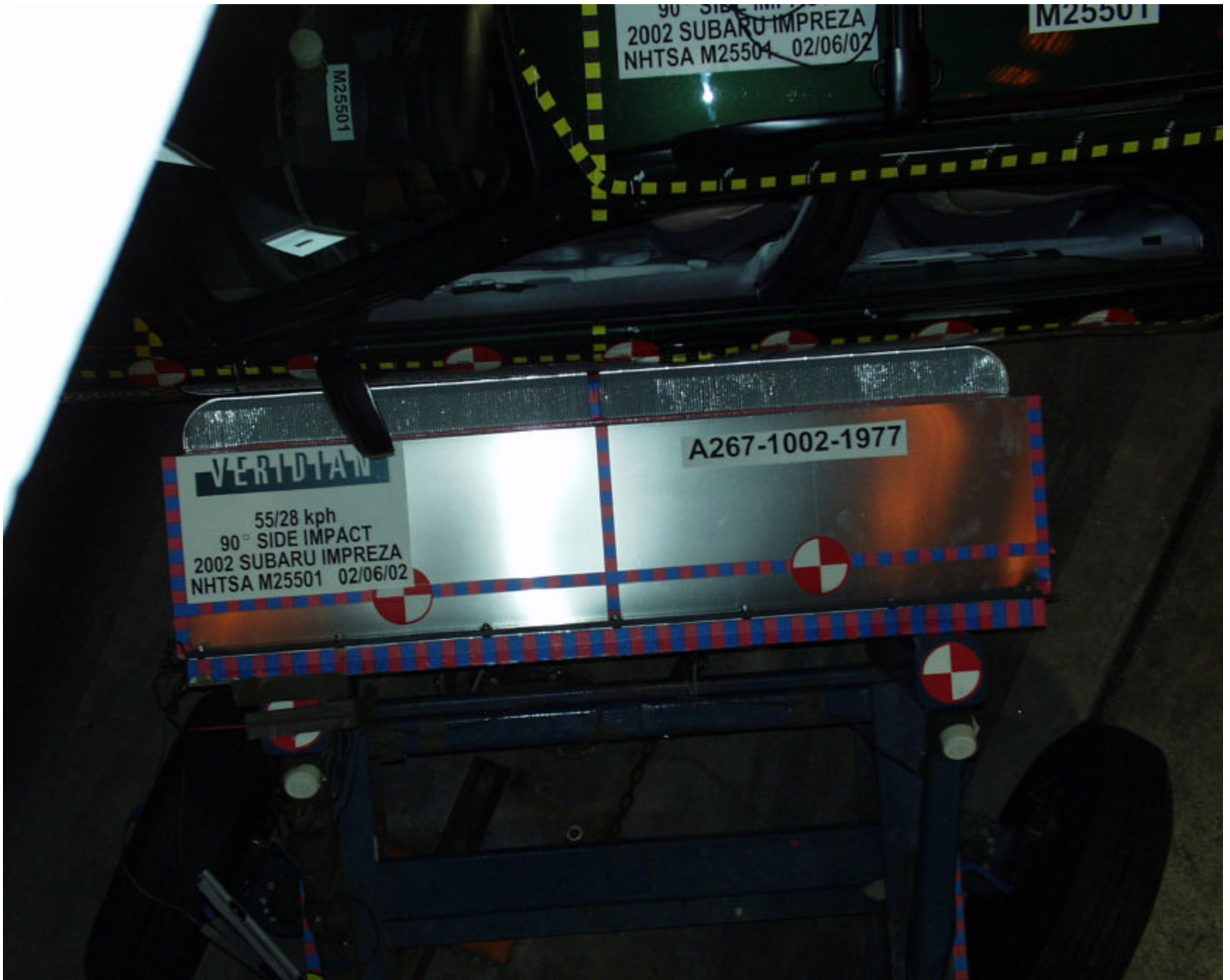
Figure A-21 PRE-TEST TOP VIEW OF IMPACTOR FACE
