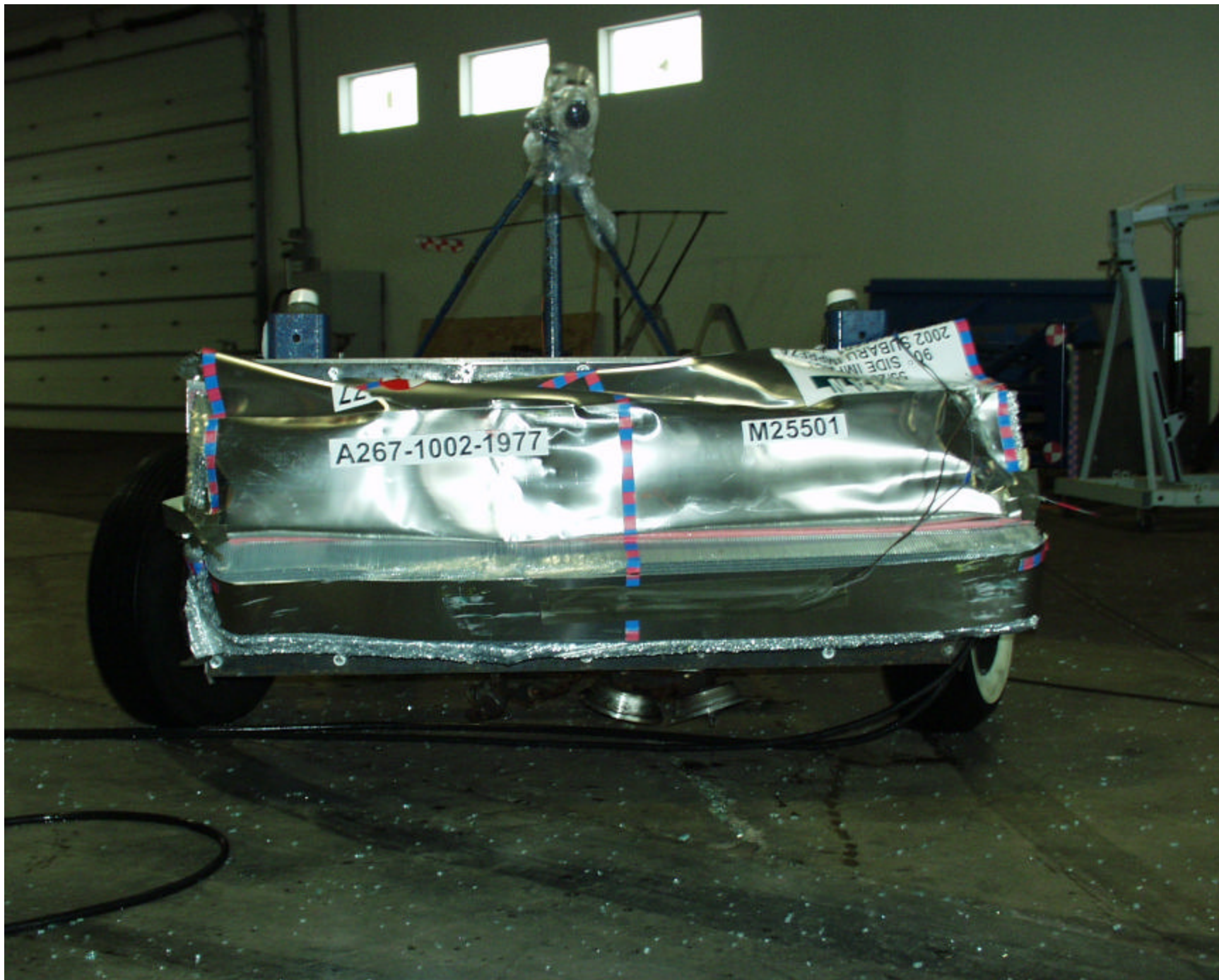
Figure A-16 POST-TEST FRONTAL VIEW OF IMPACTOR FACE
