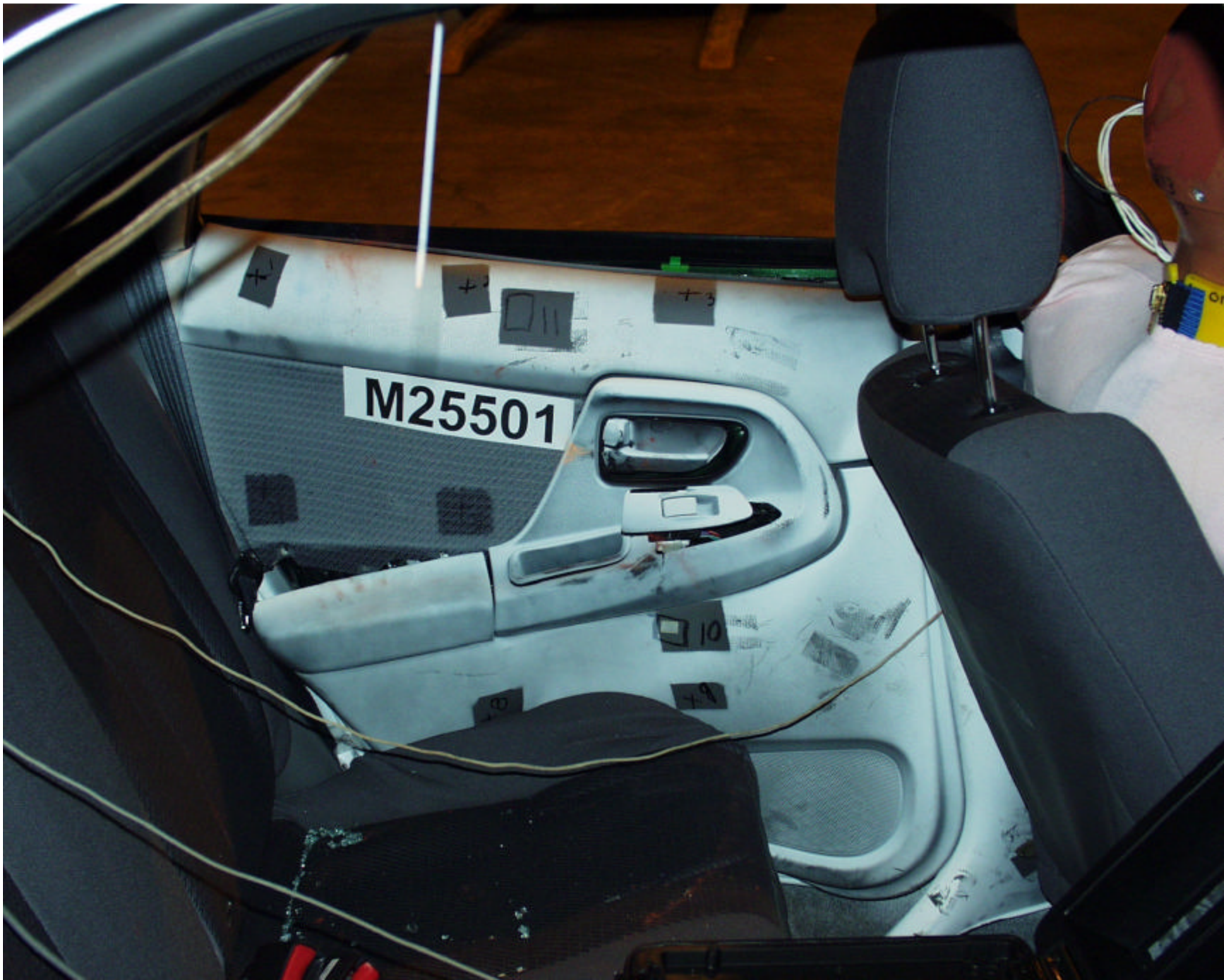
Figure A-32 POST-TEST INTERIOR OF REAR DOOR SHOWING IMPACT LOCATIONS
