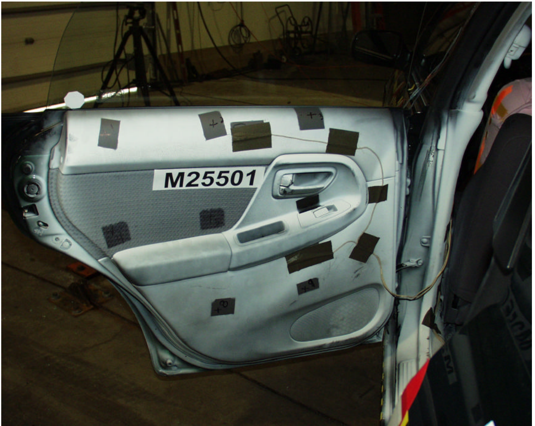
Figure A-31 PRE-TEST INTERIOR OF REAR DOOR
