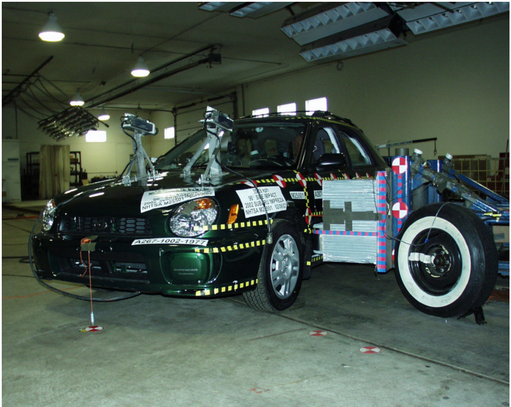
Figure A-33 PRE-TEST LEFT SIDE VIEW OF MDB WITH IMPACTOR FACE IN POSITION
