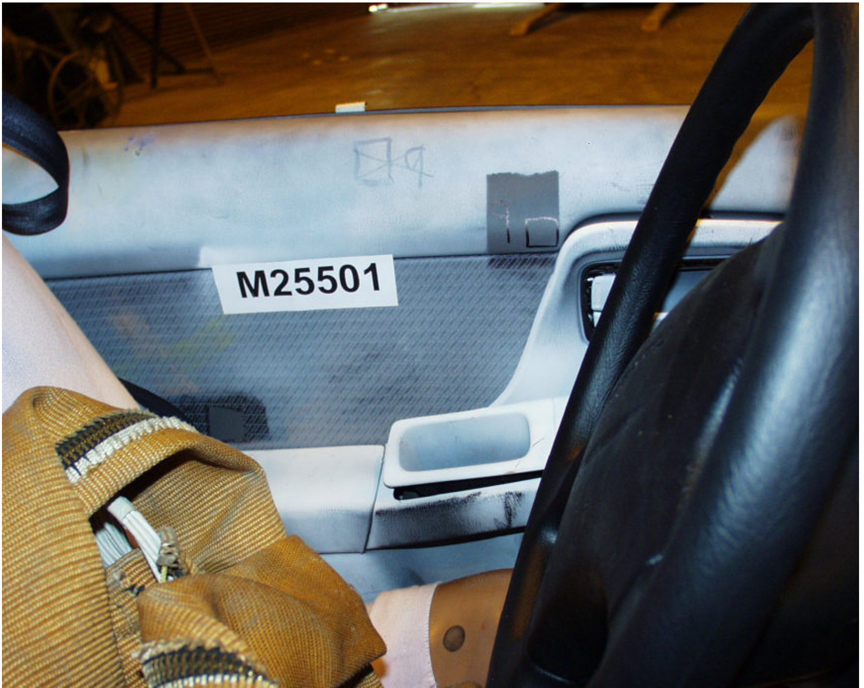
Figure A-30 POST-TEST INTERIOR OF FRONT DOOR SHOWING SID IMPACT LOCATIONS
