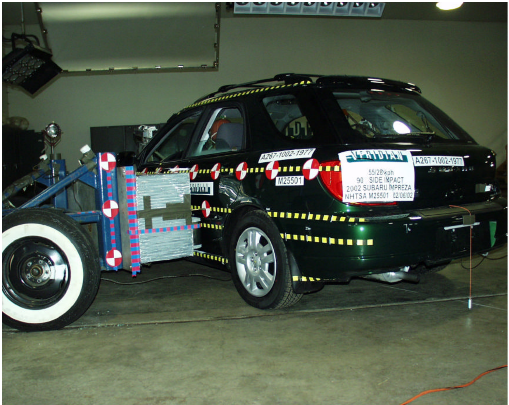
Figure A-34 PRE-TEST RIGHT SIDE VIEW OF MDB WITH IMPACTOR FACE IN POSITION
