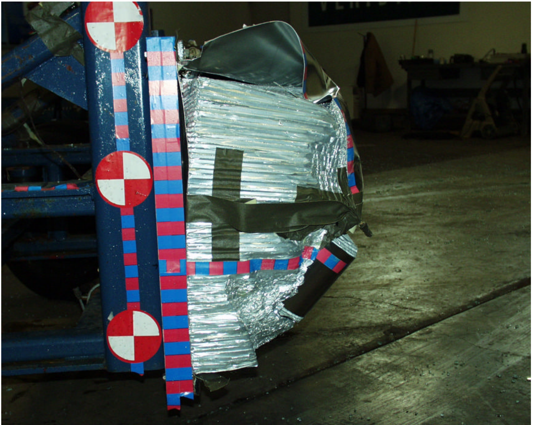
Figure A-20 POST-TEST RIGHT SIDE VIEW OF IMPACTOR FACE
