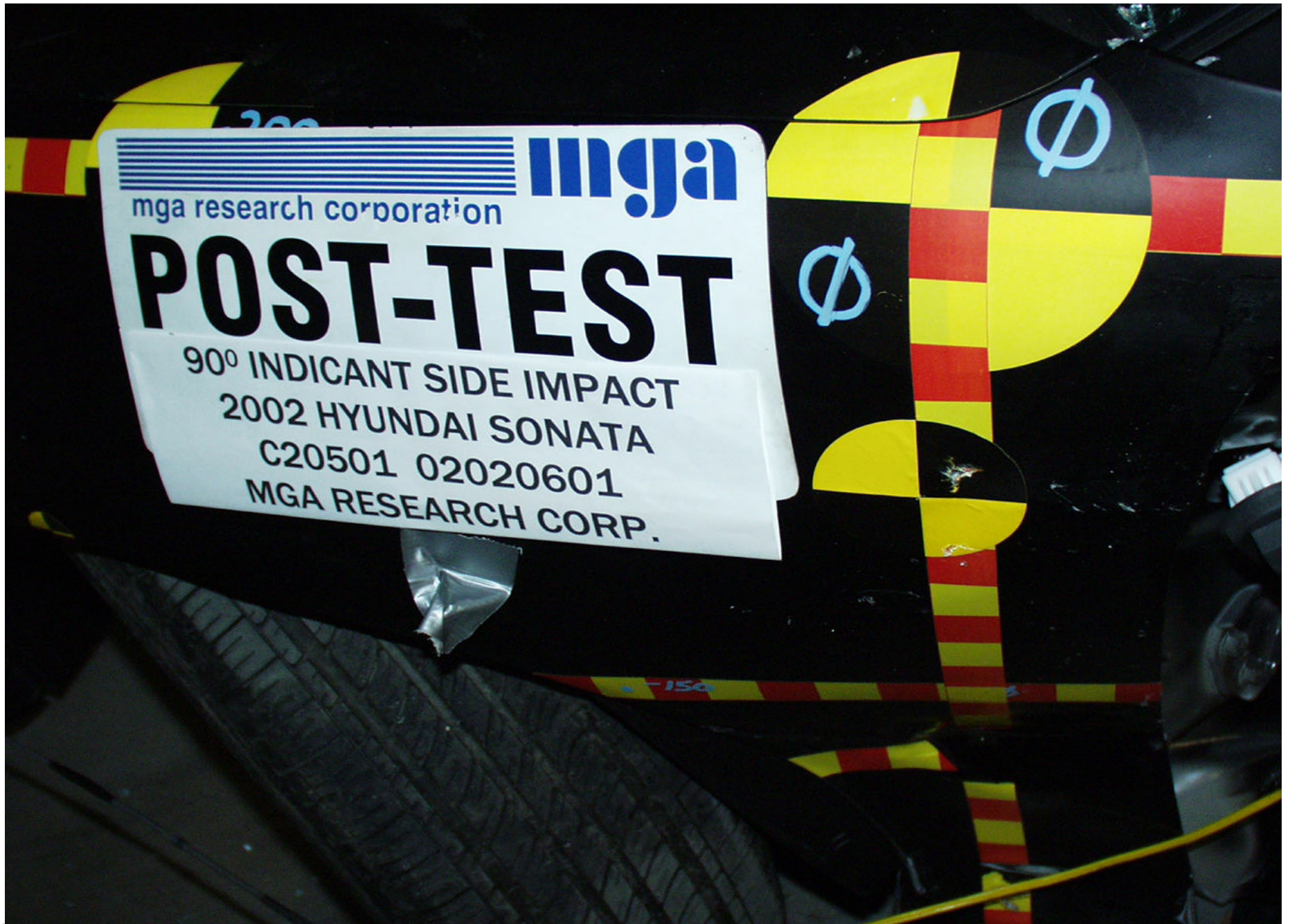
Post-Test Left Front Impact Point on Vehicle
