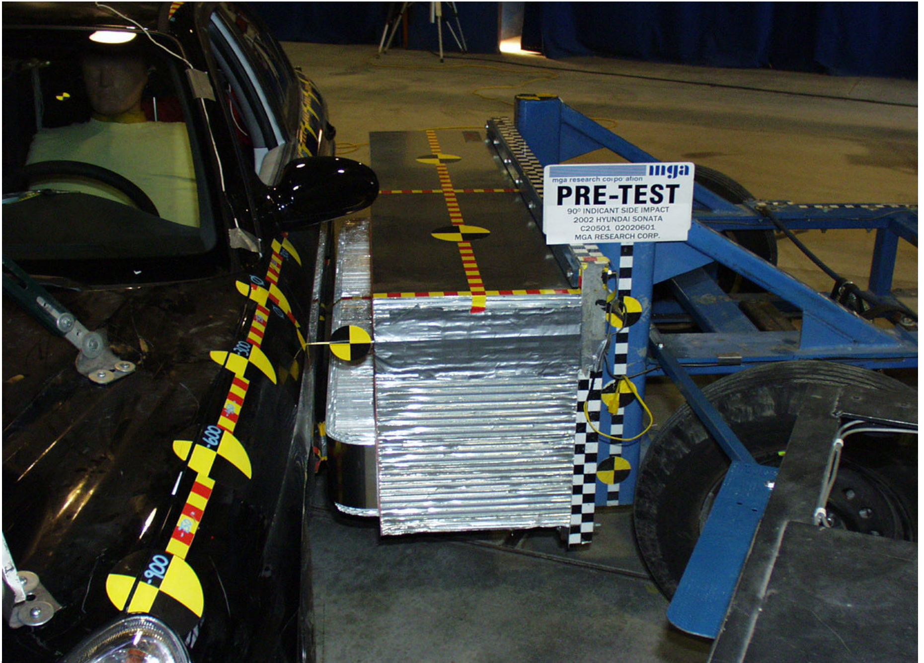
Pre-Test MDB Positioned Against Vehicle (left side)
