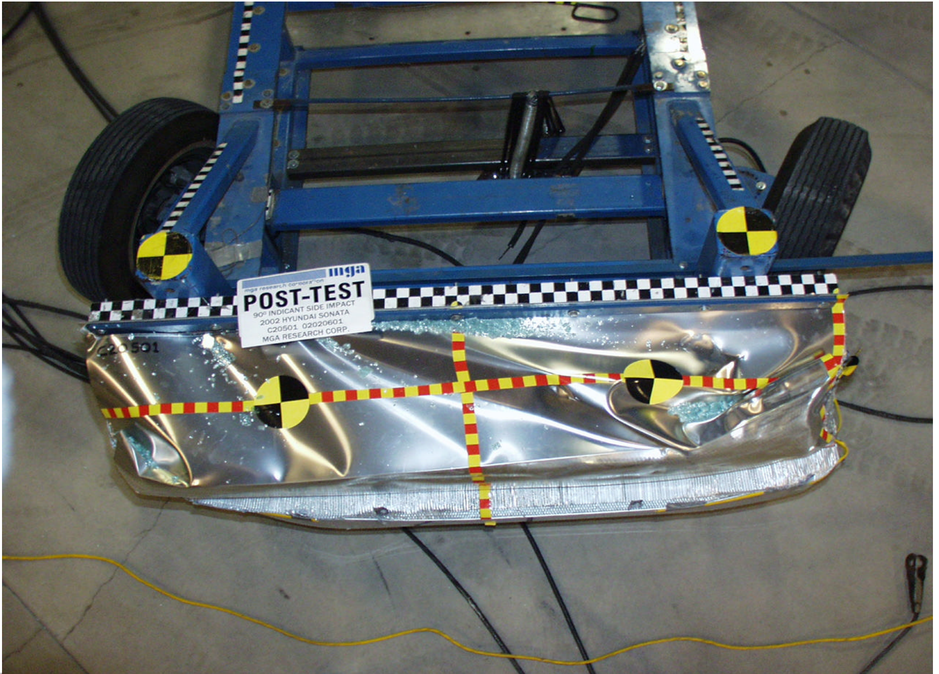
Post-Test MDB Top View
