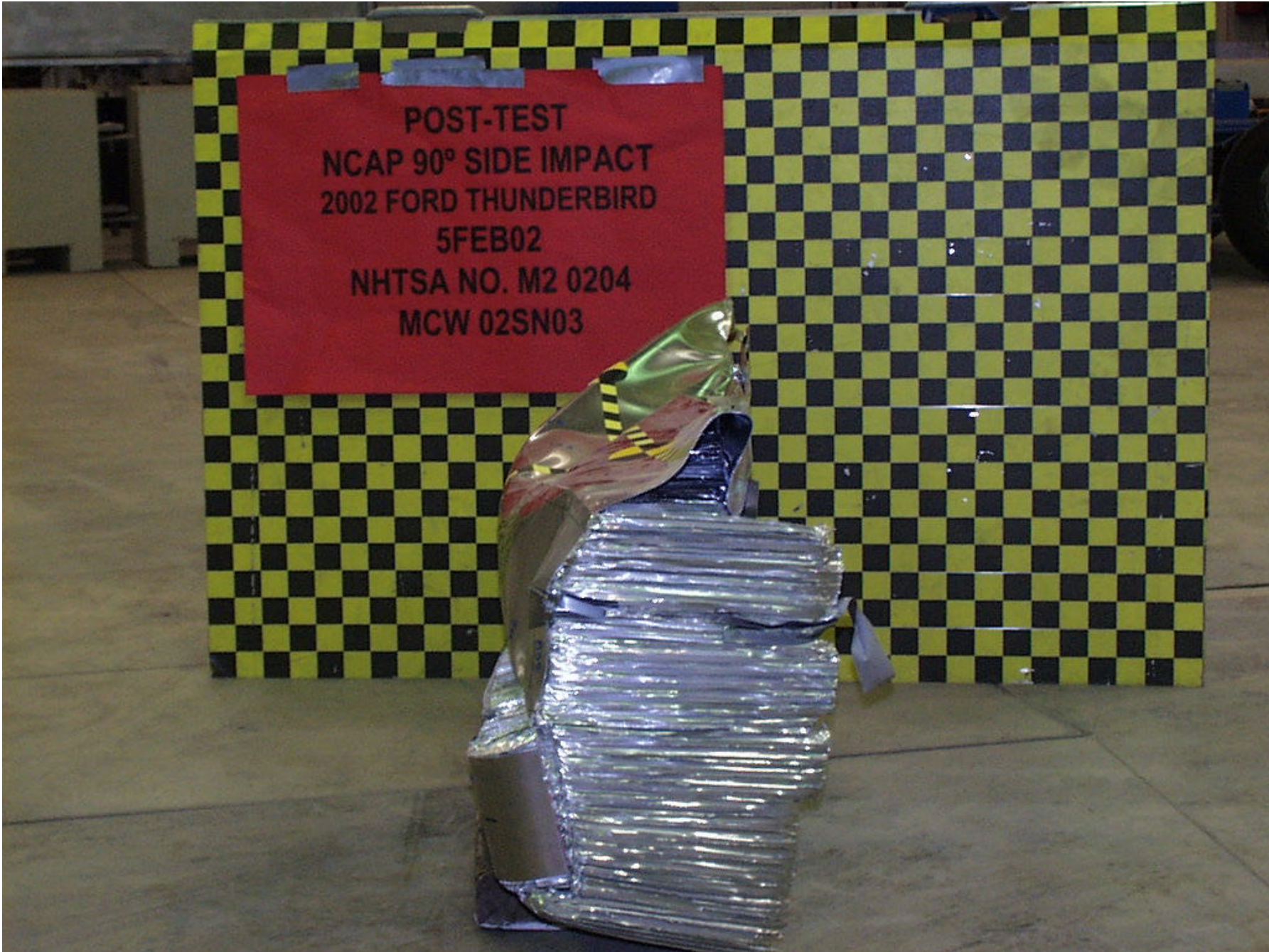
Figure A-42: POST-TEST ALUMINUM BARRIER LEFT SIDE
