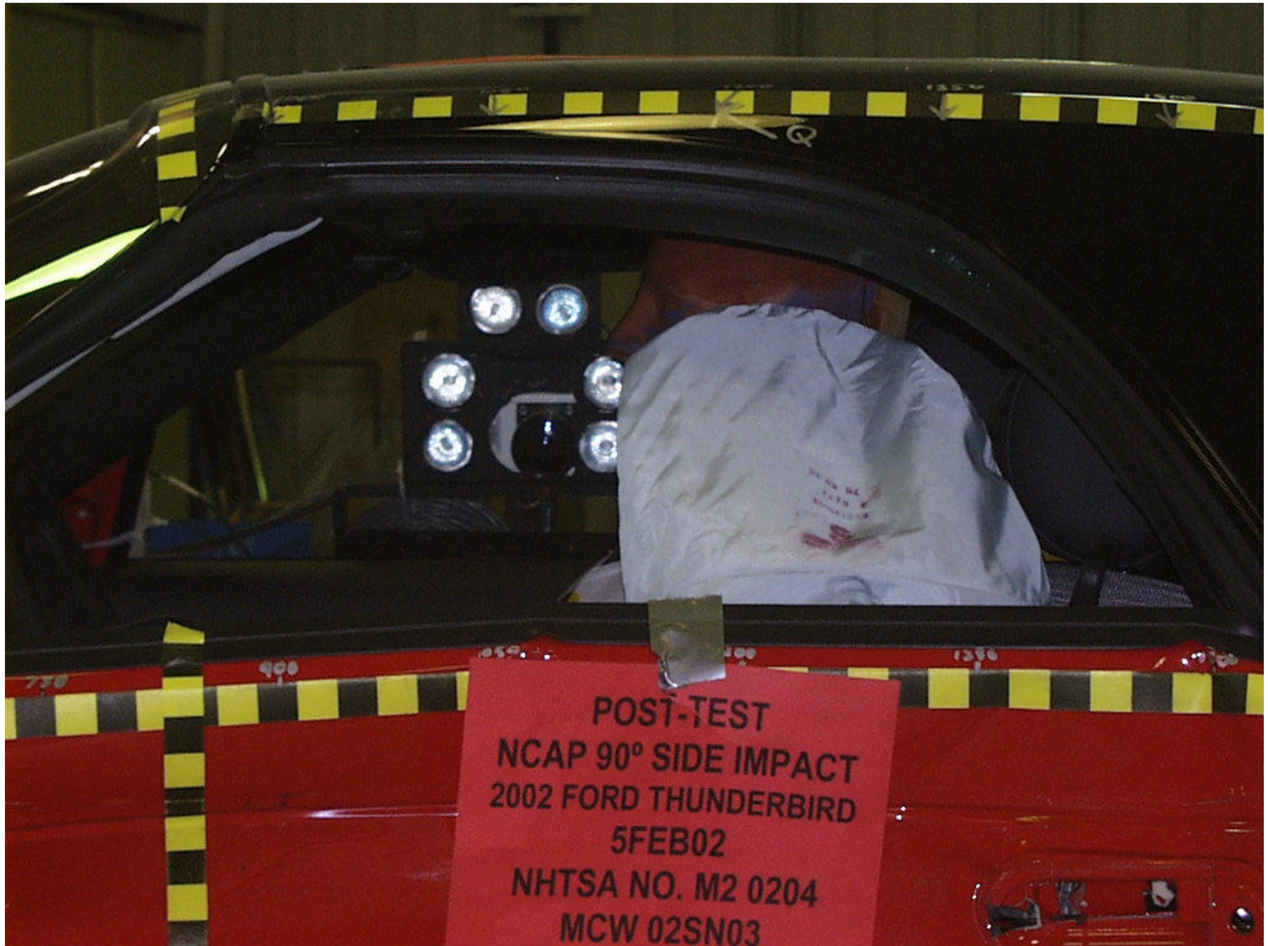
Figure A-20: POST-TEST LEFT OCCUPANT COMPARTMENT VIEW OF FRONT SID (MDB MOVED)
