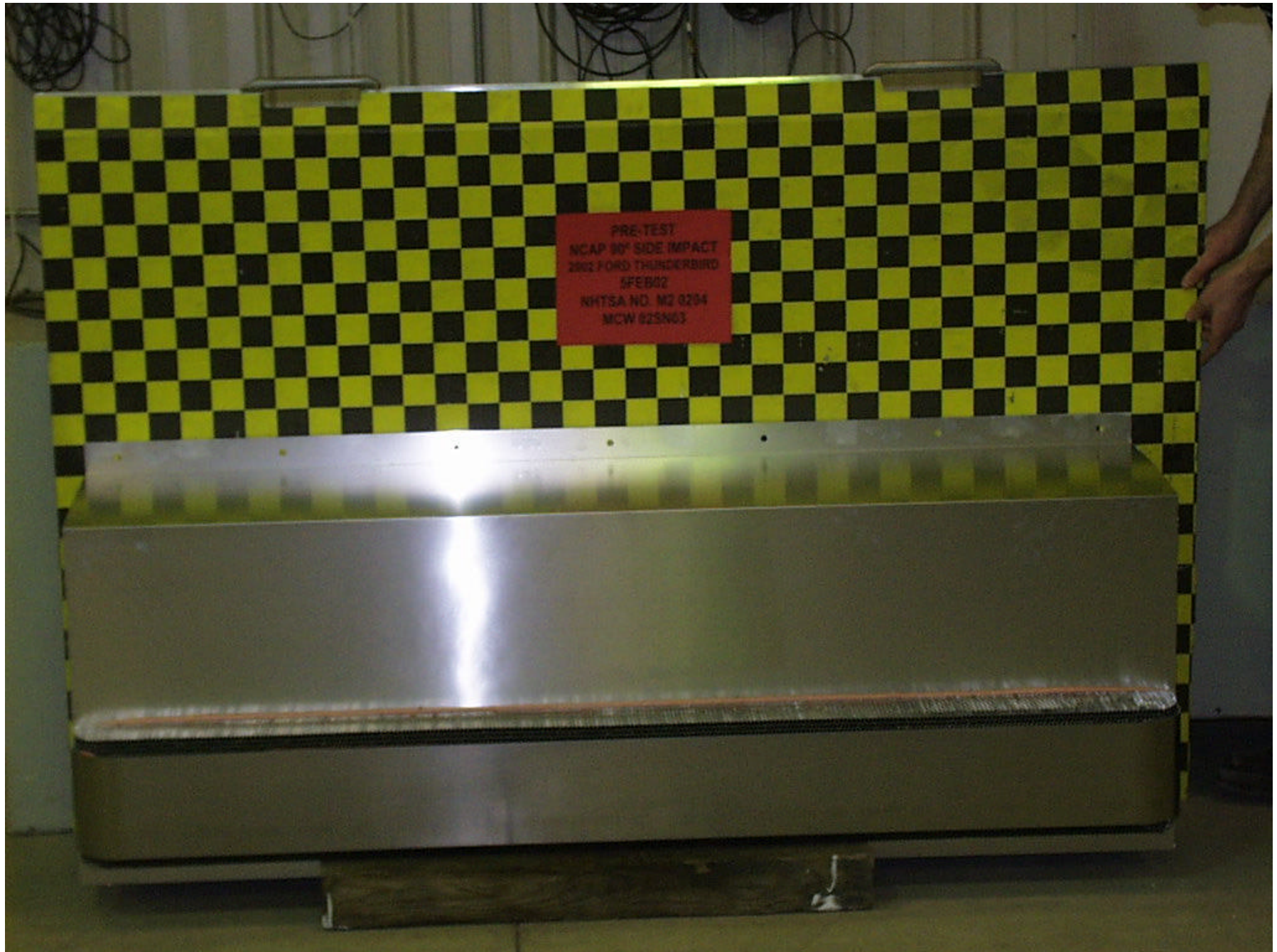
Figure A-39: PRE-TEST ALUMINUM BARRIER FRONT
