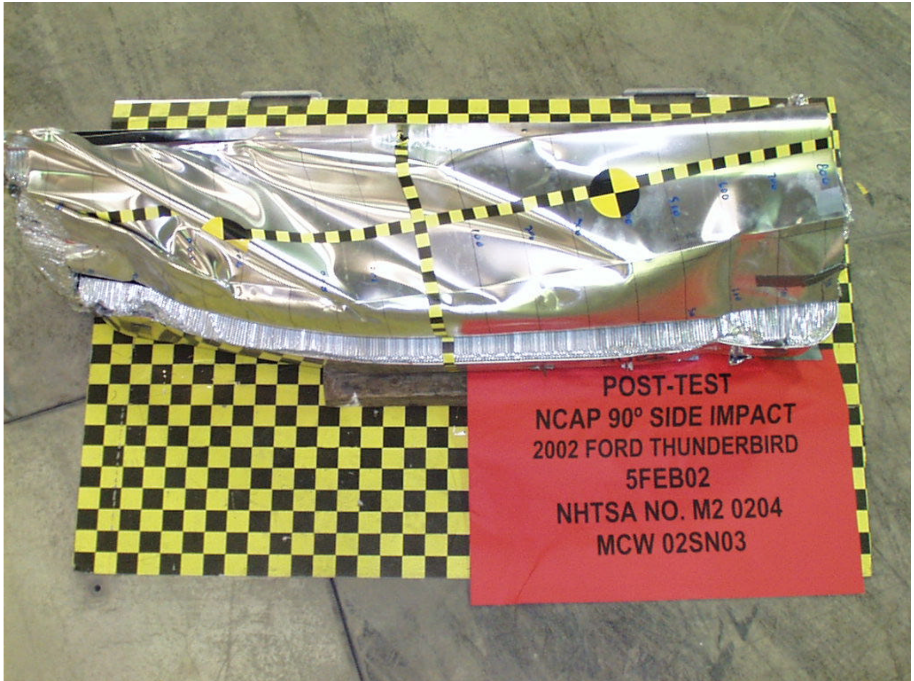
Figure A-46: POST-TEST ALUMINUM BARRIER OVERHEAD
