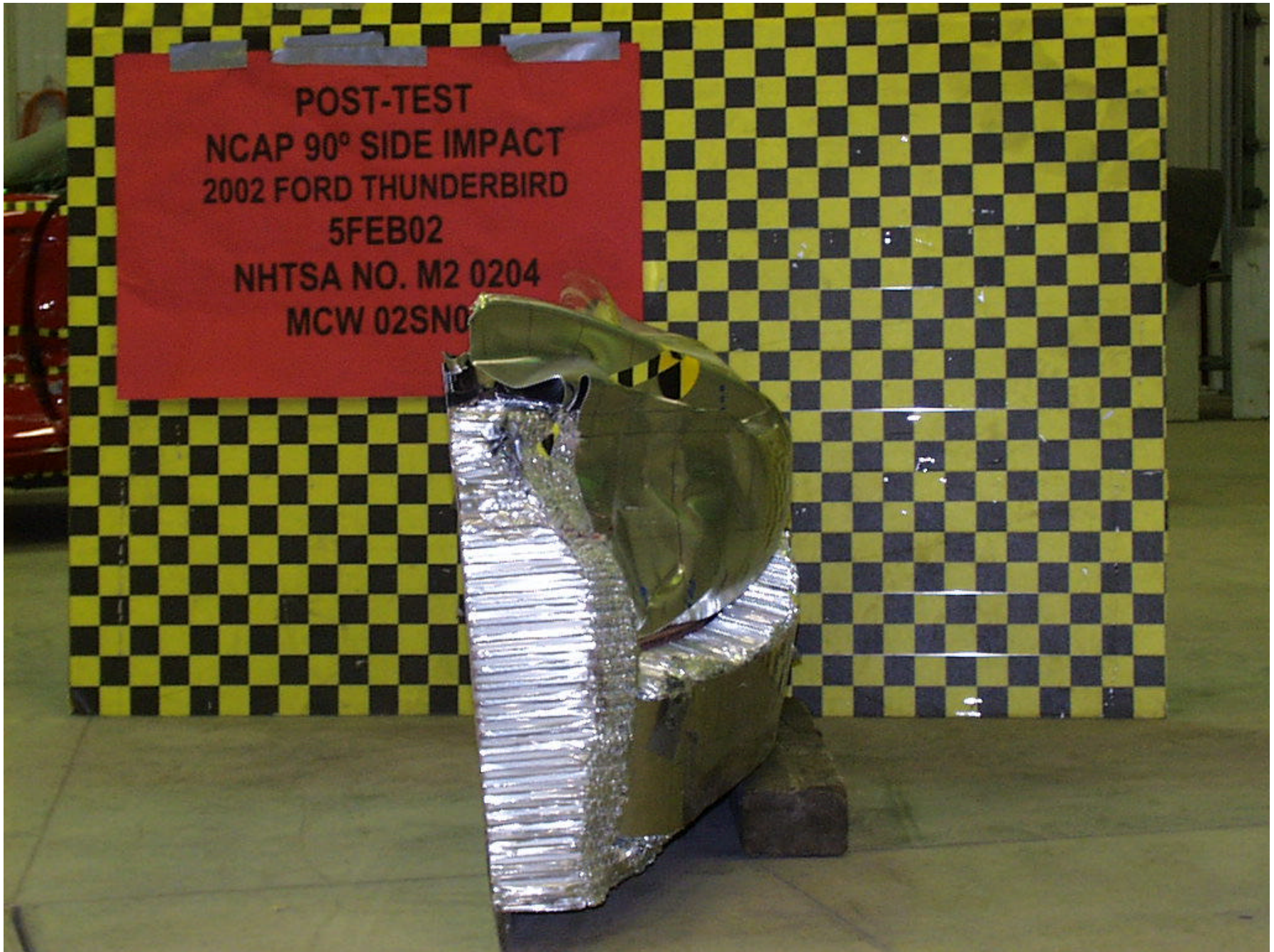
Figure A-44: POST-TEST ALUMINUM BARRIER RIGHT SIDE
