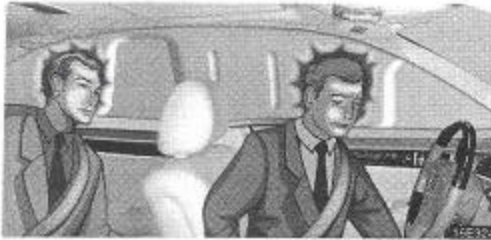
► SRS curtain shield airbags for front and rear outside occupants
