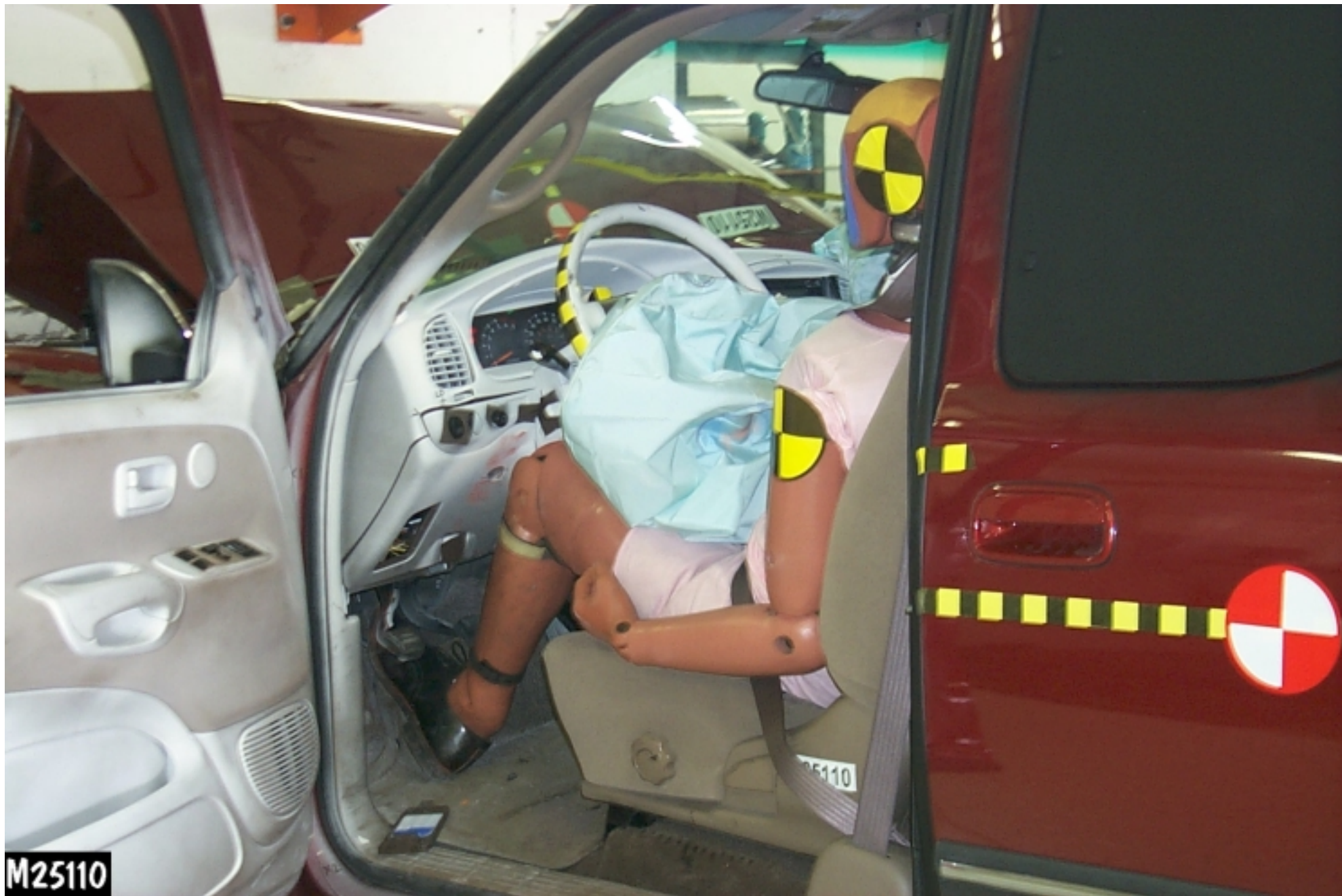
Figure A-27: POST-TEST DRIVER AND INTERIOR VIEW
