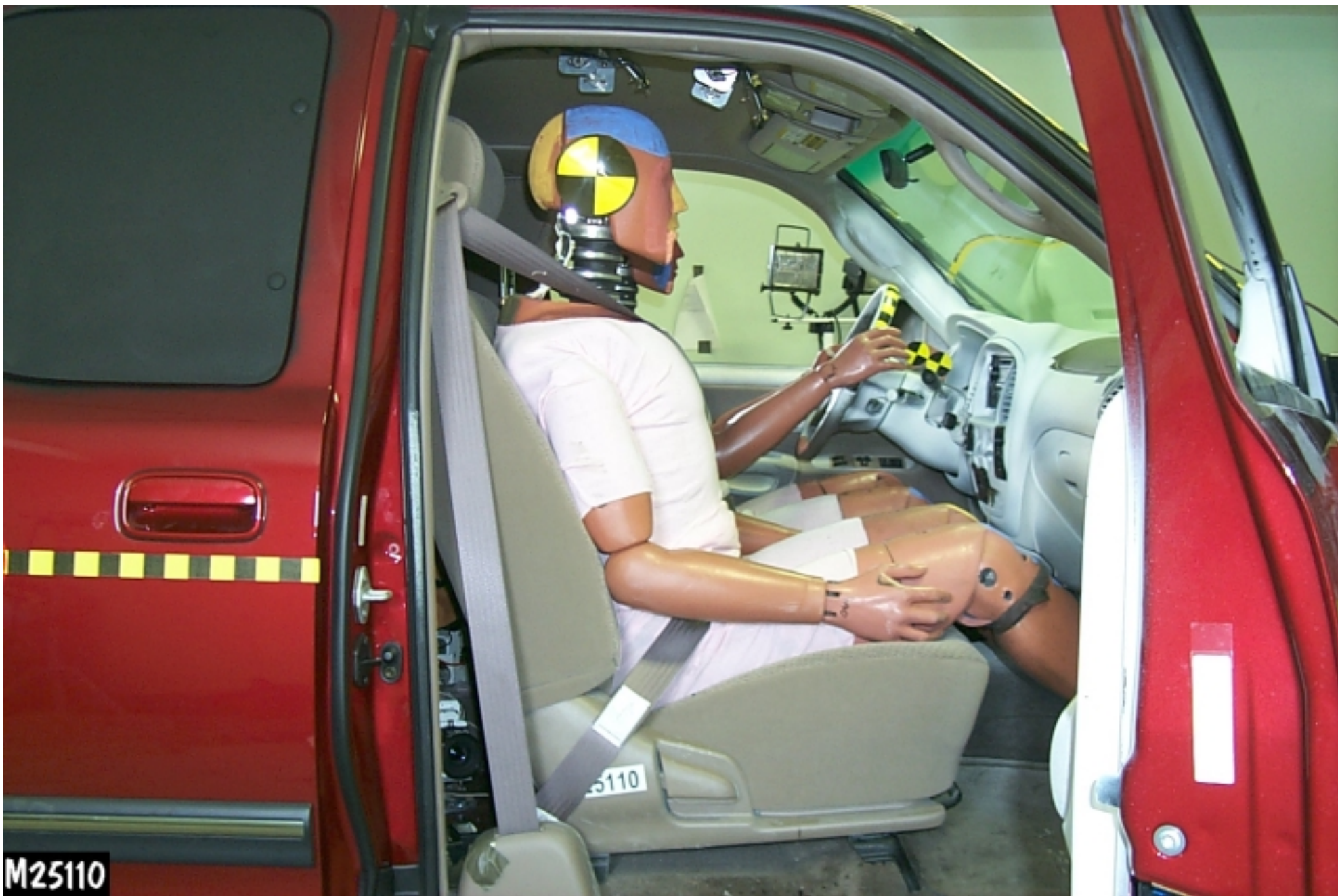
Figure A-24: PRE-TEST PASSENGER POSITION VIEW
