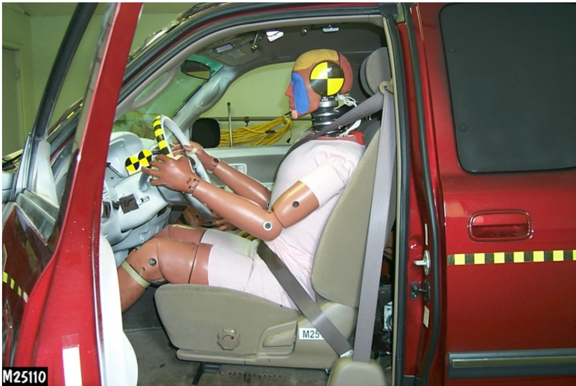
Figure A-22: PRE-TEST DRIVER POSITION VIEW
