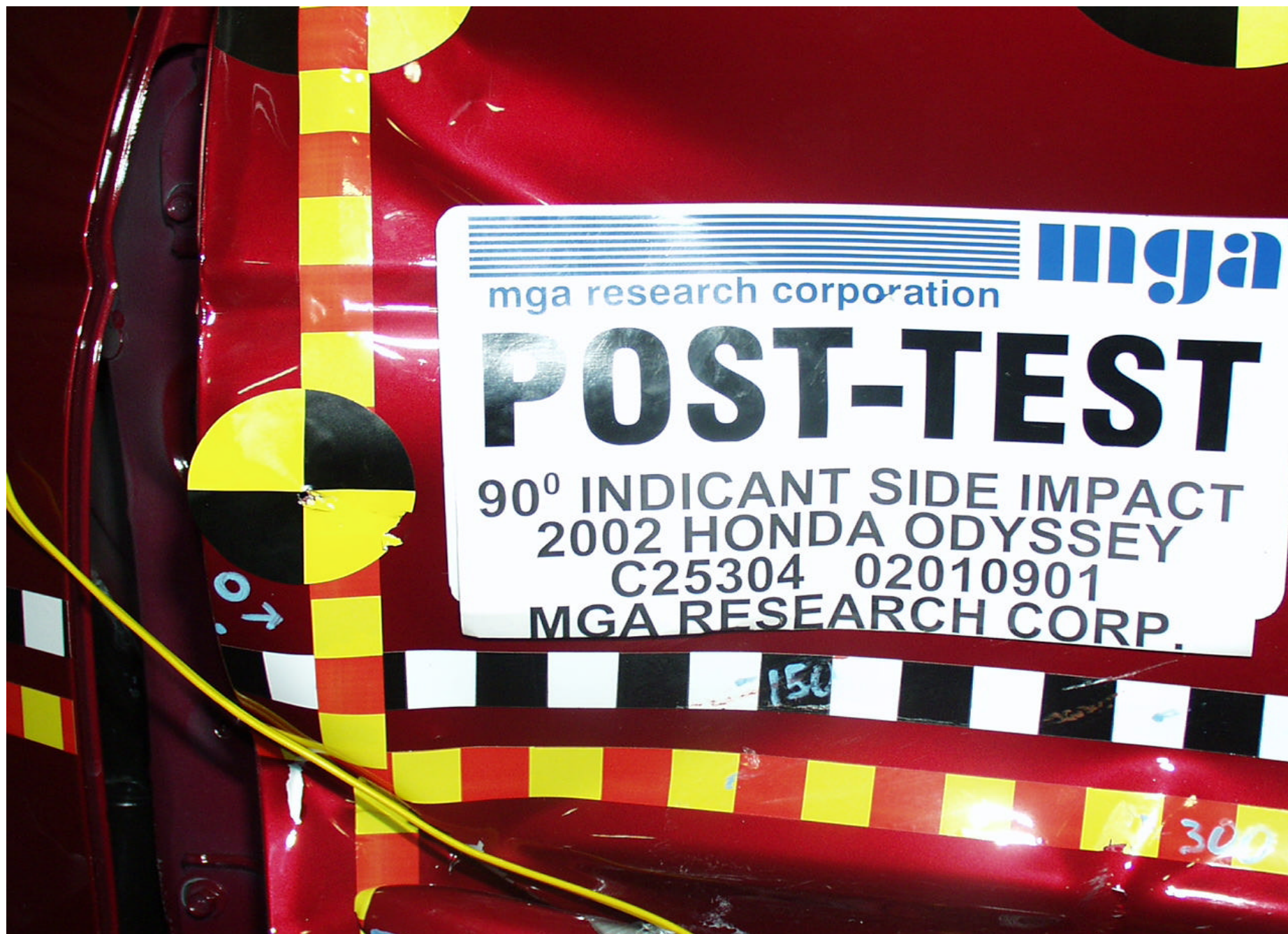
Post-Test Left Front Impact Point on Vehicle
