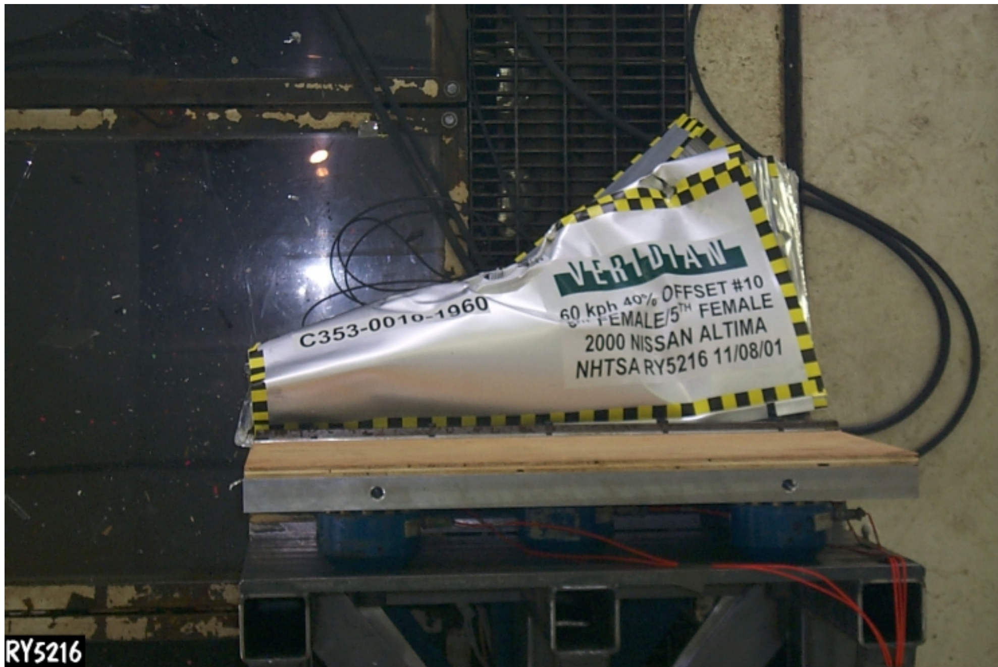
Figure A-44: POST-TEST BARRIER TOP VIEW
