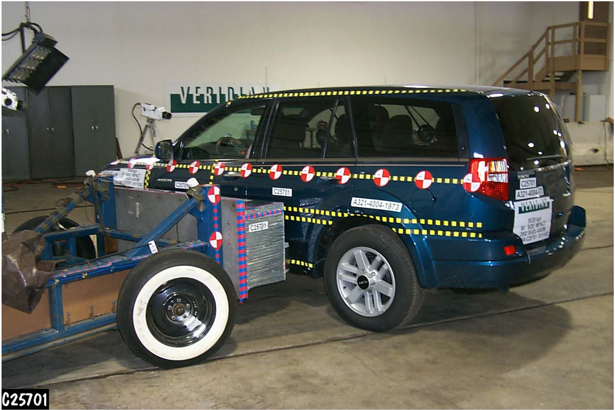
Figure A-30: PRE-TEST RIGHT SIDE VIEW OF MDB WITH IMPACTOR FACE IN POSITION
