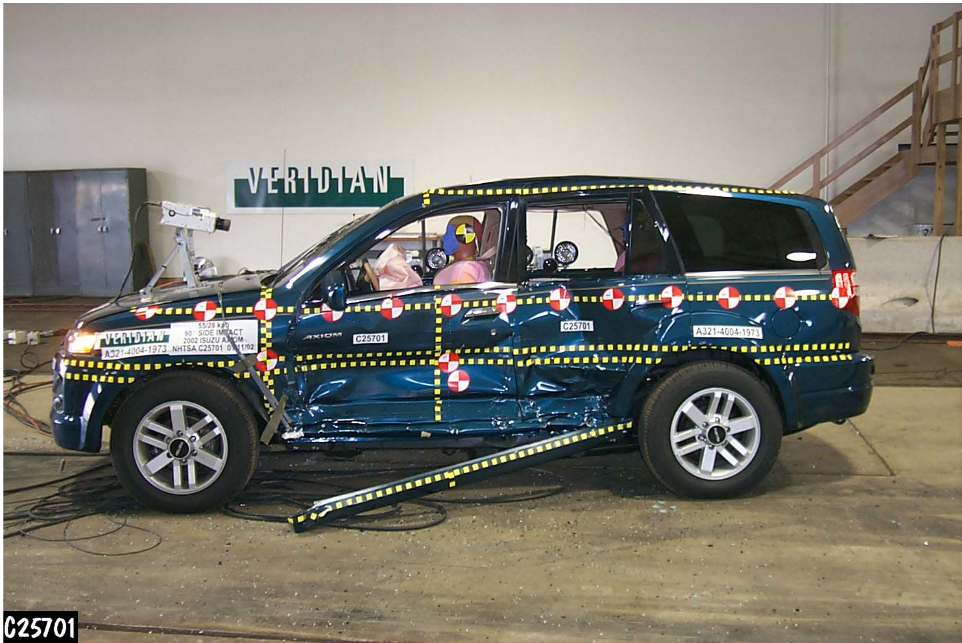
Figure A-6: POST-TEST IMPACTED SIDE VIEW OF TEST VEHICLE
