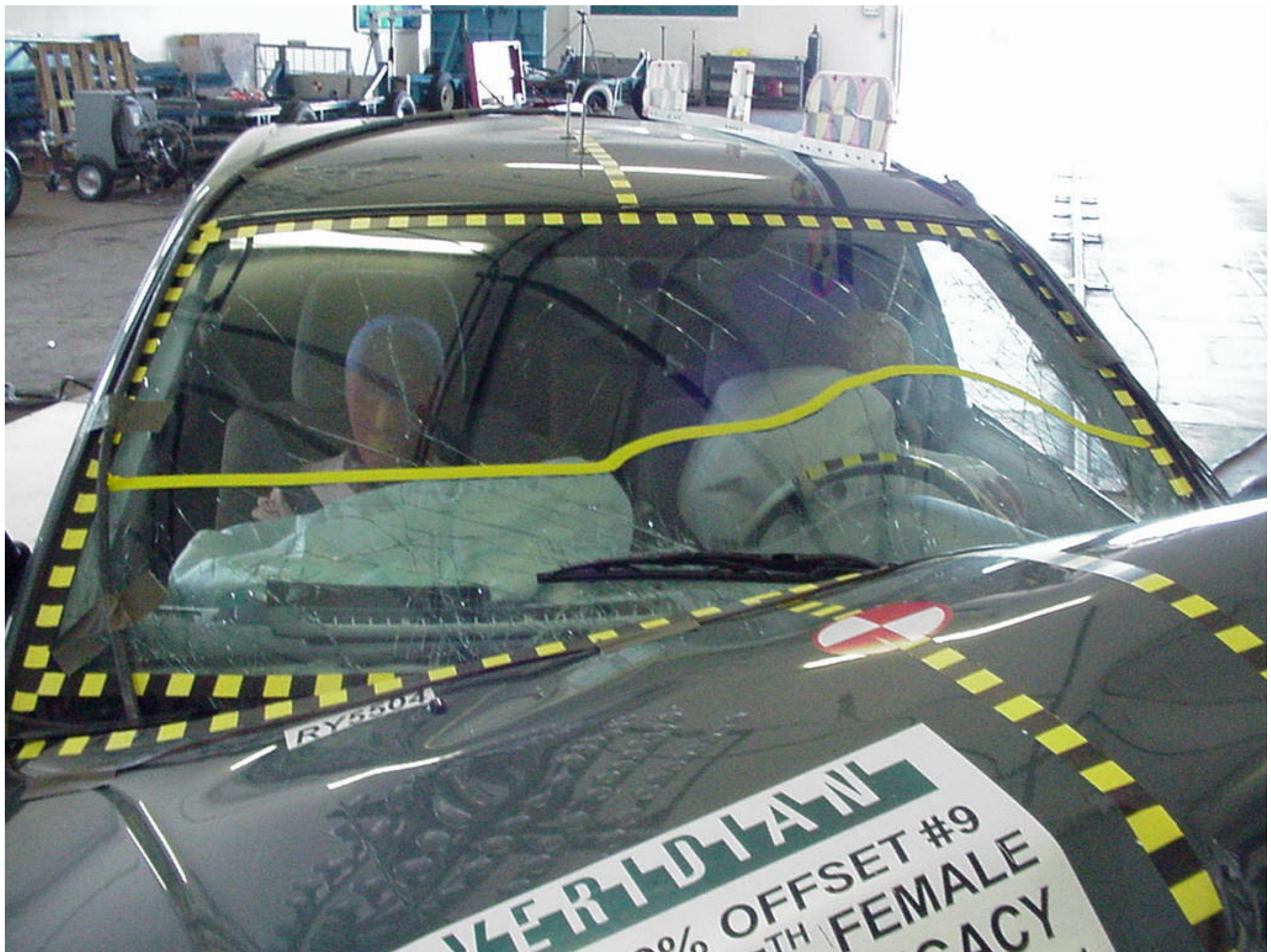
Figure A-12 POST-TEST WINDSHIELD VIEW
