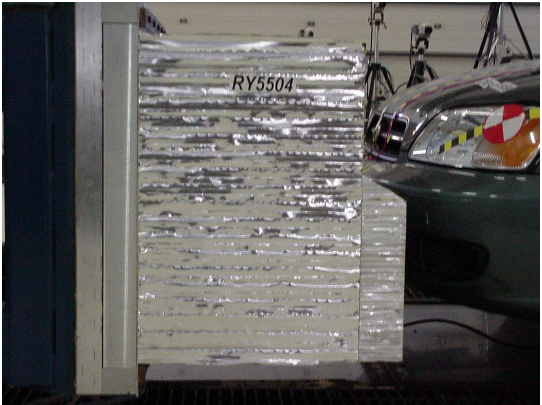
Figure A-41 PRE-TEST BARRIER RIGHT SIDE VIEW
