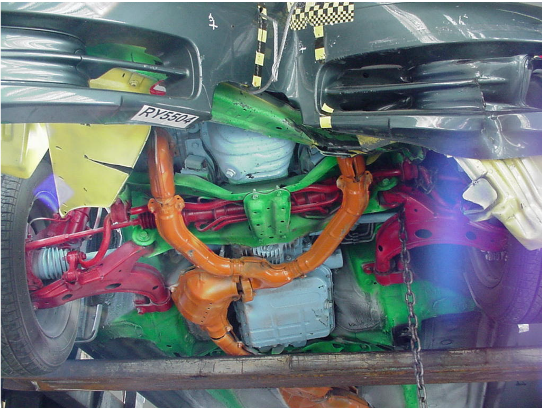
Figure A-16 POST-TEST FRONT UNDERBODY VIEW
