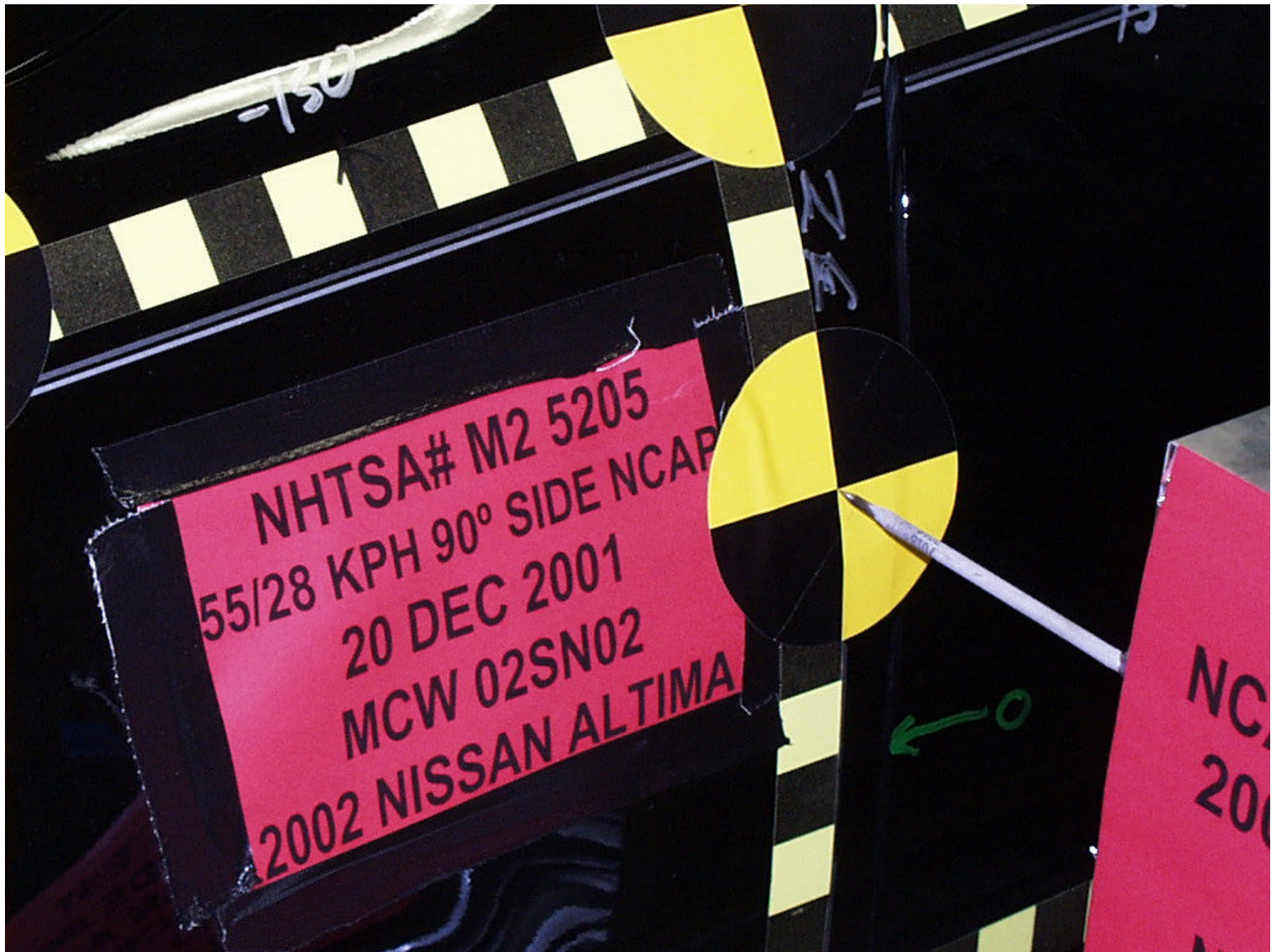
Figure A-27: PRE-TEST CLOSE-UP OF IMPACT POINT TARGET SHOWING WELDING ROD
