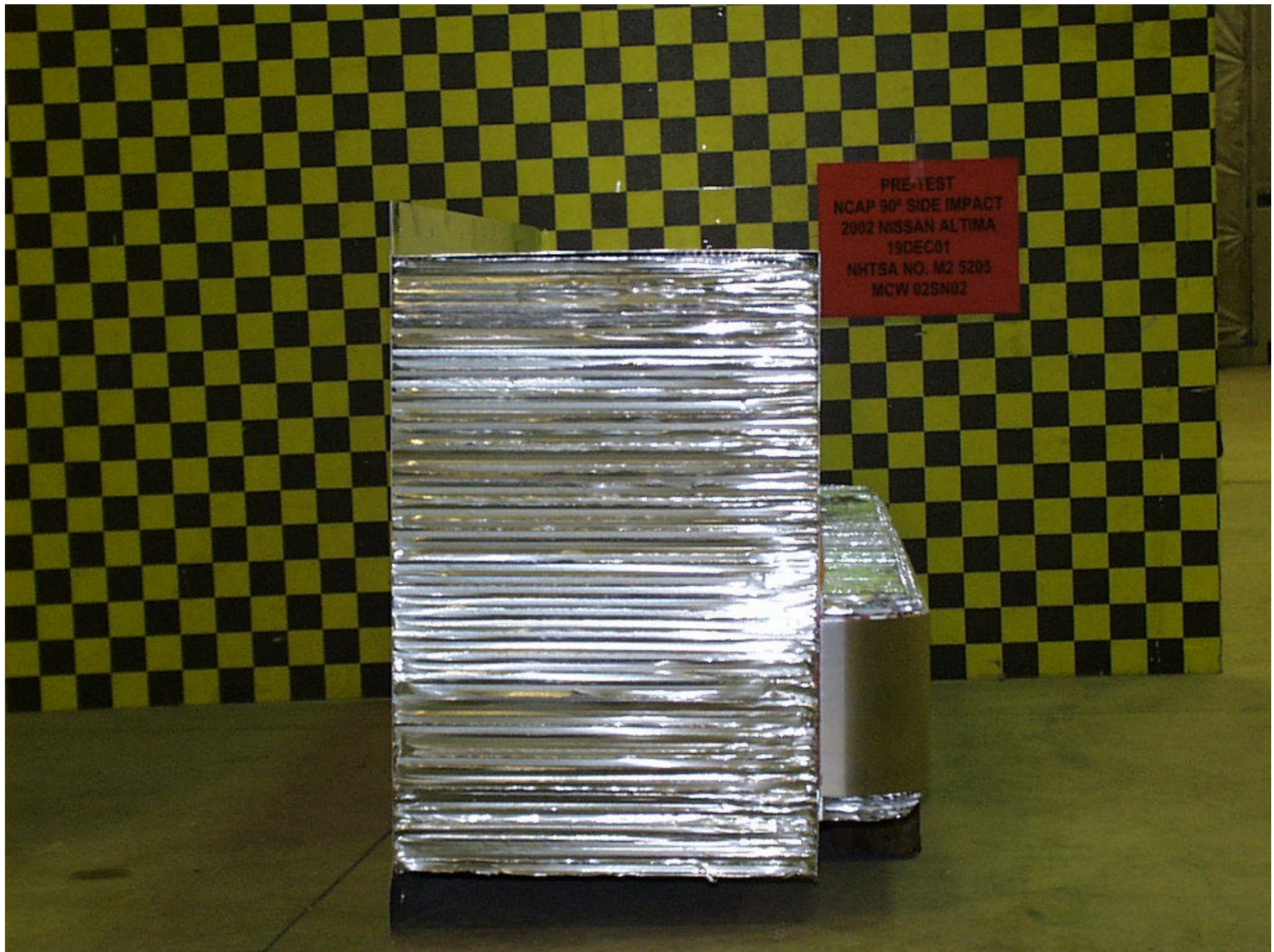
Figure A-41: PRE-TEST ALUMINUM BARRIER RIGHT SIDE
