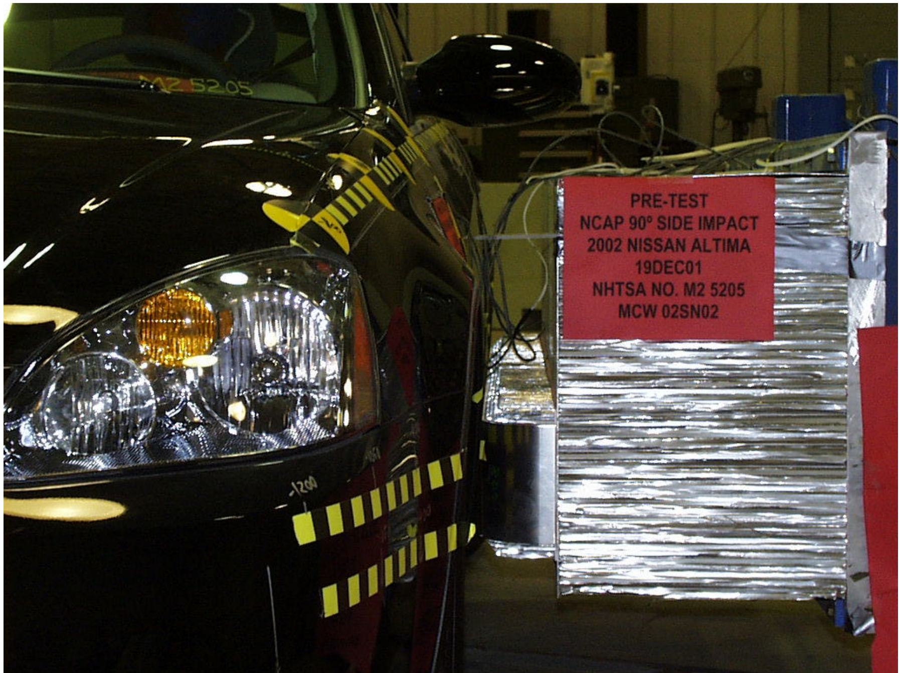
Figure A-21: PRE-TEST LEFT SIDE VIEW OF MDB IN IMPACT POSITION
