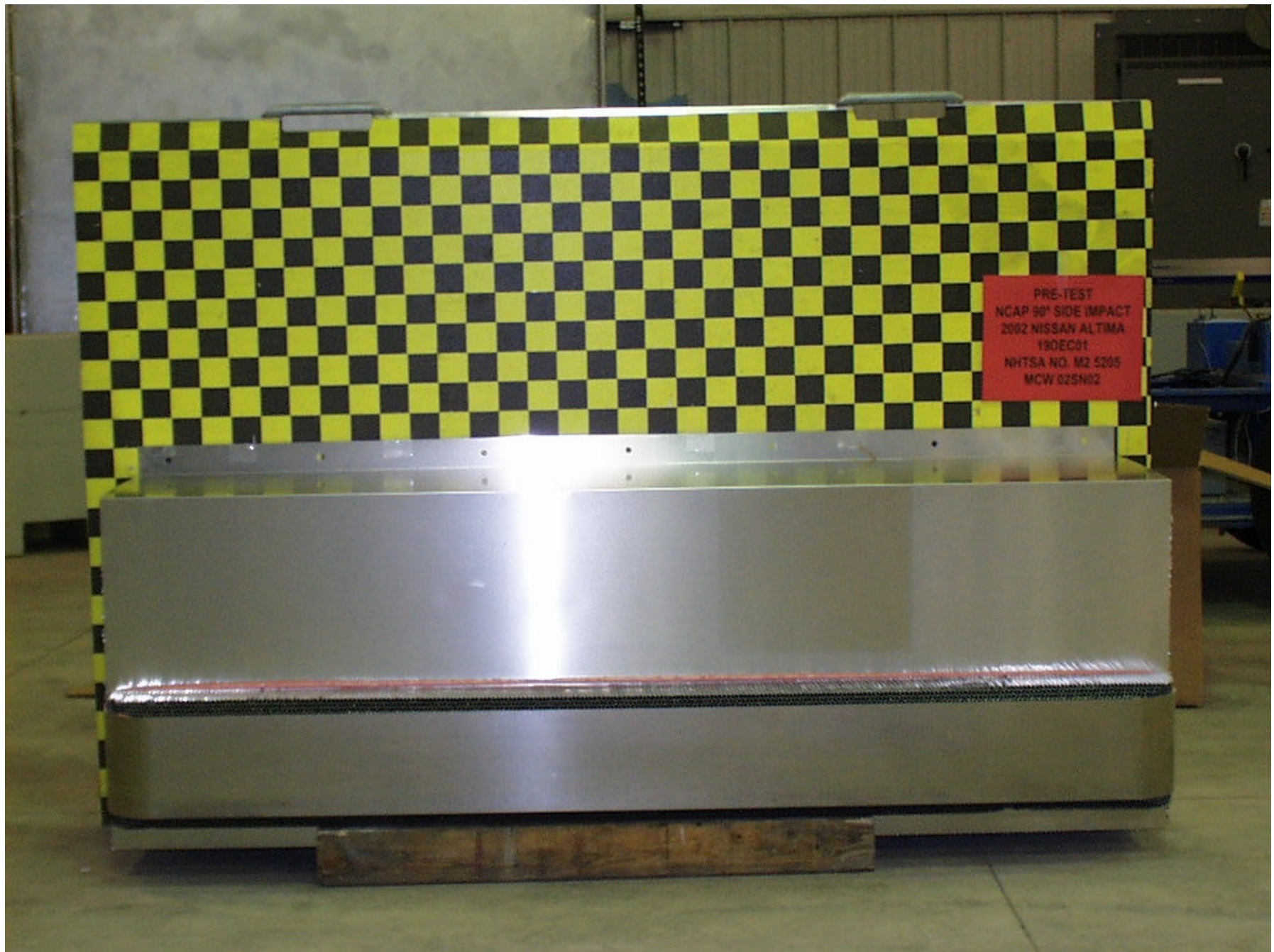
Figure A-37: PRE-TEST ALUMINUM BARRIER FRONT
