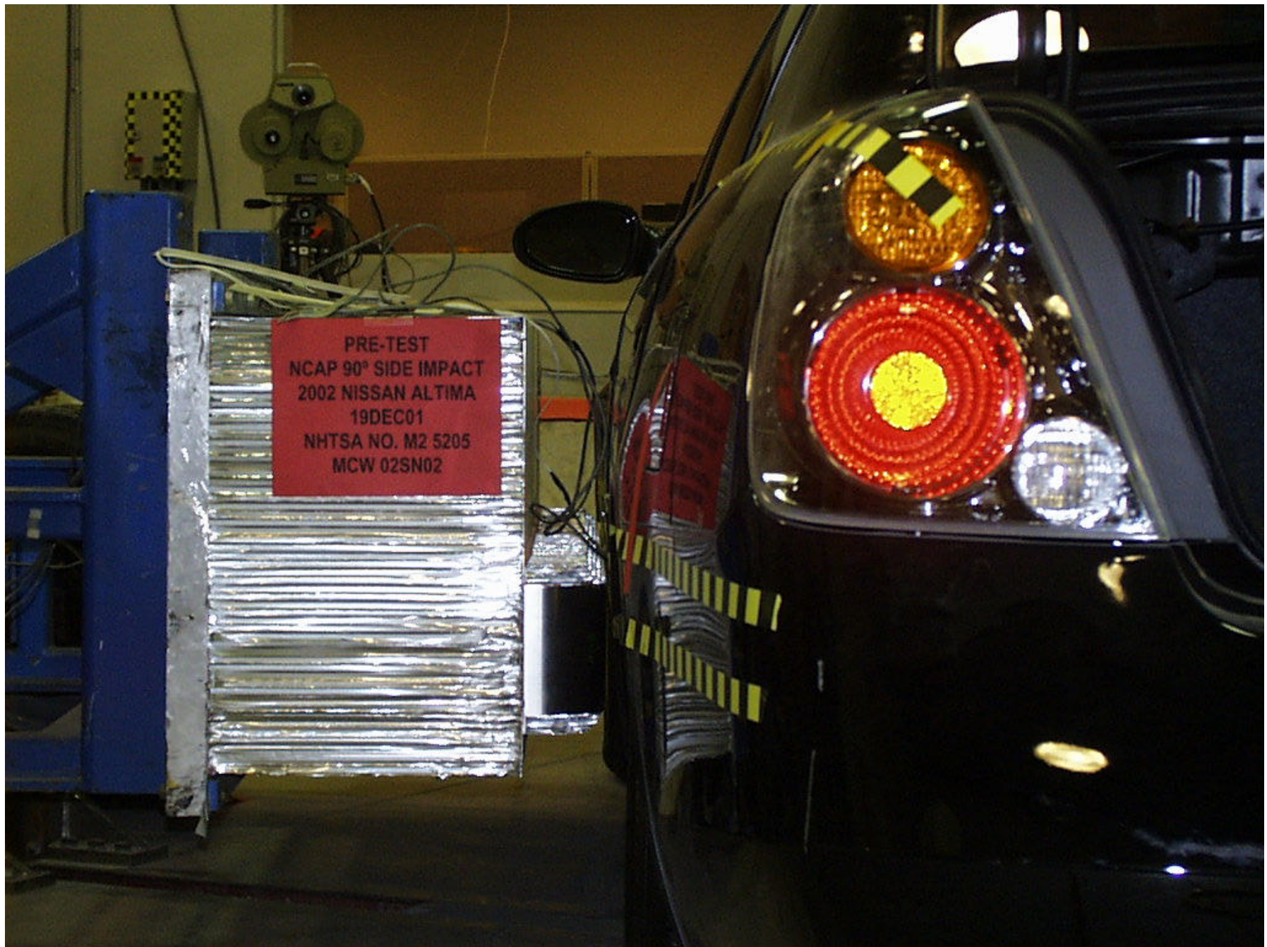
Figure A-23: PRE-TEST RIGHT SIDE VIEW OF MDB IN IMPACT POSITION
