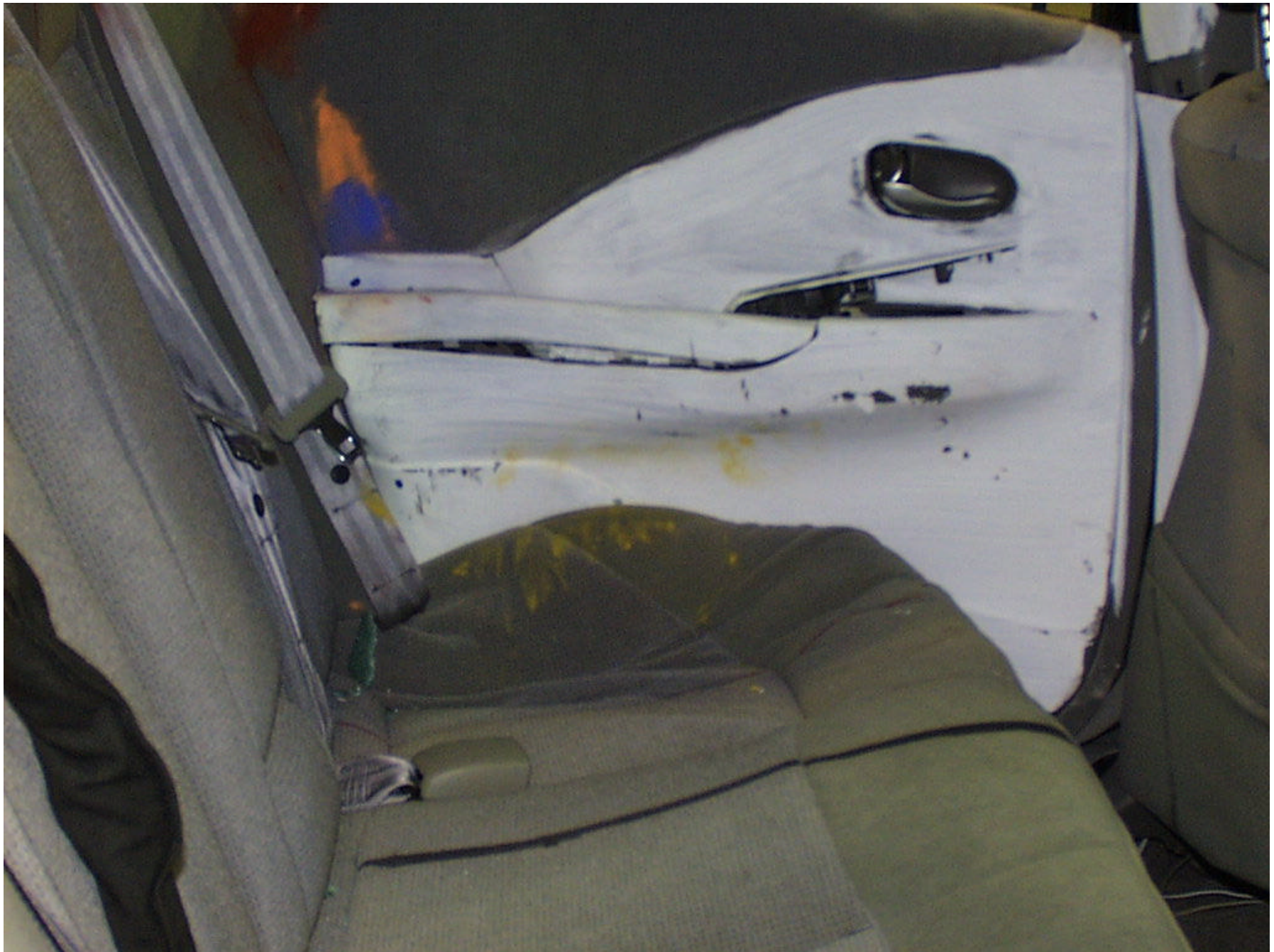
Figure A-20: POST-TEST INTERIOR OF REAR DOOR SHOWING SID IMPACT LOCATIONS
