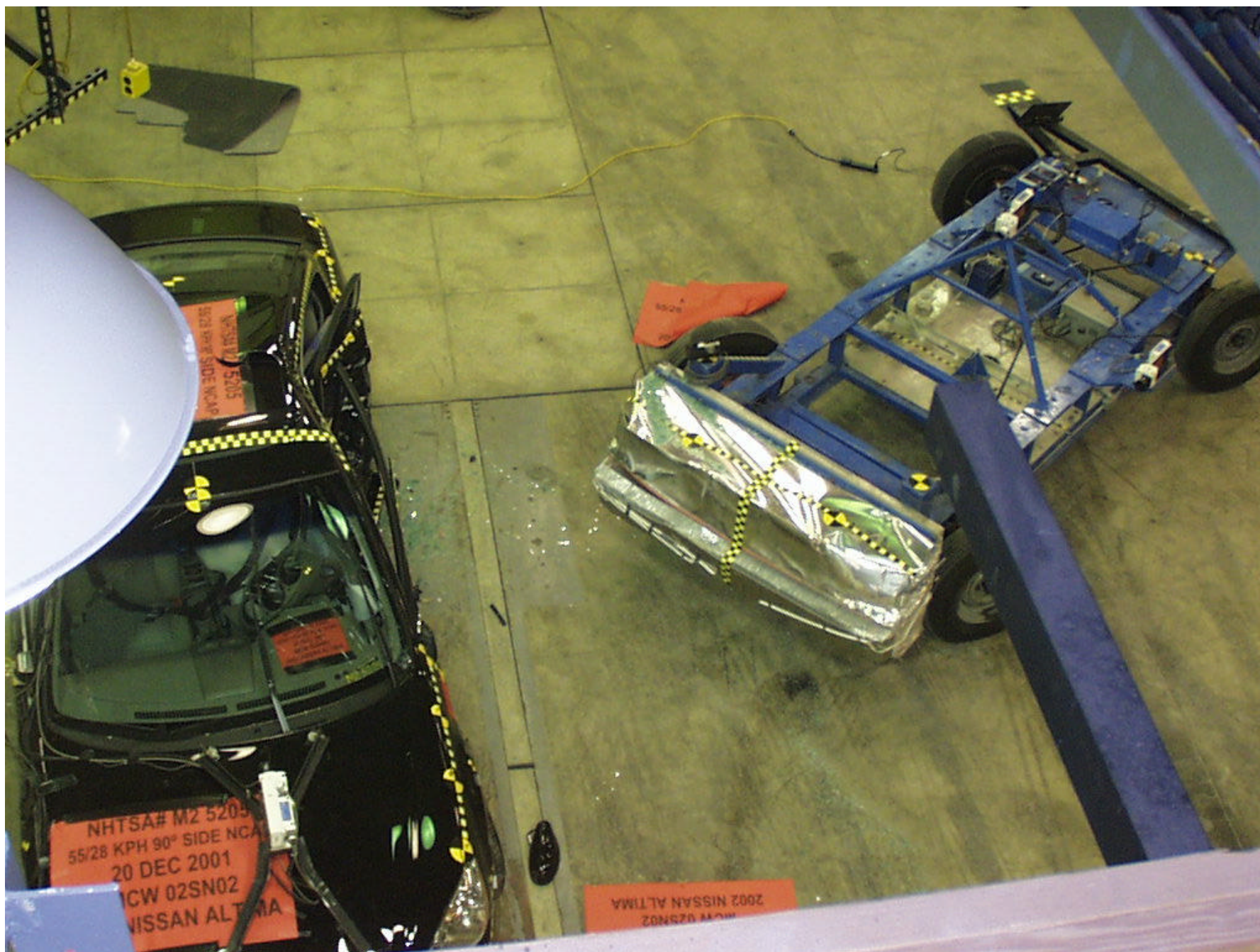
Figure A-26: POST-TEST OVERHEAD VIEW OF MDB
