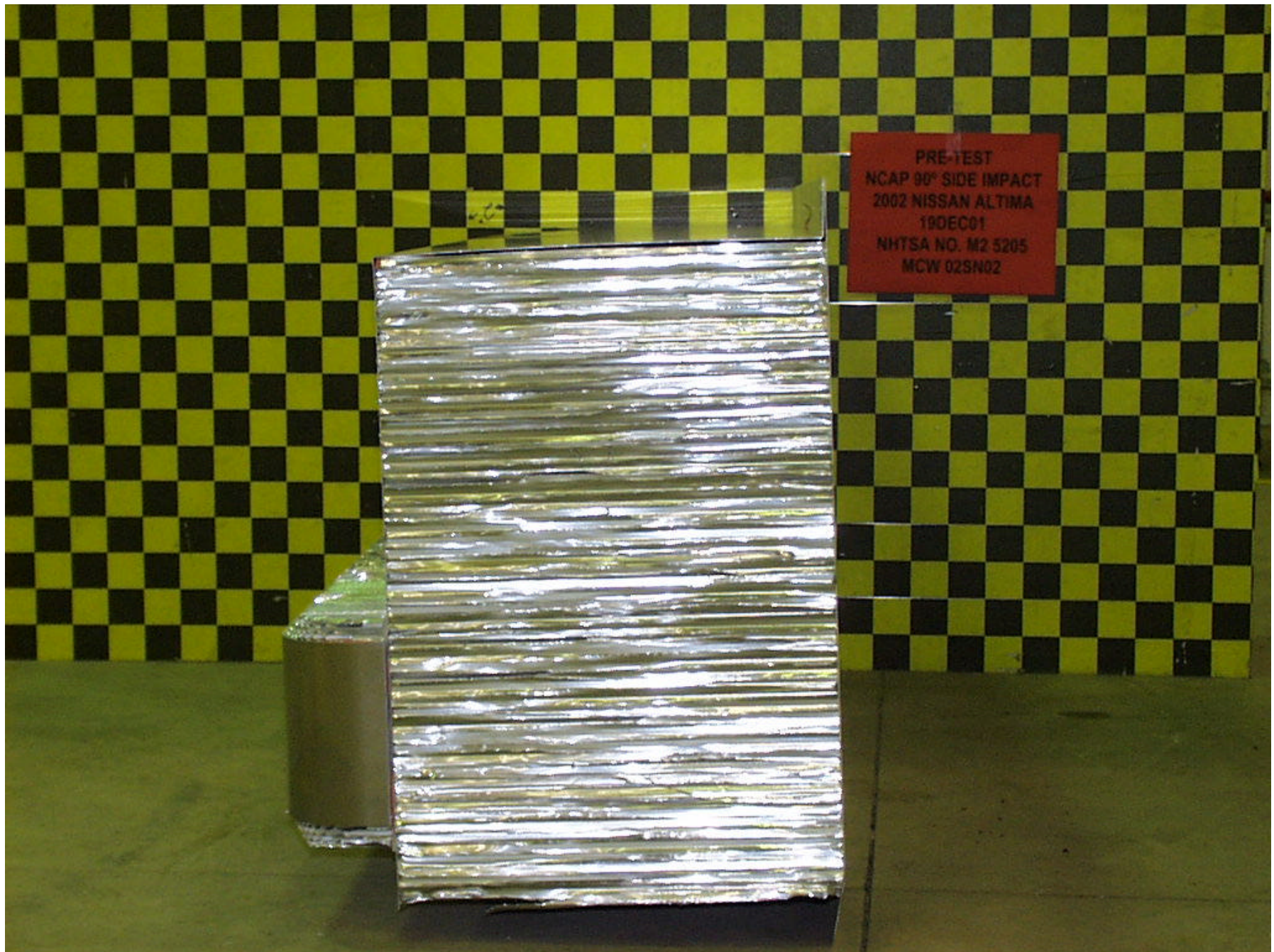
Figure A-39: PRE-TEST ALUMINUM BARRIER LEFT SIDE
