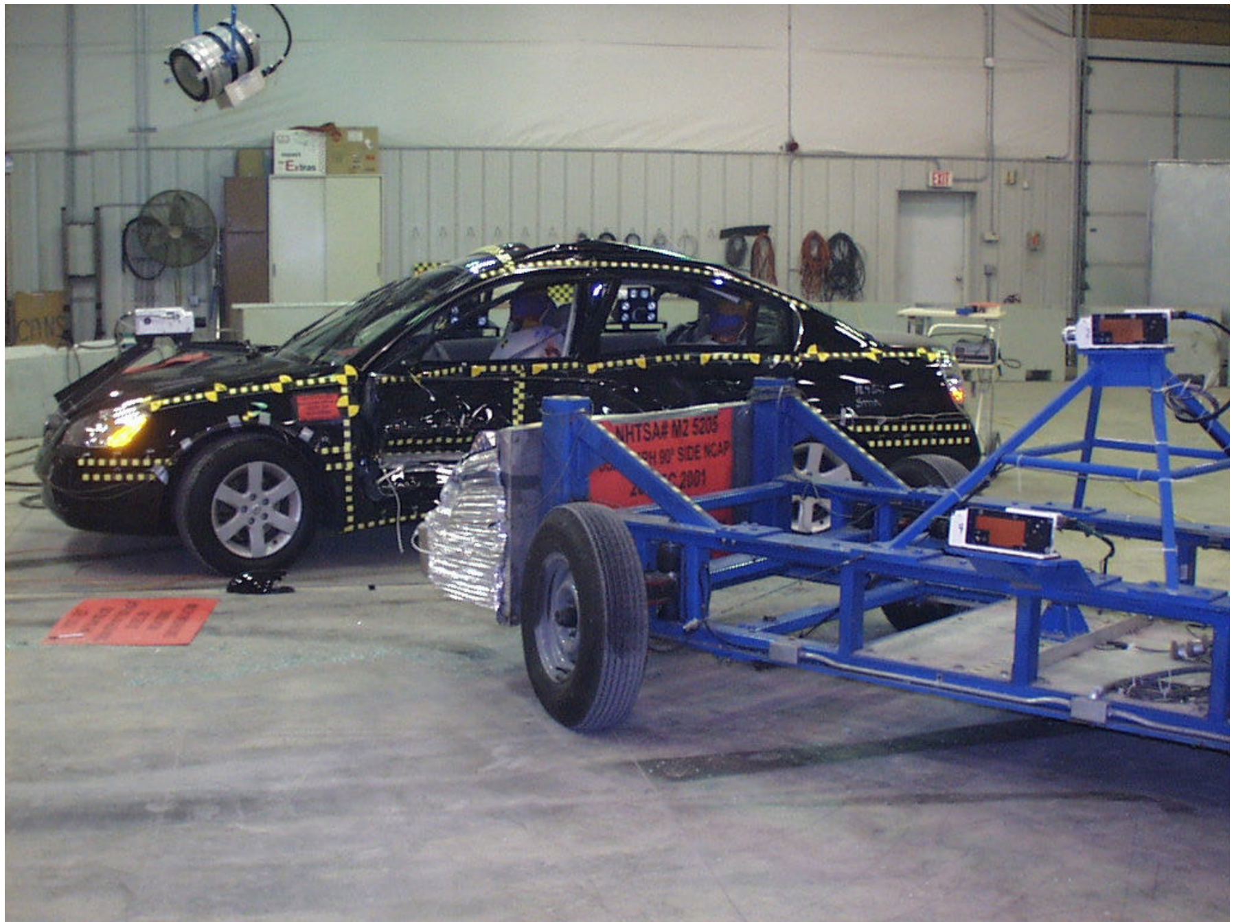
Figure A-22: POST-TEST LEFT SIDE VIEW OF MDB
