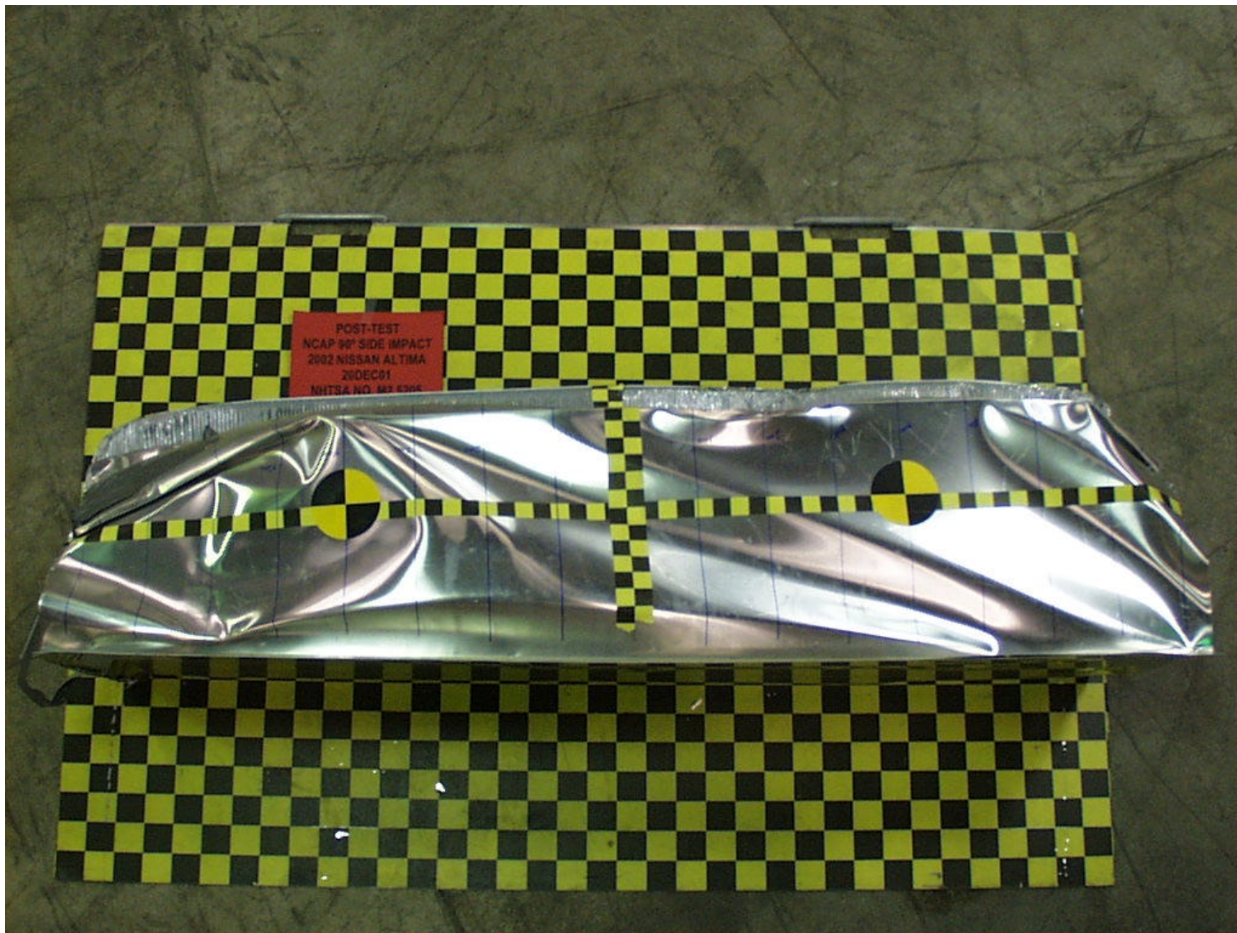
Figure A-44: POST-TEST ALUMINUM BARRIER OVERHEAD
