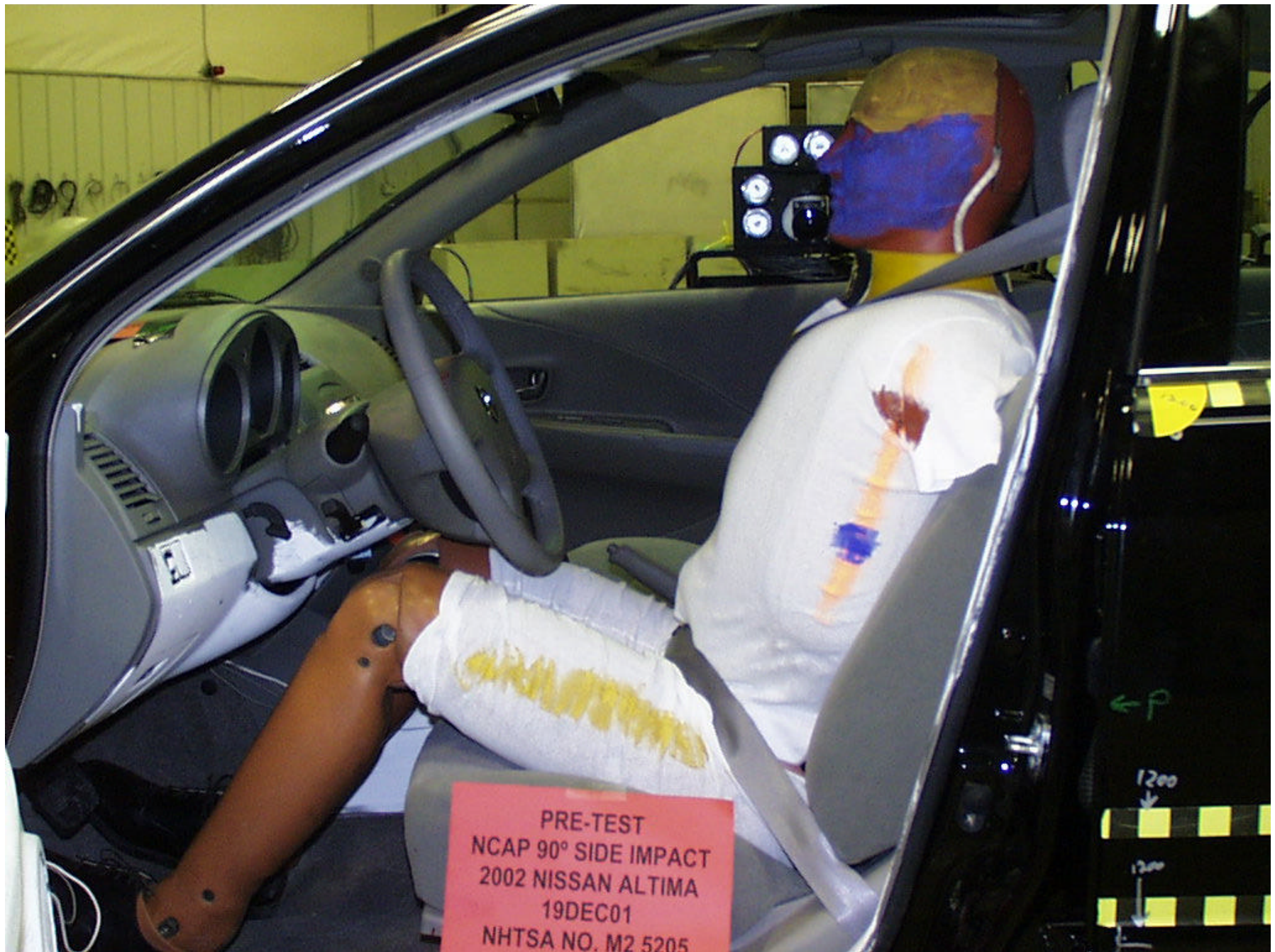
Figure A-13: PRE-TEST LEFT OCCUPANT COMPARTMENT VIEW OF FRONT SID
