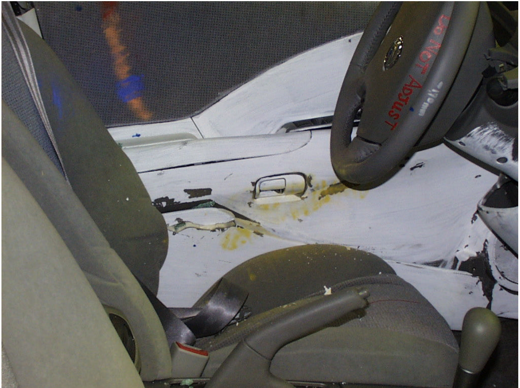
Figure A-18: POST-TEST INTERIOR OF FRONT DOOR SHOWING SID IMPACT LOCATIONS
