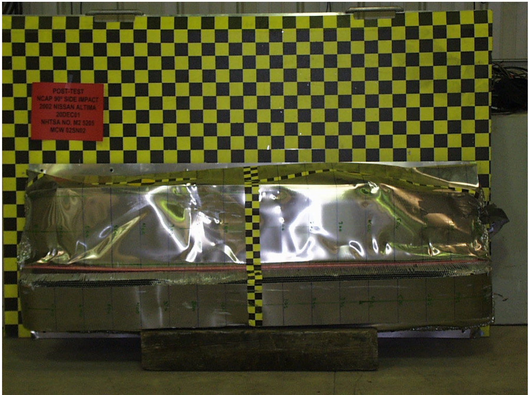
Figure A-38: POST-TEST ALUMINUM BARRIER FRONT
