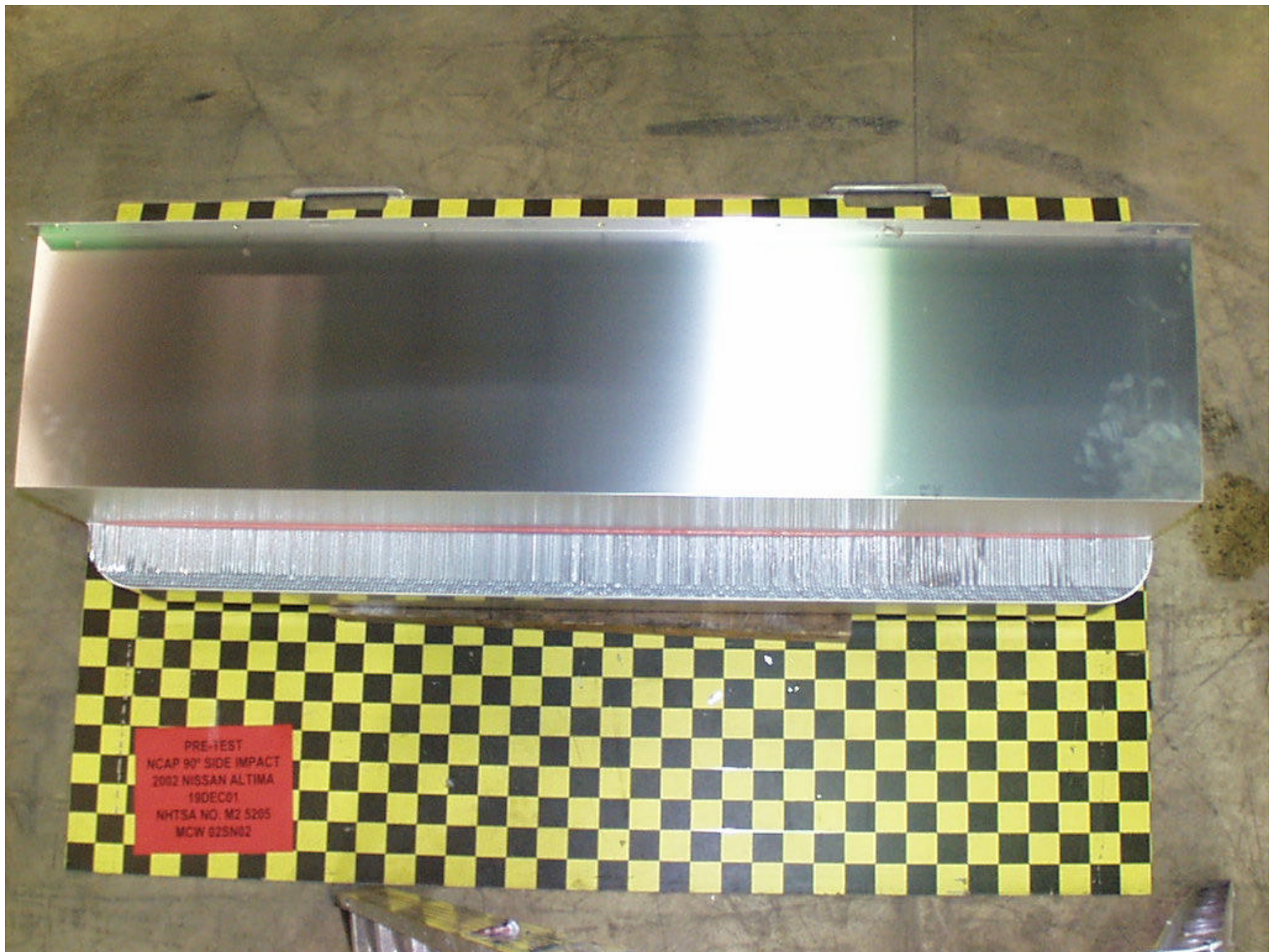
Figure A-43: PRE-TEST ALUMINUM BARRIER OVERHEAD
