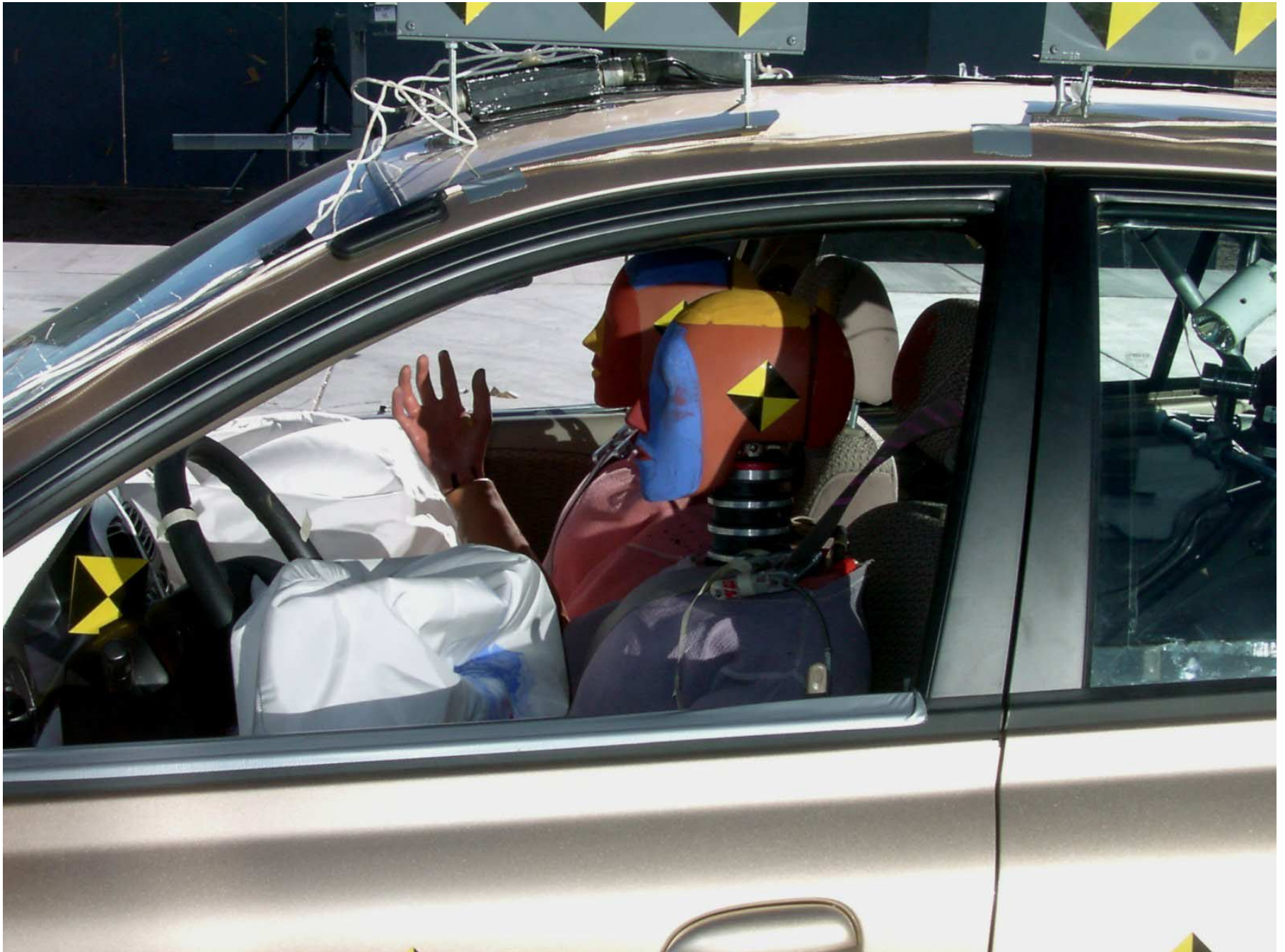
Figure A-28: Driver Dummy Through Window, Post-Test
