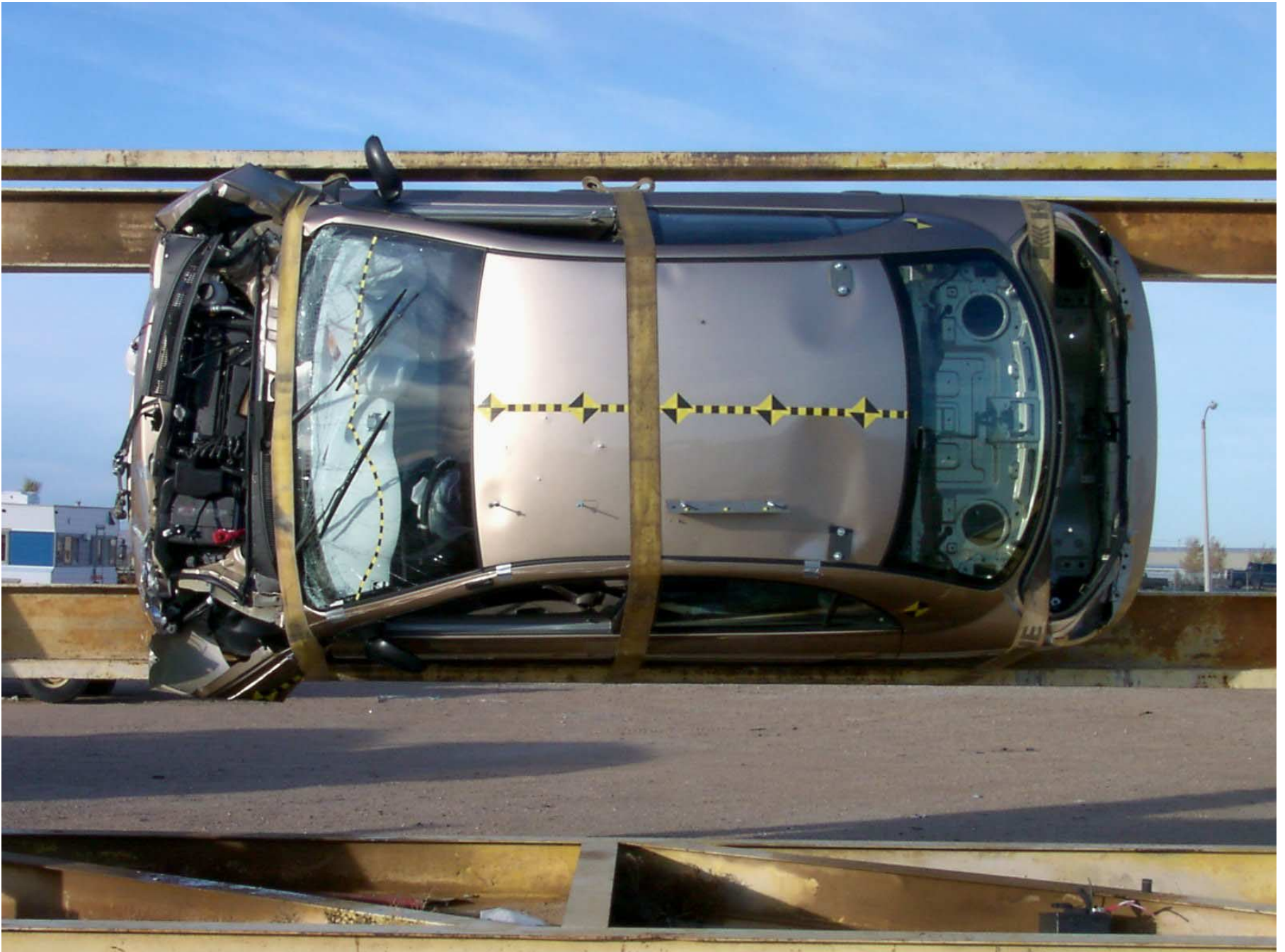
Figure A-57: Vehicle on Rollover Device
