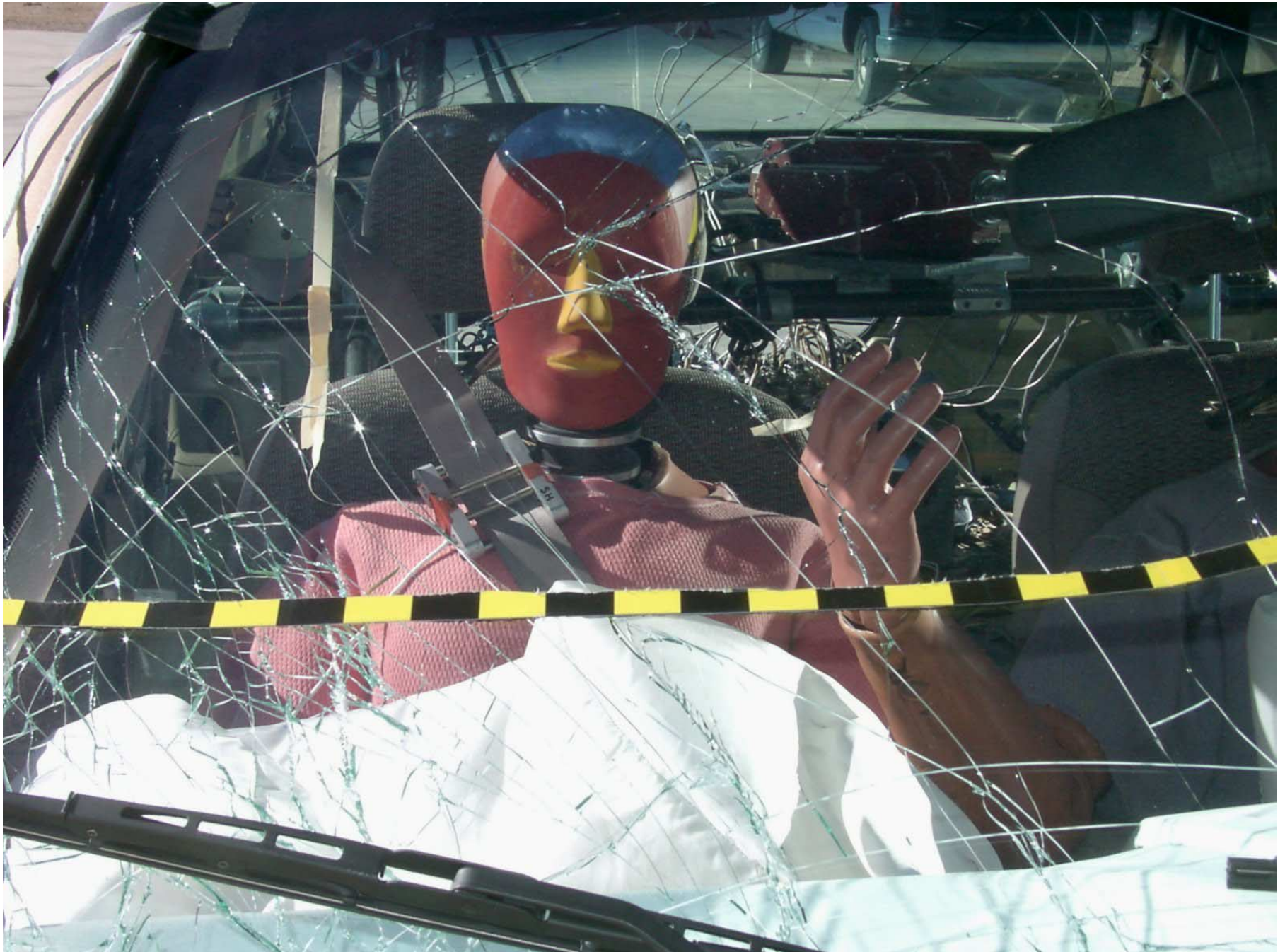
Figure A-42: Passenger Dummy Front View, Post-Test
