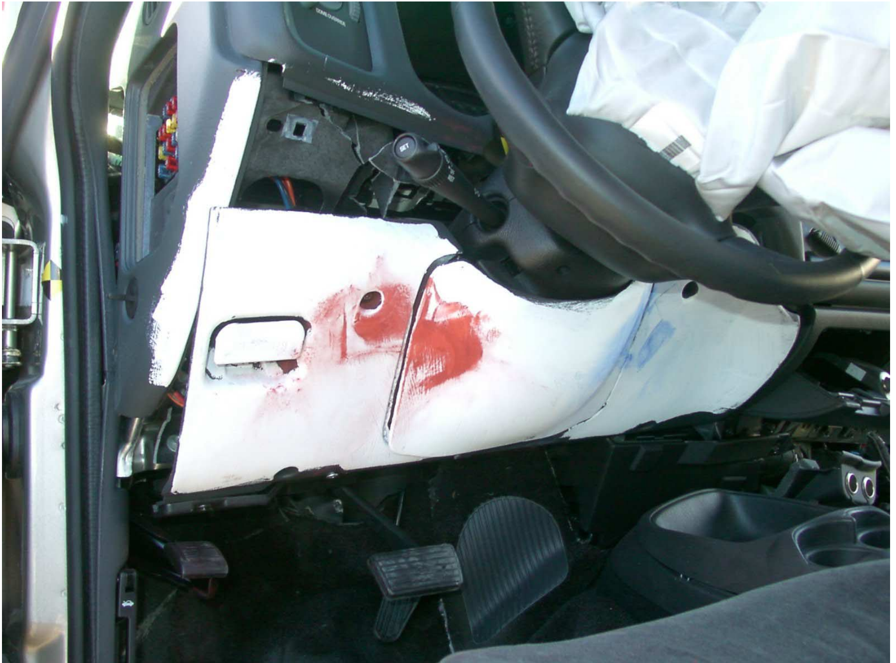
Figure A-36: Driver Side Knee Bolster, Post-Test
