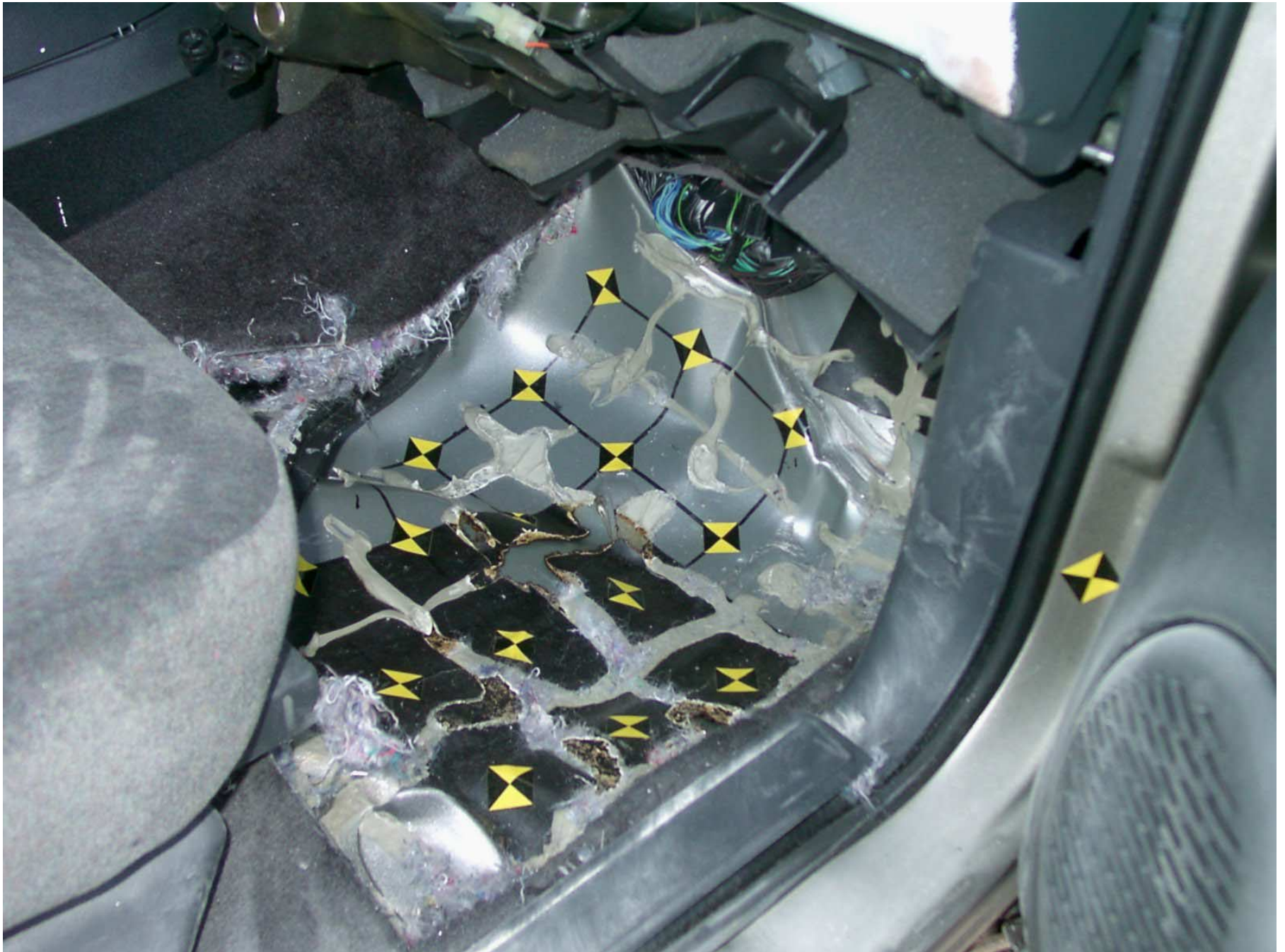
Figure A-52: Passenger Side Floor Pan, Post-Test
