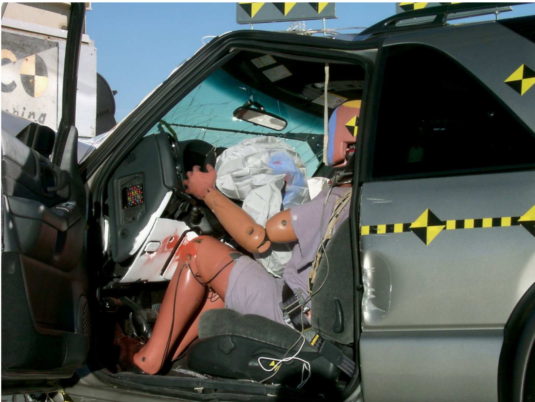
Figure A-30: Driver Dummy Door Open, Post-Test
