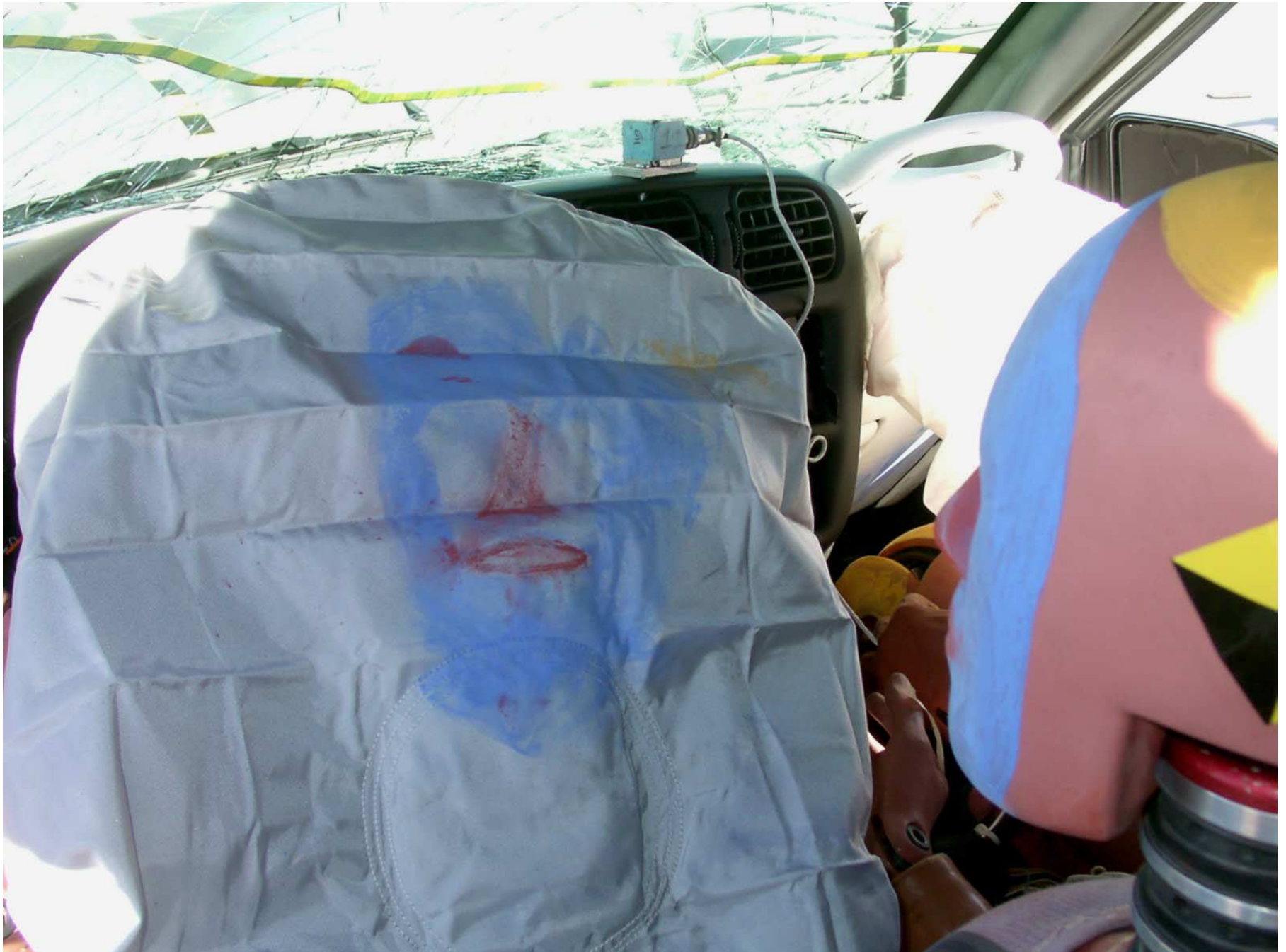
Figure A-40: Driver Dummy Contact, Post-Test
