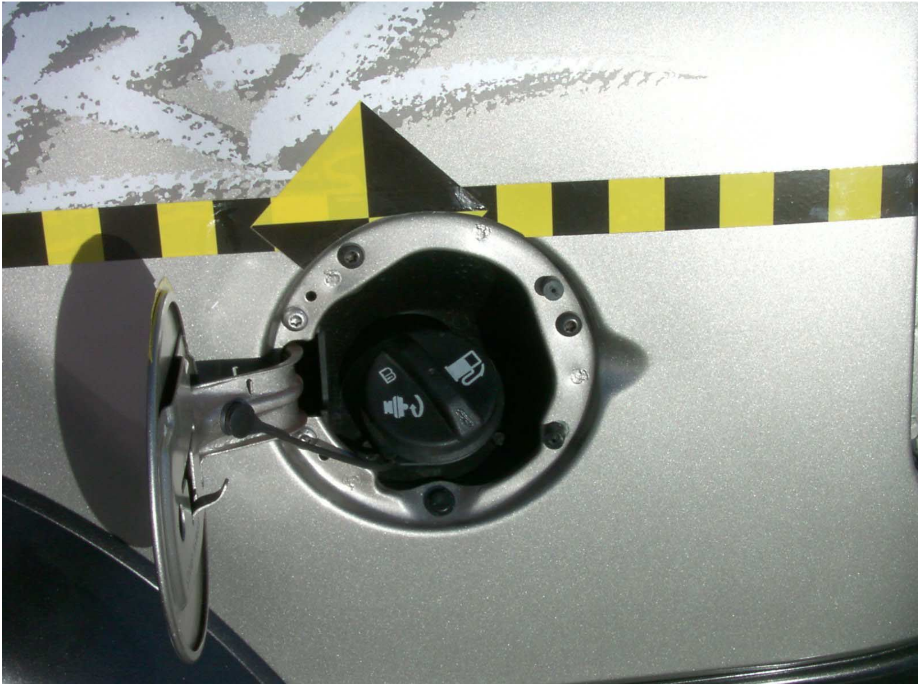
Figure A-20: Fuel Cap, Post-Test
