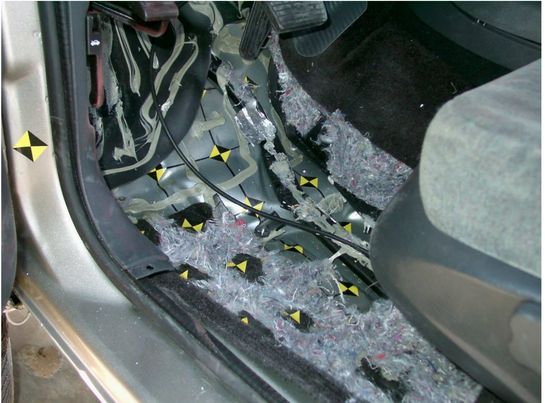
Figure A-38: Driver Side Floor Pan, Post-Test
