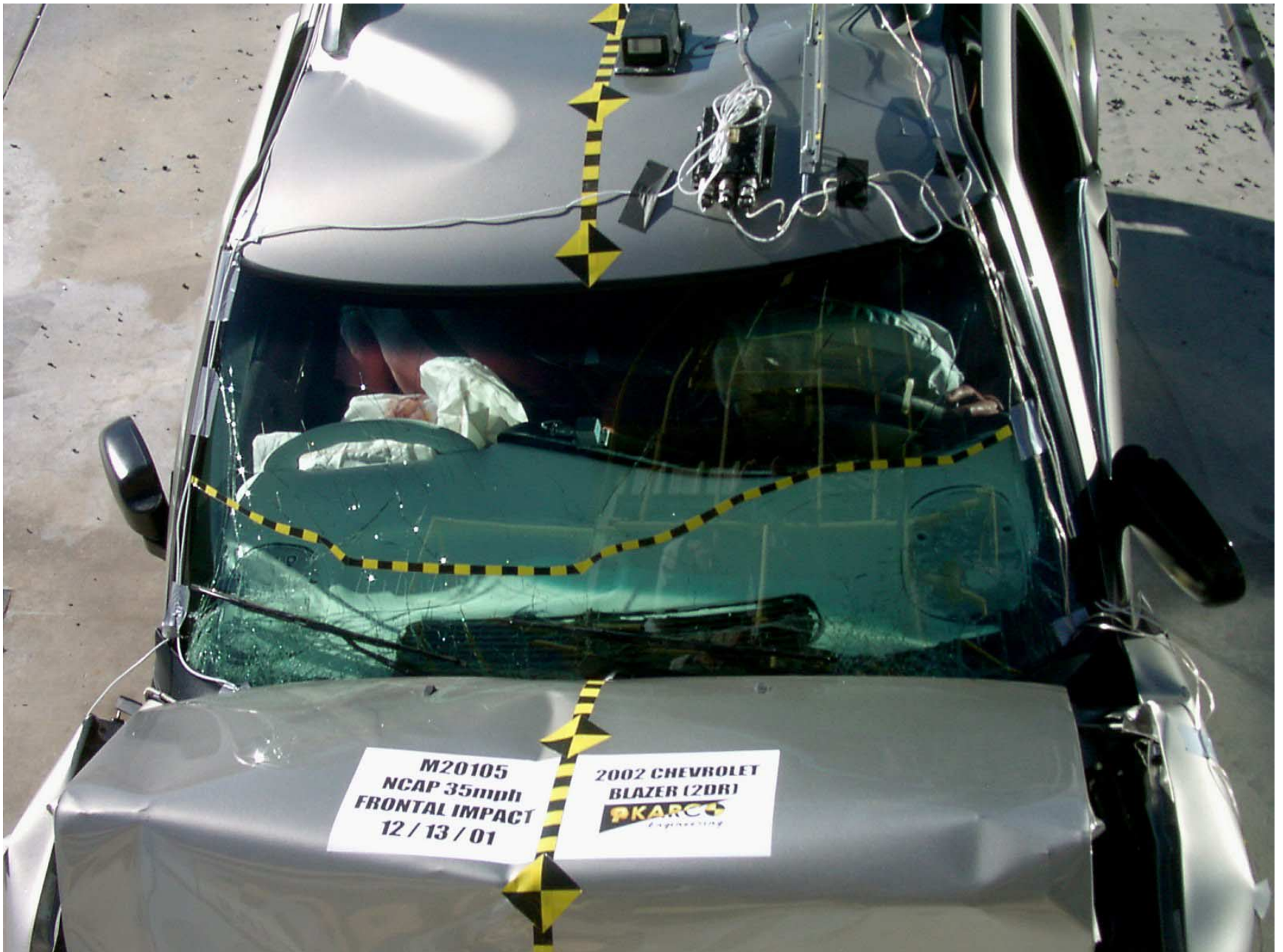
Figure A-16: Windshield, Post-Test
