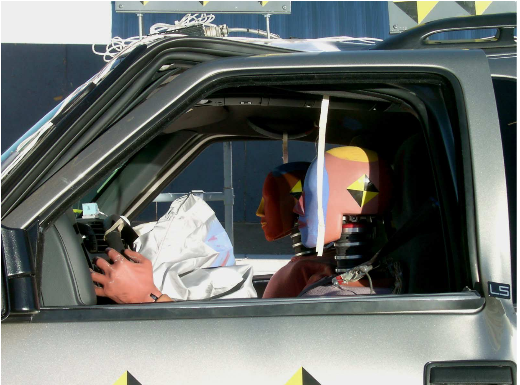
Figure A-28: Driver Dummy Through Window, Post-Test
