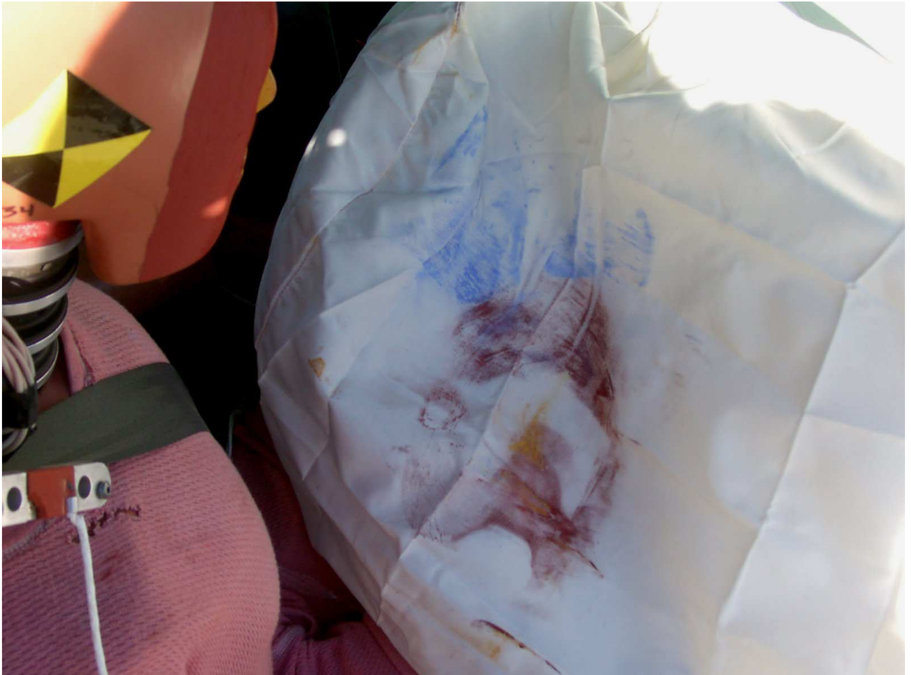
Figure A-56: Passenger Dummy Contact, Post-Test
