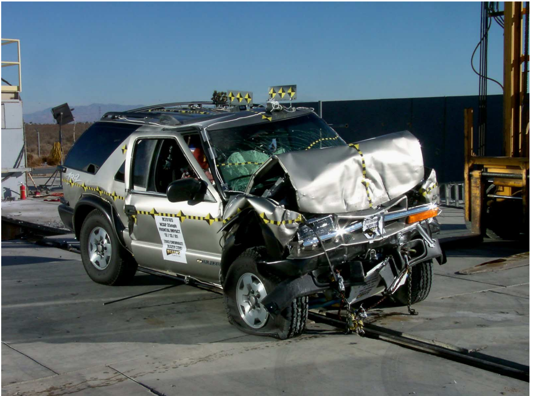
Figure A-12: Right Front View, Post-Test
