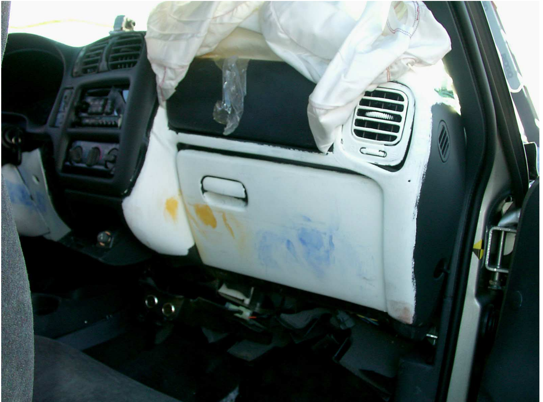
Figure A-54: Passenger Side Knee Bolster, Post-Test
