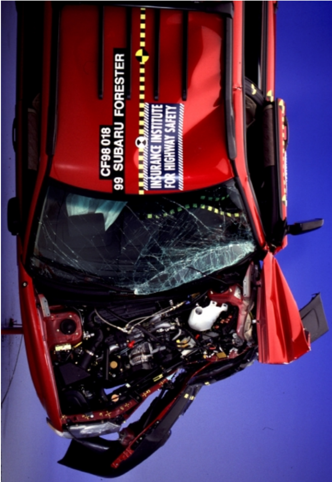
Figure 2 Overhead View of Crash Deformation — 1999 Subaru Forester
