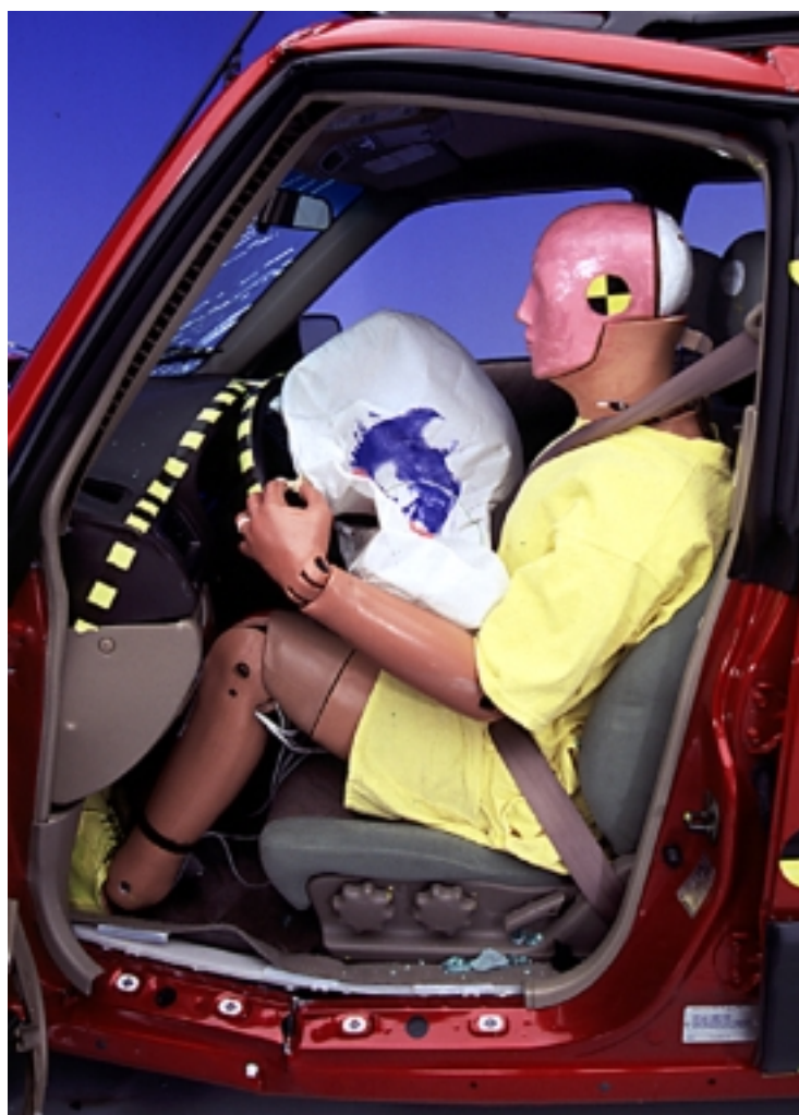
Figure 7 Dummy and Vehicle Interior, Postcrash — 1999 Subaru Forester
