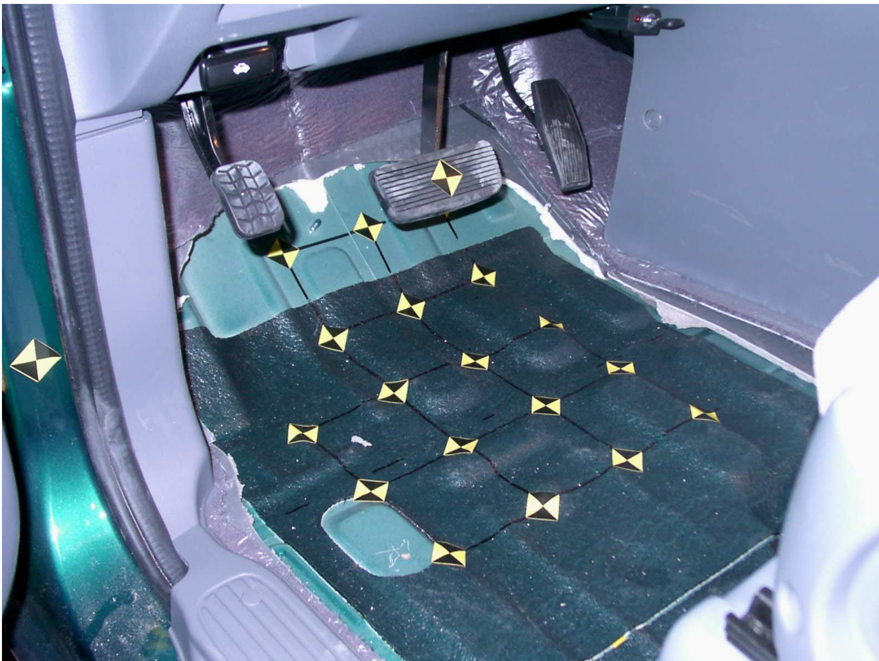
Figure A-37: Driver Side Floor Pan, Pre-Test
