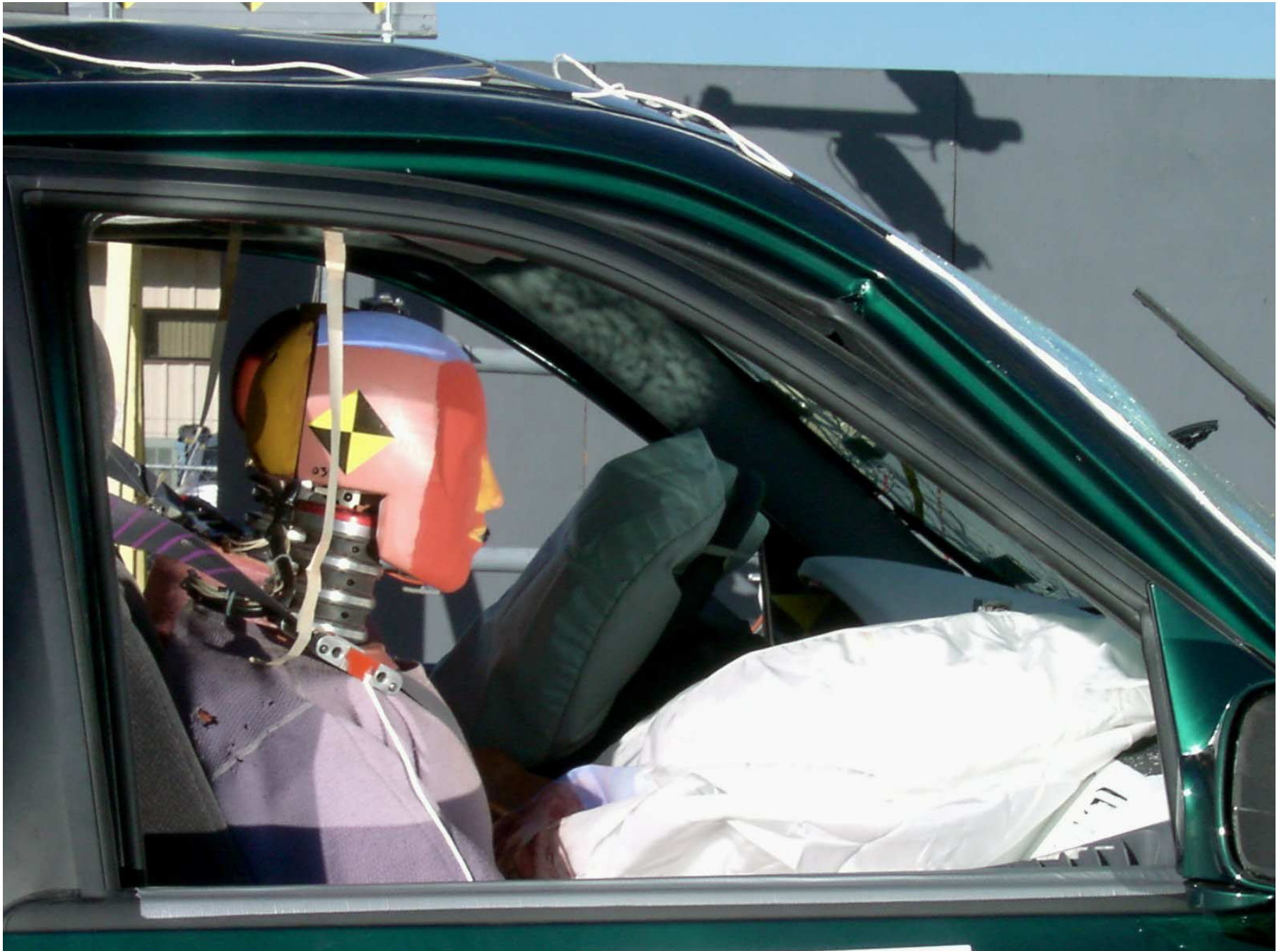
Figure A-44: Passenger Dummy Through Window, Post-Test
