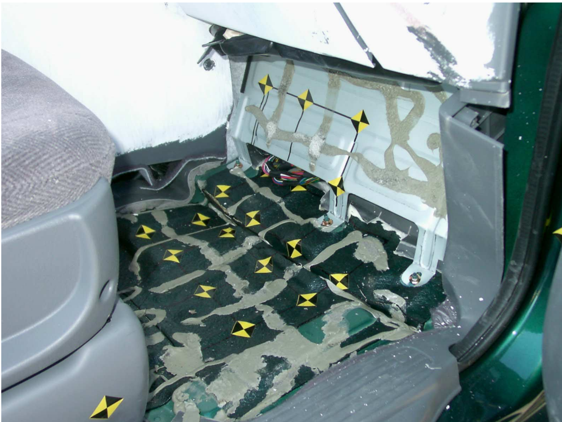
Figure A-52: Passenger Side Floor Pan, Post-Test
