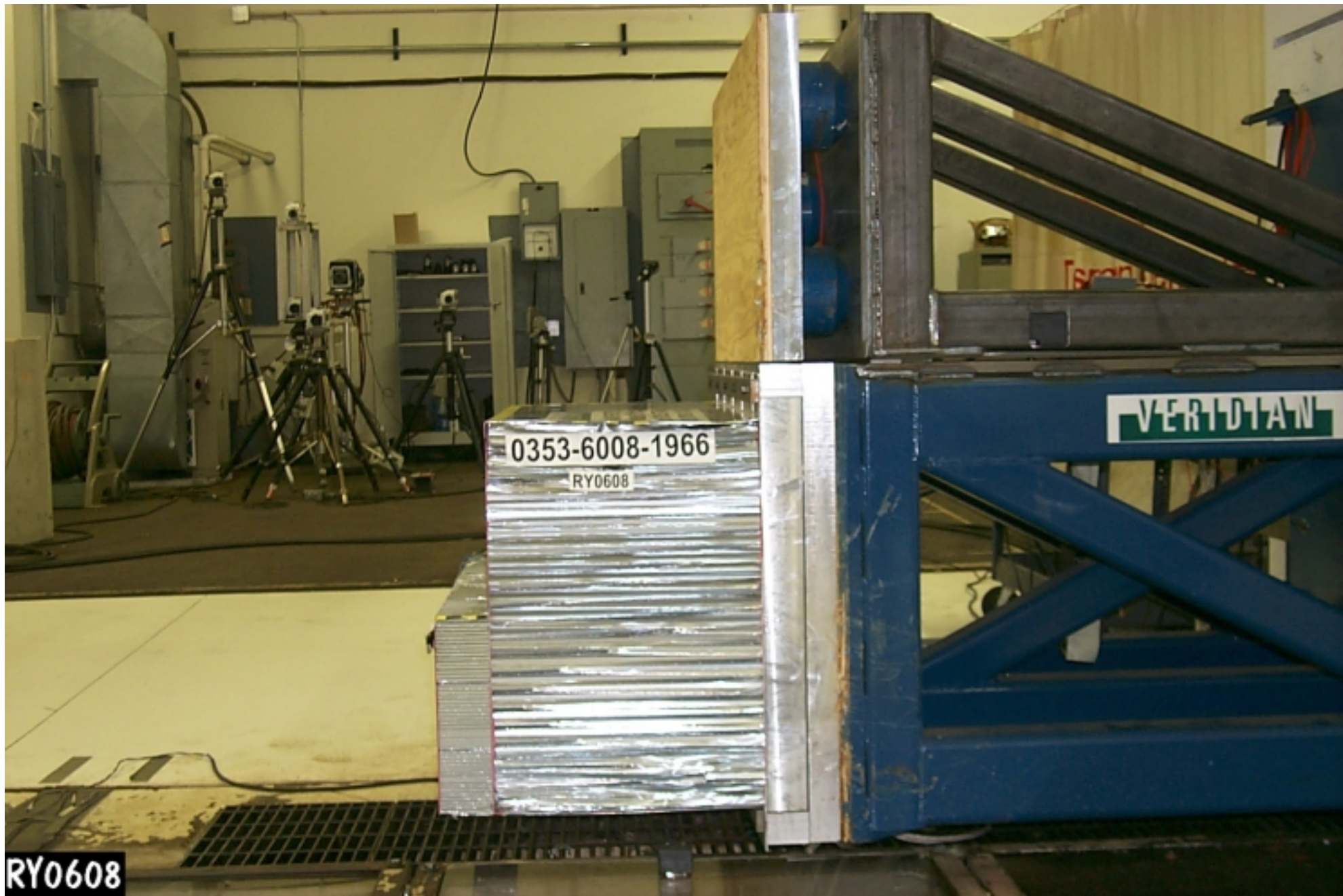
Figure A-41: PRE-TEST BARRIER RIGHT SIDE VIEW
