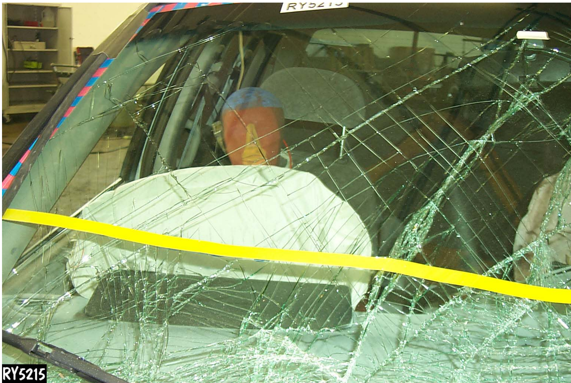
Figure A-32: POST-TEST PASSENGER HEAD LOCATION
