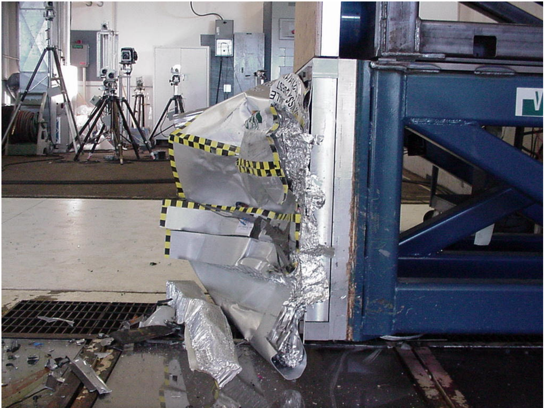
Figure A-42 POST-TEST BARRIER RIGHT SIDE VIEW
