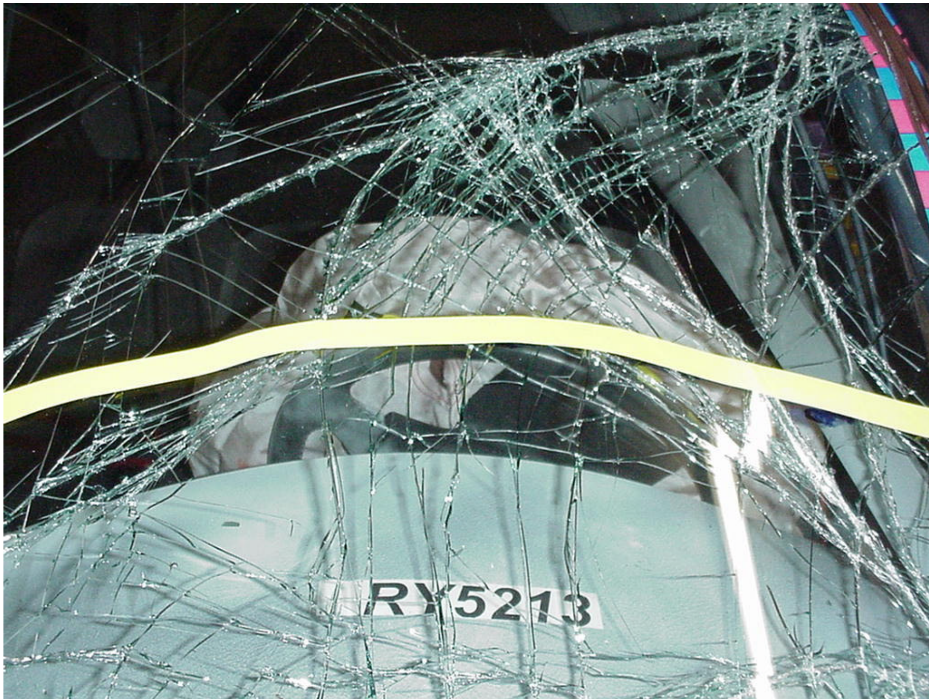
Figure A-30 POST-TEST DRIVER HEAD LOCATION
