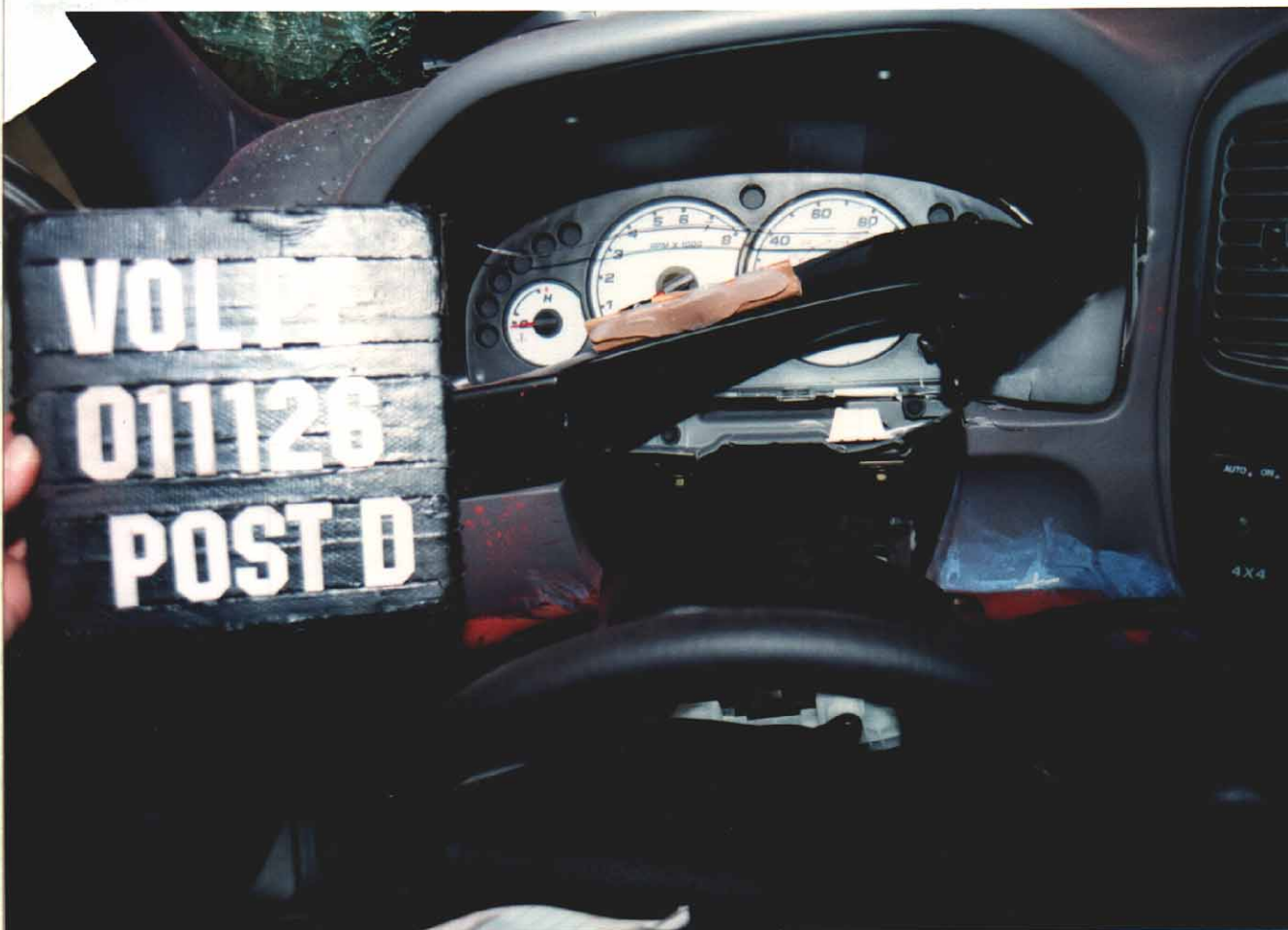
Figure A-81 Post-Test Steering Column Damage View
