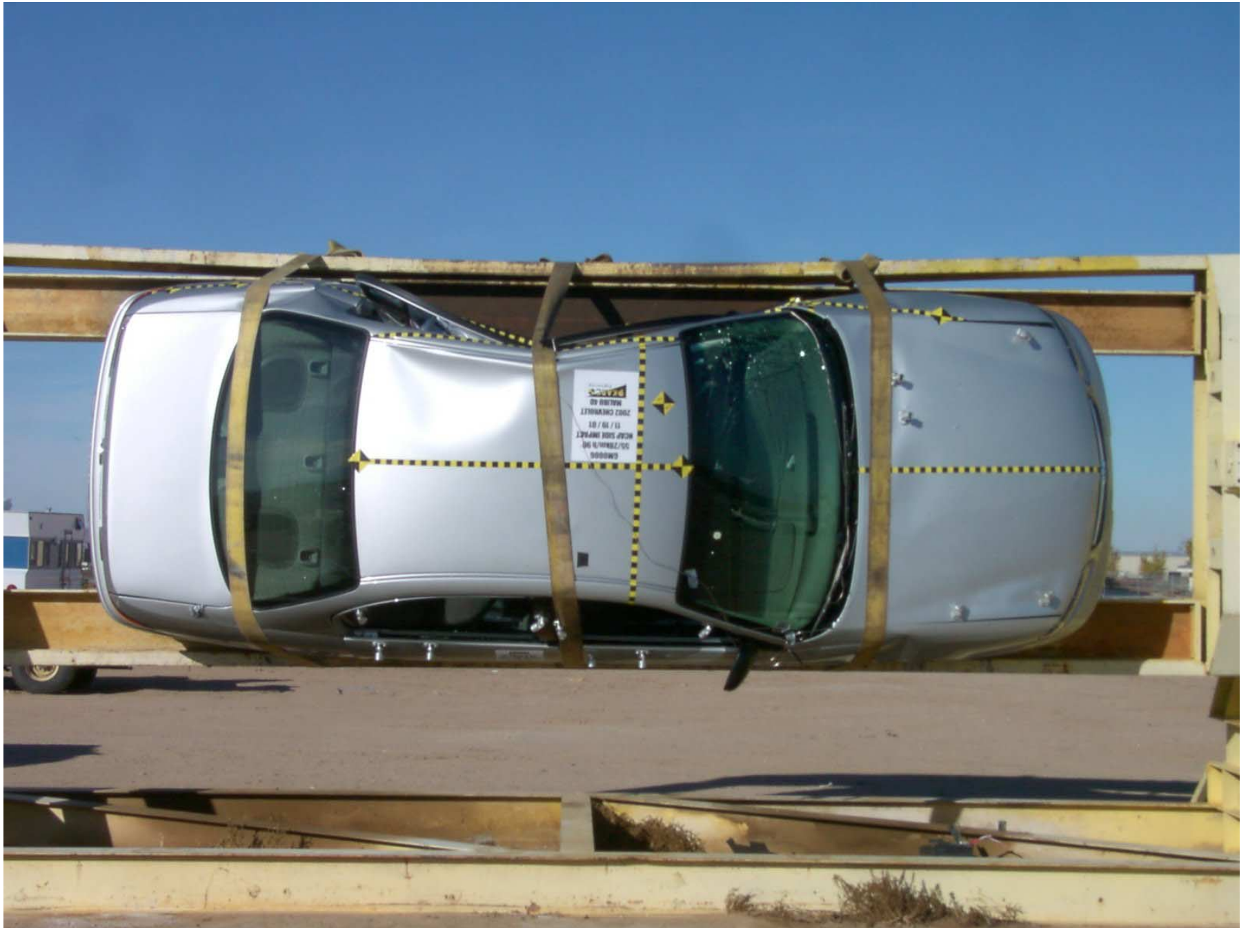
Figure A-48: Vehicle on Rollover Device, Top View
