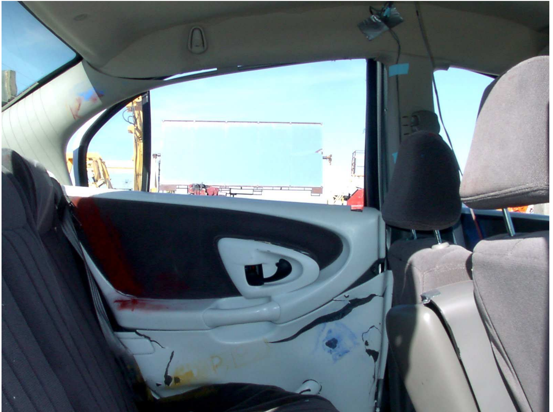
Figure A-39: Passenger Dummy Contact Points Inside View, Post-Test
